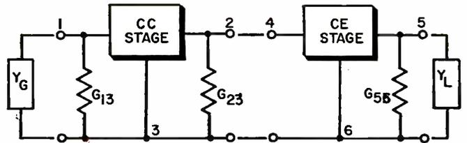
Fig. 7: Equivalent circuit of the three-terminal stages shown in Fig. 6.
