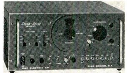
fixed frequency bands. Four ranges of sweep width are provided using 4 separate oscillator and sweep circuits. Other specs: sweep rate, 0.3-30 CPS in 3 ranges, 30 CPS, and line lock; sweep voltage, approx. 5.0 v. at low impedance out; r-f output: approx. 1.0 v. RMS into 70 ohms; audio, approx. 1.0 v. RMS into 600 ohms. Kay Electric Co., Dept. EI, Pine Brook, N. J.
