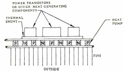
Fig. 3. Power transistor cooling device.
