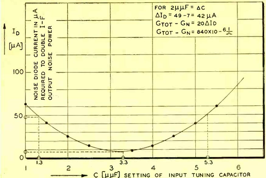
Fig. 2: Input conductance tuning curve is a parabola.
