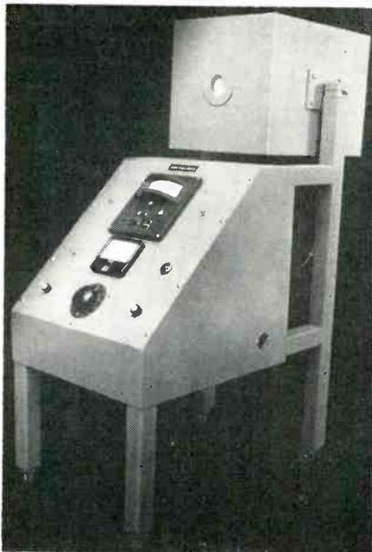
position at temperatures up to 1100°C. A clock motor is mounted for use in the growth of single crystals by the Bridgman technique. Furnace cores may be replaced within 2 min. while the furnace is still at temperature. A cast one piece insulation makes this a clean and simple operation. Replacement cores are supplied in wooden carrying cases. An anticipating controller, variac and ammeter are provided. Materials Research Corp., 47 Buena Vista Ave., Yonkers, N. Y.
