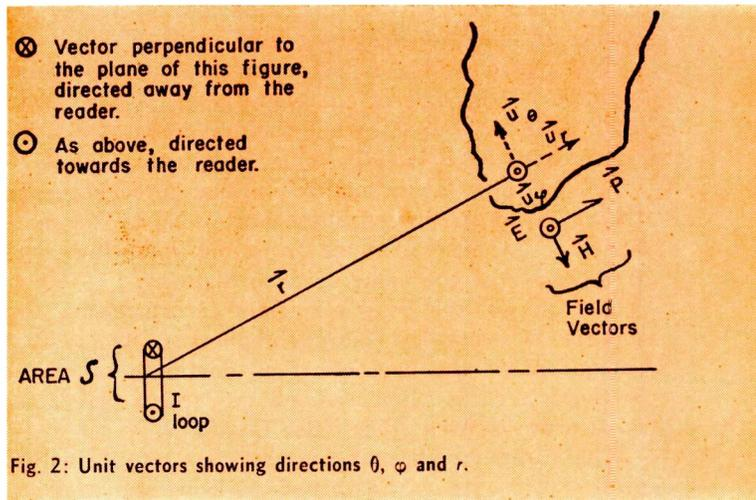
Fig. 2: Unit vectors showing directions  $\theta, \phi$  and  $r$ .
