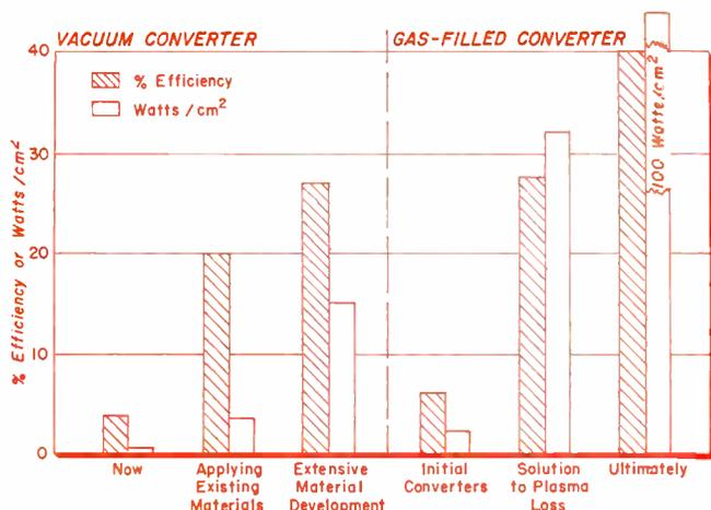
Fig. 17: The substantial research efforts of companies like General Electric (chart by Dr. Wilson of G.E.) indicate the "ultimate" column is feasible. At 40% efficiency, thermionic devices could effectively compete with conventional equipment.
