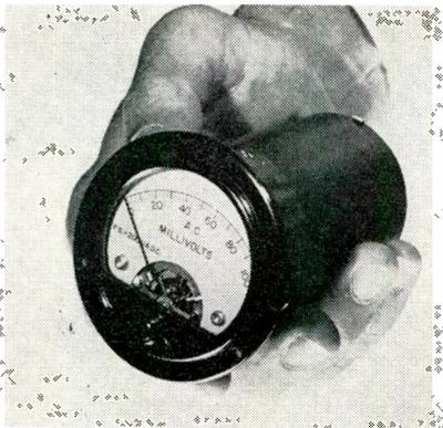
2 in. in dia. and less than 4¼ in. long. Basic range is 0. to 100 mv RMS. Input impedance is 1 megohm, parallel by 10 µmf adding almost no load to the circuit. It can be provided with any voltage range up to 300 v RMS. Frequency response is 20 cps to 20 KC, ±2%. Accuracy is ±3% of full scale deflexion. Metronix, Inc., Chesterland, Ohio.
