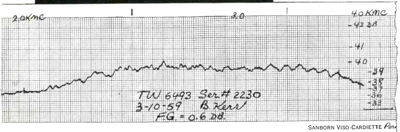
Actual strip chart recording of test on a production tube shows the uniform gain characteristics of this Sylvania tube over the 2.0 KMC to 4.0 KMC spectrum
