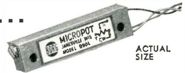
Borg Trimming Micropot® Potentiometers permit fine adjustments because of 40 turn lead-screw actuation. No hunting is required to make even the most critical adjustments. Settings remain stable. Unique contact carrier assembly drive prevents damage when either end of linear excursion is reached. Wide range of resistance values . . . 10 to 30,000 ohms. Other values on special order.
