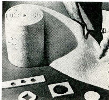
good tensile strength, density in the range of 20 lbs/cu. ft., good compression-deflection characteristics, useable temperature range -65°F to 500°F. It is available from pilot plant equipment in sheets ¼ in. thick, 9 in. wide and 6 ft. long. The Connecticut Hard Rubber Co., 407 East St., New Haven 9, Conn.
