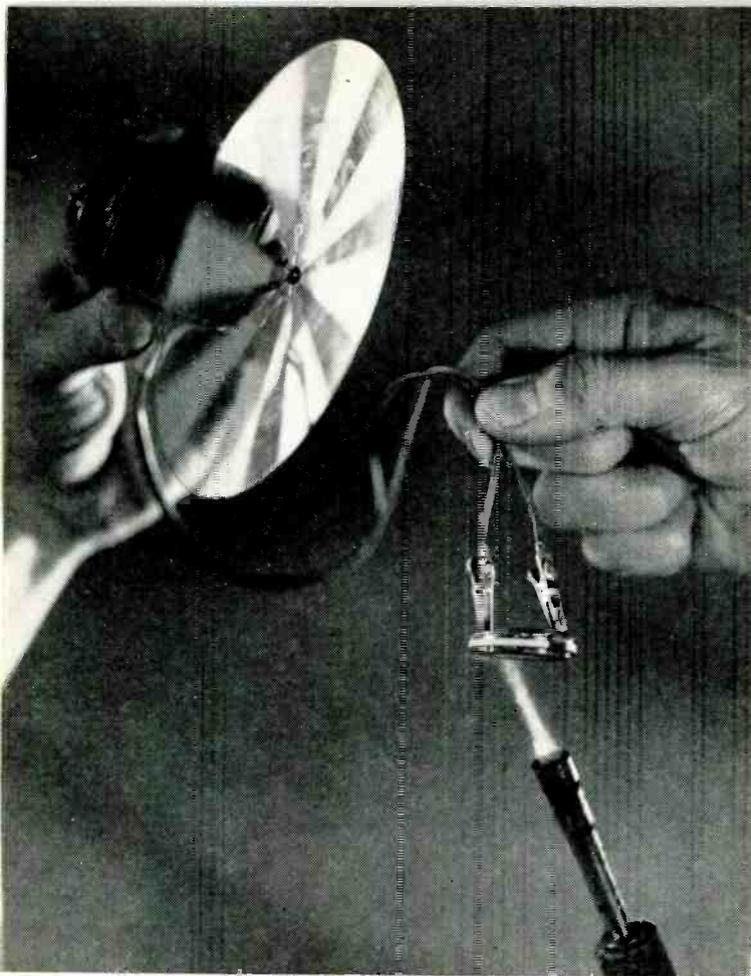
Fig. 15: Thermionic converter drives a small motor. Converter employs special cathode and anode materials which have appropriate "work functions". Electrodes are about 1/1000 inch apart. General Electric Research Laboratory.
