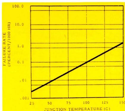
Fig. 1: Failure rate curve for the 2N6577.
