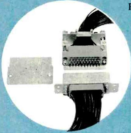
the all-important contact insulator block, for example . a *glass-filled* diallyl phthalate composition with high strength, lightweight, and excellent dielectric properties. Snap-in contacts stay put in the block and individually resist a rear axial pull of 20 lbs. . . . that's a CEC guarantee!
