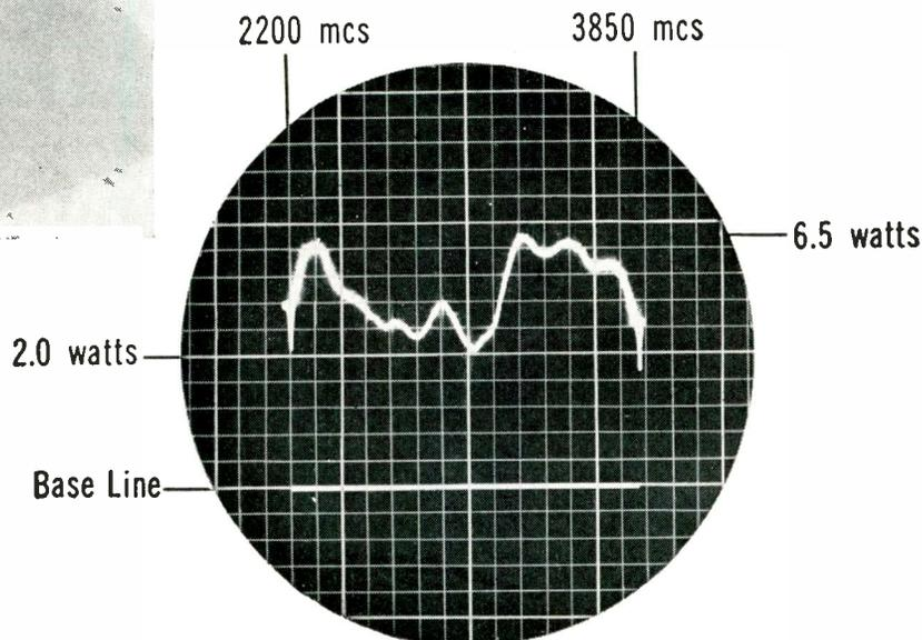
◀ Typical power — frequency of the GL-7398 shows power constant over the full band to within plus-or-minus 3 db.
