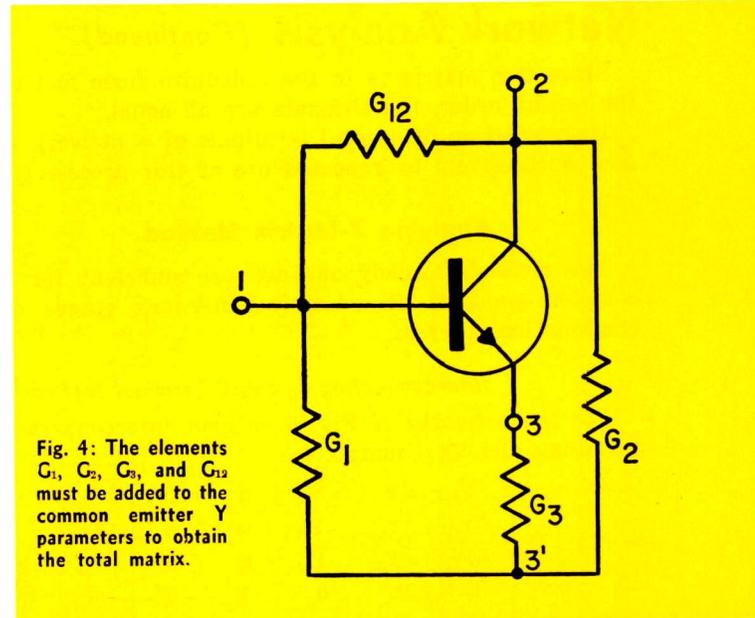
Fig. 4: The elements  $G_1$ ,  $G_2$ ,  $G_3$ , and  $G_{12}$  must be added to the common emitter Y parameters to obtain the total matrix.
