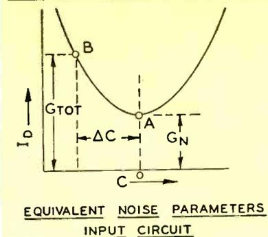
$G_n = 20 I_{D \text{ MINIMUM}}$  AT POINT A
