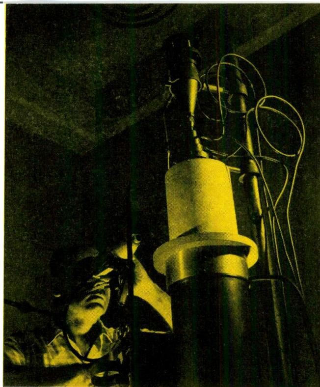
Fig. 10: Ceramic-type thermoelectric materials are prepared by Westinghouse in this special furnace (on a laboratory scale). Materials could operate in the 2000° to 3000° F range.
