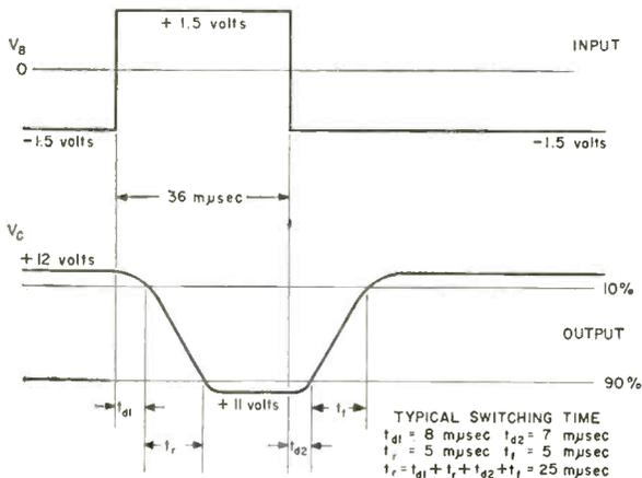
TOTAL SWITCHING TIME NON-SATURATED CIRCUIT
