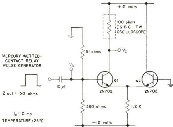
TYPICAL NON-SATURATED LOGIC SWITCHING CIRCUIT
