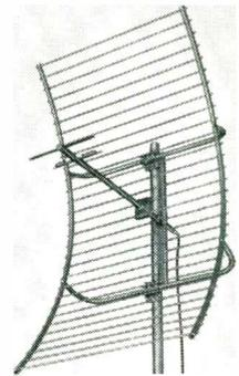
**PARAFLECTOR\*** performance equals that of a parabolic dish of the same aperture. Yet the Paraflector costs less, weighs only 25 pounds, and is easier to assemble and install. Basically a parabolic section in one plane, the rugged Paraflector withstands 100-mile winds with a 1/4-inch radial ice load. Driver is focused at the point source.
