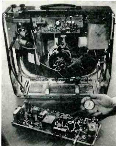
Loosening 3 screws, disconnecting 4 clip leads, and activating a spring loaded lever ejects the plated chassis board from Motorola's new TV set. Complete removal, or loosening for trouble shooting takes 33 sec.
