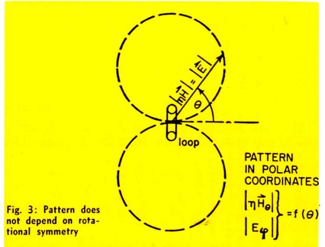
Fig. 3: Pattern does not depend on rotational symmetry
