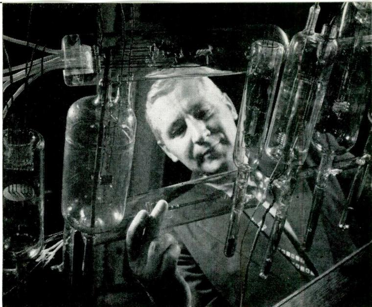
Fig. 3: Dr. Volney C. Wilson, G.E. physicist, inspects one of the experimental thermionic converters he developed. Research aims at efficiencies of over 30% for these devices.
