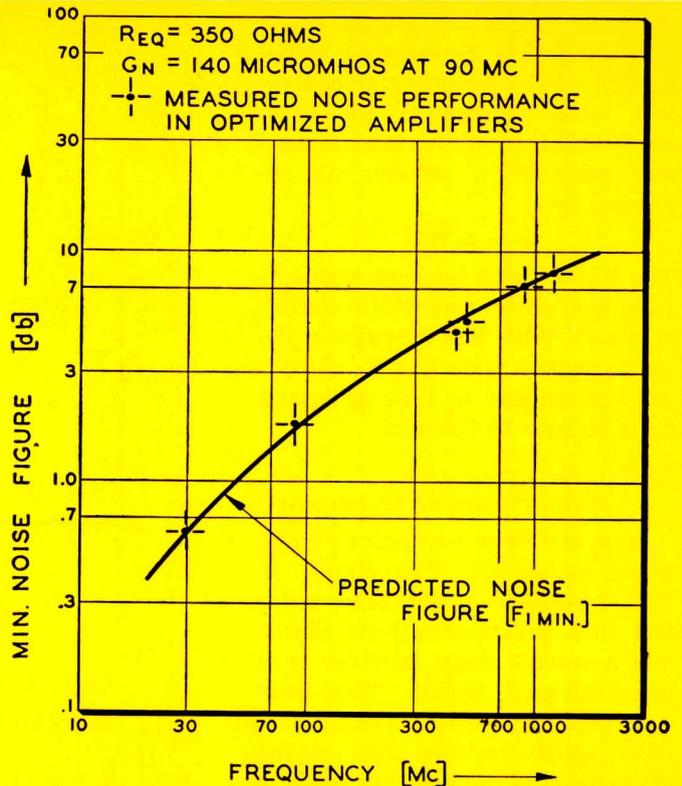
Fig. 5: Measured values agree with predicted values for G.E.'s 7077 tube.
