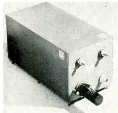
acteristics of the new Dual Delay Line are as follows: Delay, 1 to 1.5  $\mu$ sec.; independently variable in each channel in increments of 0.05  $\mu$ sec.; impedance—1000 ohms; output rise-time—0.06  $\mu$ sec. per channel; dimensions—8 x 4 x 4 inches. ESC Corporation, 534 Bergen Boulevard, Palisades Park, New Jersey.
