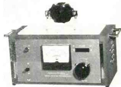
breakdown tests of insulating oils may be made where the equipment is located. Test voltage is continuously adjustable from 0 to 35 kv ac at a 2 kva rating to meet ASTM and Federal specs. Measurement of test potential is made directly at the test electrodes to assure accuracy. Set operates from 110-120 vac. Associated Research Inc., 3777 W. Belmont Ave., Chicago 18, Ill.
