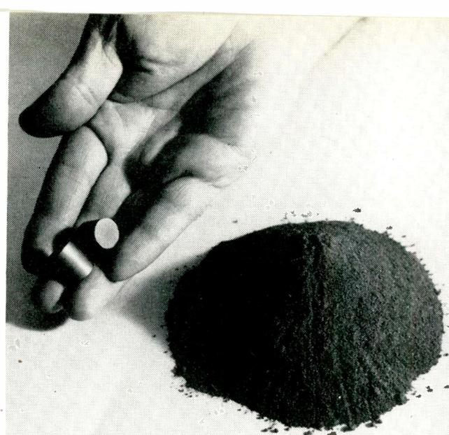
Fig. 19: Powdery "mixed-valence" compounds are pressed into pellets for thermoelectric use. Materials are abundant, relatively inexpensive, and can be used at high temperatures. Westinghouse Electric Co.
