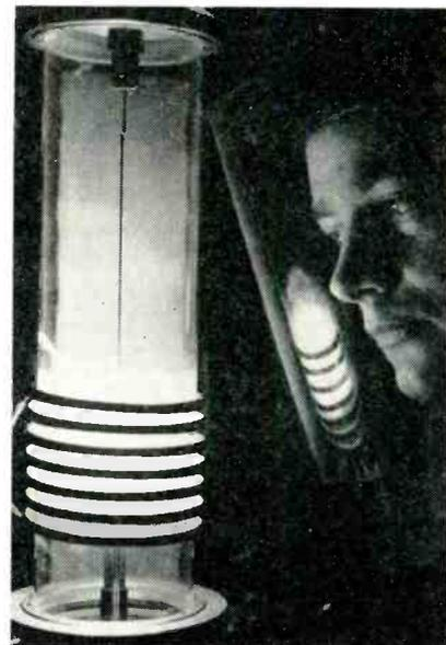
Westinghouse's J. J. Coleman watches ribbon-like germanium crystal rise from a molten pool in this furnace at the Company's Research Labs. Strips require none of the costly, cutting and grinding that wastes up to 80% of conventional ingots used in semiconductor device fabrication.
