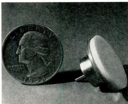
Fig. 2: High vacuum thermionic converter has special ceramic insulators developed by the General Electric Co. Coefficient of expansion of metal and ceramic parts are the same. Device operates from any heat source, nuclear or conventional.
