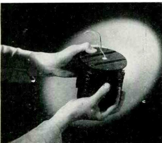
Fig. 6: 5 watt TE generator built by Minnesota Mining and Manufacturing Co. is about the size of a qt. fruit jar. Efficiency is about 6%. Cooled by air it uses an isotope heat source. Semiconductors used here are in pilot plant production.
