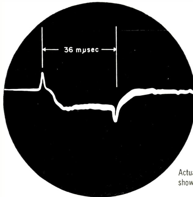
Actual photo of collector wave form as shown on traveling-wave oscilloscope
