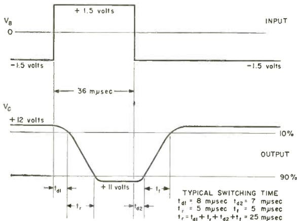
TOTAL SWITCHING TIME NON-SATURATED CIRCUIT
