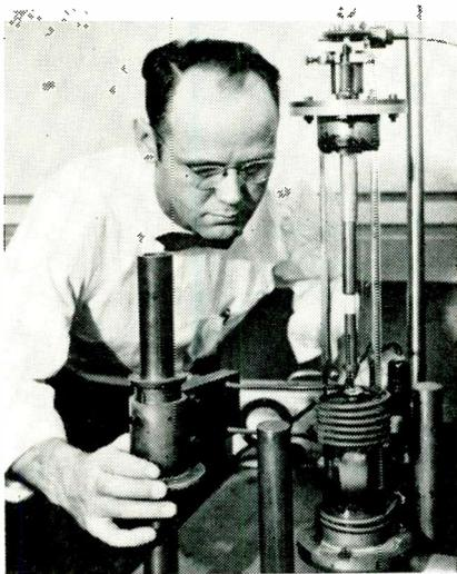
Fig. 13: Research scientists at the National Bureau of Standards use this furnace to grow large single crystals by the Kyropoulos technique. The crystals are used to study the thermoelectric (and other) properties of materials.
