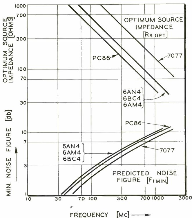
Fig. 6: Predicted min. noise and optimum source impedance for several tubes.
