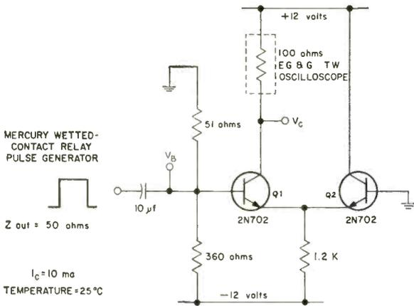
TYPICAL NON-SATURATED LOGIC SWITCHING CIRCUIT
