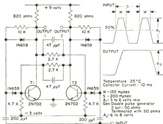
TYPICAL CIRCUITRY FOR OBTAINING 5-MC REP RATE
