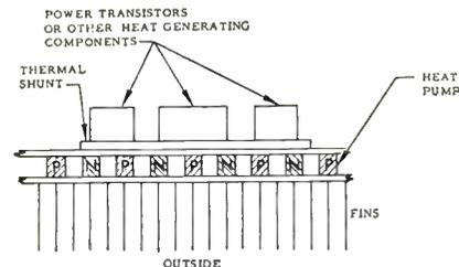
Fig. 3. Power transistor cooling device.
