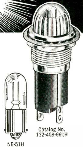
In the DIALCO assembly, the built-in current limiting (ballast) resistor (18,000 ohms) is completely insulated in moulded bakelite and sealed in metal (U. S. Patent No. 2,421,321) ... Small space required—units are available for mounting in 9/16" or 11/16" clearance holes ... A wide choice of optional features includes lens styles, shapes, and colors; terminal types; metal finishes, etc. ... Meet applicable MIL Spec and UL and CSA requirements.
