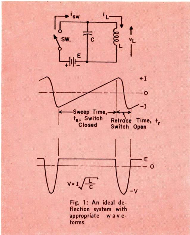
THE transistor, in some respects, is well suited to providing a linear current sweep for horizontal deflection. Its ability to act as a bilateral switch, i.e., conduct in both directions, and its relatively high efficiency as such, are two advantageous properties.
