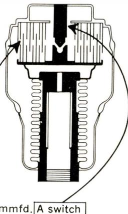
Jennings capacitors are obtainable either fixed or variable and since there is no dielectric to puncture they are self healing after moderate arc-over.
