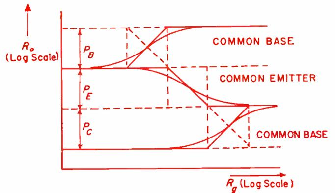
Fig. 9: Configuration of asymptotes for output resistance vs. generator resistance follows a similar pattern to that shown in Fig. 4.
