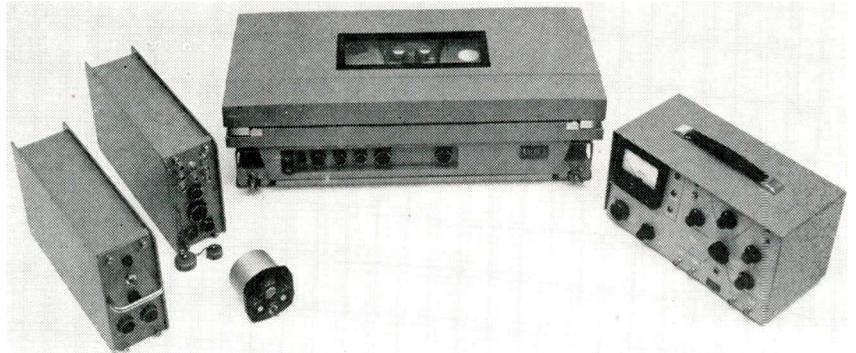
The complete recorder system includes, from left to right, a power converter, electronics box, the remote control unit, the AR-200 tape transport, and a test unit.
