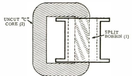
Fig. 2: Split bobbin fitted on the core.
