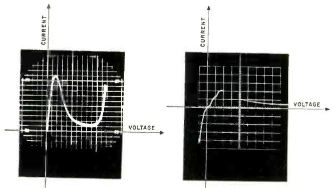
"Wiggles" in performance curve of tunnel diodes prove that ultrasonic vibrations of the crystal are involved in tunneling process
