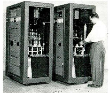
series of modulators is applicable for tube development work or for incoming tube inspection by equipment manufacturers. Combined with traveling-wave tubes, the units become broadband high-power pulsed microwave amplifiers; or, with klystrons, narrow-band systems. Booth 305. Levinthal Electronic Products, Inc., Stanford Industrial Park, Palo Alto, Calif.
