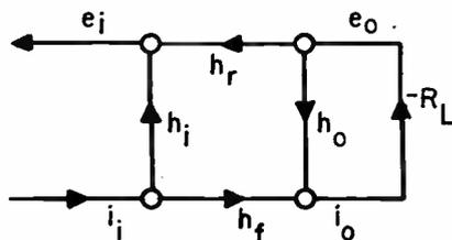
$$R_i = \frac{h_i - (h_i h_o - h_r h_f) R_L}{1 + h_o R_L} \quad (2)$$
