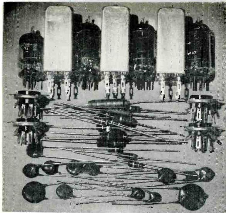
Functions of all these components can be handled by "tunnel diode"
