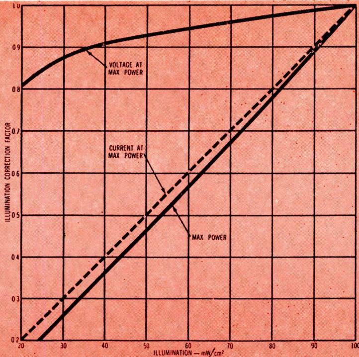
Fig. 5: Typical variation of power, voltage and current at maximum power output versus incident solar radiation
