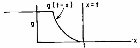
This function is illustrated in Fig. 3; it is seen to be analogous to closing a switch.
