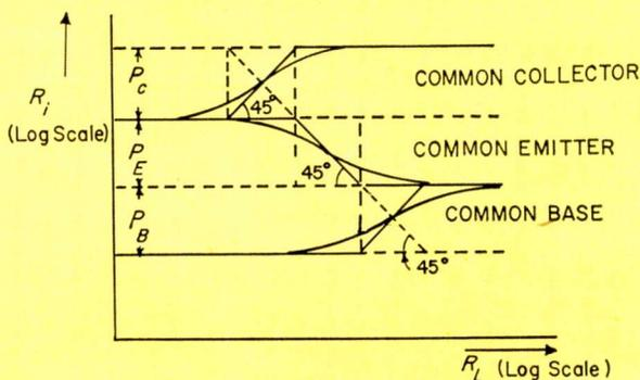
Fig. 5: A practical case of asymptotes and curves for a transistor.
