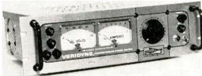
puts can be used as either positive or negative supply. Provision is made for remote sensing so that supply values can be determined at the load. Input is a standard 2-conductor receptacle. Output is through jacks (front panel) or terminals (rear of the chassis). Ripple in the "Z" series is under 1 mv; the "W" version is below 5 mv. Both types available in 2, 5, 10 and 15 max. output. Consolidated Diesel Electric Corp., 880 Canal St., Stamford, Conn.
