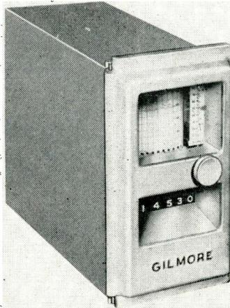
readout. It indicates and records forces, fluid flow, weights, or rpm's which can be converted into ac or dc mv. and eliminates errors due to parallax and interpolation of readings. It has a permanent recording chart. Dimensions: 6 x 1 1/8 x 12 in. Digital readout accuracy: 1/10 of 1%; chart accuracy is ±1%. Gilmore Industries, Inc., 13015 Woodland Ave., Cleveland 20, Ohio.
