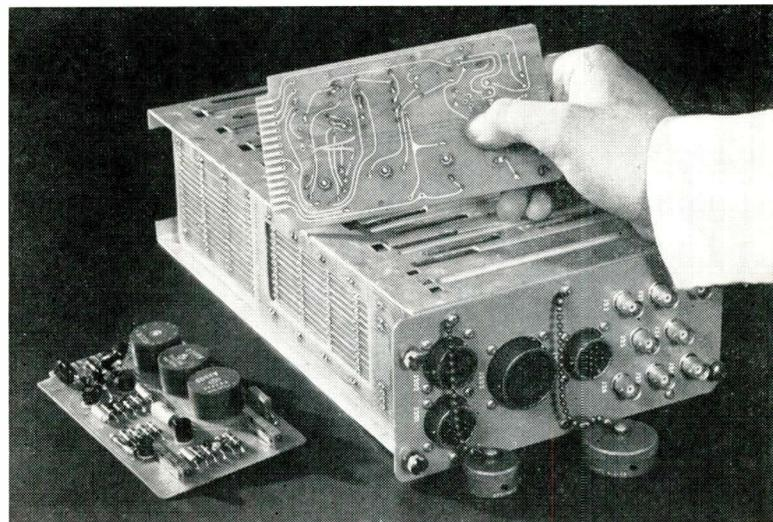
Solid-state devices and etched-board circuitry makes the electronic section of the new mobile recorder a compact unit
