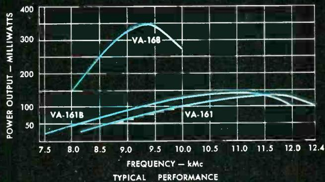
Varian X-band BWO's are now the standard of the industry for systems requiring long life, low voltage operation, and small size. Characteristic of Varian BWO's is a uniform power output and helix voltage relationship with frequency. The metal and ceramic construction offers the most reliable tube at the lowest cost and assures dependability in severe environments.
