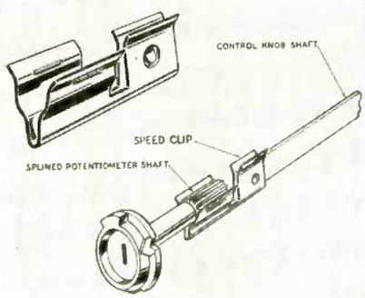
snapped into the U-shaped end of the speed clip where it is locked in position by a spring tab. The splined potentiometer shaft can then be inserted by pressing it between the semi-tubular spring legs, or by sliding it into the open end. Once the potentiometer has reached its turning limits, further turning of the knob results only in slippage of the clip. Tinnerman Products, Inc., Cleveland, Ohio.
