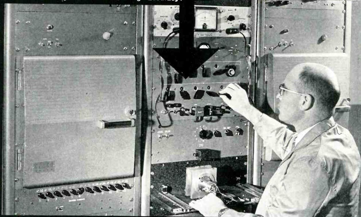
This Test Stand handles 12 units simultaneously, all temperature compensated to -55°C to +150°C. Also tests output voltage, phase shift and linearity. Test Stand has a speed accuracy of .01%, transformation accuracy of .001% and phase shift accuracy of 2 minutes.
