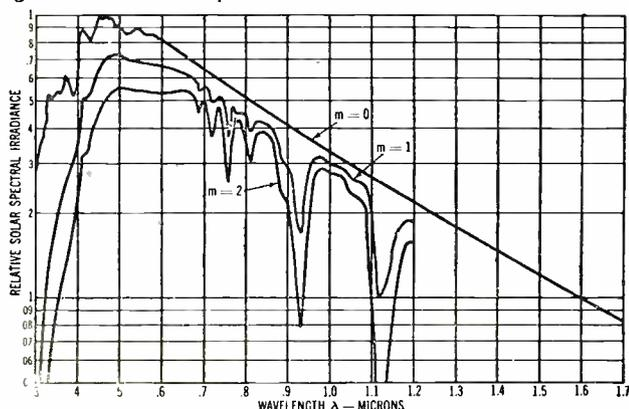
Fig. 8: Relative spectral response of short circuit current for solar radiation (uncoated cell), at three air masses
