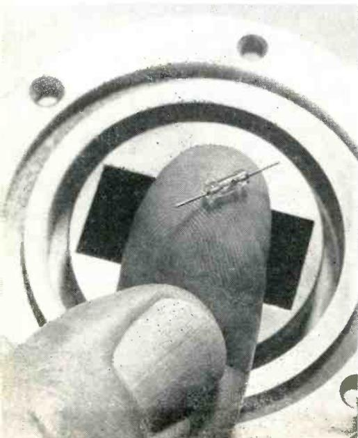
Laboratory comparator magnifies the inner structure of this gold-bonded diode.
