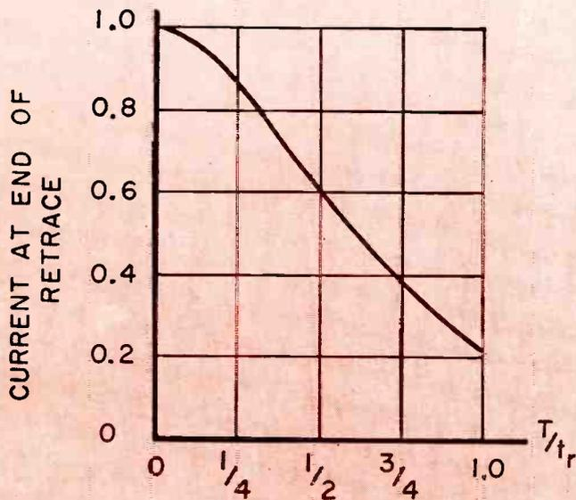
Fig. 5 (above): The value of the yoke current at the end of the actual retrace period is plotted as a function of switching speed.
