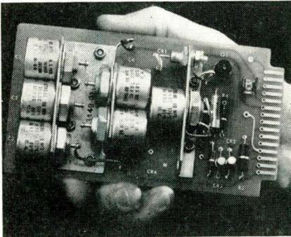
This view of the regulator reference board, part of the electronic unit, shows method of mounting some of the components.
