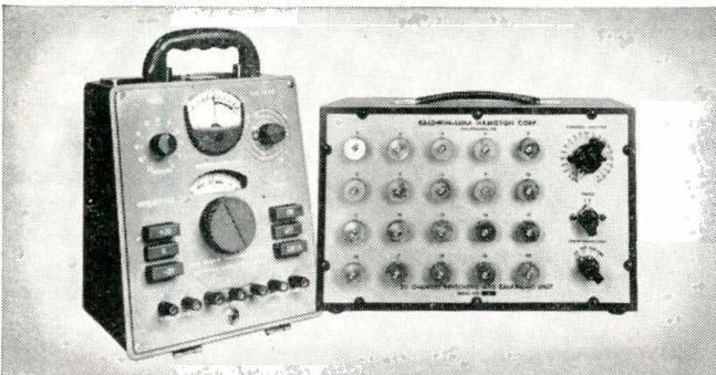
A full line of strain instruments—for static and dynamic strain measurements—is available through your B-L-H Sales-Engineering Representative. Instruments include (left) the B-L-H Type N Strain Indicator, calibrated to read directly in microinches per inch; (right) B-L-H switching and balancing unit, designed to facilitate bridge balancing and gage readout on multiple gage installations.
