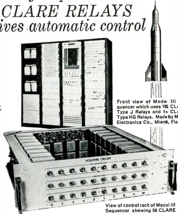
Front view of Model III Sequencer which uses 762 CLARE Type J Relays and 14 CLARE Type HG Relays. Made by Milgo Electronics Co., Miami, Fla.
