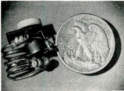
Complete transmitter using tunnel diode
