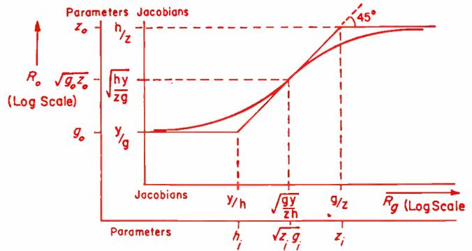
Fig. 6 (left): Common emitter curve and asymptotes for output resistance vs. generator resistance.
