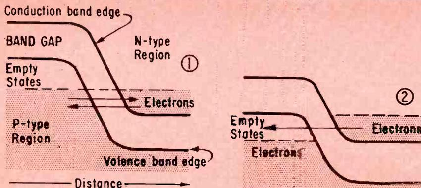
Fig. 1 (far left): Electrons at same level on both sides of junction. No net current.
