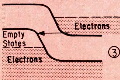
Fig. 4: Electrons are all opposite forbidden gap. Very small current is flowing.
