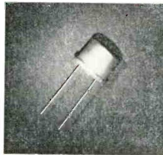
THE tunnel diode, first reported in 1958 by Japanese scientist Leo Esaki, is first cousin to a transistor, but operates on a different principle and offers advantages that the transistor does not. Before long it should find its way into high-speed computers, television sets, communication equipment, nuclear controls, satellites and space vehicles, according to Dr. Guy Suits, GE Vice President and Director of Research.
