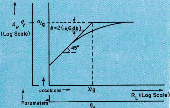
Fig. 13 (above): Relationship of voltage gain and load resistance.
