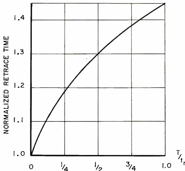
Fig. 9: Increase in retrace time due to decrease in switching speed.
