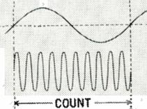
Frequency ratio measurements
