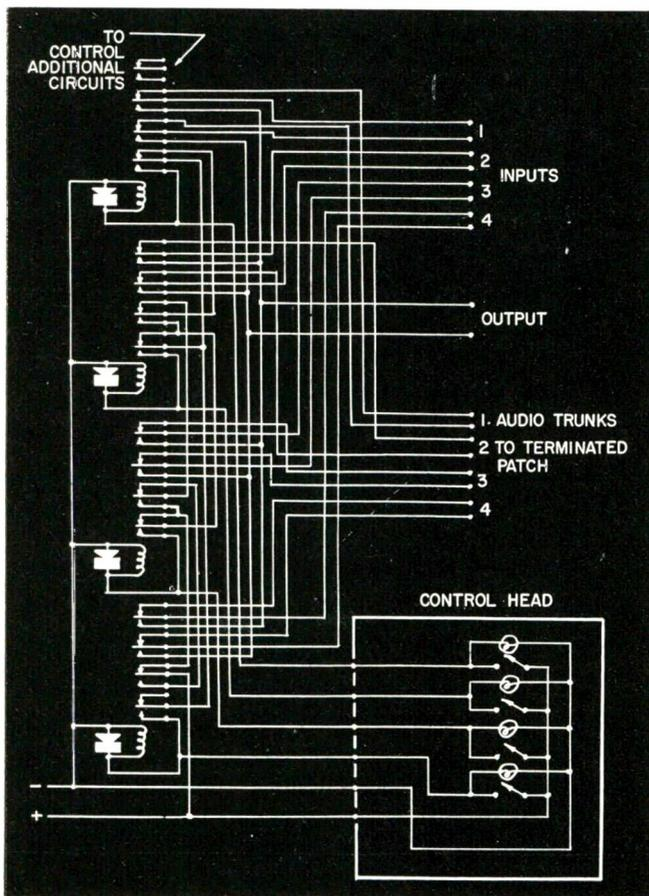
Fail-safe is provided for this switching system by feeding the audio from each program relay, when off, to a terminated patch. Manual switching is then available and the trunks are kept correctly loaded.
