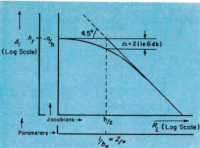
Fig. 12 (above): Sketches for current gain vs. load resistance.
