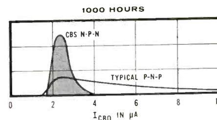
The superiority of CBS NPN transistors is achieved by special processing: For example, advanced surface chemistry techniques seal out moisture and contamination. Precise control of alloying produces high back voltages. Thorough bake-out stabilizes gain. The result is reliable NPN computer-type switching transistors featuring fast switching . . . high voltage . . . low cutoff current . . . and low saturation resistance . . . in a welded JETEC TO-9 package
