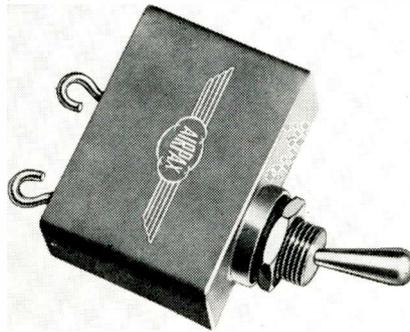
of ambient or operating temp. Units available for interrupting 50dc volts at currents from 0.05 to 10 amperes and for interrupting 120 RMS volts, 60 to 400 CPS at currents from 1.0 to 10 amperes. The toggle handle of the breaker is similar to conventional on-off switches. Booth 521, Airpax Electronics Inc., Cambridge Division, Cambridge, Maryland.
