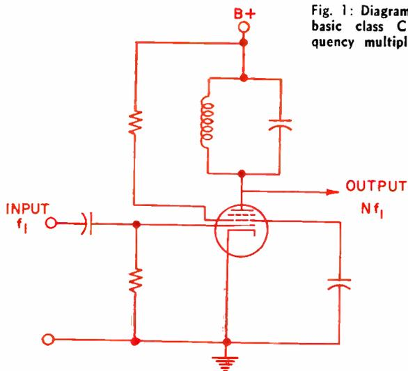
Fig. 1: Diagram of a basic class C frequency multiplier.
