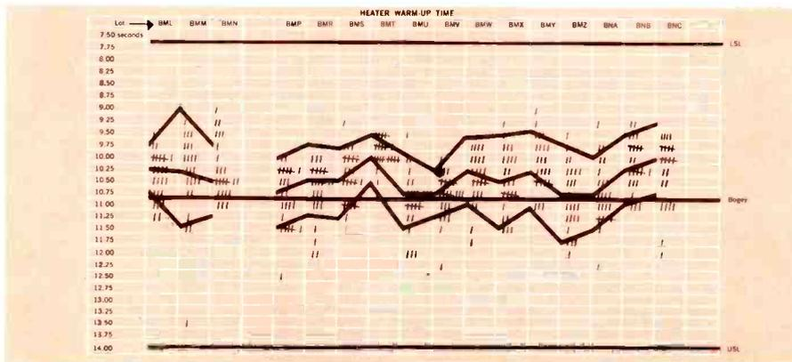
Picture of Reliability—Actual graph of mixed variable-attribute inspection shows how individual tube lots meet a particular specification
