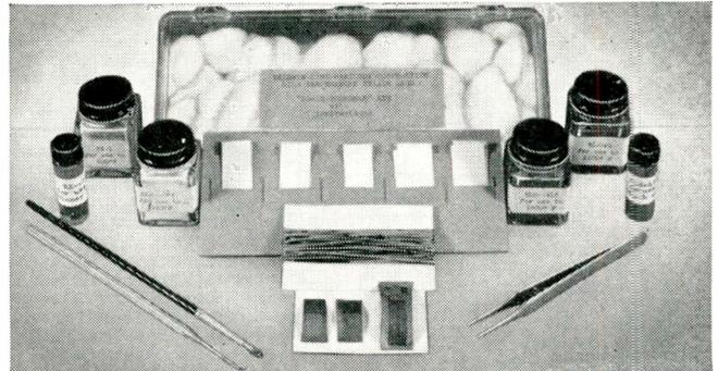
The proper application of a strain gage to a surface is fundamental in obtaining accurate strain data. B-L-H cements, solvents, waterproofing and lead materials and accessory equipment help you do the job right. Convenient strain gage application kits contain everything you need, including detailed instructions. Kit materials can also be supplied in bulk form in large or small quantities to suit your needs.
