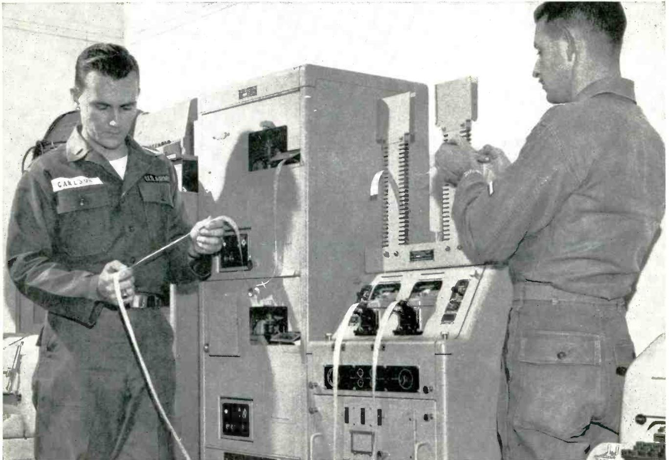
**At U.S. Army field communications centers, Kleinschmidt torn tape relay units send, receive, retransmit messages to widely-dispersed commands**
