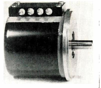
All joints and screw holes are sealed with a rubber potting compound on this humidity resistant Potentiometer. Teflon shield creates moisture barrier for shaft.
