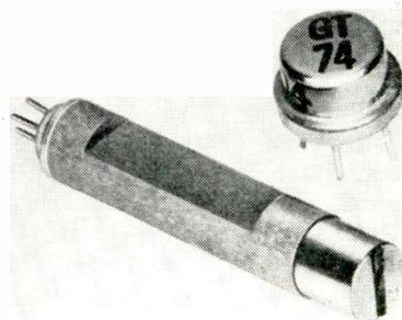
can be mounted so that the gaps of two adjacent heads are only 0.150 apart circumferentially, making the head ideal for close recirculating registers. The heads are low inductance for efficient transistor driving. Mechanically the diameter of the head is only 0.216 with an overall length of 1.062. The head is available with shielded and jacketed cable. Magne-Head Div., General Transistor Western Corp., 2660-64 So. La Cienega Blvd., Los Angeles 34, Calif.
