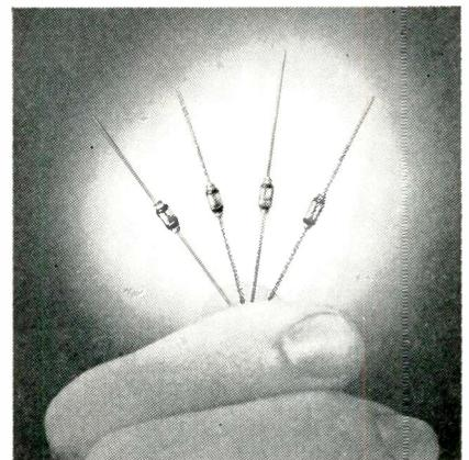
Major step in the trend to ever smaller radar and microwave equipment to meet today's military and commercial demands is represented by Sylvania's new line of subminiature Micro-Min diodes. The new diodes meet the electrical performance of their larger counterparts and are equivalent in ruggedness and reliability. They combine in one unit Sylvania's unmatched experience in diode packaging and proven technical excellence in microwave diode design.
