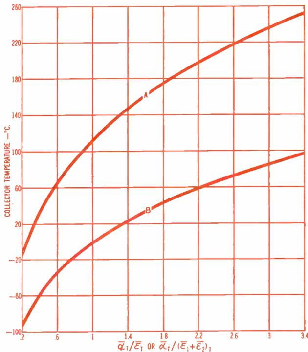
Fig. 9: Surface temperature of solar collectors in space
