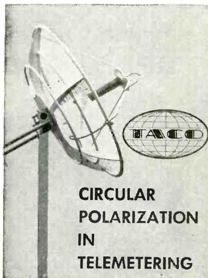
Telemetering antenna systems available for all bands—215-265, 940-980 mc. Gain up to 26 db. Either wide or narrow beam. Single or tri-helical models, and single helical feeds utilizing parabolic reflectors of 6, 8, or 10-foot diameters.
