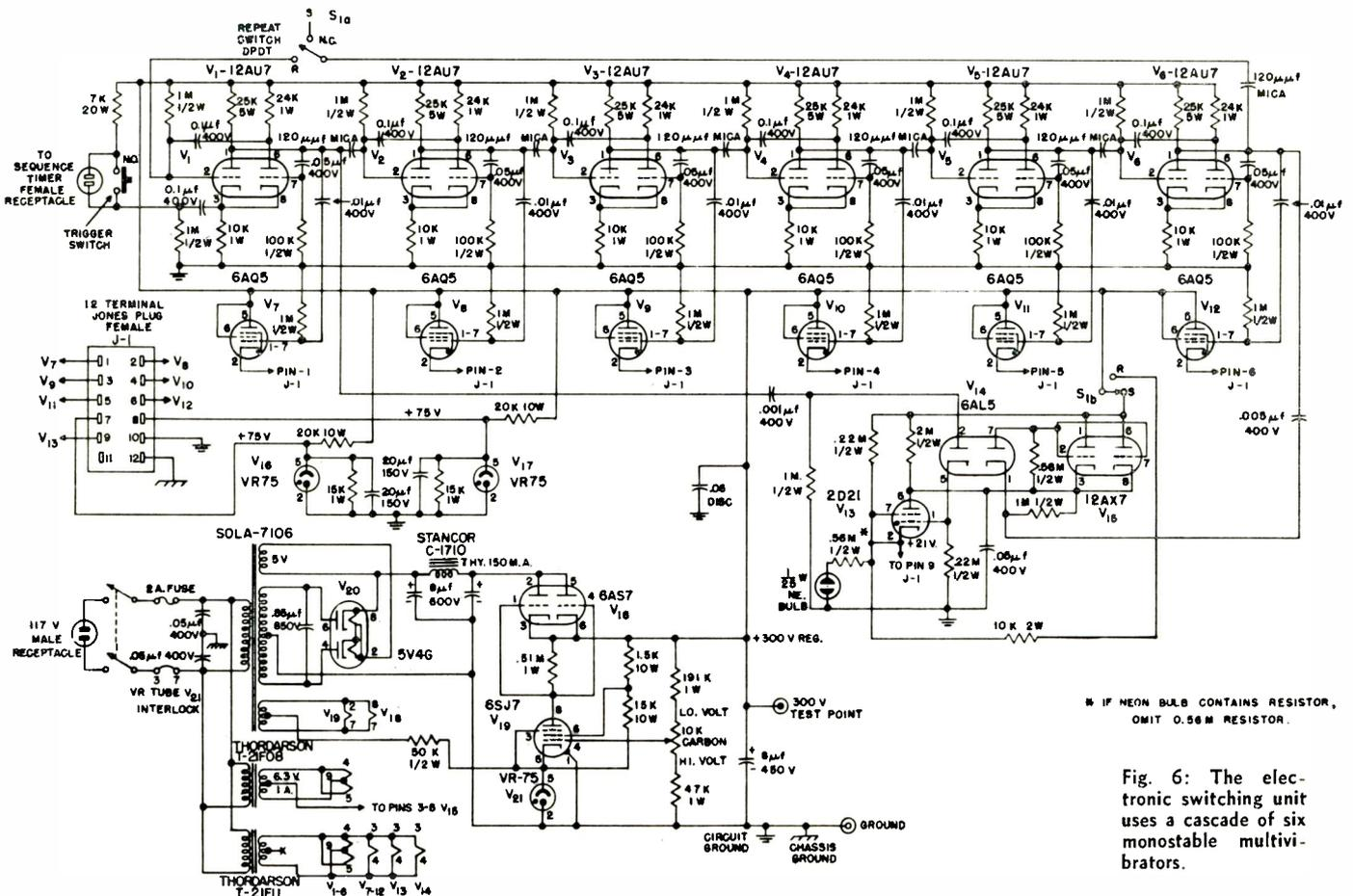
Fig. 6: The electronic switching unit uses a cascade of six monostable multivibrators.
