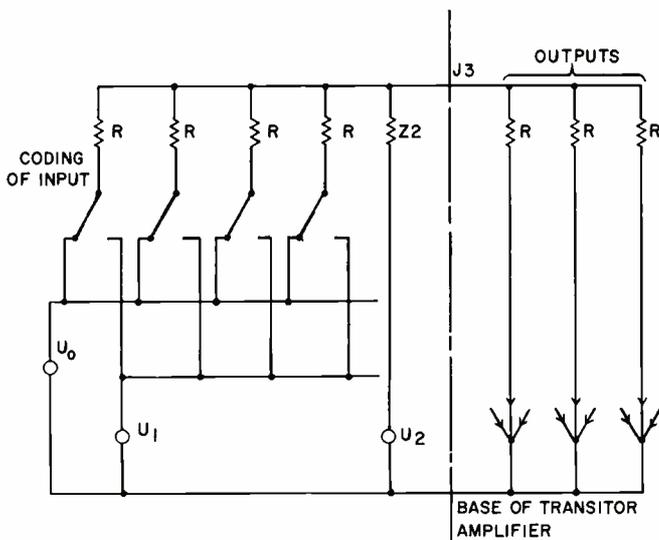
Fig. 7a (left): Logic of linear network, basic circuit; while Fig. 7b (below) illustrates an equivalent circuit
