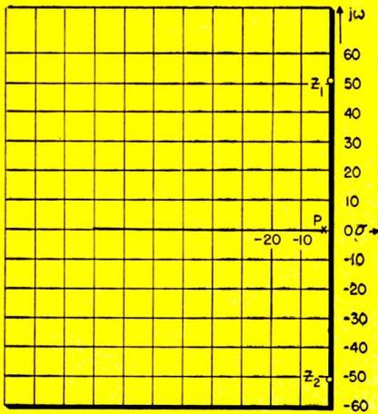
Fig. 7: Pole-zero plot of impedance plot which realizes  $h_{11}/h_{12}$ .
