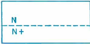
Fig. 10: Industrial bars are doped so that slices include N and N+ germanium.
