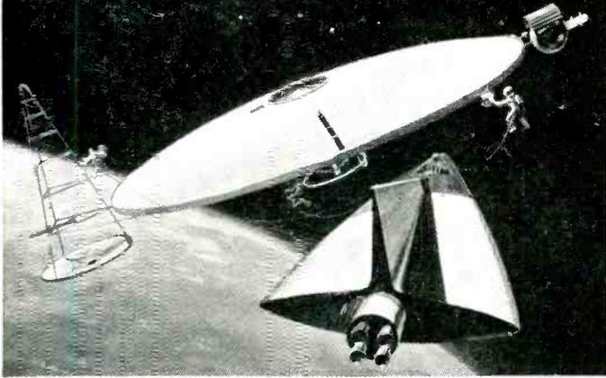
**MARS VEHICLE.** Drawing, based on Boeing study, of space vehicle designed for launching from orbiting platform for reconnaissance flight to Mars and return. Lunar, orbital and interplanetary system studies, and expanding programs such as the advanced Minuteman solid-propellant ICBM, are typical of challenging, long-range assignments Boeing offers electronic-electrical engineers.
