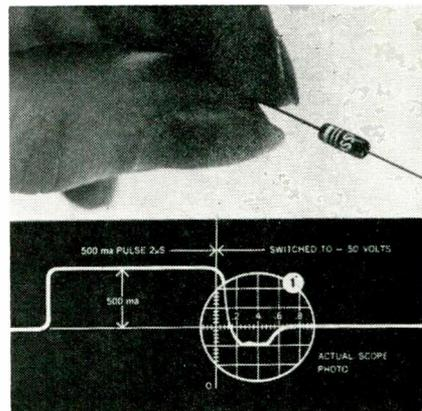
ance (400 ma at 1 v.) and low leakage (50  $\mu$ a at 150°C). Units feature a max. recovery time of 0.8  $\mu$ sec to return to 10K ohms when switched from a forward current 2  $\mu$ sec pulse of 500 ma to a reverse voltage of -50 v., with a loop impedance of 1K ohm. Typically, they switch from a 5 ma forward pulse to -40 v. (-30 v. for 1N690 diode) and recover to 100K ohms in 0.5  $\mu$ sec. ( $R_i = 2k$ ,  $C_i = 10 \mu$ mf). Sperry Semiconductor Div., Sperry Rand Corp., So. Norwalk, Conn.
