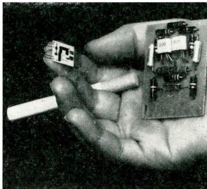
Miniaturized module makes it possible to pack five times more electronic gear in the nose cones of missiles.
