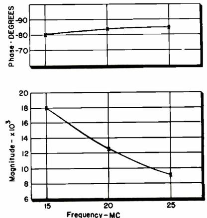
Fig. 8: Magnitude and phase shift of impedance represented by pole-zero plot of Fig. 7.
