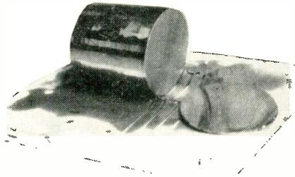
Fig. 1: Germanium crystal is shellac-mounted on tile for easy diamond saw slicing. One of the slices is on the right.
