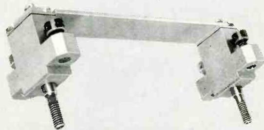
**HYDRAULIC STOP** A minimum size buffer used in a ballistic missile device to prevent inadvertent operation through handling shock. Provides tremendous damping force for its size.
