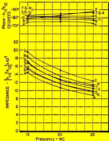
Fig. 6: Magnitude and phase plot for  $h_{11}/h_{12}$  over a 10 MC band.
