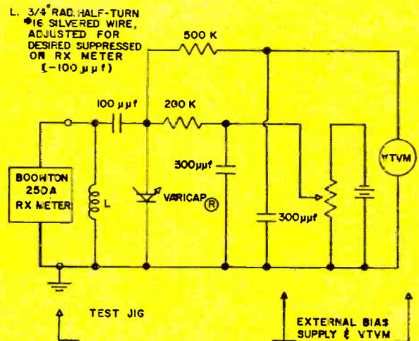
VALUES INDICATED ARE FOR 50 MC TESTS FOR CAPACITANCES UP TO 170 μf
