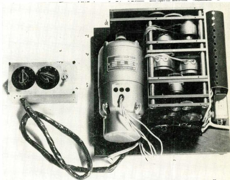
measure  $4\frac{1}{4}$  in. in width,  $7\frac{1}{4}$  in. in length and is only  $3\frac{5}{8}$  in. high. Torque developed at the various speeds range from 50 oz.-in. to well over 100 oz.-in.
