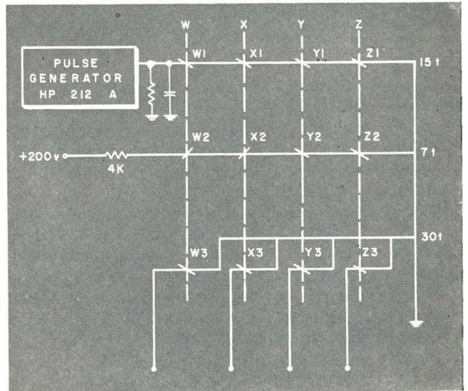
Fig. 2: Drawing shows magnetic drivers for diode matrix input
