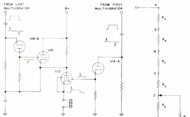
Fig. 7 (above): Simplified diagram of the calibration schematic circuit is shown
