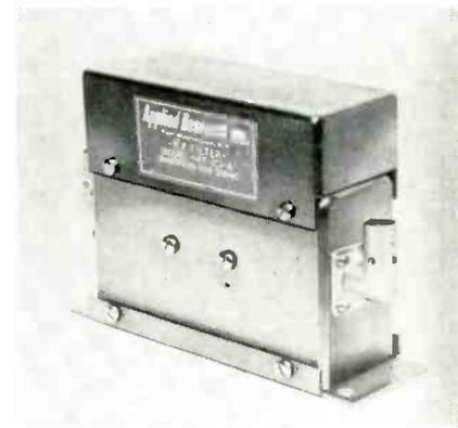
They are aligned to obey the Butterworth condition, and have a low insertion loss. Typical unit operates at 332 MC with 3 db bandwidth of 24 MC. With this center frequency, weight of the filter is 20 ounces. Dimensions are 5½ in. x 1 11/16 in. x 3¼ in. Applied Research Inc., 76 South Bayles Ave., Port Washington, N. Y.
