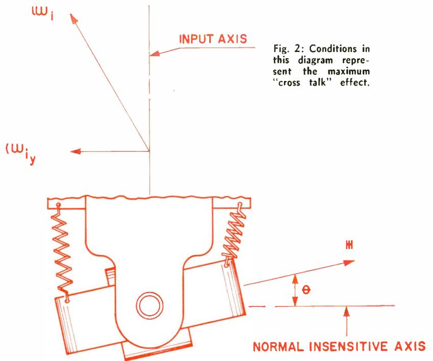
Fig. 2: Conditions in this diagram represent the maximum "cross talk" effect.
