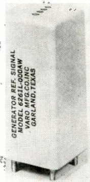
It has an output of 2.5 v. with frequencies from 300 to 4000 CPS at accuracies of 0.1% to 0.01%. Fork and oscillator are in a hermetically sealed can. Varo Mfg. Co., Inc., 2201 Walnut St., Garland, Tex.
