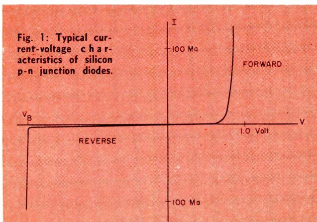
Fig. 1: Typical current-voltage characteristics of silicon p-n junction diodes.
