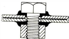
Finishing Washers are popular for use on the surface of finished panels as they lessen the possibility of scratched finishes.
