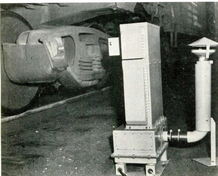
Foolproof detection is provided through unique temperature sensing and comparison mechanisms; thermocouple is used in place of a bolometer.
