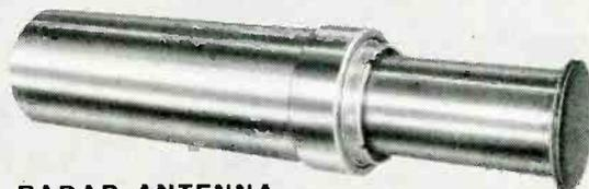
**RADAR ANTENNA LIMIT STOP** Designed and built for Project BMEWS, this buffer limits the travel of 85-foot diameter radar antennas. By absorbing the energy of extreme shock loads it prevents damage by high windage, failure of electrical system or other malfunction. Filled with silicone fluid for uniform performance at all temperatures. Capable of being mounted in any position.
