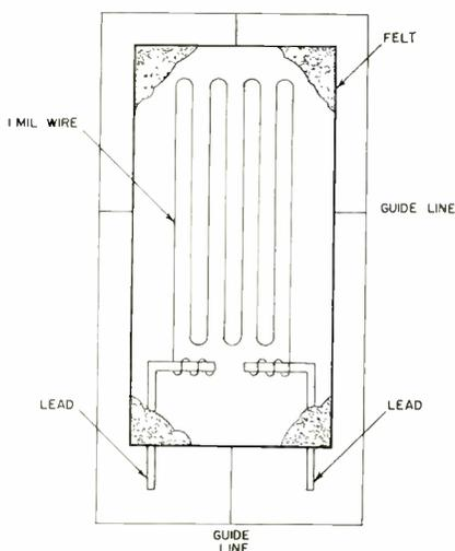
Fig. 3: This British invented strain gage element is made of foil.
