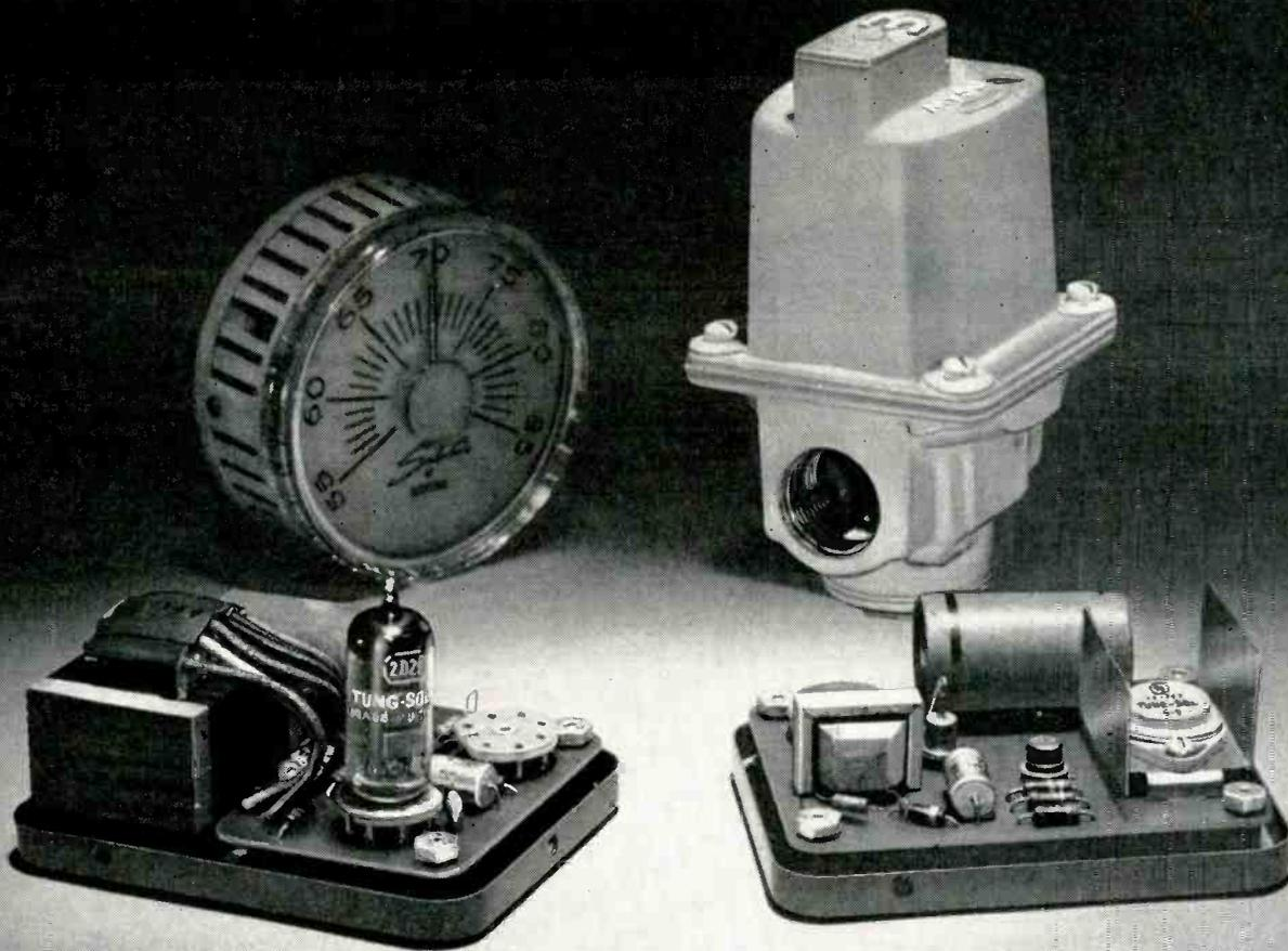
End alternate chills and hot blasts. Shown in front of the thermistor wall unit and the furnace modulator valve are the tube type and transistorized amplifiers for the new Selectra home gas furnace control now in production at Maxitrol Company, Detroit, Michigan.
