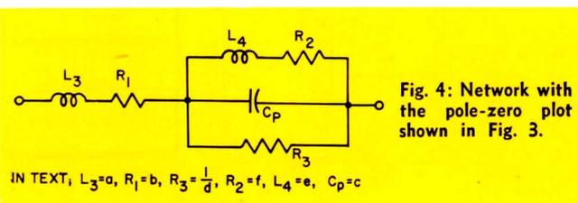
Fig. 4: Network with the pole-zero plot shown in Fig. 3.
