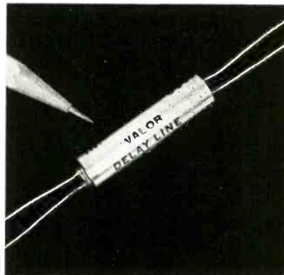
sistor applications. Specs: characteristic impedance 1400 ohms; attenuation 3%; temp. characteristic  $-0.03\%/^{\circ}\text{C}$ ; temp. range  $-55^{\circ}\text{C}$  to  $+105^{\circ}\text{C}$ ; built to MIL specs; molded in hermetically sealed brass tube with leads brought out through glass-to-metal end seals; case finish—fused tin plate. Valor Instruments Inc., 13214 Crenshaw Blvd., Gardena, Calif.
