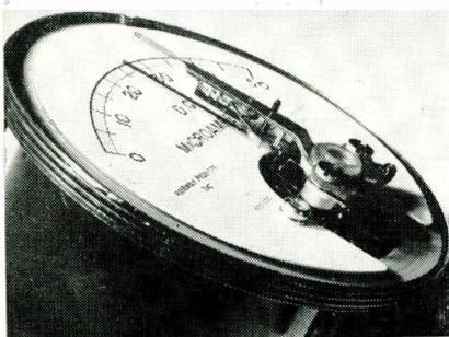
(Left) Control action begins when a round vertical contact on the indicating pointer meets a flat contact on the toggle mounted beneath adjustable pointer.
