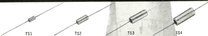
**TS1**, size: .125" x .250", .33mfd/35v to 6.8 mfd/6v . . . **TS2**, size: .172" x .438", 4.7 mfd/35v to 56 mfd/6v . . . **TS3**, size: .279" x .650", 15 mfd/35v to 180 mfd/6v . . . **TS4**, size: .341" x .750", 27 mfd/35v to 330 mfd/6v.
