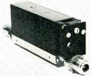
ing; in-line shaft adjustment; and direct reading, calibrated dial. Specs include: frequency band, available band widths from 4-7 to 7-11 KMC; attenuation variation with frequency less than ±5% expressed in db; VSWR on all settings less than 1.5; power handling capacity, 4 w; designed to produce a max. 40 db attenuation. Merrimac Research and Development, Inc., 584 Washington Ave., Belleville, N. J.
