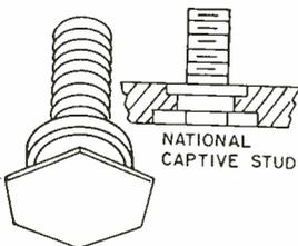
National Captive Studs provide a permanently fixed male thread in thin sheets of aluminum, brass, and some plastics. A hole is drilled or punched a few thousandths greater in diameter than the cylindrical pilot and the stud is pressed-in until the entire hexagonal portion is imbedded in the panel. The stud is locked-in by the cold flow of metal around the barrel or undercut sec-
