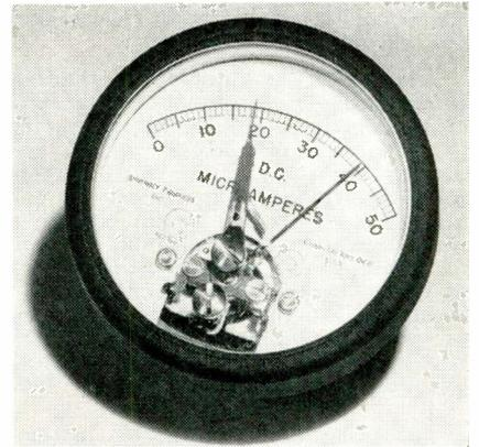
Indicating pointer has passed set point but control circuits remain energized. Note position of toggle, on adjustable pointer.
