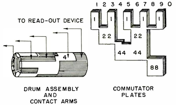
Fig. 3 (Left): Brushes read consumption in a 4-digit, binary code, from position on commutator.
