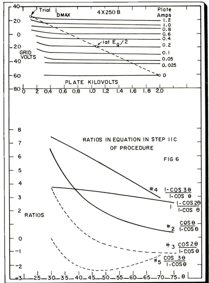
In general,  $e_{bmin}$  may be set lower than  $E_{sg}$ , for the tetrode, providing the constant plate current curves do not bend sharply upwards, and providing screen grid current is not excessive. For the triode,  $e_{bmin}$  may be equal to—or slightly higher than— $e_{cmax}$ , if the grid current is not excessive.
