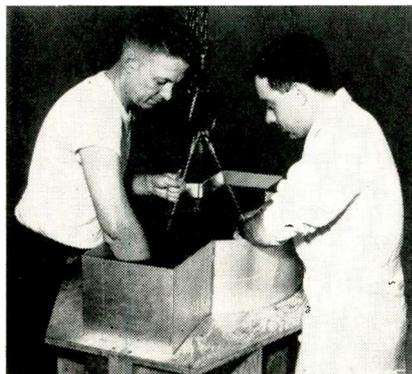
Martin Co. engineers are using castor oil at 100° F to keep air out of an electronic transducer assembly. Assembly is used in Martin's Sonar. Rubber shells prevent short-circuiting when transducer is immersed in water. Castor oil, a dielectric, is also a sound energy conductor.
