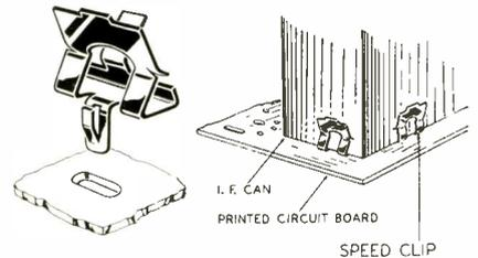
bottom edge of the i-f can, requiring no special cut-outs in the can or special assembly tools. Two barbs on the clip bite into the side of the can, providing firm retention and an excellent grounding connection between can and clip. A spring tab supplies tension until the final soldering operation. Tinnerman Products, Inc., Cleveland, Ohio.
