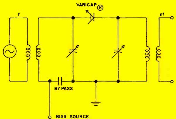
Fig. 5: Basic circuit of the harmonic generator. The voltage variable capacitor is driven at a frequency "mf."
