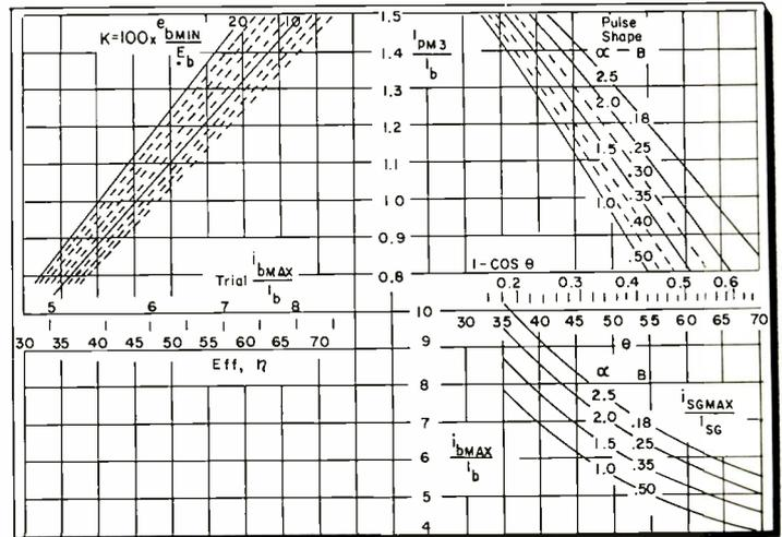
Fig. 4: Frequency tripler design is eased with this chart.
