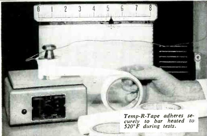
Temp-R-Tape adheres securely to bar heated to 520°F during tests.
