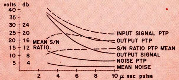
Fig. 4: Graph shows threshold signals of printed diode matrix for operating magnetic shift register
