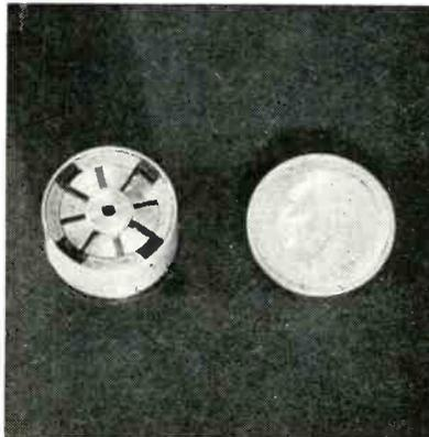
protection. Its qualifications are: Adjustable, torque range 0 to 100 in.-oz.; repeatable breakaway torque; no backlash, chatter, or gauling; corrosion resistant; small; 0.630 x 0.450 in.; weight: 0.03 lbs.; concentricity: to 0.003 in.; may be supplied with integral gear blank; gear made per order: Special shaft configurations available. Northern Union, Inc., 1020 Holly Ave., Arcadia, Calif.
