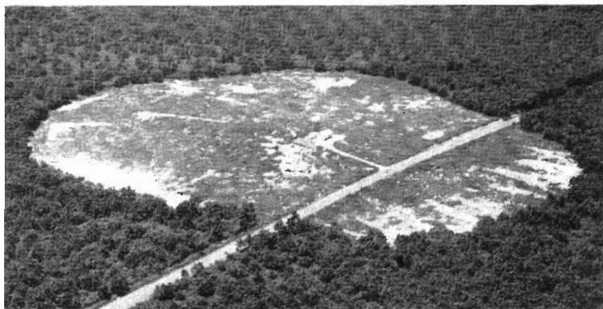
Fig. 2. Typical VOR Transmitter site at Philipsburg, Pa. Although the actual installation is small a large clearing around the antenna is essential to prevent radiation shadows.
