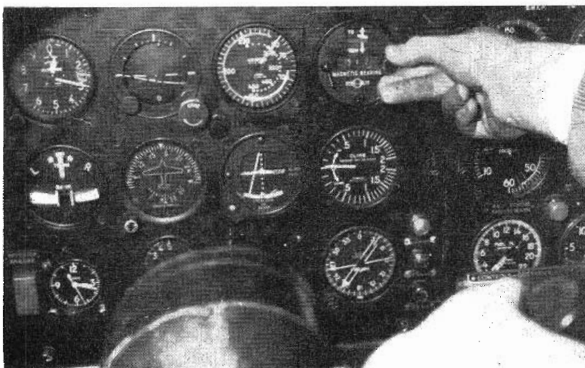
Fig. 1. (Above) Typical aero radio navigation installation in Navion aircraft belonging to Aircraft Radio Corporation. VOR and LF range receivers are installed together with tower receiver and 10 Channel VHF tower transmitter on left panel.
