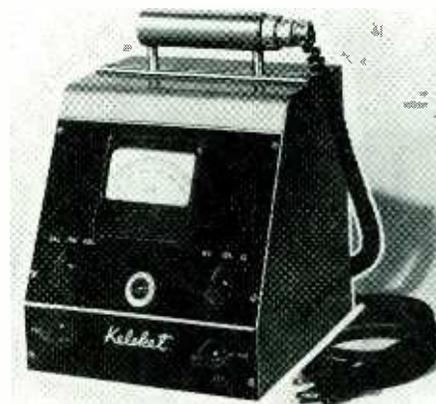
as model K-900. Geiger tube detecting element permits differentiation between beta and gamma radiation. The Geiger tube probe is connected to the main cabinet by a self-retracting cord. When not in use, the probe is mounted in the handle of the cabinet.—Kelly-Koett Manufacturing Co., 12-T East 6th St., Covington Ky.—TELE-TECH
