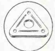
E. Patented Plate spaced every 2' for rigidity.
