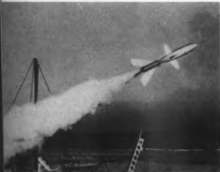
NACA two-stage radio-guided interceptor missile MX-570 taking off at Wallops Island test station, Langley Field, Va.
