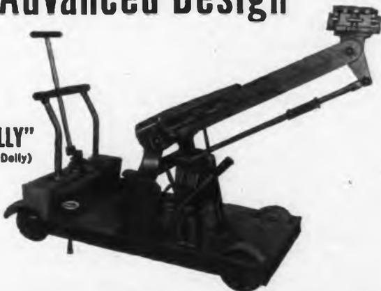
Hydraulic lift type for fast upward and downward motion of TV cameras. Lightweight—sturdy—easily transported in a station wagon. Fits through a 28" door. Adjustable leveling head. In-line wheels for track use. Steering wheel and floor locks.
