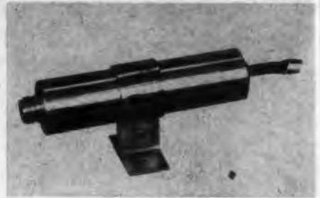
Fig. 29: Balun for matching balanced 300-ohm line to unbalanced 75-ohm coaxial
