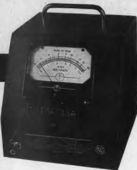
INPUT IMPEDANCE: 1 megohm shunted by 30 mmfd.
