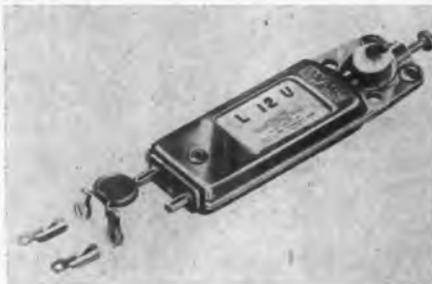
Slipping off the condenser raises output. Range is 5 KC. Minimum needle pressure is one ounce; weight of the cartridge is 19 grams.—Astatic Corp., Conneaut, Ohio.—TELE-TECH.
