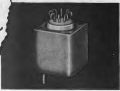
**EXAMPLE:** Working with the North Electric Manufacturing Co., Galion, Ohio, we developed a new miniature hermetically sealed relay to meet exacting military requirements. Features include an 8-terminal sealed header .600" O.D. and a new design balanced armature relay, sealed in a 7/8" x 7/8" x 7/8" drawn aluminum can. The entire unit may be panel mounted from either the top or bottom. The unit can be furnished either with a dry air fill or vacuum-pumped and pressure filled with dry nitrogen.
