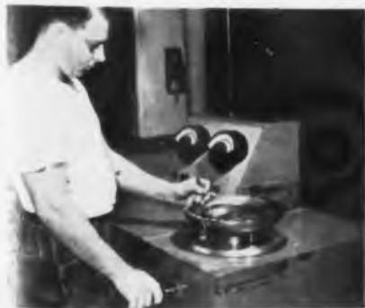
Given part of torque converter turbine is dynamically balanced on Chrysler's Timius-Olsen machine which compares off-center pulse with reference pulse to locate unbalance
