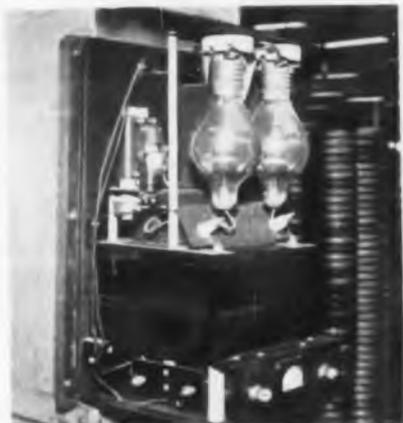
Electronic rectifier supplies dc to operate magnetic chucks in Nash production machinery. Electron tubes also control speed of motors
