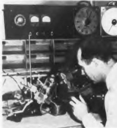
Fig. 4: Operator carefully observes etching of germanium for surface-barrier transistor
