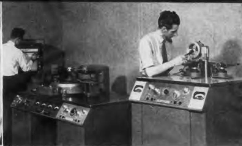
X-ray diffraction film record (left) is scanned in microphotometer in GM lab. Beam is picked up on phototube, whose output is then amplified. Resulting signal is displayed on strip chart. In photo (right above) Engineer at left checks angular position on recorder of GE X-ray spectrogoniometer in Ford Scientific Laboratory. Researcher at right adjusts specimen position on X-ray diffraction camera
