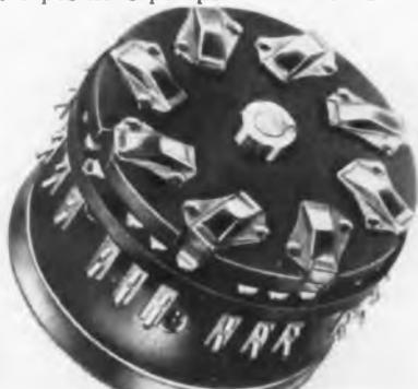
ing action. Spacing is 15° between live positions with shorting-type action; 30° spacing with non-shorting action. Silver alloy rotors, slip rings and contacts are used exclusively. Contact panels and rotors are fabricated from XXXP phenolic in accordance with MIL-3115B. The Daven Co., 191 Central Ave., Newark, N. J.—TELE-TECH & ELECTRONIC INDUSTRIES.
