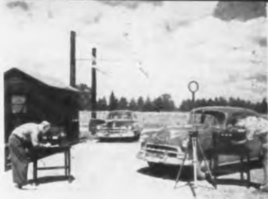
Radiation from ignition system is checked to see if it will cause radio or TV interference on General Motors Proving Grounds
