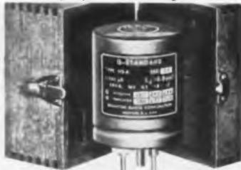
consists of a specially developed winding in a hermetically sealed copper shield can filled with dry helium. A convenient carrying and storage case is included. Normal inductance is 250  $\mu$ h and is specified to +1%. Distributed capacitance, when mounted on the type 160-A or 260-A Q meter is approx. 9  $\mu$ mf and is specified to +2%. **Boonton Radio Corp., Boonton, N. J.—TELE-TECH & ELECTRONIC INDUSTRIES.**
