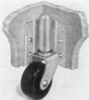
**Swivel Type Caster and Bracket** with 1 3/8" non-marking wheel. Constructed with narrow mounting area for purposes of concealment. Strengthens corner cabinet, so that customary corner block could be eliminated.
