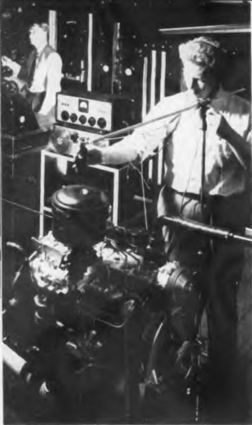
Chrysler engine on mount produces sounds which are picked up by mike and taped on Magne-corder. Subjective sound tests aid designers
