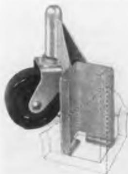
**Swivel Type Caster**, designed to eliminate screws. Caster slips into grooves cut in corner block and can be inserted by dealer, making casters an optional purchase.
