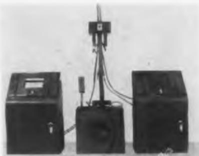
are translated into thickness readings and shown by a pen trace on a recorder chart. **Tracerlab Inc., 130 High St., Boston 10, Mass.— TELE-TECH & ELECTRONIC INDUSTRIES.**
