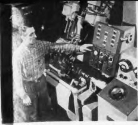
Impulses produced by rotating Ford crankshafts are stored in electronic memory. With crankshaft stationary, drills automatically remove metal to bring part to 0.5 oz.-in. perfect dynamic balance
