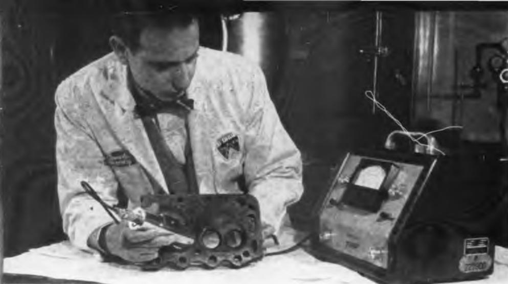
Radiation detector shows cylinder head leakage of isotope-tagged coolant on Tracerlab monitor
