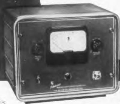
**MODEL 904 NOISE GENERATOR** - A direct reading noise source permitting measurements of noise factors up to 20 db. for r-f amplifiers and receivers operating from 10 to 1000 Mc/s. The TT-1 coaxial diode has nominal input impedance of 50 ohms. VSWR Approx. 1.25.
