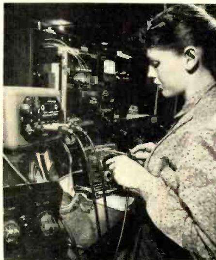
Electronic relay which adjusts indoor temperature according to signals from two electronic thermostats, one mounted outdoors, is assembled at Minneapolis-Honeywell. Punched grid circuit is used instead of conventional wiring
