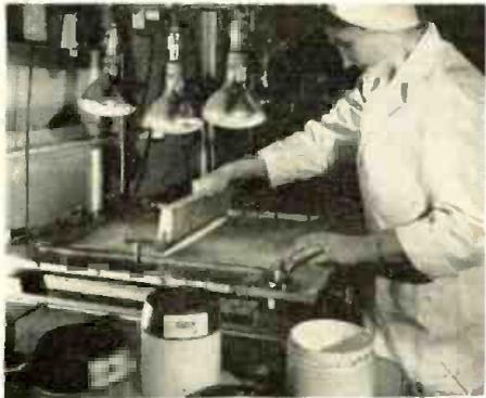
**4** Phosphor material of whipped cream consistency is silk screened through gelatin stencil and deposited as dots on plate
