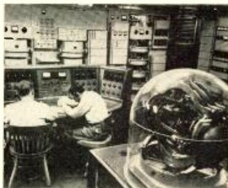
Technicians at Bell Labs. set up simulated firing course to study action of Nike, guided missile for aircraft defense. Flight problems are introduced into electro-mechanical simulator and computer through control panel. Unit will be installed at Ft. Meade, Md.
