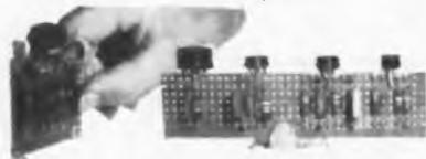
Alden standard components, to mount your circuitry in compact vertical planes as illustrated here, consist of Prepunched Terminal Card, Miniature Staking Terminals, Card-mounting Sockets.
