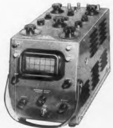
Repetitive or trigger sweep is variable from 5 cps. to 500 kc with 5X sweep expansion. Sweep, marker, and dc. calibrating voltage is available externally. Operates from 50 to 400 cps. at 115 v. ac. Size, 8½ x 6¼ x 13¾ in. Weight, 22 lbs. **Waterman Products Co., 2445 Emerald St., Philadelphia 25, Pa.—TELE-TECH & ELECTRONIC INDUSTRIES.**
