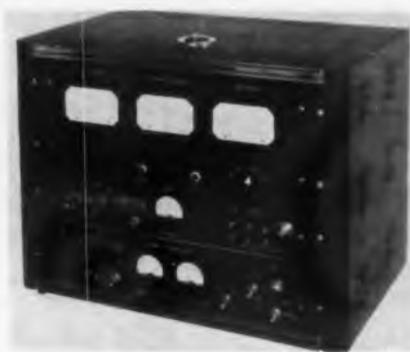
Fig. 5: Telemetering transmitter test unit
