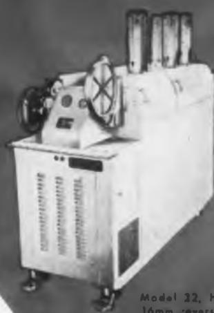
Model 22, H-F developer for 16mm reversal films. It is self-contained, easy to operate, entirely automatic, daylight operating. Adaptable to negative, positive or 35mm films.
