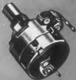
TYPE C2-45, 15/16" diameter variable composition resistor. Wattage rating: 1/2 watt for resistances through 10,000 ohms, 1/3 watt for resistances over 10,000 ohms through 100,000 ohms, 1/4 watt with 500 volts maximum across end terminals for resistances over 100,000 ohms. Available with or without illustrated attached switch and in concentric shaft tandem construction C2-45 as shown above.
