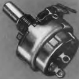
TYPE C2-35, 1 1/8" diameter variable composition resistor. Wattage rating: 3/4 watt for resistances through 10,000 ohms, 2/3 watt for resistances over 10,000 ohms through 25,000 ohms, 1/2 watt with 500 volts maximum across end terminals for resistances over 25,000 ohms. Available with or without illustrated attached switch and in concentric shaft tandem construction C2-35 as shown above.
