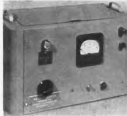
voltmeter, magnetic counter and felt cup electrode. A flashing lamp and bell indicates the frequency of the pinholes. In conjunction with the footage counter, the instrument produces a continuous display of total number of pin holes for a given footage. Peschel Electronics, Inc., 13 Garden St., New Rochelle, N. Y.—TELE-TECH & ELECTRONIC INDUSTRIES.
