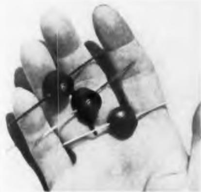
and leads are then assembled and vacuum-impregnated with tropicalized r-f wax. Values of inductance range from 2.2 to 220 mh. Nominal tolerance is  $\pm 10\%$   $\pm$  one turn. Nominal Q tolerance is  $\pm 20\%$ . Core material is Ferroxcube 3C. Curie temperature, 172° C. (342° F.) Weight,  $\frac{1}{2}$  oz. Mico Instrument Co., 75 Trowbridge St., Cambridge 38, Mass.—TELE-TECH & ELECTRONIC INDUSTRIES.
