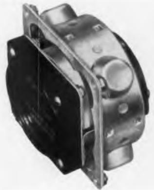
mounting system. It is a center-of-gravity type that employs stainless steel resilient cushions that are corrosion-resistant and unaffected by extreme temperature exposure, oil, water, solvents, fungi, or dust. Multi-directional design is said to provide maximum stability and protection at any altitude under the most adverse flight and landing conditions. Robinson Aviation, Inc., Teterboro, N.J.—TELE-TECH & ELECTRONIC INDUSTRIES.
