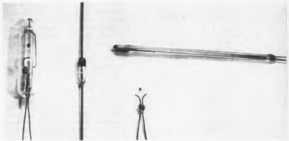
Fig. 2: Bead types made by American Radio. Unit at left is in bulb, others exposed or in glass
