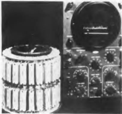
output is applied to the stator of a capacitance commutator. When scanned by the rotor, this yields the output of all the filters in frequency sequence. Maximum sensitivity is attained by high-Q magnetostriction rods as filters. **Raytheon Manufacturing Co., Equipment Engineering Div., 148 California St., Newton 58, Mass.—TELE-TECH & ELECTRONIC INDUSTRIES.**
