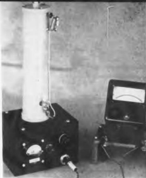
Fig. 7: Transistorized UHF oscillator and cavity resonator. Supply current is stabilized with the aid of a saturated vacuum tube
