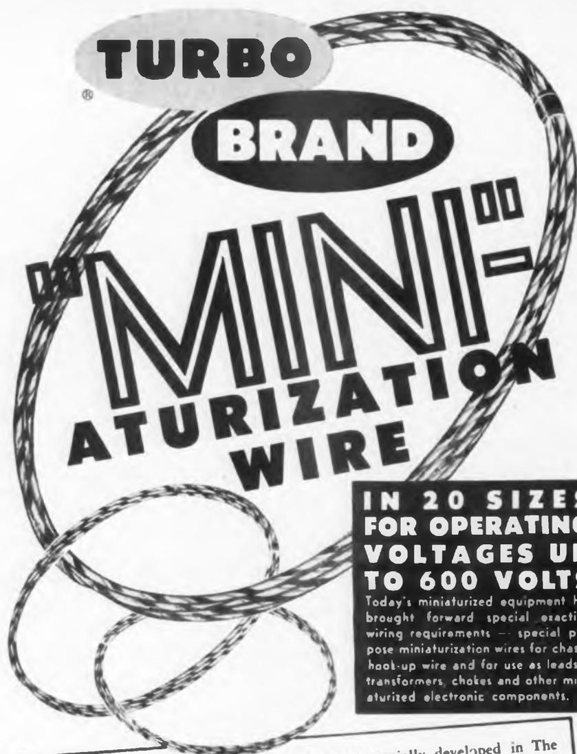
**TURBO BRAND** Miniaturization Wire was specially developed in The William Brand laboratories to meet a use need within the range of  $-55^{\circ}\text{C}$  to  $+105^{\circ}\text{C}$  and maximum operating voltage of 600 volts rms. This "mini" wire is available in 20 strandings, ranging from 7/38 to 19/25 and in a graduated scale of AWG sizes from 30 to 12. It is available in both solid and stranded — in solid colors or "candy striped" with 1, 2 or 3 tracers.
