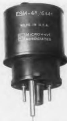
ESM-48, the 6444 is fixed-tuned, incorporates the Philips dispenser-type cathode, and delivers 1 w. of CW energy into a standard klystron type output. Microwave Associates, Inc., 22 Cummington St., Boston 15, Mass.—TELE-TECH & ELECTRONIC INDUSTRIES.
