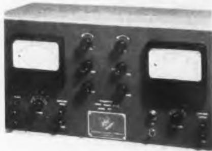
cally many times per second obtains a continuous direct reading of noise figure which reduces measurement to a simple meter reading. Noise figure is measured in accordance with IRE standards, one cycle band width at 1,000 cps. **Electronic Research Associates, P.O. Box 29, N. Caldwell, N.J.—TELE-TECH & ELECTRONIC INDUSTRIES.**
