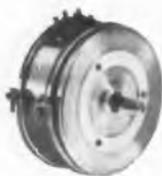
**TYPE 753** – Sine-cosine potentiometer – Full sine-cosine function without mechanical cams and linkages – can be ganged up to 6 cups. 20,000 ohms per quadrant; linearity,  $\pm 0.5\%$  peak-to-peak; 3" diameter,  $1\frac{1}{4}$ " long from front of servo flange to rear of cup. Also available as straight sine function.
