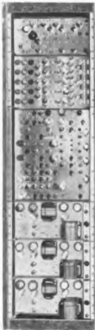
An integrated basic package for producing color signals. Converts monochrome synchronizing generator for color, generates standard color bars, and encodes output of Color Bar Generator, color camera chain, or color slide scanner to produce composite color video signal. Requires 70 inches of standard rack space. Includes units listed below.
