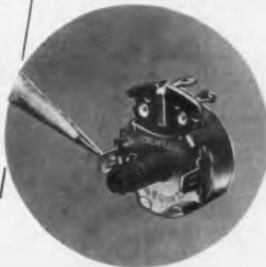
Twist-Tab Mounted Series 47. Eliminates usual bushing, lockwasher, nut. Compression element control. Metal or plastic shaft. Plastic shaft has rear slotted protrusion, therefore adjustable from front or rear.
