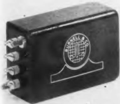
example, provides a 9 kc total pass band at 455 kc. The TX-455-SB is a side band filter. The size of either type is equivalent to an ordinary i-f transformer. Arnell & Co., Inc., 45 Warburton Ave., Yonkers, N. Y.—TELE-TECH & ELECTRONIC INDUSTRIES.
