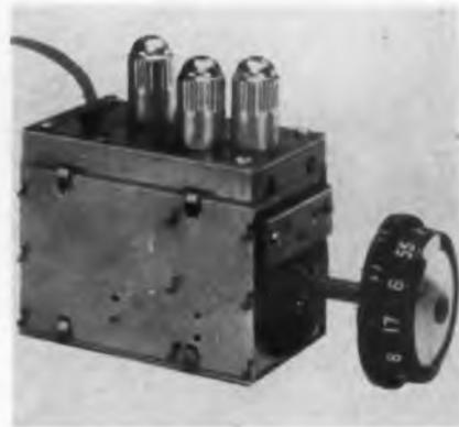
space used for any VHF tuner, or on the side of the cabinet. Improved performance is achieved by use of the new 6AN4 tubes. One is employed as an r-f amplifier for all 82 channels. The other is used in place of a crystal mixer. A 6T4 oscillator operates at the fundamental with full output, even on channel 83. Anchor Radio Corp., 2215 S. St. Louis Ave., Chicago 23, Ill.—TELE-TECH & ELECTRONIC INDUSTRIES.
