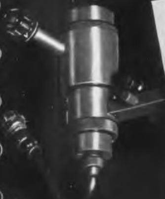
**DIC-2217 — KLYSTRON MOUNT FOR 2K25, "X" BAND**
