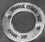
Designed to fit around 7-pin miniature tube sockets, these capacitors may contain 1, 2, or 4 sections. They result in a neat physical layout while reducing space to a minimum. Positive positioning of the ultra short leads between the capacitor and socket terminals eliminates lead dress problems and, consequently, allows "hot" circuit designs. Voltage ratings from 100 to 500 d-c. Write for Engineering Bulletin 610.
