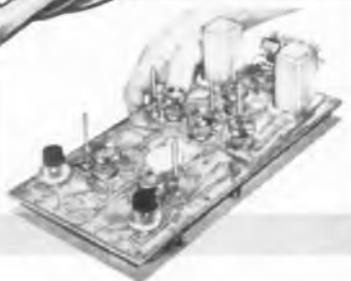
NOW further **COST REDUCTION** and **PROFIT POTENTIAL** accrue from Photocircuits development of cross-through connections by *plating through panel holes*. This is another good reason for having your products engineered and produced by Photocircuits Corporation.
