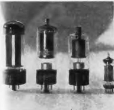
ode for the power supply of TV receivers. The 6AR8 is a double-anode wet beam deflection tube for use as a synchronous detector in color receivers. The 6BU5 is a low-current, high voltage beam pentode for use as a shunt voltage regulator in the high voltage power supply of color TV receivers. General Electric Tube Department, Menectady 5, N. Y.—TELE-TECH & ELECTRONIC INDUSTRIES.
