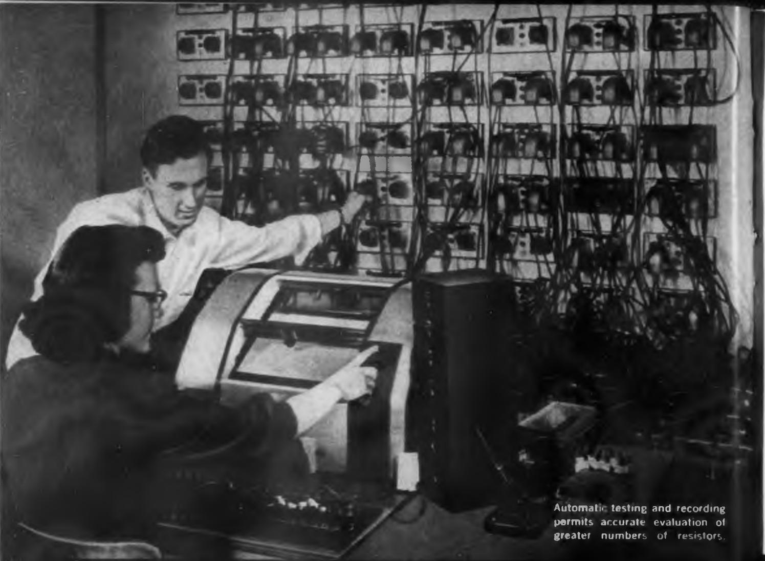
Automatic testing and recording permits accurate evaluation of greater numbers of resistors.
