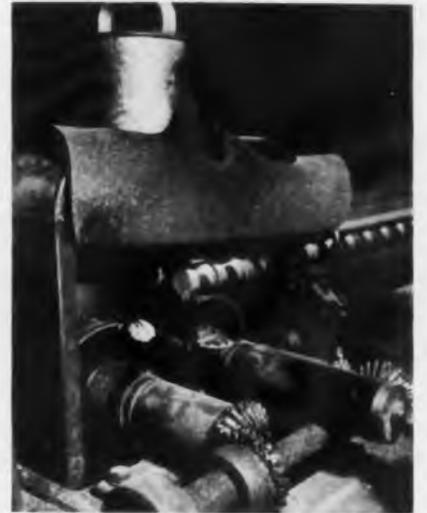
The electronic nutcracker, which fires 65 kv, 5,000 a. bursts 20 times per second, has achieved a one-third increase in shelled walnut production. Special capacitors developed by Westinghouse are the key units.
