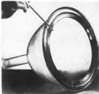
End welded studs installed on flange of tube simplify alignment of shadow mask and screen
