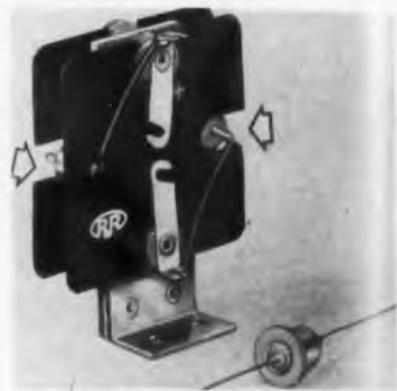
mounted on a cooling fin. Two diodes, No. 1N158—indicated by arrows—are connected in series on a cooling fin. Type 1N153, for example, with a peak inverse voltage rating of 300 v is capable of delivering 0.5 amps into a restrictive load with a voltage drop of only 0.7 v. **Selectron & Germanium Div., Radio Receptor Co., Inc., 251 West 19th St., New York 11, N.Y.—TELE-TECH & ELECTRONIC INDUSTRIES.**
