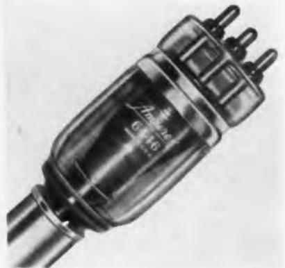
duty, and the high dissipation reserve allows extreme mismatch of load to tube impedance. The 6446 uses only  $\frac{1}{2}$  the water flow required for Type 892 for equivalent anode dissipation. The tube is also available in an air-cooled version, Type 6467. **Amperex Electronics Corp., Engineering Dept., 230 Duffy Ave., Hicksville, L.I., N. Y.—TELE-TECH & ELECTRONIC INDUSTRIES.**
