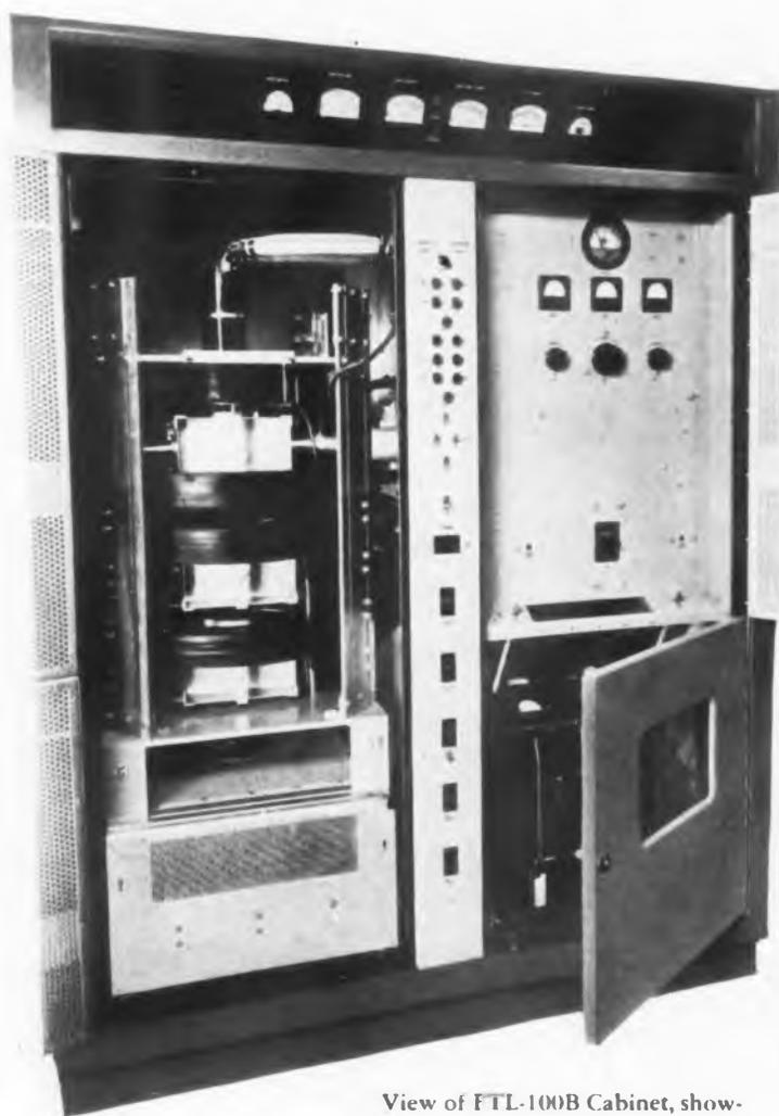
View of FTL-100B Cabinet, showing cavities and magnet structure designed for rapid tube change.
