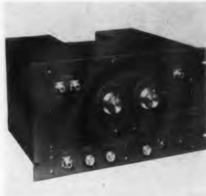
600 cathode-ray indicator, the maximum sweep speed is 200 in./ $\mu$ sec. Controls and connectors on the front panel include sweep speed controls, trigger input, gate output, and external horizontal deflection input jacks. Power connections are at the rear. **Spencer-Kennedy Laboratories, Inc., 186 Massachusetts Ave., Cambridge 39, Mass.—TELE-TECH & ELECTRONIC INDUSTRIES.**
