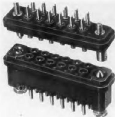
lock, a stainless steel guide socket with a detent for a bayonet guide pin, is also a self-aligning guide pin and guide socket for positive polarization. These connectors are available in 12, 18, 24, and 34 contacts with bayonet locks, either chassis or cable-mounted. DeJur-Amsco Corp., 45-01 Northern Blvd., Long Island City 1, N.Y.—TELE-TECH & ELECTRONIC INDUSTRIES.
