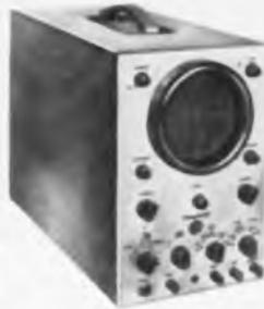
The new WO-78A 5-inch Oscilloscope permits accurate voltage measurements of TV signals throughout the video range in both color and black-and-white receivers. In the wide-band position, the WO-78A has a response flat within -1 db, from 3 cps to 4.5 Mc, with sensitivity of 0.1 volt peak-to-peak per inch (0.035 volt rms per inch). In the narrow-band position, sensitivity is 0.01 volt peak-to-peak per inch. Phase characteristics are excellent throughout entire frequency range.
