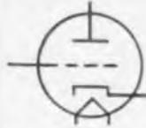
Triode, Indirectly Heated Cathode. Add grids for tetrode, pentode, etc.
