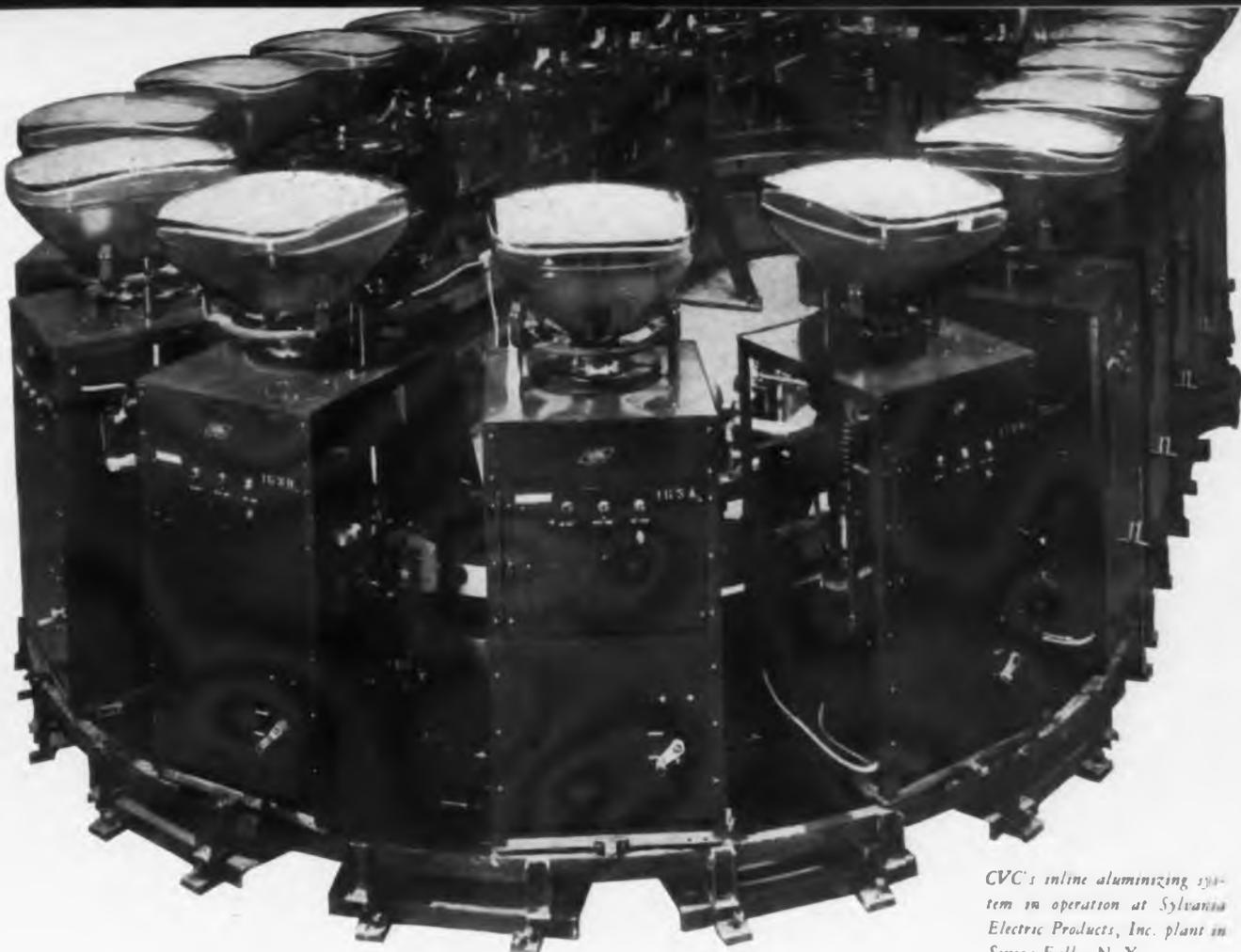
*CVC's inline aluminizing system in operation at Sylvania Electric Products, Inc. plant in Seneca Falls, N. Y.*
