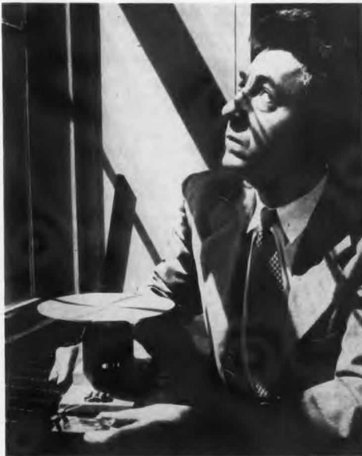
Sunlight provides power to turn motor-driven wheel at Bell Labs. D. M. Chapin, one of the three-member team who invented the solar battery, holds unit which contains strips of specially prepared silicon about the size of common razor blades. Reported to be the first successful device of its type, solar battery converts sun's energy directly into electricity with 6% efficiency. Device opens new horizons for power generation. Details on p. 128
