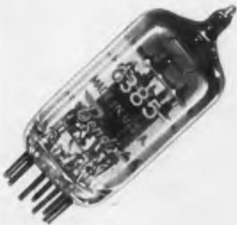
oscillator. As an oscillator, the upper limit of its frequency is approximately 500 mc.  $\mu$  is 35 and  $g_m$  is 5000  $\mu$ mbos. Withstands severe shock and vibration. Red Bank Div., Bendix Aviation Corp., Eatontown, N.J.—TELE-TECH & ELECTRONIC INDUSTRIES.
