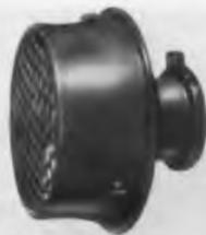
The features of all AIR MARINE motors include Stainless steel thru-bolts, Rigid die-cast aluminum housings, and Riveted stator to insure Extra-Rigid Construction assuring positive bearing alignment and uniform air gap. Motors are protected against humidity and fungus growth—can be mounted in any position—are equipped with ball bearings using lubricants for high and low temperatures—meet all AN specifications.
