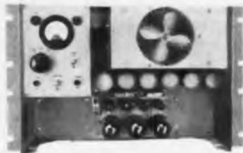
**FTL-279A Low Voltage Power Supply:** Mounts in 14" height in standard rack cabinet. Employs long-life selenium rectifiers. Low heat dissipation and unusually light weight are features of this equipment. Weighs only 40 lbs.
