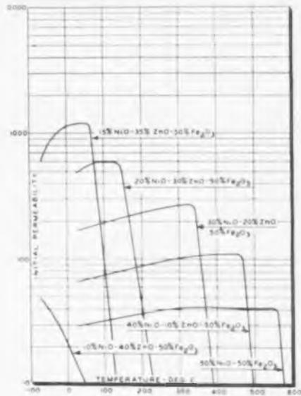
Fig. 6: Variation of initial permeability and Curie temperature as function of composition
