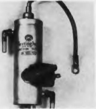
mostatic control. A calibrated thermostat on the side of the tube can be used to stop tube operation if water flow is insufficient, or with a solenoid water valve to turn cooling water on and off. The tube is designed primarily for resistance welding control. Westinghouse Electronic Tube Div., Box 284, Elmira, N. Y. —TELE-TECH AND ELECTRONIC INDUSTRIES.
