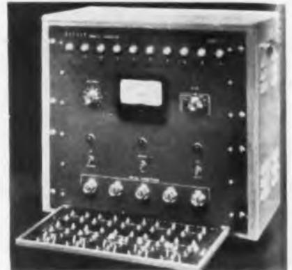
printed circuit problem boards are a special feature, and a schematic layout of the amplifier and initial condition connections enable rapid problem setup. Donner Scientific Co., 2829 Seventh St., Berkeley 10, Calif.—TELE-TECH & ELECTRONIC INDUSTRIES.
