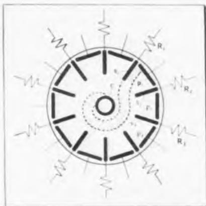
Fig. 6: Trochotron design: c, cathode; s, spade; p, plates; R, impedances for beam locking
