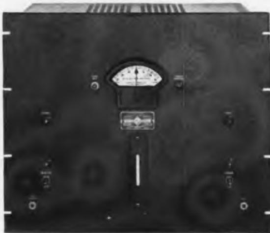
**Type 1181-AT Color-Subcarrier Monitor** . . . indicates directly both magnitude and direction of frequency deviation of the color subcarrier . . . has high reliability for continuous service
