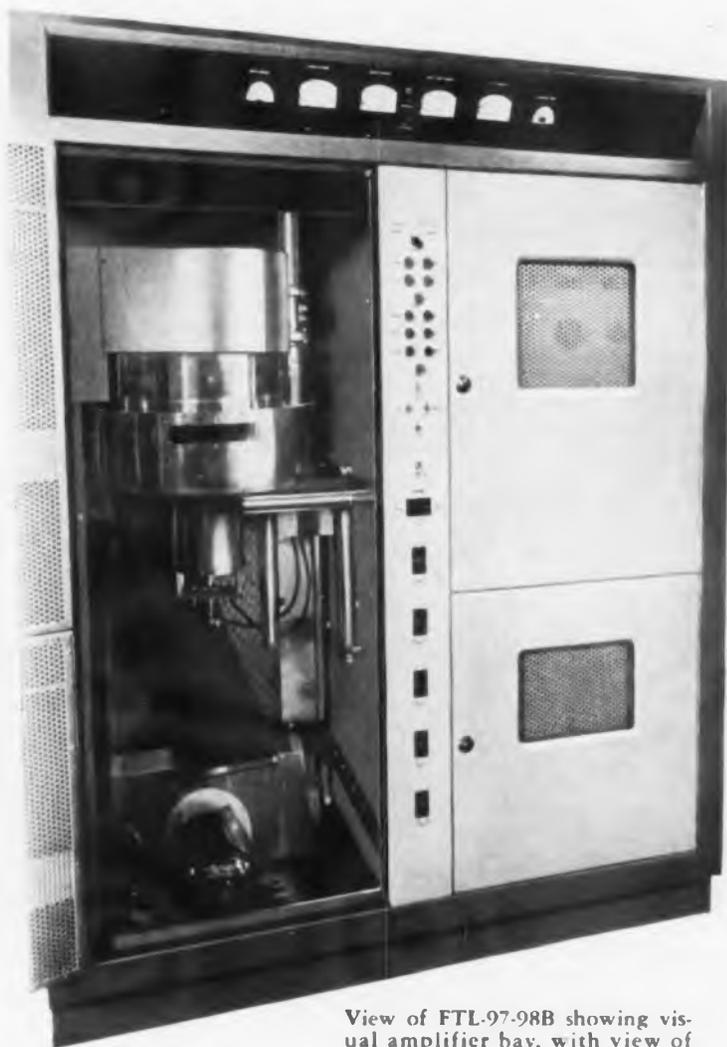
View of FTL-97-98B showing visual amplifier bay, with view of high-power amplifier cavity circuit.
