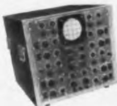
✦ **Four Channel Scopes**—Same separate controls. #H-43, DC-200kc range, for use with continuous film strip camera. #H-45, DC to 300kc range, sensitivity over .028 Vdc/in.
