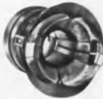
The new RCA-220D1 yoke is designed for rectangular-type 90° kinescopes operating at ultor voltages up to 18 kv. A ferrite core and precision-shaped cosine-type windings, treated with anti-corona silicone resin, provide high efficiency and good side and corner resolution. Molded insulation is employed to withstand the high peak voltage between the horizontal and vertical coils. The 220D1 is designed for use with the RCA-238T1 and RCA-239T1 horizontal-output and high voltage transformers.
