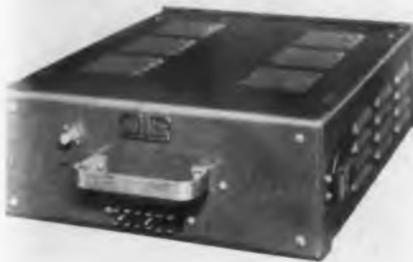
chassis. Operating control head has a drop-out panel to provide accessibility. Also available, MCA 101A mobile two-way radio is rated at 35 w output at 25-25 mc. Transmitter, receiver, and power supply are in one metal cabinet. Designed for dashboard mounting. Mobile Communications Dept., Allen B. Du Mont Laboratories, Inc., 1500 Main Ave., Clifton, N.J.—TELE-TECH & ELECTRONIC INDUSTRIES.
