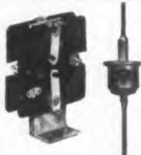
Featuring very low forward resistance along with high back resistance which results in high rectification efficiencies of close to 100%. Intended for power rectification service.
