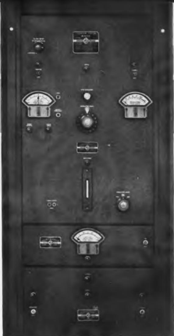
**Type 1183-T TV Station Monitor** indicates visual-carrier deviations with an accuracy of better than  $\frac{1}{2}$  ppm . . . indicates aural-carrier deviations to better than 1 ppm . . . measures modulation level . . . and makes provision for checking distortion and noise for "proof-of-performance" testing.
