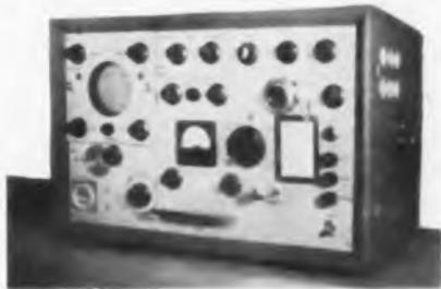
Fig. 1: Portable version of radar test unit
