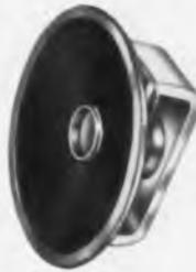
Contoured for economy of space, this new RCA-222S1 PM speaker features a 2 1/2-in. cone and measures only 2 3/4 in. in diameter by 1 1/4 in. in depth. The weight is only 4.6 ounces, including a 1.0-ounce Alnico V magnet for high efficiency. Frequency range is 300-3500 cps and the voice-coil impedance is 12 ohms. Life-tested at 250 milliwatts, the speaker is designed for long trouble-free service in applications where space is at a premium.
