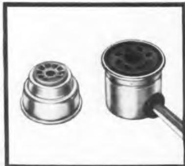
For high voltage tubes these corona caps and socket combinations for both octal and noval sizes feature generously rolled outer surfaces. Assemblies are designed for screw mounting to condenser studs or stand offs and are available with general purpose black or low loss mica phenolic insulators. Noval caps available with 1-5/16" or 1-1/2" major rim diameter. Octal units have insulating fibre liners.
