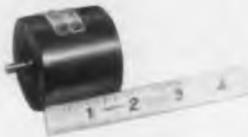
A08C1—2 phase control motor for operation on 60 cycle supply 115 Volt on one phase and 40 Volt on control phase. 3.0 oz/in starting torque on above voltages. 1500 RPM. No load speed.
