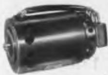
A15HF—115 Volt 60 cycle single phase capacity start & run synchronous motor running at 3600 RPM. This unit has special terminal block mounted on end of motor.
