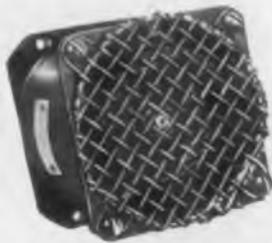
A11A-2—115 Volt 400 cycle single phase axial vane blower delivering 70 CFM at 1" static pressure at 11,000 RPM.
