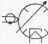
Magnetron Tunable, Loop Coupled
