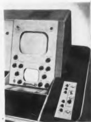
**FTL-278A Camera Control and Monitor:** Mounts in handsome console section (13.5-16" wide). The FTL-271A Projector Control Panel is shown on the right of the FTL-278A. Camera control and monitor provides 10" picture and 5" waveform. Simplified panel permits one operator to fully control two film projectors, automatic slide projector and opaque projector. Weighs 60 lbs.
