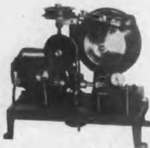
FILAMENT COIL WINDING MACHINE
