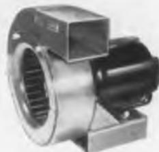
631 x 1—115 Volt, 60 cycle, 3450 RPM 100 CFM @ 2½" water gauge. Fits in space 9½" long, 8¾" wide, 7¾" high.
