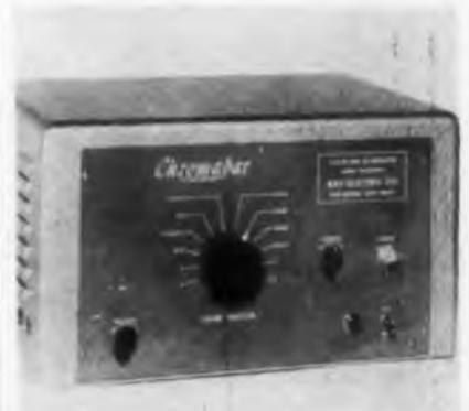
vergence and linearity. No other equipment needed to produce colors on TV receivers. Output at video frequency, variable to 1.4 v peak-to-peak positive and negative into 75 ohm load. Kay Electric Co., Pine Brook, N.J.—TELE-TECH & ELECTRONIC INDUSTRIES.
