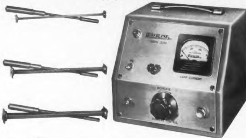
The WAVELINE Model 2200 microwave noise source—gas noise tube in combination with its Waveguide mount and power unit—provides a random noise source of known output level in the frequency range from 2,600 to 26,000 MCS. Throughout this range it also functions as an untuned termination.
