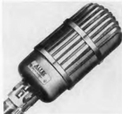
back discrimination averaging 18 db. A new feature enables variation from omni-directional through figure 8 to cardioid pattern, and provides output impedance of 30/50 ohms and 150/250 ohms. Output level is -58 dbm. Provided with three standard thread fittings and an XL plug. Altec Lansing Corp., 161 Sixth Ave., New York 13, N.Y.—TELE-TECH & ELECTRONIC INDUSTRIES.
