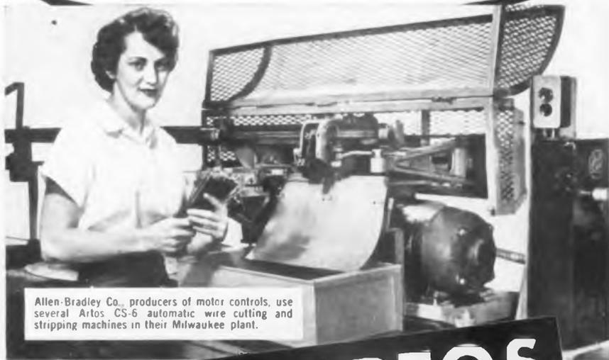
Allen-Bradley Co., producers of motor controls, use several Artos CS-6 automatic wire cutting and stripping machines in their Milwaukee plant.
