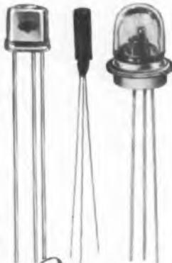
Types RR14, RR20, RR34, 2N34, 2N36, 2N37 and 2N38 intended for applications in low level audio circuits. Particularly applicable where small size and economy of operation are desirable.
