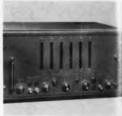
can be measured with a maximum accuracy of  $\pm 1.0$  cps. As an electronic counter, the instrument operates at rates up to 1,000,000 cps. The unit utilizes the Models 705AF and 707AF decimal counting units that provide binary coded output information for data reduction requirements. **Berkeley Div., Beckman Instruments, Inc., 2200 Wright Ave., Richmond, Calif.—TELE-TECH & ELECTRONIC INDUSTRIES.**
