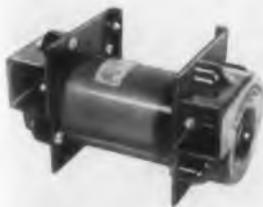
A15BD—115 Volt 400 cycle single phase double blower delivering 26 CFM total at 0 static. This unit has special mounting brackets.
