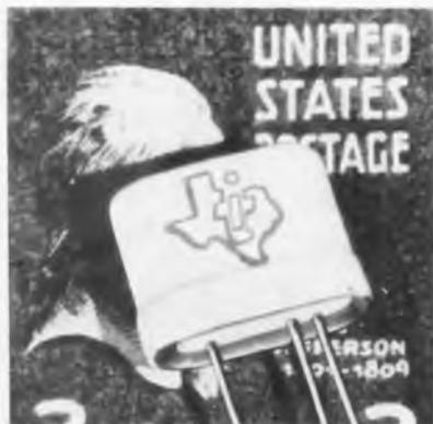
conductor crystal rather than make it mechanically. The manufacturer specializes in grown junction germanium transistors also. Texas Instruments, Inc., 6000 Lemmon Ave., Dallas 9, Texas.—TELE-TECH & ELECTRONIC INDUSTRIES.
