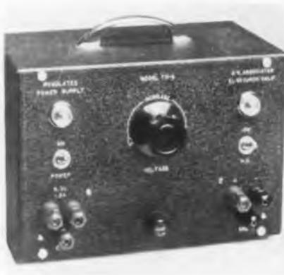
is 0 to 50 ma, max. Regulation, less than 0.1% from no load to full load at line voltages 105v—125v. Ripple, less than 1.5 mv, rms. AC output, 6.3 v at 1.2 amp, max. Output impedance, 2 ohms. Power source, 105-125 v, 60 cps, 50 w. Dimensions, 5 x 6 x 9 in. Available for standard rack and panel mounting. G. W. Associates, P. O. Box 2263, El Segundo, Calif.—TELE-TECH & ELECTRONIC INDUSTRIES.
