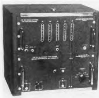
A front panel switch selects the number of output pulses/sec. from the timing unit. One function unit circuit is used to generate a sharp pulse when the input signal  $E_1$  intersects the zero axis to start the timing unit counting. The other function unit circuit generates a sharp pulse when the input signal  $E_2$  intersects the zero axis and is used to stop the counting. Advance Electronics Co., 451 Highland Ave., Passaic, N. J.—TELE-TECH & ELECTRONIC INDUSTRIES.
