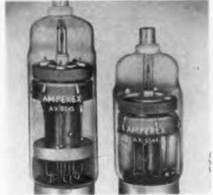
directly interchangeable with RETMA tubes with the same designation. Each is a three electrode Xenon-filled tube with negative characteristics. The inert gas filling enables reliable operation at maximum ratings over a wide temperature range. Complete data is available at the Engineering Department, Ampere Electronic Corp., 239 Duffy Ave., Hicksville, L. I., N. Y.—TELE-TECH & ELECTRONIC INDUSTRIES.
