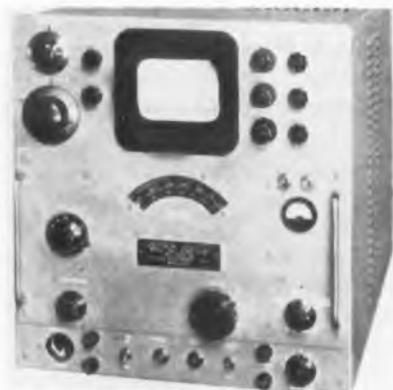
frequency spectrum. A swept i-f yields constant dispersion characteristics independently of the frequency setting. Frequency dispersion from 250 kc to 25 mc can be realized with a resolution of 25 kc. An internal marker measures frequency differences up to  $\pm 12.5$  mc on a 5 in. CTR display. Polarad Electronics Corp., 100 Metropolitan Ave., Brooklyn 11, N. Y.—TELE-TECH & ELECTRONIC INDUSTRIES.
