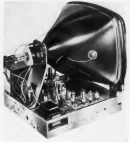
New Admiral TV chassis with 21-in., 90° deflection tube also include printed circuits
