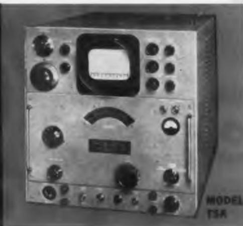
Now, a new Polarad spectrum analyzer only 21 inches high that covers the entire frequency range 10 to 22,000 mcs with but 3 interchangeable R-F tuning heads. The model TSA operates simply—single dial frequency control—with utmost frequency stability. It provides highest accuracy, and reliability for observation and true evaluation of performance over the entire R-F spectrum—saving engineering manhours.
