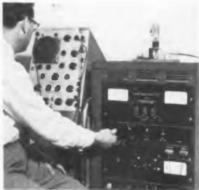
Checking cathode emission visually at NBS labs
