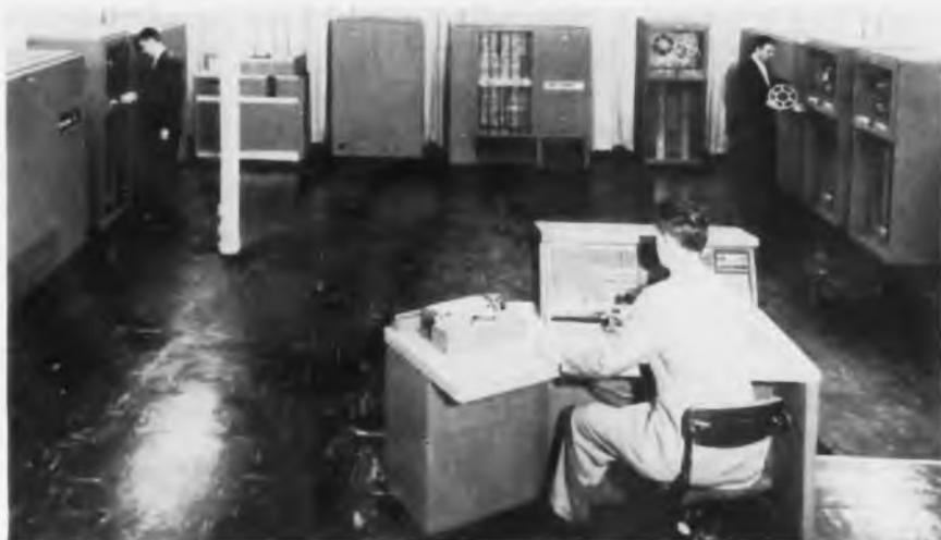
Partial view of the IBM '702' electronic data processing machine. Control over the entire system is maintained from the operator's console in foreground. Arrangement of units is varied to fit particular applications. Prime users of this equipment will be insurance companies and manufacturing industries.
