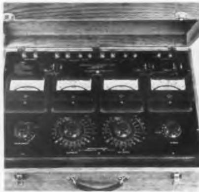
that can be used down to 10% power factor; also, 7 current ranges from 10 ma to 10 amps, full scale, and 4 v ranges from 30 v to 300 v, full scale. Wattmeter "A" is a high range dynamometer unit; wattmeter "B" is low range. The voltmeter is the moving type. The ammeter is a transformer-coupled instrument. Sensitive Research Instrument Corp., 9-11 Elm St., Mt. Vernon, N. Y.—TELE-TECH & ELECTRONIC INDUSTRIES.
