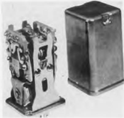
switch circuits are open. One polarity of coil current or unbalance current closes one throw of the switch. Opposite polarity closes the other switch. Rated double-pole sensitivity is 12 mw. The relay measures 2 5/8 in. high above octal or magnal socket by 1 5/8 in. square. Sigma Instruments, Inc., 170 Pearl St., South Braintree, Boston 85, Mass.—TELE-TECH & ELECTRONIC INDUSTRIES.
