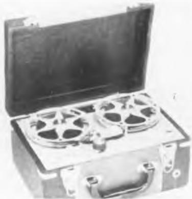
tape speeds with low flutter of  $\pm 0.25\%$  over the full winding cycle of 30 minutes is accomplished by a patented centrifugal flyball governor on the spring motor. Dual track recording provides 2 hr./track or 4 hrs. total playing time on a 5 in. reel that accommodates 600 ft. of standard  $\frac{1}{4}$  in. width tape. **Magnemite Div., Amplifier Corp. of America, 398 Broadway, New York 13, N. Y.—TELE-TECH & ELECTRONIC INDUSTRIES.**
