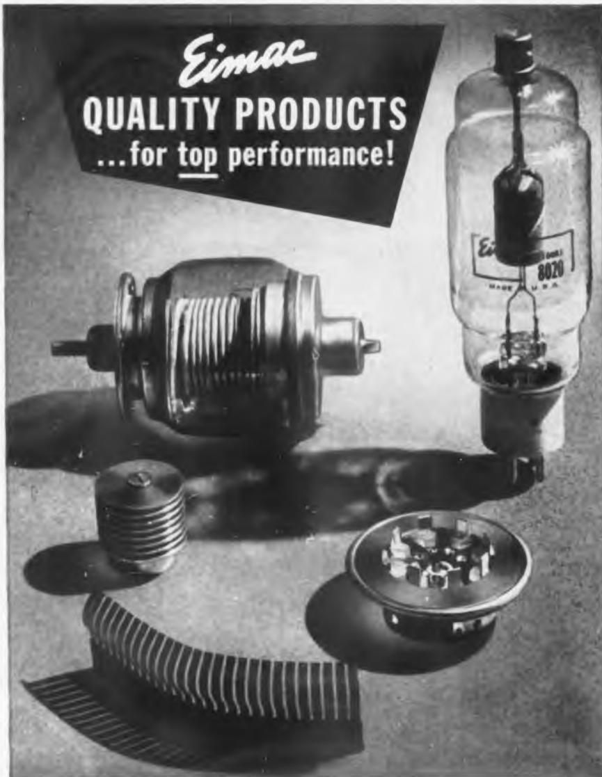
**Preformed Contact Finger Stock** is an ideal electrical weather stripping around doors of equipment cabinets as well as being excellent for use with VHF and UHF circuitry. Silver plated, it comes in three widths— $\frac{1}{8}$ ,  $\frac{3}{16}$  and  $1\frac{1}{16}$  inches.
