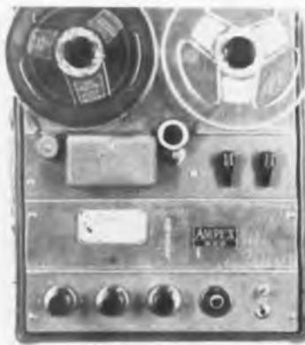
has these performance characteristics: frequency response, 40 to 15,000 cps, signal-to-noise ratio over 55 db, flutter and wow under 0.25%. Timing accuracy within  $\pm 3.6$  secs. for full 30-minute tape length, direct reading meter for record level control, 3 separate heads (erase, record, and playback) and separate record and playback amplifiers. **Ampex Corp., 934 Charter St., Redwood City, Calif.—TELE-TECH & ELECTRONIC INDUSTRIES.**
