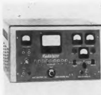
loss or gain, and a receiver frequency of 30 mc. Operating (signal) frequency range is 40 mc to 10  $\mu$ mc—furnished by external equipment under test. Input rating is 50 mv maximum of 30 mc into 50 ohm line. Attenuators are 0-101 db—(steps, 1, 2, 3, 5, 10, 20, 20, 20, 20.) Precision 10-turn potentiometer, 0-10 db, calibrated. **Kay Electric Co., Pine Brook, N. J.—TELE-TECH & ELECTRONIC INDUSTRIES.**
