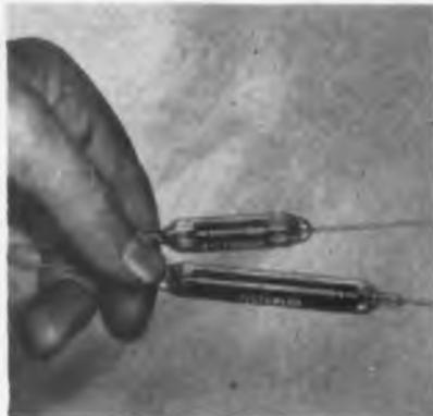
200 kilohms and dissipates up to 5 w. Type RX5 has a rating of 200 ohms to 650 kilohms and is capable of loads up to 10 w. Tolerances can be furnished from a maximum of  $\pm 10\%$  to a minimum of  $\pm 1\%$ . Operating temperature for maintained stability for all three types is listed as from  $-65^\circ$  to  $+225^\circ\text{C}$ . Available in production quantities. Victoreen Instrument Co., 3800 Perkins Ave., Cleveland, O.—TELE-TECH & ELECTRONIC INDUSTRIES.
