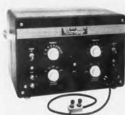
measures their amplitude. Frequency range is from 10 cps to 1 mc continuously variable over decade steps. A low impedance output provides 10 v p-p. At high impedance, 100 v p-p is available. A 60 db step attenuator and 20 db continuous attenuator enables use of the generator as a voltage calibrator. **New London Instrument Co., P. O. Box 189, New London, Conn.—TELE-TECH & ELECTRONIC INDUSTRIES.**
