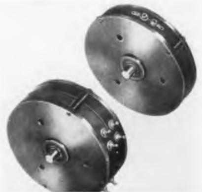
drical Kohlrausch winding. Ganging is accomplished by interlocking surfaces rigidly secured by threaded tie rods. Housing is one-piece molded BM17748 Bakelite. Phasing can be accomplished by staggering housings in  $90^\circ$  increments, or unit contact brushes can be phased to keep end and collector terminals in alignment. **DeJUR-Amsco Corp., 45-01 Northern Blvd., Long Island City 1, N. Y.—TELE-TECH & ELECTRONIC INDUSTRIES.**
