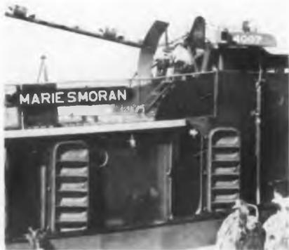
Tugboat lowers mast to duck under low bridges. The vessel's radar transmitter and receiver is built entirely within the vessel's antenna housing
