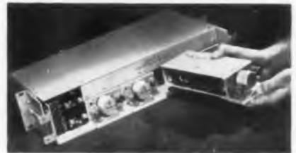
Fig. 6: Single units plug into shelf assembly
