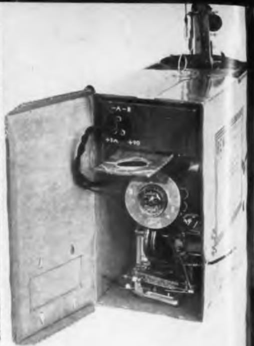
Radiosonde is suspended from a free balloon and telemeters data on weather conditions
