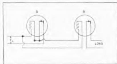
Fig. 8: Timing is made independent of voltage
