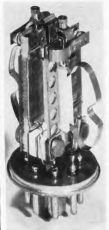
Fig. 3: (l) Bimetal element at left bends in proportion to heat until contact is made. Fig. 4: (r) Relay in which heater voltage has little effect on timing
