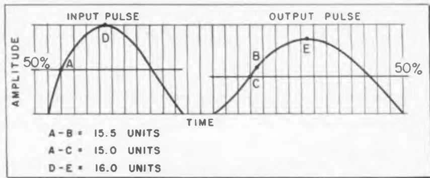
Fig. 3: Three time measurements on same delay line. Rise and decay times are exaggerated
