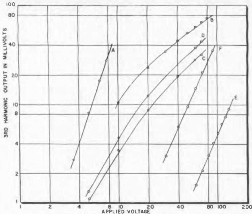
Fig. 5: Third harmonic content measured for A—Thyrite resistor; B—Resistor F  $\frac{1}{2}$ -2-12; C—Resistor F  $\frac{1}{2}$ -1-10; D—"C" packed in dry ice; E—Resistor A  $\frac{1}{2}$ -1-10; F—Resistor B  $\frac{1}{2}$ -1-10
