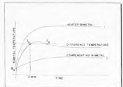
Fig. 6: Curve for ambient-compensated relay
