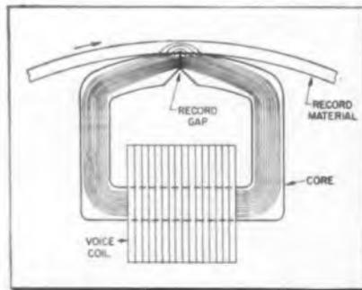
Lines of flux in record head and gap
