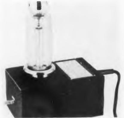
tential divider with most CRO's for displaying high potential waveforms. An applied voltage is attenuated 10,000 to 1 with 2% accuracy between 60 cps and 6mc. Connection is made to an associated instrument by a 6 ft. cable. Input capacitance is 3.8 µmf. Shunt resistance is above 10<sup>6</sup> megohms. **Ballantine Laboratories Boonton, N. J.**—TELE-TECH & ELECTRONIC INDUSTRIES.
