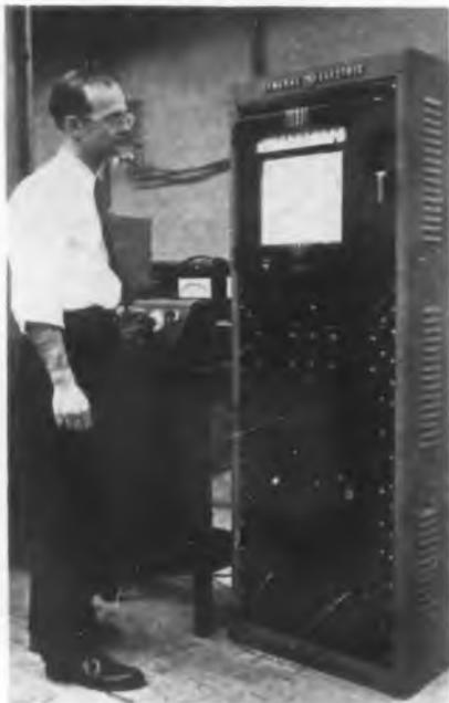
This recording hysteresis graph in the Carboly Dept. of GE in Detroit makes a complete record of a magnet's entire hysteresis loop automatically. Any part of loop is explored at will
