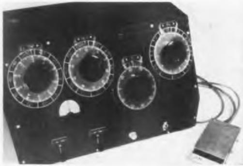
Analogue computer for solving the radio refractive index equation, a product of CPRL research
