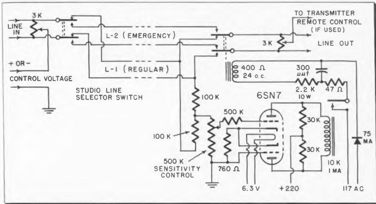
Automatic changeover circuit switches program and control circuits simultaneously to emergency loop in case of line failure
