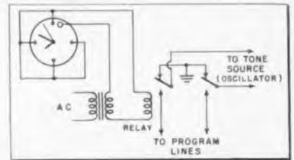
Minute and second hands open and close this circuit to provide quarter-hour timing signals
