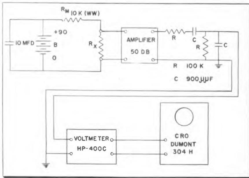
Fig. 6: Noise measurements. Noise voltage generated by resistor is first amplified and filtered
