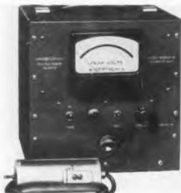
to-peak voltage of a wave form. Voltage range of the unit is 100 v full scale; with available multipliers, to 30 kv. The measuring elements are housed in a probe to allow direct connection to the voltage source. **Gertsch Products Inc., 11846 Mississippi Ave., Los Angeles 25, Calif.—TELE-TECH & ELECTRONIC INDUSTRIES.**
