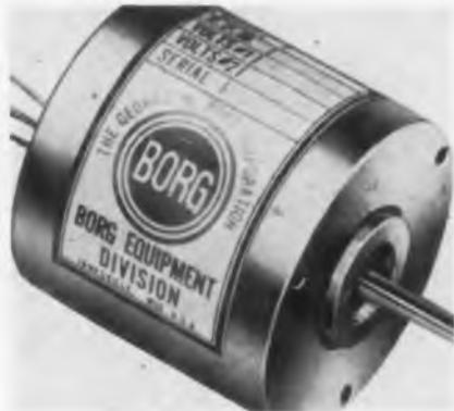
oz.-in. in either direction when operated at 115 v. Mounts firmly with three mounting screws tapped into the housing. Induction type, 2 phase, 115 v, 400 cps, 5500 rpm no-load speed. **Borg Equipment Div., The George W. Borg Corporation, 120 S. Main St., Janesville, Wis.—TELE-TECH & ELECTRONIC INDUSTRIES.**
