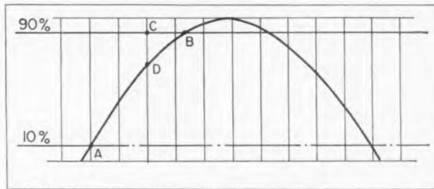
Fig. 5: Reference points for measurement of pulse rise time. Decay time will be identical
