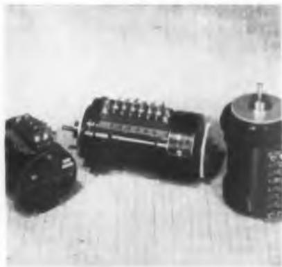
ture range of  $-65^{\circ}$  to  $+165^{\circ}$  F. They are also designed for a maximum torque of 16 oz.-in. and for intermittent duty at speeds to 1,000 rpm. Life expectancy, 200,000 cycles at 30 rpm with load inertia of 1 oz.-in. Weights, single clutch, 0.8 lbs., double clutch, 1.5 lbs., clutch brake 1.2 lbs. Electrical requirement 25 v dc. **Ford Instrument Co., Div. of Sperry Corp., 31-10 Thomson Ave., Long Island City 1, N. Y.—TELE-TECH & ELECTRONIC INDUSTRIES.**
