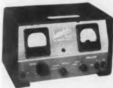
strength meter. A built-in speaker is provided for aural checking of transmitter quality, and an oscilloscope connection enables one to "see" the modulation. Dimensions: 7 x 12 x 7¼ in. Weight, 14 lbs. **Lampkin Laboratories, Inc., Bradenton 17, Florida.—TELE-TECH & ELECTRONIC INDUSTRIES.**
