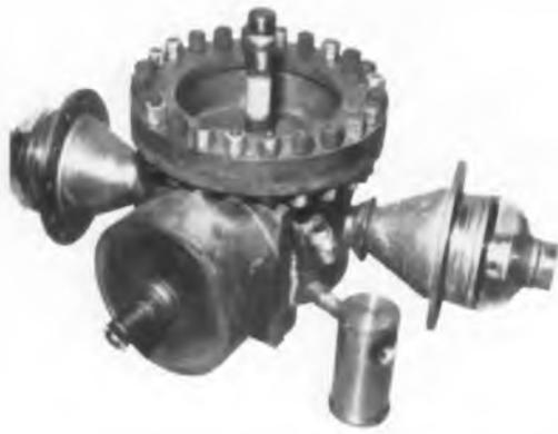
Fig. 1: Complete magnetron assembly has two outputs and tuning cavity coupled to anode cavity
