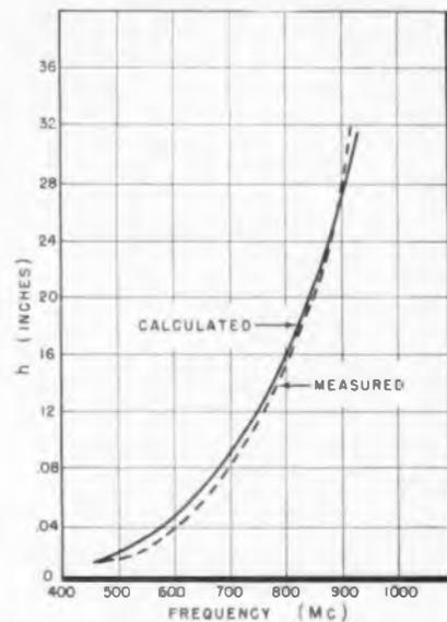
Fig. 10: Curves of frequency vs. plate spacing
