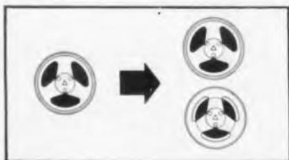
**EXTRA THIN TAPE**—50% thinner, more potent oxide coating, 30% thinner backing permit more 190A tape to be wound on standard-size reel. Result: one roll of new tape does job of 1½ reels of standard tape.
