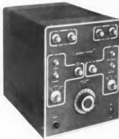
Fig. 1: Marker-Pulser for delay-line testing
