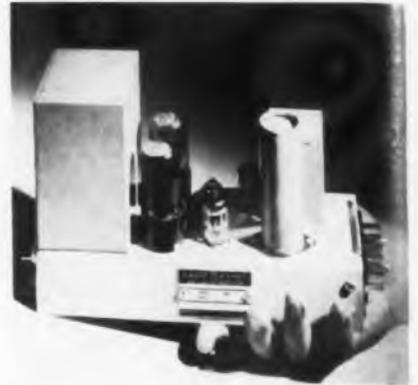
the output will be compressed for incoming signals exceeding the preset level and expanded for signals below it. Differences between recordings, film projectors, microphones, or network signals are automatically controlled so that the amplifier audio output level remains relatively constant without apparent sound distortion. **General Electric Co., Electronics Park, Syracuse, N. Y.—TELE-TECH & ELECTRONIC INDUSTRIES.**
