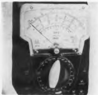
resistances from 0.1 ohms to 150 megohms-decibel and output readings. VTVM, four, including 1.2 volt range for grid voltage and accurate discriminator alignment. First division mark at 0.02 v. Sensitivity, V-O-M, 20,000 ohms v on dc, 500 ohms/v on ac; VTVM, 11 megohms. One switch selects all ranges. **Triplet Electrical Instrument Co., 122 Main St., Bluffton, Ohio.—TELE-TECH & ELECTRONIC INDUSTRIES.**
