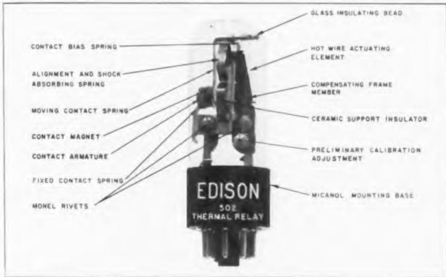
Fig. 1: Hermetically sealed thermal relay employing direct expansion element of hot wire type
