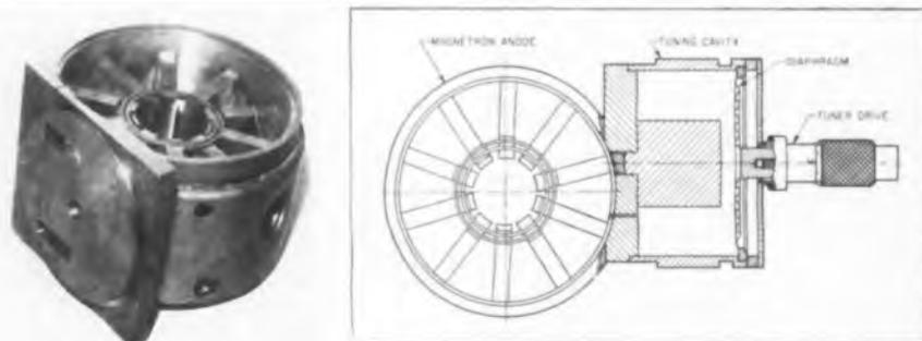
Fig. 2: (l) Ten-cavity, vane-type anode Fig. 3: (r) Tuning cavity is coupled to anode resonator
