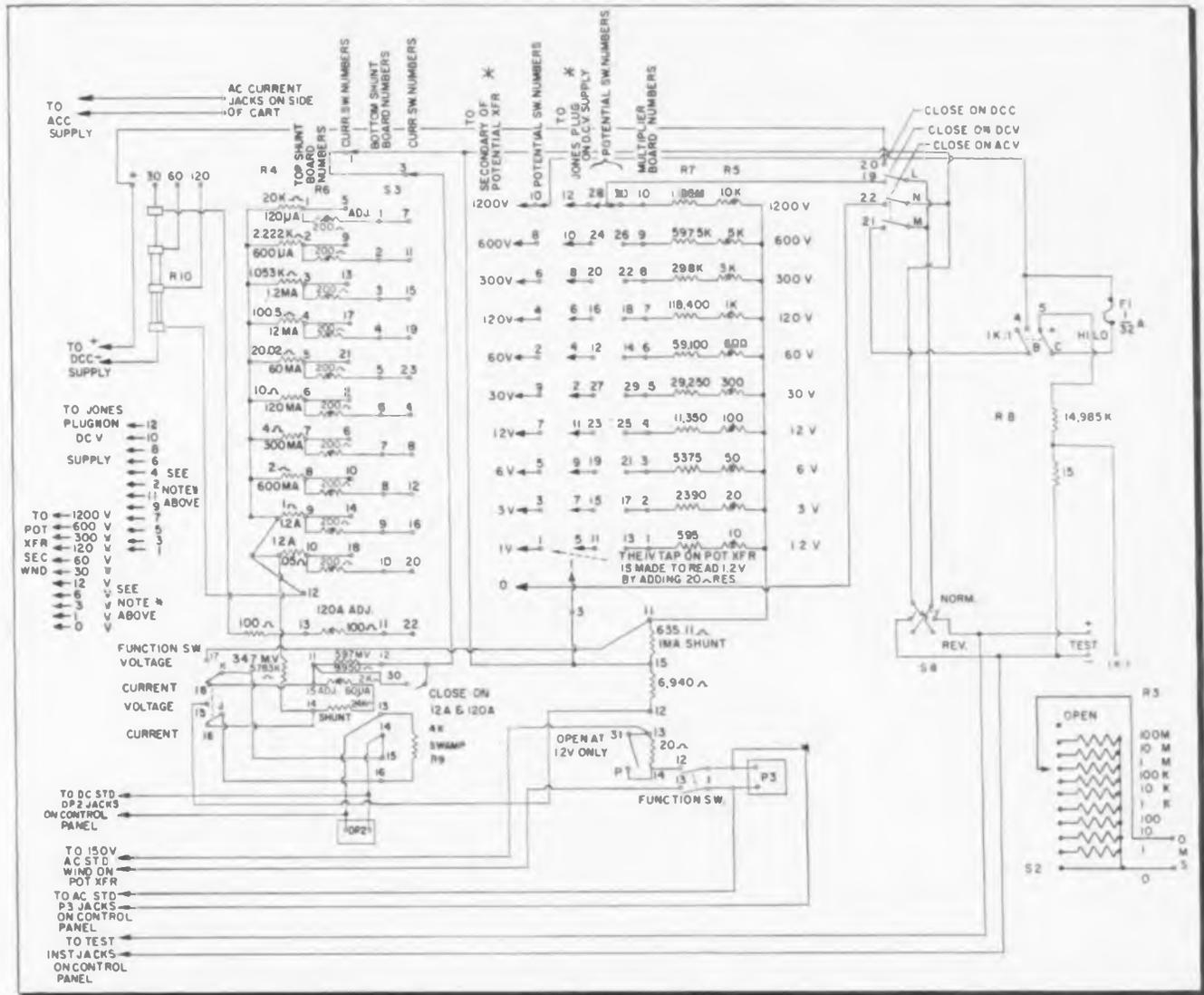
Fig. 5: Schematic diagram of measuring circuit and secondary power distribution
