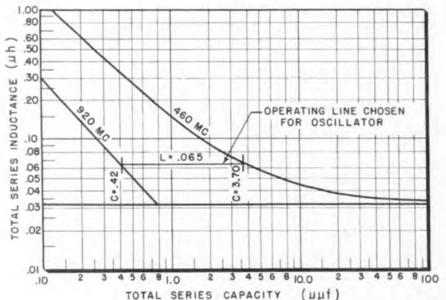
Fig. 1: Capacity variation required vs. series external inductance
