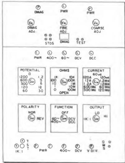
Fig. 6: Front panel layout of calibrating cart
