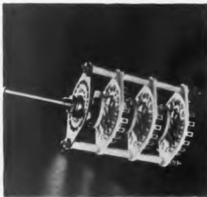
ing, power supply converter, and other special applications. Rated at 750 w at sea level ( $7\frac{1}{2}$  amps, 60 cps, 115 v ac), 375 w at 35,000 ft. Has been used up to 20 mc. Breakdown point, 3,000 v RMS—60 cps. The unit is available in 1 pole 2 to 17 positions per section or 3 pole 2 to 5 positions per section up to six sections. Centralab, Div. of Globe-Union Inc., 900 E. Keefe Ave., Milwaukee 1, Wis.—TELE-TECH & ELECTRONIC INDUSTRIES.
