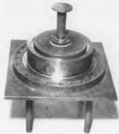
Fig. 6: Cathode is mounted in top cover assembly
