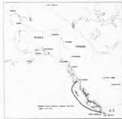
cation filed with the F.C.C. sets the terminal points of the cable as Port Angeles, Washington and Ketchikan, Alaska, a distance of 800 nautical miles. Present telephone service between Alaska and the U. S. is provided over 13 radio and land line circuits.
