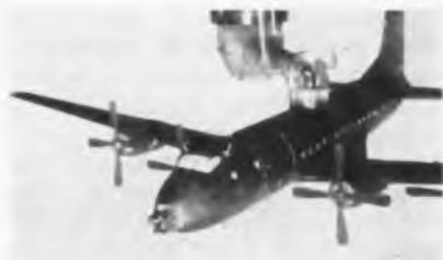
Fig. 4: Cut outs simulate glass windows
