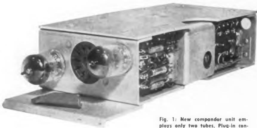
Fig. 1: New compandor unit employs only two tubes. Plug-in construction allows easy replacement
