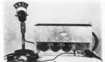
Fig. 4: Simply constructed remote equipment with recessed knobs ready for sportscast
