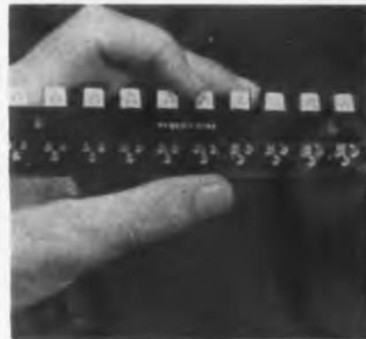
larly in computer circuitry. Dimensions of the first model which has 10 sockets are 6 x 1 x 1/4-in. Other models are being developed to accommodate 30 or more sockets in a single phenolic strip. Contacts are phosphor bronze. Solder contacts are copper. **Hydro-Aire, Inc., Electronics Div., 3000 Winona Ave., Burbank, Calif.—TELE-TECH & ELECTRONIC INDUSTRIES.**
