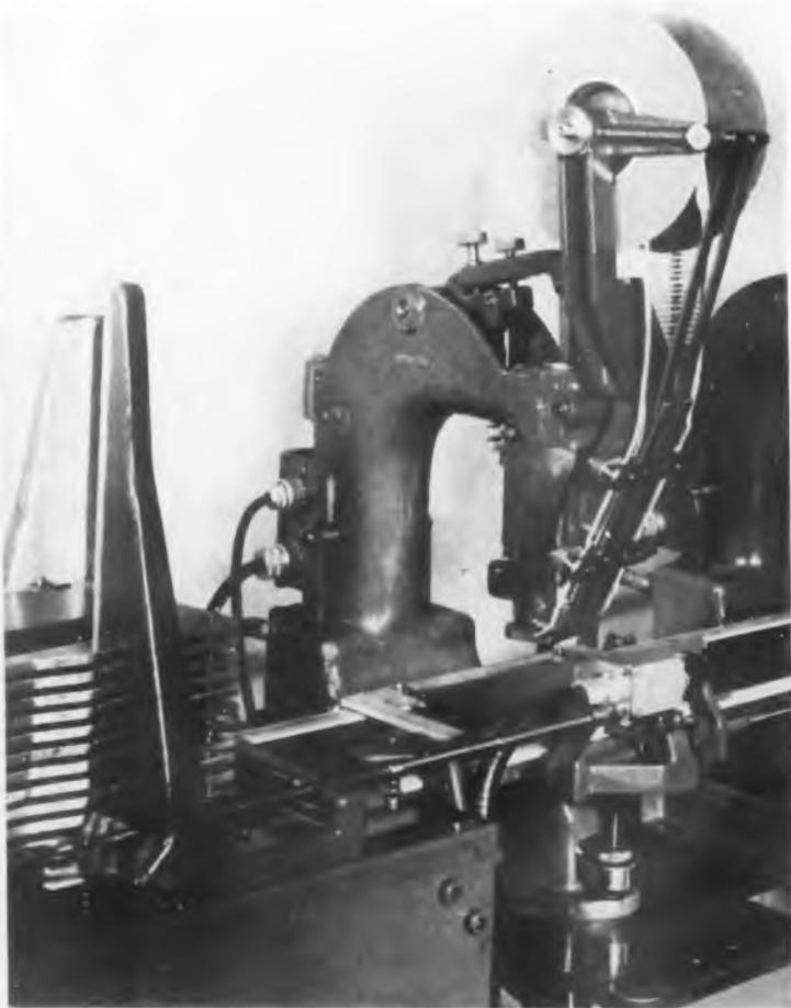
Close-up of one station in automatic production system developed by United Shoe Machinery Corp., Boston, Mass. Printed wiring boards with pre-punched holes are conveyed from pallets at left to inserting head. Components on tape belt are fed from reel at upper right. Head automatically cuts and forms component leads and inserts them in holes. Board then moves to next station. See p. 88 for details
