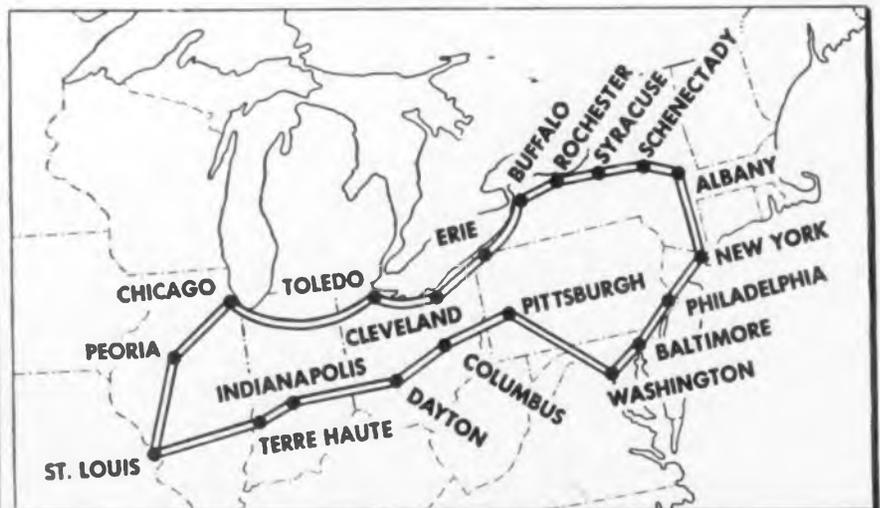
New television pathway, 2,400 miles long, links stations in the northeastern quarter of the U.S. Network provides four video channels, two in each direction, along radio relay route extending from N.Y. to Chicago, via Buffalo and back through St. Louis, Pittsburgh and Washington. Any station in the loop can transmit to or receive programs from other loop stations with minimum of switching
