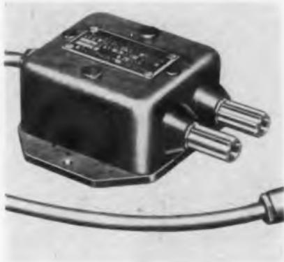
connected to the Q Meter—is 500 ohms; output impedance—provided by voltage injection circuit of Q meter—0.3 ohms; frequency range 1 kc to 50 kc; input voltage requirements—variable up to 22 v. Case is 1¼ x 2½ x 3¾ in. Provides binding posts for connecting the external oscillator; also a coaxial cable and BNC connector to the Q meter. **Boonton Radio Corp., Boonton, N. J.—TELE-TECH & ELECTRONIC INDUSTRIES.**
