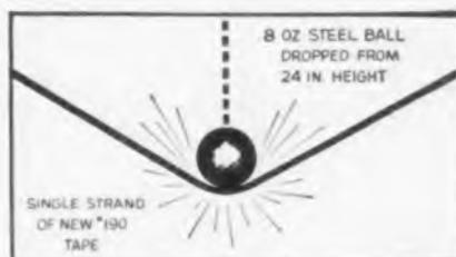
**STRENGTH TO SPARE**—New 190A tape stands up under even grueling steel ball drop test. Naturally it’s tough enough to withstand severe stresses of sudden machine stops, starts and reverses.
