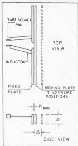
Fig. 3: Oscillator tank circuit assembly
