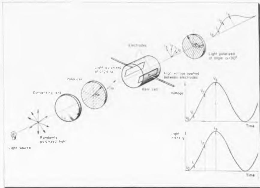
Fig. 3: Method of modulating light beam. Receiver sensitivity is also varied at same frequency
