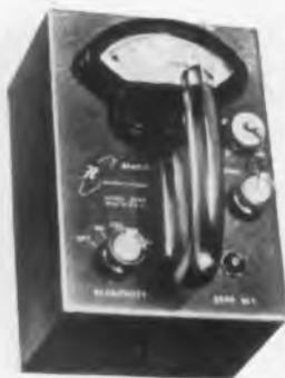
dow protected by a stainless steel grill. Three alpha ranges cover any count rate from 0 to 12,500 counts/min. corresponding to radium gamma ranges of approximately 0 to 18 milliroentgens/hr. The unit will detect alphas with energies as low as 1.0 mev; betas as low as 15 kev. **Nuclear Instrument & Chemical Corp., 223-233 W. Erie St., Chicago 10, Ill.**—TELE-TECH & ELECTRONIC INDUSTRIES.
