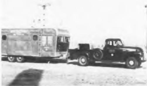
Mobile research unit is used to determine the range of transmitted signals and interference
