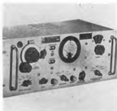
cillator covering a frequency range of 10 to 1,100 kc in five bands. The three variable adapters have maximum resistance values of 500k, 50k, and 5k. Two other adapters are furnished that enable testing crystal units contained in HC-5 U and octal base holders. **Radio Frequency Laboratories, Inc., Engineering Dept., Boonton 20, N. J.—TELE-TECH & ELECTRONIC INDUSTRIES.**
