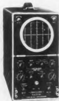
response of 20 cps to 500 kc within 2 db. Vertical square wave response is from 20 cps to 50 kc; frequency response, 20 cps to 200 kc within 3 db (at full gain); 1 v, peak-to-peak, vertical, built-in calibrator. Internal linear sweep 10 cps to 30 kc. Negative and positive sweep sync. **Precision Apparatus Co., Inc., 92-27 Horace Harding Blvd., Elmhurst 6, L. I., N. Y.**—TELE-TECH & ELECTRONIC INDUSTRIES.
