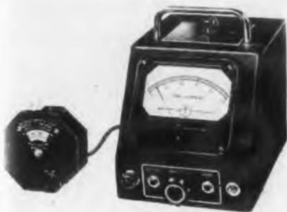
use with a sweep-frequency generator, wavemeter or heterodyne frequency meter and as a low sensitivity receiver or field-strength meter for tracing sources of spurious oscillations in receivers and transmitters. Rated at 30 w. Operates from 117 v, 60 cps. Employs separate power supply and indicating unit. **Measurements Corporation, Thomas A. Edison Subsidiary, 116 Monroe St., Boonton, N.J.—TELE-TECH & ELECTRONIC INDUSTRIES.**
