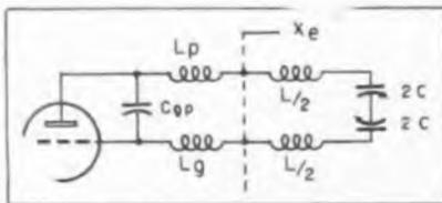
Fig. 8: Equivalent tank circuit of oscillator
