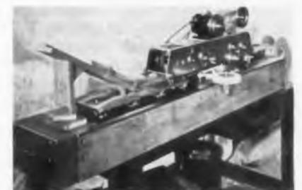
Key to automatic insertion of axial lead components is belting machine which feeds parts through lead straightening and taping sections. Belted components are then wound on reel
