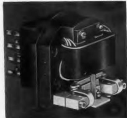
meet specified performances. Coils are in four sections. Sensitivity as low as 2 ma can be obtained by placing all coil windings in series-aiding. "Break-to-make" travel time, when the armature is in transit touching neither contact, varies with the degree of energization of the operating windings. Automatic Electric Co., 1033 West Van Buren St., Chicago 7, Ill.—TELE-TECH & ELECTRONIC INDUSTRIES.
