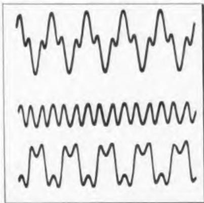
Fig. 3: Two typical third harmonic voltages
