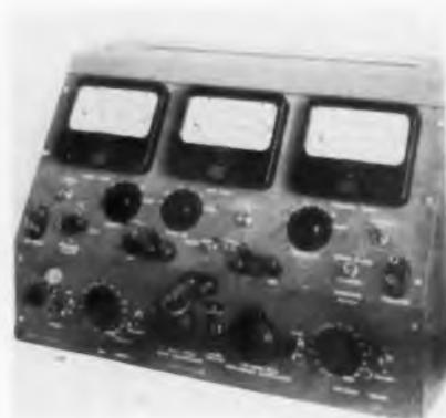
at low frequencies. Generally, small signal T-equivalent-circuit parameters are the basis for transistor operation analysis and design. The new instrument makes direct measurements of these parameters. **Armour Research Foundation of Illinois Institute of Technology, Technology Center, Chicago 16, Ill.—TELE-TECH & ELECTRONIC INDUSTRIES.**
