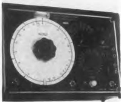
Salient features are direct reading of vector magnitude and phase angle. Because the phase arm presents 1,000 ohms impedance regardless of position of phase switch, the phase arm and magnitude can be varied without interaction. The prominent reactive component can be determined as capacitive or inductive by noting the position of the function switch that null is detected. **Republic Engineering Co. Inc., Beltsville, Md.**—TELE-TECH & ELECTRONIC INDUSTRIES.
