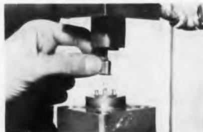
Header with rate grown transistor and attached end leads and base lead is placed in main seal welding machine to protect assembly. Later air will be exhausted from the device
