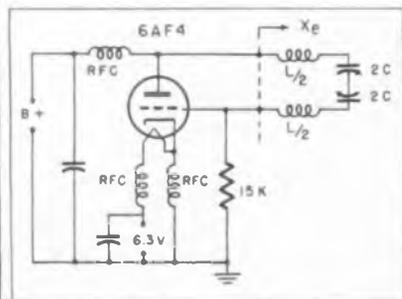
Fig. 7: Modified Colpitts oscillator circuit
