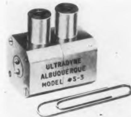
metering systems. When the gage is connected in an electrical bridge circuit, the output signal is proportional to the input pressure. The unit features 50 μsec rise time, 1% or less non-linearity, 0.1 to 0.4% hysteresis, 0.3% acceleration sensitivity, 0.01% F. zero shift with temperature. Weighs 2 oz. and is 3/4 x 3/4 x 1 1/8 in. in size. **Ultradyn Engineering Labs., Inc., P.O. Box 8007, Albuquerque, New Mexico.—TELE-TECH & ELECTRONIC INDUSTRIES.**
