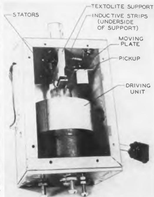
Fig. 4: (r) Oscillator with side plate removed. The stators and inductors are supported by textolite
