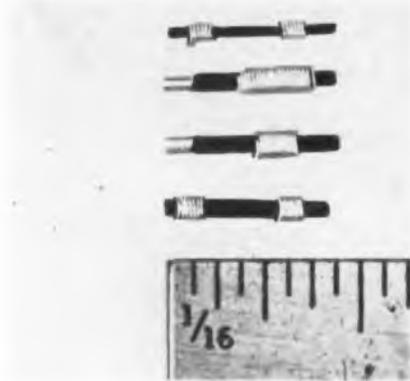
dielectric constant of 2.0 at all operating frequencies. Power factor at all operating frequencies is 0.0005. Moisture absorption factor is zero. Silver plated terminals allow soldering directly into circuits, but leads can be furnished if desired. **Anchor Radio Corp., 2215 S. St. Louis Ave., Chicago 23, Ill.—TELE-TECH & ELECTRONIC INDUSTRIES.**
