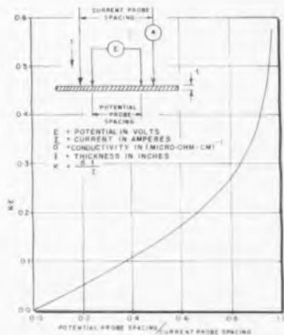
Fig. 4: Probe spacing is determined by potential
