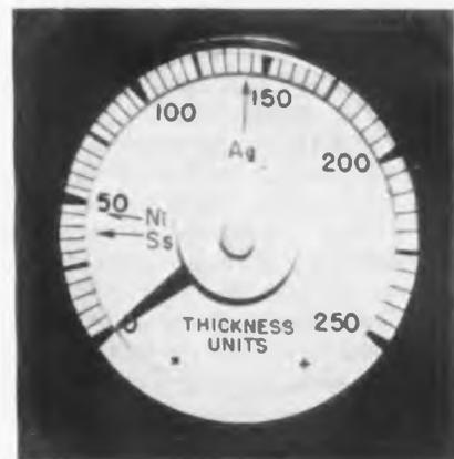
Fig. 6: Meter scale is in units of 0.001 in.
