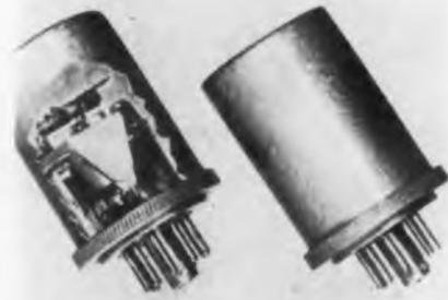
infinite for 0.2  $\mu$ a to 10 amps, or 0.1 mv to 500 v. Higher volts or ampere sensitivities with external multipliers. Accuracy, trip point to 1.0%; differential, less than 1.0%. Response time 50 sec. to 5 second time delay. Contacts, SPST or SPDT. Standard rating 5 to 25 ma; dc.; other ratings to 1/2 amp. Weight, 4 oz. Assembly Products, Inc., Main at Bell St., Chagrin Falls, O.—TELE-TECH & ELECTRONIC INDUSTRIES.
