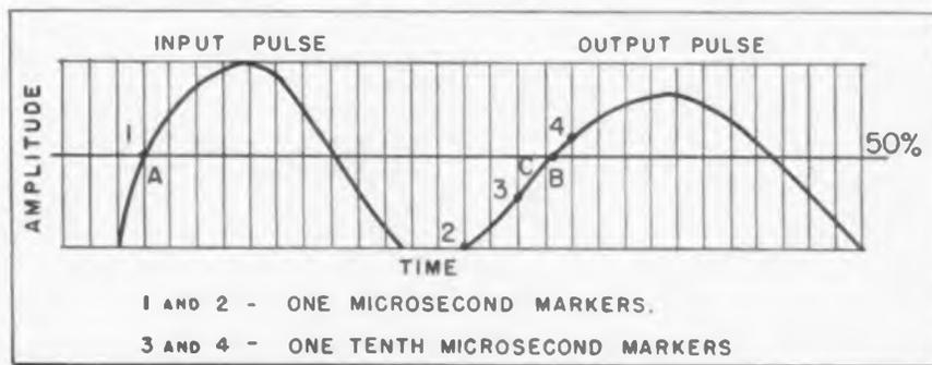
Fig. 4: Reference points for marker adjustments as seen against background of scope graticule
