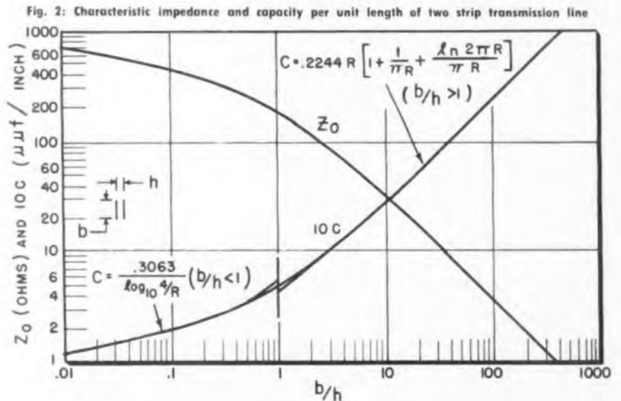
Fig. 2: Characteristic impedance and capacity per unit length of two strip transmission line
