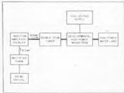
Fig. 9: Set-up for double-loop injection tests
