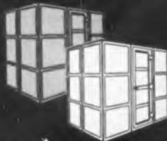
An economical enclosure, available in copper or galvanized wire cloth, that meets basic requirements for suppressing r-f radiations of industrial or laboratory equipment. Copper Screen: 70db from 100kc to 1000mc, 40db at 14kc. Galvanized Screen: 40db from 15kc to 400mc (Uniform-Field measurements).
