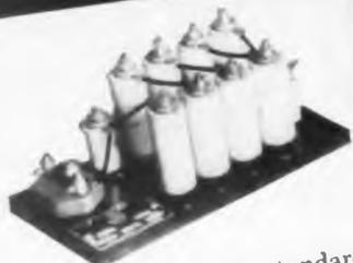
Rust offers many standard metering units which sample any voltages or currents. By *investigating* you will find that Rust metering units use only precision wire-wound resistors of low temperature coefficient to provide readings of high accuracy and stability. Shown is the 108-8A, 0-2000v dc metering unit.
