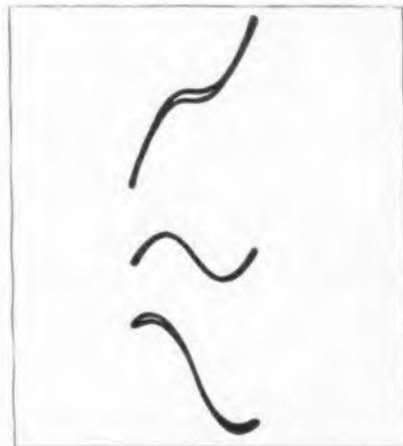
Fig. 5: Lissajous figures at balance point
