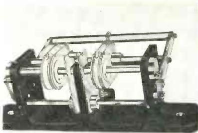
Fig. 1: Foot-operated machine for lead tailoring now being manufactured
