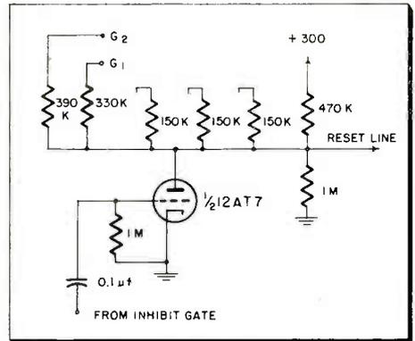
Fig. 7: (l) Reset with switch tube which cuts off when signal appears, allowing reset line to drift up. Fig. 8: (r) Similar "forced" reset switches 200 volts to line
