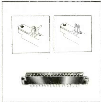
two terminal styles; (1) a slotted eyelet for soldering up to three No. 20 AWG cable wires per contact (2) a plain terminal to permit wire wrapping by the Western Electric Co. "Wire-Wrap" tool. Contact mv. drop is 10.5 dc at 3 amps rated current. Gold plating over silver provides low electrical resistance, corrosion prevention, and soldering ease. Winchester Electronics, Inc., Willard Rd., Norwalk, Conn.—TELE-TECH & ELECTRONIC INDUSTRIES. (Ask for 12-19)
