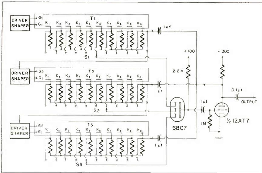
Fig. 9: Cascaded 10-count tube circuit for counting up to 1000
