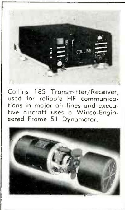
Collins 185 Transmitter/Receiver, used for reliable HF communications in major air-lines and executive aircraft uses a Winco-Engineered Frame 51 Dynamotor.
