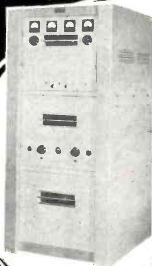
Designed to meet all customer and F.C.C. requirements in the specially assigned paging service bands of 35.58 and 43.58 megacycles.
