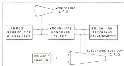
Fig. 5: Block diagram of equipment and circuitry used for frequency analysis
