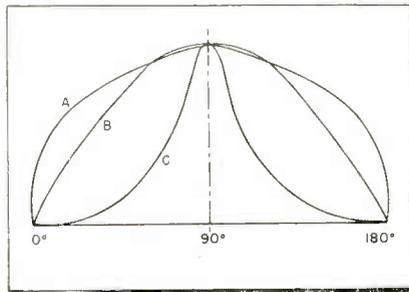
Fig. 2: Low-current curves are due to inaccuracy. A) Copper oxide rectifier vs ac sine current; B) Sinewave; C) rectifier vs ac sine voltage
