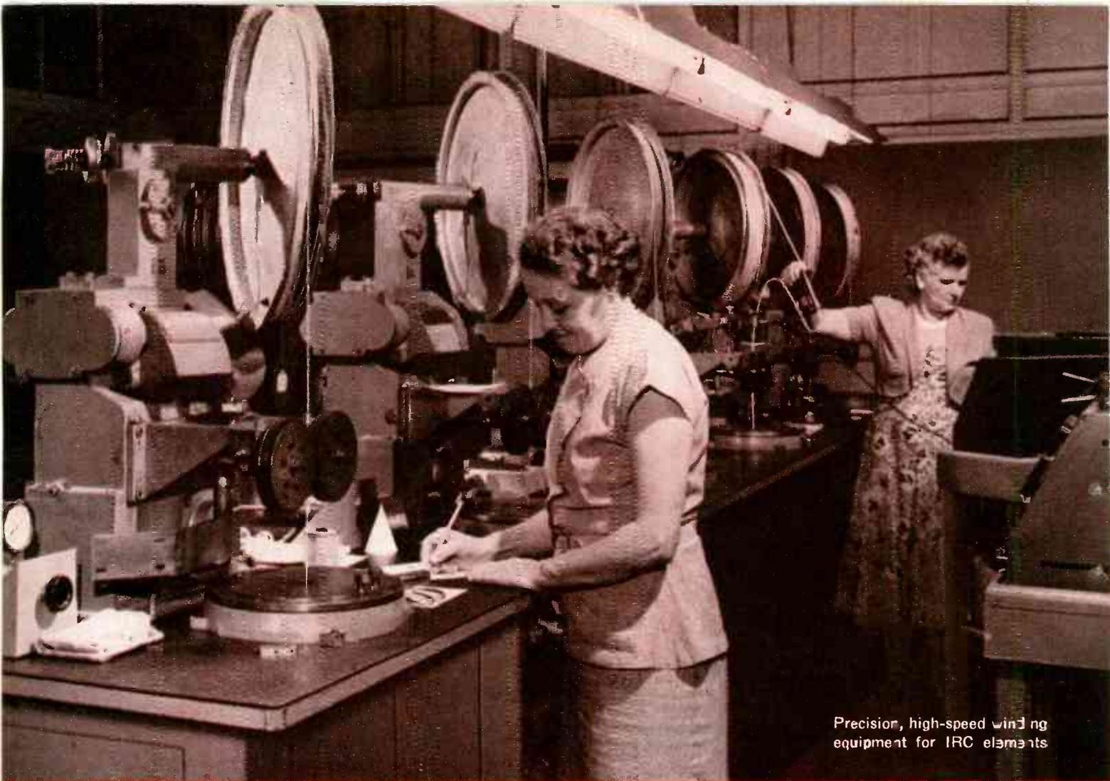
Precision, high-speed winding equipment for IRC elements
