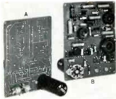
Fig. 1: Top & bottom views of printed circuit frequency standard show component arrangement
