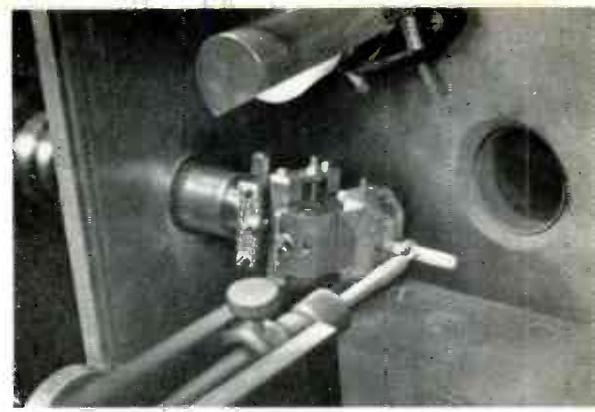
(l) Cutting a continuous spiral groove in a deposited carbon film resistor, using a straight nozzle with 0.006 x 0.06 in. rectangular orifice. Cut width is 0.007 in. (r) Cutting and shaping cylindrical crystals used in neutron diffraction. Sizes are as small as fraction of mm dia., and 1.5 cm long
