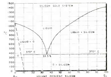
Fig. 7: Gold-silicon phase diagram
