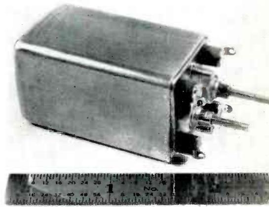
Fig. 1: Stabilized i-f transformer in can
