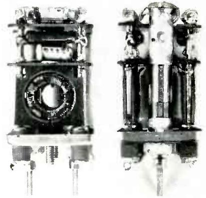
Fig. 3: (l) I-F transformer construction details, showing toroidal coil and resistors. Fig. 4: (r) View showing unit's plunger capacitor
