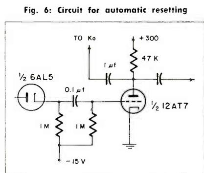
Fig. 6: Circuit for automatic resetting
