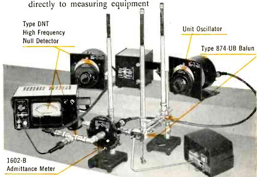
The Type 1602-B Admittance Meter and Balun setup to measure admittance or impedance of converter input. One Type 1208-A Unit Oscillator supplies the vhf power, while the local oscillator in the Type DNT Null Detector Assembly beats with the Admittance Meter output to provide a 30-Mc difference frequency. This signal is detected by the new Type 1216-A Unit I-F Amplifier, also an element of the Null Detector Assembly.
