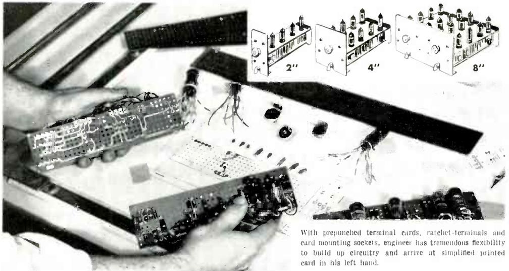
With prepunched terminal cards, ratchet-terminals and card mounting sockets, engineer has tremendous flexibility to build up circuitry and arrive at simplified printed card in his left hand.
