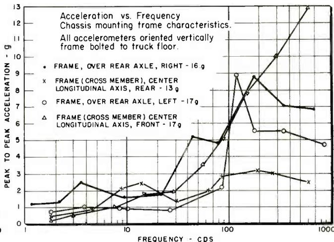
Fig. 8: (l) Acceleration spectrum of radio chassis during test. Fig. 9: (r) Acceleration spectrum of mounting frame during test
