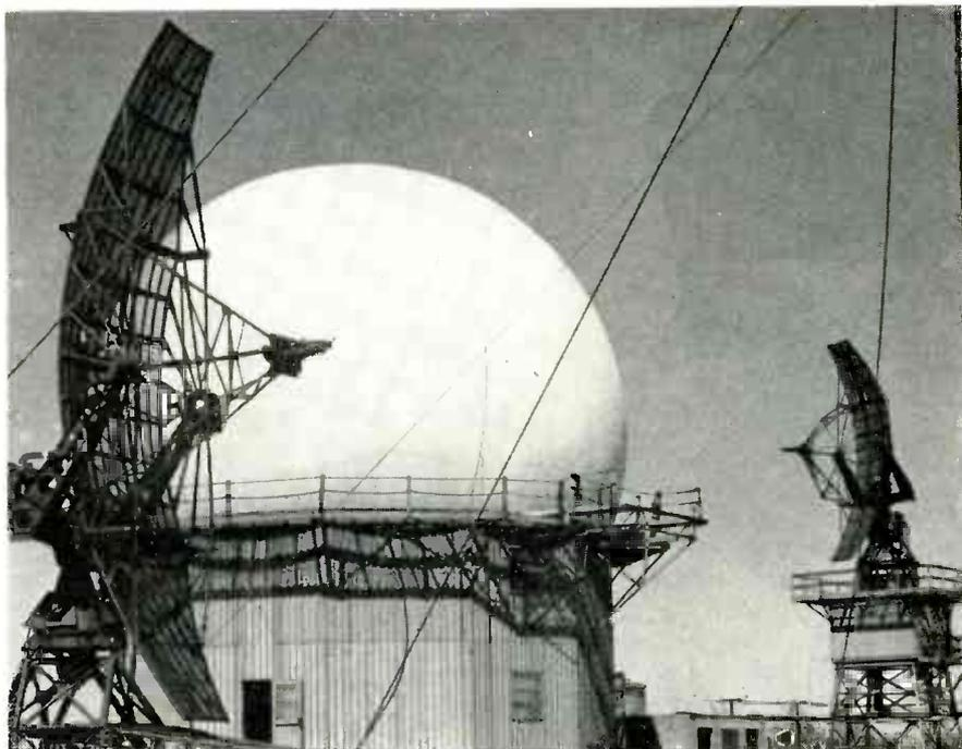
Three versions of new radar height finder made for U.S. Air Force are (l) mobile unit, (c) radome for radar in Arctic climates, and (r) unit for fixed installations in temperate regions
