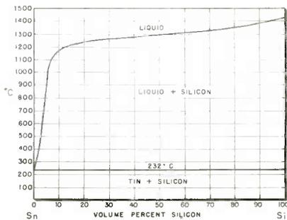
Fig. 1: Phase diagram of silicon-tin system
