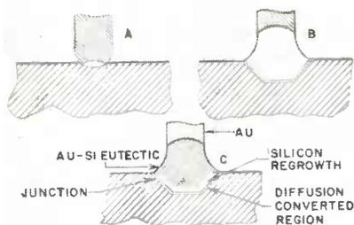
Fig. 8: Diagram of fusion mechanism
