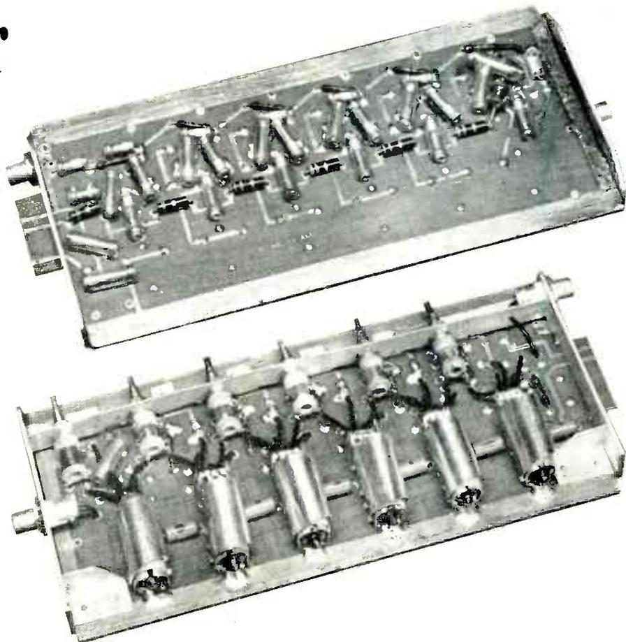
Fig. 2: (Above) Photo of both sides of seven inch unit with cover removed. Design features high reliability, simplified production and circuit uniformity. Fig. 3: (I) Cover plates are held together by sliding clips, not screws
