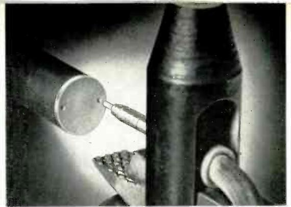
(l) Cutting a 24-pitch thread on inside wall of glass tubing having ID of  $\frac{1}{2}$  in., using right angle nozzle with 0.006 x 0.06 in. rectangular orifice. Similar helices have been cut in ceramic tubing with 0.17 ID. (r) Drilling depression in quartz disc. Hole is 0.03 in. dia., 0.015 in. deep.
