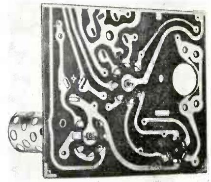
which enables printing jumpers to connect different pin positions. Static load tests indicate that, when properly dip-soldered in a multiple hole pattern in a printed wiring panel, the socket will withstand a force of 10 times normal tube withdrawal force. Available in 7 or 9 pin types. Methode Mfg. Corp., 2021 W. Churchill, Chicago, Ill.—TELE-TECH & ELECTRONIC INDUSTRIES. (Ask for 12-27)
