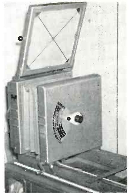
Fig. 2: Printed circuit distortionless camera
