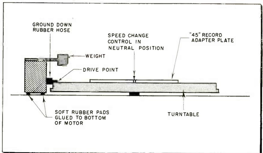
Diagram showing 45 rpm conversion details to Fairchild 254
