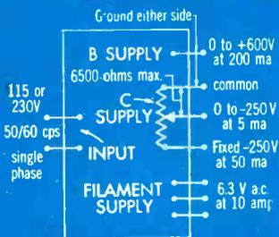
Flexible ground permits stacking of supplies to provide up to  $-600V$ . cathode voltage and an additional 0 to  $-250V$ . for the reflector of low voltage klystrons.
