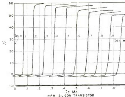
Fig. 12: Characteristic curves of fairly good silicon transistor with alpha 0.9
