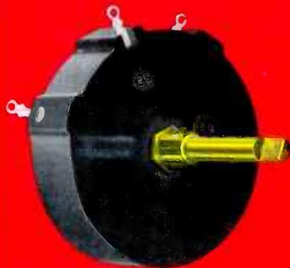
High voltage control for focus applications. Rated up to 5,000 volts DC across end terminals and 2 1/2 watts depending on total resistance. Will operate up to 15,000 volts DC above ground when mounted on insulated panel. CTS type 85.
