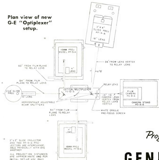
**CAPABLE OF HANDLING FOUR PROJECTION SOURCES** as illustrated at left in conjunction with the new G-E "Optiplexer". By using this highly efficient optical system there's *no need to flip mirrors!* And, the new G-E Vidicon channel offers a choice of monitors... 1. Studio console type. 2. Lightweight portable design.
