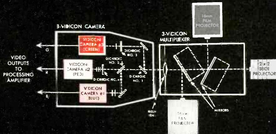
\*Close-up view of the TK-26A — RCA's remarkable 3-V Color Film Camera. Heart of the 3-V is the revolutionary new, inexpensive Vidicon Camera tube — RCA-6326!
