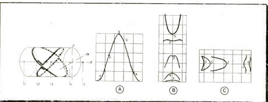
Fig. 5: Magnetic field plots for crossed field coils.
