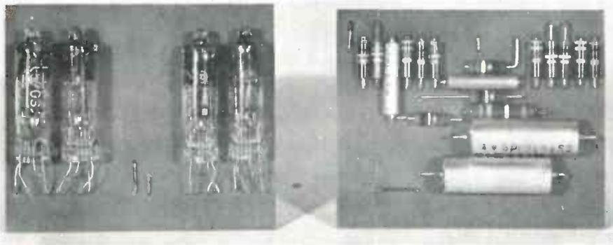
Fig. 2c: Reverse side of boards in Fig. 2b shows tubes and components connected to wiring
