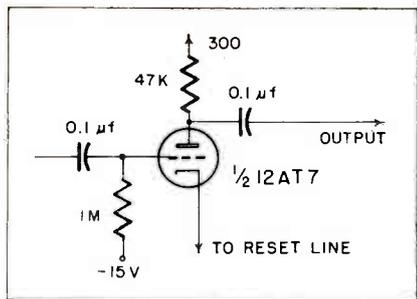
Fig. 5: Inhibit gate eliminates positive pulse
