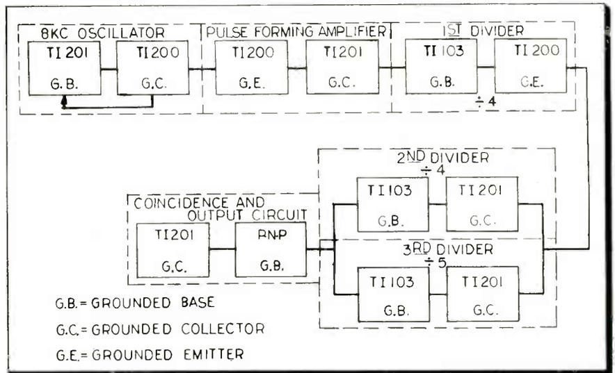
Fig. 2: Counting circuit with oscillator, dividers, pulse forming amplifier and coincidence circuit
