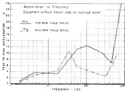
Fig. 11: Spectrum of equipment without transit case measured on package tester
