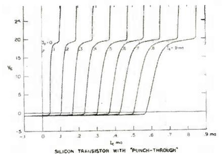
Fig. 6: "Punch-through" curve characteristics of a tin silicon fusion transistor
