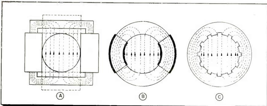
Fig. 2: (A) Using square or rectangular core is simplest way to obtain uniform deflecting field. (B) Ring core is better but requires cosine winding to restore field uniformity (C) More recent and still better approach is in castellated core
