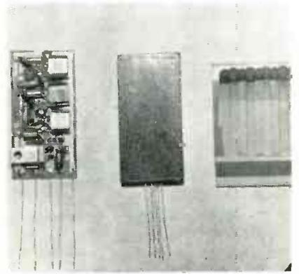
sistors. The printed unit is now available in sample quantities with solder terminals, or as a plug-in device. Size,  $\frac{1}{2}$  x 1 x 2 in. Weight, less than  $\frac{1}{2}$  oz. Input impedance, 400 to 1,200 ohms; output impedance, 120 to 2,000 ohms. Power output, 73 mw. Sensitivity, 500  $\mu\text{v}$ . Power source, 28 v. dc. Plastics & Electronics Corp., 272 Northland Ave., Buffalo 8, N.Y.—TELE-TECH & ELECTRONIC INDUSTRIES. (Ask for 12-23)
