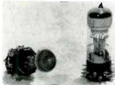
Fig. 10: Multi-element glow transfer tube
