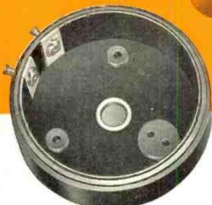
**Good Linearity at Moderate Cost** Resistance wire is uniformly wound and finished card is cemented tightly into base — uniform thickness around base prevents unequal curing and aging out of round — every unit produced is inspected for conformance with linearity specifications.
