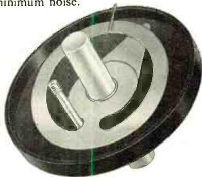
**Bearing Durability** Bearings are at extreme ends of enclosure for greatest mechanical stability — brush arm is positively keyed to hub which rotates on brass insert; this bearing is in the same plane as brush, and is closely fitted, minimizing effects of side thrust on shaft — other end of shaft is guided by stainless-steel insert molded in base.
