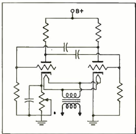
Fig. 7: Multivibrator, using variable bias
