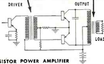
CLASS B TRANSISTOR POWER AMPLIFIER
