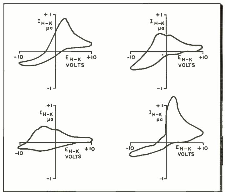
Fig. 4: Leakage with below 10 v between h & k
