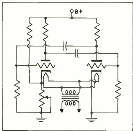
Fig. 8: Voltage divider bias lowers leakage
