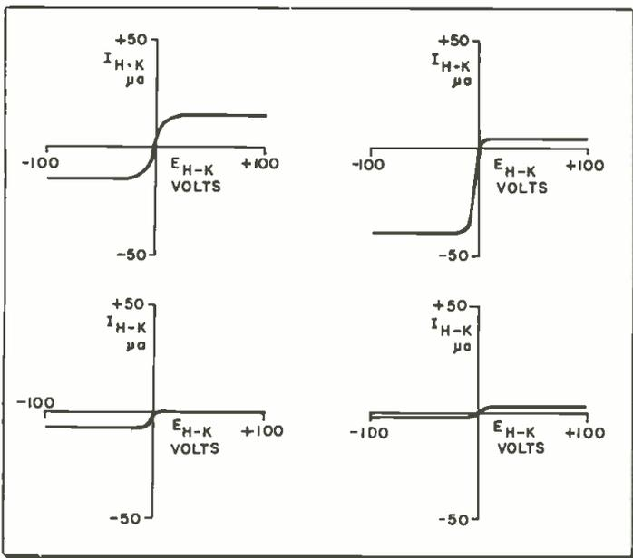
Fig. 3: Leakage with 10-15 v between h & k
