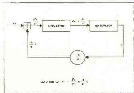
Fig. 5: Simple computer consists of two cascaded integrators in a closed loop system
