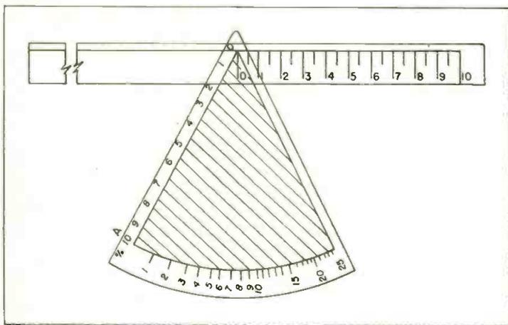
Fig. 3: Applying rule to typical load line
