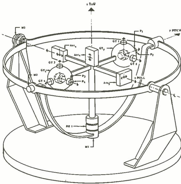
Fig. 1: Inertial platform contains gyros and accelerometers on a gimbal mounting
