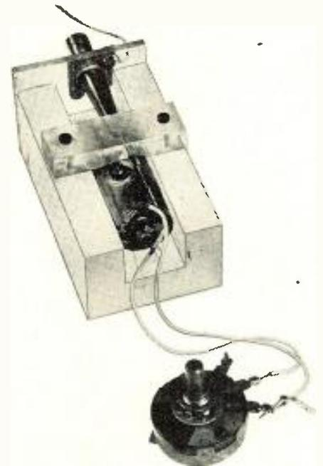
Fig. 1: Converting probe type output of 5794 tube to conventional coaxial output
