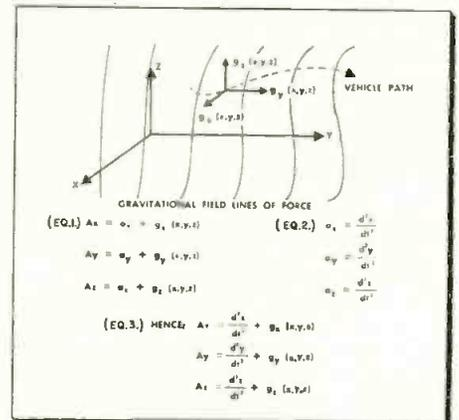
Fig. 3: Equations indicate gravitational and vehicle components of acceleration
