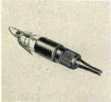
be used. Terminals may be made from commonly used metals and may be sq. or rectangular. Max. terminal dimensions are: .132 x .132 in. with a min. .375 in. spacing between terminals. Connection is 11/32 in. long. Tool weighs 2 lbs. An automatic device stops the bit in the correct starting position. Keller Tool Div., Gardner-Denver Co., Grand Haven, Mich. TELE-TECH & ELECTRONIC INDUSTRIES (Ask for 1-38)
