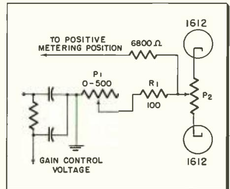
Tap off limiter provides remote metering
