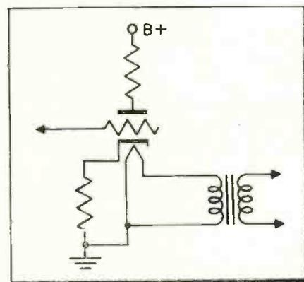
Fig. 6: Class A amp, with grounded heater
