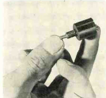
cal rotation, 360°; electrical rotation, 352° ±5°; resistance range, 5 ohms to 25K; standard resistance tolerance, ±10%; standard linearity tolerance, 10%; wattage rating, .8W; ambient temp. range, -55° to +85°C.; 5 oz. wt. per section; starting torque (max.) .75 oz.-in., running torque (max.) .7 oz.-in. General Scientific Div. of San Fernando Electric Mfg. Co., San Fernando, Cal. TELE-TECH & ELECTRONIC INDUSTRIES (Ask for 1-12)
