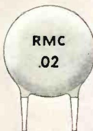
The exclusive wedge design of the leads on these DISCAPS lock them in place on printed circuit assemblies prior to the soldering operation. "Wedg-Loc" DISCAPS are available in capacities between 2 MMF and 20,000 MMF in TC, by-pass and stable capacity types. Suggested hole size is an .062 square.
