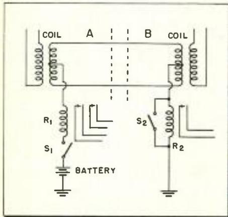
Remote control circuit for audio signalling
