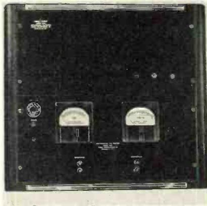
it measures differences in voltage levels as low as 0.01%, regardless of their relation. Also useful to observe drift in amplifiers, meters, and filters. Difference voltage range: -10% to +5% in 0.01% increments. Input level: 0.1 v. to 100 v. Freq. range: 30 cps to 20 kc. Input impedance: 500K ohms. Power supply: 115 v., 60 cycles. Freed Transformer Co., Inc., 1715 Weirfield St., Brooklyn, N. Y. TELE-TECH & ELECTRONIC INDUSTRIES (Ask for 1-2)
