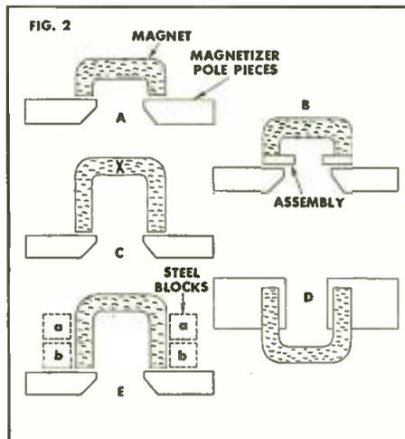
When a "U" shaped magnet is tall or larger than the generally accepted setting of the magnetizer, the field produced at point "X" (see Fig. 2-C) may not be sufficient to saturate the magnet. In this case there are two acceptable methods of magnetization. One is to place the magnet with its side on the pole pieces as shown in Fig. 2-D. This allows the yoke of the magnet to become magnetized. The magnet is then raised to the position in Fig. 2-C and again magnetized.
