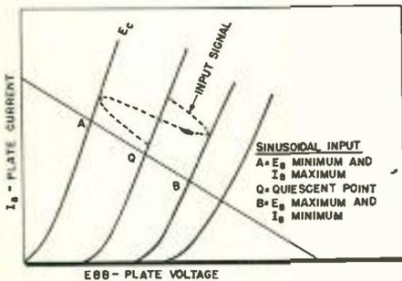
Fig. 4: Typical triode characteristic curve
