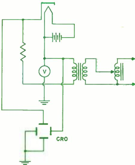
Fig. 1: Method of observing heater-cathode leakage, using an oscilloscope
