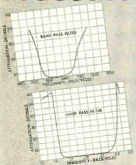
Above curves are representative of filters made for aircraft equipment manufacturers featuring very steep skirt response and high frequency. All filters are hermetically sealed in metal cases.
