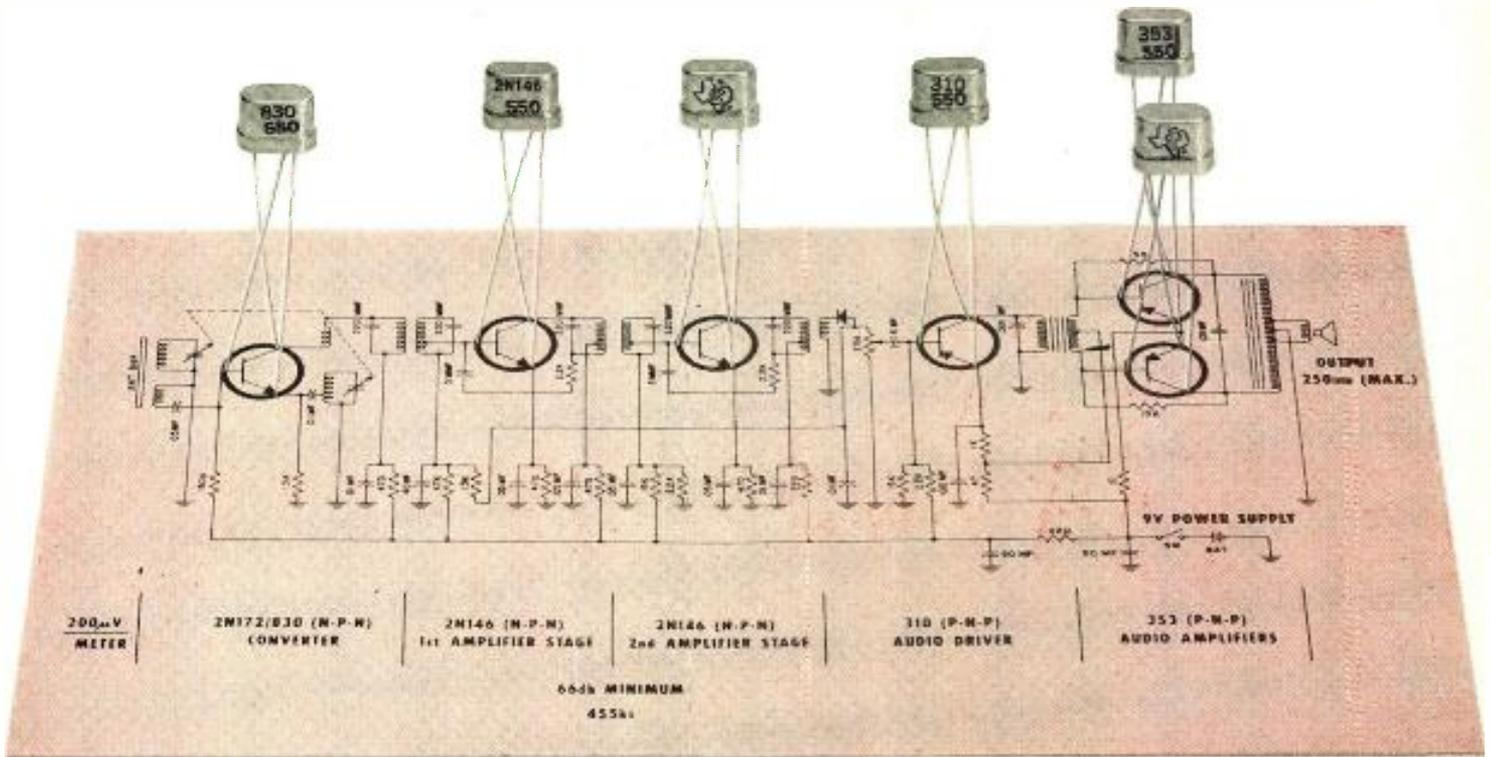
Texas Instruments germanium transistors are used in 85% of the many brands of transistorized radios now being manufactured! Since TI transistors made possible the FIRST transistorized radios 15 months ago, improved mass production methods have rapidly increased performance and decreased prices.
