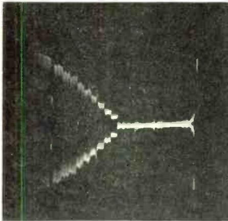
Fig. 6: X-1x response to gray scale
