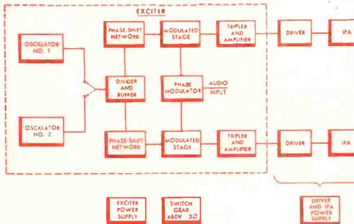
SIMPLIFIED BLOCK DIAGRAM—BTA-50G TRANSMITTER
