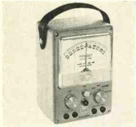
erence freq. in lab. applications or as a secondary freq. standard. Two scales cover the range 395 to 405 cps, and 350 to 450 cps. Measures inputs of 2 to 200 v. Overall accuracy is better than 0.1%; accuracy of calibrator reference freq. is 0.05%. Similar in size and appearance to a small electronic voltmeter. Dimensions: 5¼ in. W., 7⅞ in. H., and 4¼ in. D. VARO Manufacturing Co., Inc., 2201 Walnut St., Garland, Texas. TELE-TECH & ELECTRONIC INDUSTRIES (Ask for 1-6)
