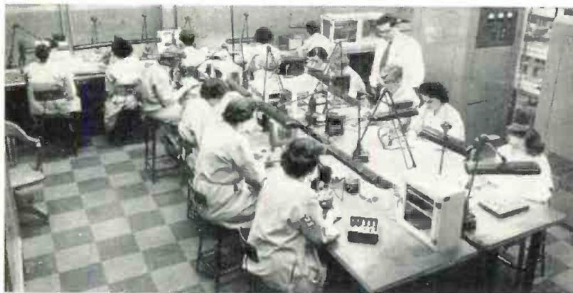
Typical klystron mount assembly line.
