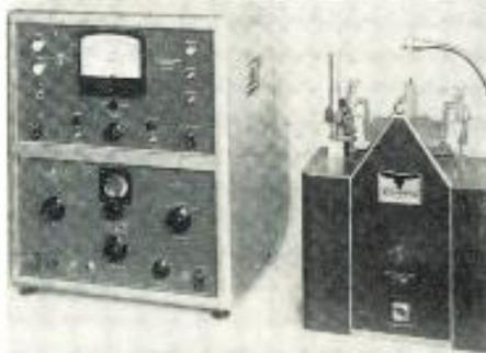
an oscilloscope in the form of a Lissajou pattern or by recording these quantities on a recorder. The table with its associated amplifier is a high performance servo system with a natural frequency in excess of 15 cps and a threshold of less than 5 microradians. Damping ratio is adjustable from approximately 0.1 to 1.0. Max. angular displacement is  $\pm 10^\circ$ . **Micro Gee Products, Inc., Box 1005, 6100 W. Slauson Ave., Culver City, Calif. Tele-Tech & ELECTRONIC INDUSTRIES (Ask for 5-13)**
