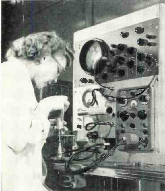
Presetting cavity resonant frequency.
