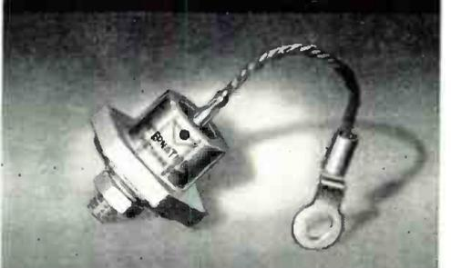
High power-5 amp to 100 amp-silicon fused junction type. Input ratings to 200 PIV. Temp. range: up to  $150^{\circ}\text{C}$  case temperature. Available in individual diodes or all usual power rectifier circuits. Data available on models for forced air and liquid cooling.
