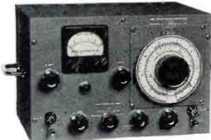
\* Type 405 precision—Accuracy  $\pm 1/4^\circ$ , sensitivity 0.3 v rms, no amplitude adjustment. 8 cps to 100 kc.
