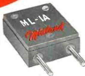
**Type ML-1A.** Range: 2.0 mc–15.0 mc. Supplied per mil Type CR-1A when specified. Holder is phenolic, gasket-sealed.
