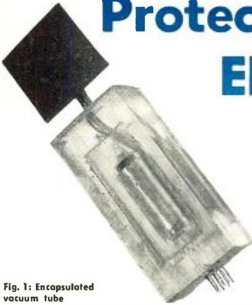
Fig. 1: Encapsulated vacuum tube
