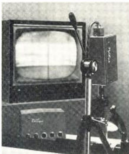
RCA "TV Eye" closed-circuit system is used at Cincinnati Machine Shop of American Can Co. for remote microscopic inspection of thin scraper blades used in Canco lithography coating presses. Camera projects magnified image of blade on a receiver marked with vertical lines to indicate tolerance limits.
