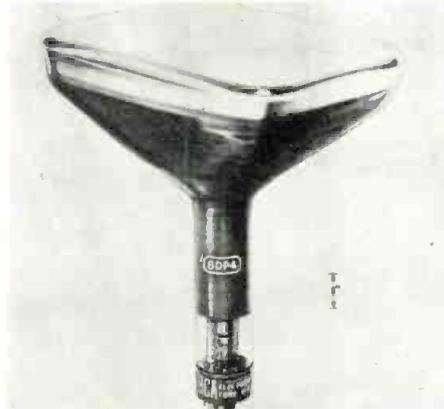
single-field ion-trap magnet; and an external conductive bulb coating which with the internal conductive coating forms a supplementary filter capacitor. **Tube Div., RCA, Harrison, N. J. TELE-TECH & ELECTRONIC INDUSTRIES (Ask for 3-132)**
