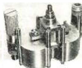
2. Pre-selector-mixer ... S bond ... 50 ohm input impedance ... high Q double-tuned ganged cavities ... detector output ... frequency stable from -55° to +85° C.
