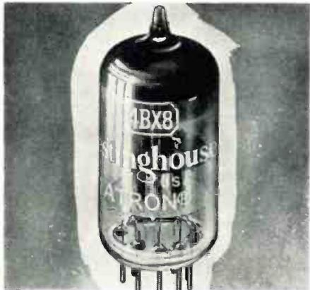
employs a 6.3 v., 400 ma. heater, while the 4BX8 with its 4.5 v., 600 ma. heater, is designed for use in series heater-string receivers. Both double triodes operate with only 60 v. plate-to-cathode voltage. Transconductance is 6800  $\mu$ mhos with a B+ of 125 v. Westinghouse Electronic Tube Div., Dept. T-075, Route 17, Elmira, N. Y. Tele-Tech & ELECTRONIC INDUSTRIES (7-3)
