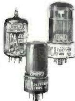
**RCA-5726\*** twin diode intended for applications where dependable performance is paramount under conditions of shock and vibration.
