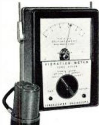
range, uses two ordinary 22½ v. dry batteries to provide power. This all-transistor design alleviates the problem of microphonics (an important consideration in jet-engine testing where high noise levels are encountered. Consolidated Electrodynamics Corp., 300 N. Sierra Madre Villa, Pasadena, Calif. Tele-Tech & ELECTRONIC INDUSTRIES (7-4)
