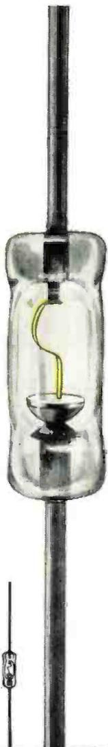
Radio Receptor's "gold standard" for outstanding diode performance is met by our new group of glass computer diodes. The RRco. controlled gold bonding process produces these diodes with fast reverse recovery and high forward conductance as well as unusual reliability and long life. They are thoroughly tested, both in our factory and in actual computer service under strenuous conditions.
