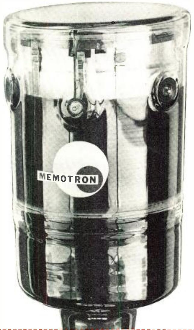
An application of the MEMOTRON is a commercial oscilloscope manufactured by Advanced Electronics Corporation, Los Angeles. MEMOTRON has an over-all length of 18½ inches, and a neck diameter of 2¼ inches. It can replace most conventional 5-inch tubes without revision of space requirements in the equipment.
