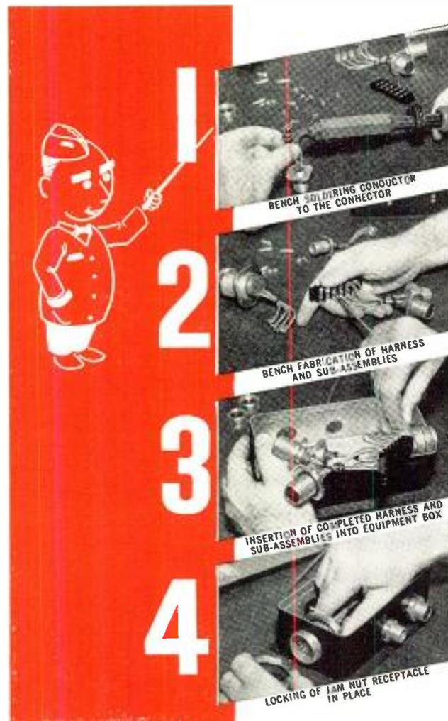
Jam nut receptacles offer such positive savings in assembly time that it will pay you to check into their application on your product. These receptacles permit bench wiring of harness and sub-assemblies prior to final installation with proven savings in assembly labor.
