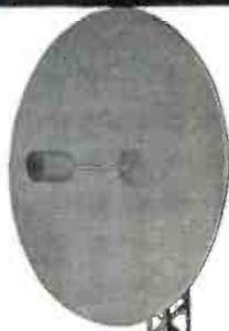
2000 mc antenna with dipole feed.
