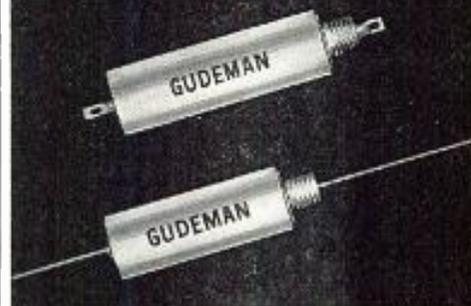
The Gudeman Feed-Thru Capacitor, Types 271 and 272, is a three-terminal component designed to be used for R.F. Interference suppression in a manner similar to a low pass filter. The typical insertion loss characteristics for these Feed-Thru Capacitors when measured in a 50 ohm line are in accordance with MIL-Standard 220.
