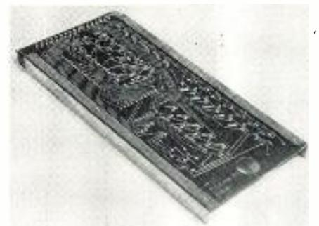
Fig. 2: Typical Formica XXXP-36 P-C board
