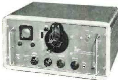
**TYPE 504 FREQUENCY RANGE:** Measures 100 to over 10,000 mc/s. Generates 500 to 900 mc/s and harmonics • **INTERPOLATION ACCURACY:** 0.03% or better • **INPUT SENSITIVITY:** -30 dbm at 500 mc/s and above • **CALIBRATION REFERENCE:** 5 and 50 mc/s quartz crystal standards.
