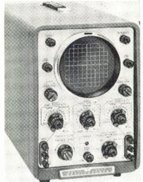
full scale deflection with pass bands from dc to 300 kc, and can accept balanced inputs on the five most sensitive ranges. Hewlett-Packard Co., Palo Alto, Calif. ELECTRONIC INDUSTRIES & Tele-Tech (Ref. No. 10-17).
