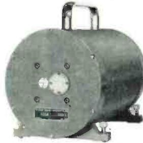
**TYPE 666 FREQUENCY RANGE:** 18 to over 75 kmc/s • **ERROR:** Because the intrinsic error is less than  $\pm 1\%$  plus  $\pm 20 \mu w$  thermal drift, the combined error including instrumentation can be held to within  $\pm 3\%$ . Good approximations can be achieved within one time constant (1.5 to 2 minutes) • **POWER RANGE:** From 30  $\mu w$  to at least 1 watt cw • **SENSITIVITY:** 35-40  $\mu v/mw$  (calibrated for each instrument) • **MAX. VSWR:** less than 1.2.
