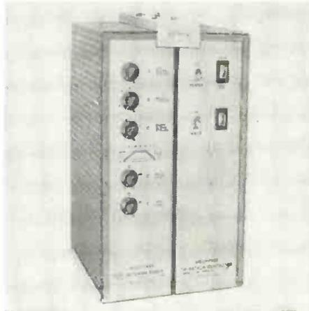
Timer provides for small parts welding on a production basis. Used with a 2 or 5 KVA thyatron contactor and welding transformer, the timer provides current which varies according to a pre-established "Program". **Raytheon Mfg. Co.**, Waltham, Mass. **ELECTRONIC INDUSTRIES & Tele-Tech** (Ref. No. 10-21).
