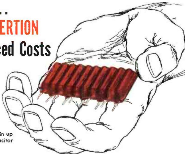
\*"PAC" modules can contain up to 90 Resistor and Capacitor elements per unit.
