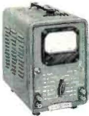
**-hp- 400D**, highest quality, wide range, maximum usefulness. Covers 10 cps to 4 MC, 0.1 mv to 300 v. New amplifier circuit provides 56 db of feedback. (mid-range) for ultimate stability. 10 megohm input impedance prevents disturbing circuits. Sealed or long-life electrolytic condensers; rugged, trouble-free. \$225.00
