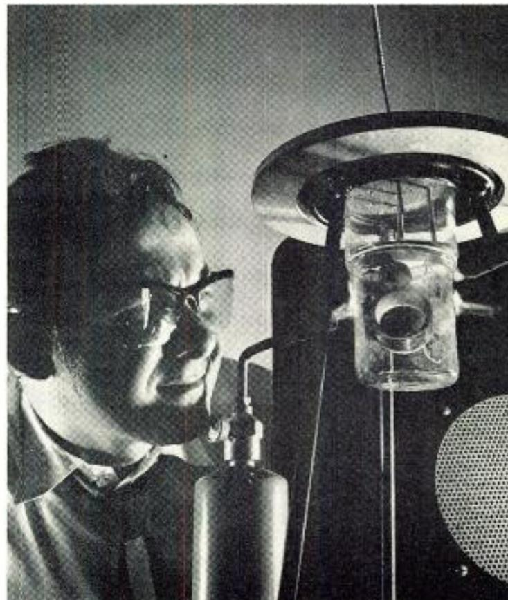
General Electric research engineer, C. B. Mayer applies blow torch to GE’s new high temperature components to illustrate their ability to operate under high ambient conditions. Among units designed for 500°C. operation are heater-less tubes, ceramic diodes
