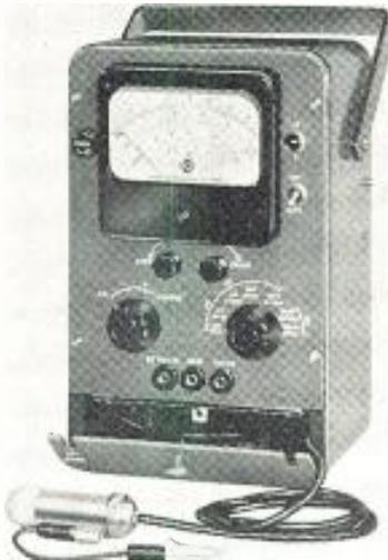
DC voltmeter with 100 megohms input resistance; and an ohmmeter capable of measuring resistance from 0 to 1000 megohms. Accurate measurements to 700 mc, and voltage measurements as high as 32,000 v DC and 1600 v AC. RCA, Camden, N. J. ELECTRONIC INDUSTRIES & Tele-Tech (Ref. No. 10-13).
