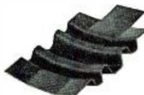
**Corrugated, bent, and punched** after forming, this insulator had to be made of extraordinary stock to withstand unusual stresses. National made use of a double die and PHENOLITE C-534-F to form the corrugated component without cracking or fracturing the piece.
