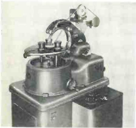
pitch control and special manual feeding attachment for hand winding. Models U-9, U-14, and U-20, to wind tape from 3/8 in. to 1 in. **Universal Manufacturing Co.**, Hillside, N. J. **ELECTRONIC INDUSTRIES & Tele-Tech** (Ref. No. 10-19).
