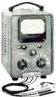
**-hp- 410B**, industry's standard for vhf-uhf voltage measurements. Wide range 20 cps to 700 MC, response flat within 1 db full range. Diode probe places 1.5  $\mu\text{f}$  capacity across circuit under test; this plus 10 megohm input impedance prevents disturbance. Instrument combines highest quality ac voltmeter with dc voltmeter (122 megohm input impedance) and ohmmeter covering 0.2 ohms to 500 megohms. \$245.00
