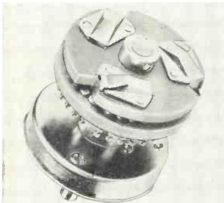
tacts, rotors and slip rings, and gold plated turret solder lug. Rotor and stator material is XXXP phenolic. **The Daven Co.**, Livingston, N. J. **ELECTRONIC INDUSTRIES & Tele-Tech** (Ref. No. 10-20).
