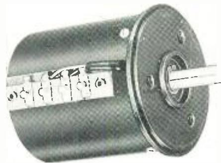
0.015% and electrical noise output only slightly above resolution level. These potentiometers have a max. dia. of 1.825 in. Optional terminal linearity makes field service practical where replacement might be necessary. All taps and terminal connections are welded to a single selected turn of wire. Three turn pots available from 500 to 75,000 ohms; 10 turn pots from 500 to .2 meg. Electromath Corp., Stamford, Conn. (Ref. No. 12-73).
