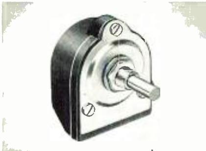
**INDUSTRIAL POTENTIOMETERS**—Type H rated at 5 watts at 40C ambient. Resistance range 50 ohms to 2 megohms. Good for 100,000 cycles with less than 10% resistance change. Derate to zero at 120C. Maximum voltage 750 v, d-c. After 100 hrs. at 40C and 98% humidity, resistance change not more than 5%.
