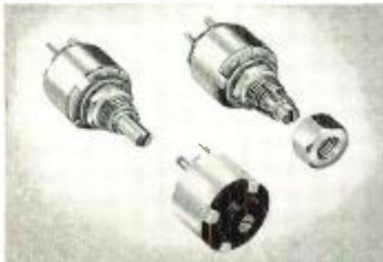
**VARIABLE RESISTORS**—Types G and F molded resistors are 1/2 inch in diameter. Total resistance from 100 ohms to 5 megohms. Ideal for use in printed circuits. The Type G all metal variable control is rated 1/2 watt; Type F control with molded end is rated 1/4 watt. Standard tapers.
