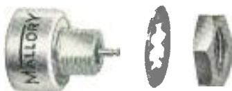
Mallory XT tantalum capacitors are now available in a single hole mounting design which will withstand severe shock and vibration. A flattened neck with  $\frac{1}{2}$ -20 threads fits through a keyed slot in the chassis . . . is held in place by a lock washer and hex nut. Assembly takes only seconds . . . requires no strap or other hardware. This design is supplied in a variety of ratings, with cases up to  $2\frac{1}{4}$ " in height. Write for information.
