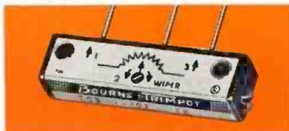
Round pin terminals on this unit may be plugged into holes in your printed circuit boards for dip soldering. Terminals are gold-plated copper, 1/2" long, .028" diameter, and spaced in multiples of 0.1". Mounting is accomplished by 2-56 screws through body eyelets, or by pins only.
