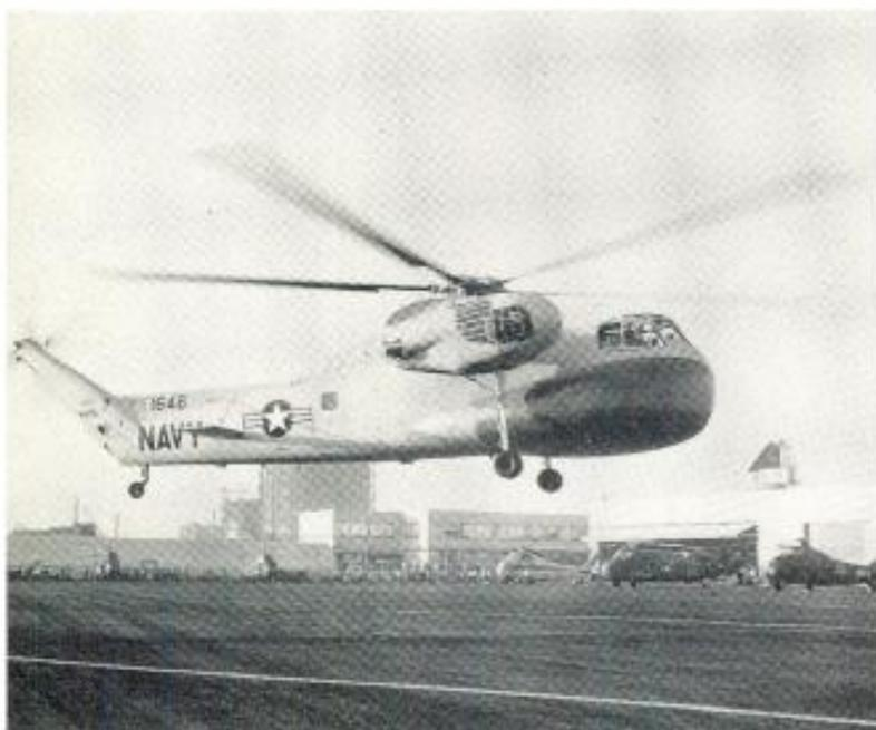
Bulging plastic radome on this Navy Sikorsky helicopter houses the antenna for an extremely high-powered GE search radar that detects low-flying planes more than twice as far as shipboard equipment.
