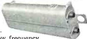
**Tuneable UHF Pre-Selector**—relatively low frequency coaxial resonator with very low insertion loss, extreme selectivity and very high signal-to-noise ratio. Especially adapted to use in aircraft or in crowded communication bands.
