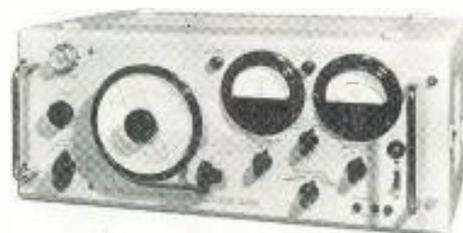
usual capability of simultaneously indicating the incidental AM in an FM signal being measured and, conversely, the incidental FM in an AM signal. The range of indication for full scale frequency deviation is 0 to 10/30/60/150 kc. However, provisions are made for connecting external indicators to be used for measuring FM deviations as low as 40 cps. Federal Telephone and Radio Co., Clifton, N. J. (Ref. No. 12-36).
