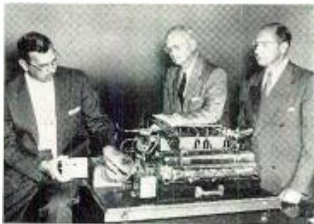
Bendix officials show details of "Electrojector" all-electronic fuel injection system
