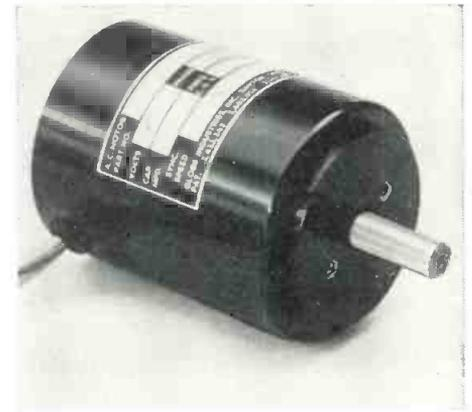
has been considered in the design. They can be wound as follows: 3-phase, 2 or 4 pole; 2-phase, 2 or 6 pole. Both 3-phase and 2-phase units can be operated single-phase with a suitable phasing capacitor. The induction rotor will provide a unit with more output than a unit with a hysteresis rotor, but the hysteresis unit will operate at synchronous speeds. Globe Industries, Inc., Dayton. (Ref. No. 12-50).
