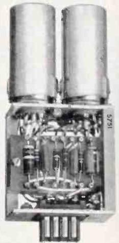
**K2-PJ** An accurate, low drift, low frequency chopper amplifier, the K2-PJ is ideally suited to stabilizing (servoing out the drift error in) an unstabilized dc amplifier such as the K2-WJ, K2-YJ, etc. When used as a preamplifier for the K2-WJ, the pair typically exhibits a long term drift of less than 100 microvolts, zero grid current, and a dc gain of 10 million. Write for details. Price (1 thru 99) ..... \$85
