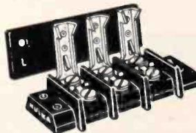
Here's a practical device to simplify your wiring work and assure correct connections. Multi-conductor cable is attached at either end of strip with a clamp. Each wire is soldered to terminal lug. Then, sliding and tightening the spade-type lugs under the binder screws of terminal block, all connections are completed. Supplied with flat lugs or with 90° upright lugs.
