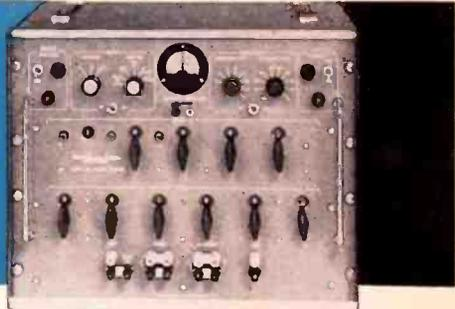
**—measures both in-phase and quadrature voltage ratios — with high accuracy**
