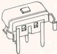
These are four-contact right angle sockets for horizontal transistor position. Nickel plated phosphor bronze clip retains transistor by snapping over beaded base. Clip is removable and reversible to facilitate mounting components either right or left handed. Bodies are low-loss phenolic and contacts are of silver plated beryllium copper. These sockets are also supplied with either 3, 4, or 5 contacts for in-line tubes or transistors. Available from Cinch Mfg. Co.
