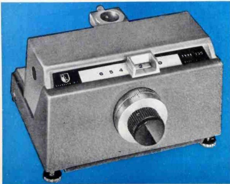
Completely covers the frequency range from 4.0 to 40.0 KMC/S with only one probe carriage.
