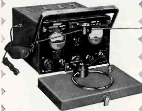
This versatile instrument is a highly sensitive interference locator—with the widest frequency range of any standard available unit! Model 500 tunes across the entire standard and FM broadcast, shortwave, and UHF-TV spectrums from 550 kc. to 220 mc. in 6 bands.
