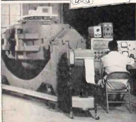
Test being conducted on the 12,500 force pound Vibration Machine. Accelerometer outputs are being automatically recorded for inclusion in the test report.
