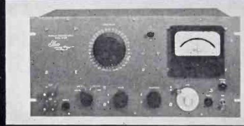
Test Equipment for Precision Computing Resolvers now in production — Instruments to measure Function Error, Inter-Axis Error, Null Spacing Error, Fundamental Null, Total Null, Electrical Zero, Winding Phasing, Phase Shift, and Transformation Ratio.
