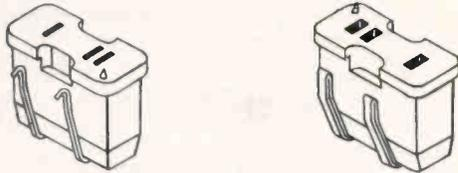
This is a military type socket designed to snap into a polarized chassis cut-out in boards having circuitry on one or two sides. Body is of low-loss phenolic. Contacts are brass, silver plated followed by a gold flash. Available from Cinch Mfg. Co.
