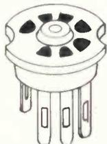
7 and 9 pin push-in miniature tube socket bodies are molded of general purpose or low-loss phenolic. They are pushed into a specially formed chassis hole and are retained by the pressure of the chassis. Considerable space and assembly
