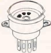
7 and 9 pin split-saddle miniature tube sockets essentially made as described previously, except that a shield base has been incorporated in the saddle to provide adequate means to accommodate a tube shield.
