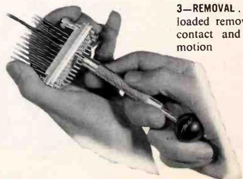
3—REMOVAL . . . Special spring-loaded removal tool removes contact and wire with one motion
