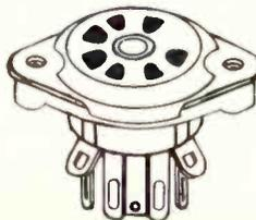
Bottom mounted, screw fastened tube sockets have the mounting nuts included as integral parts of the nickel-plated brass saddles. These sockets are available with bodies of low-loss phenolic and silver plated phosphor bronze or beryllium copper contacts with or without ground lugs and center shield from H. H. Eby Inc. and Methode Mfg. Co.
