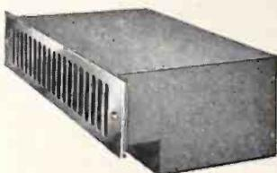
Provide higher performance with minimum panel height. Filter and blower are recessed into the unused portion of the open base commercial type rack. Fit 3 1/2", 5 1/4", 7", 8 3/4" and 10 1/2" panel heights and deliver 150 cfm to 1200 cfm. Highly reliable, rubber mounted, 115 volts, 60 cycle motors. Mil. Spec. and DC motors available. Permanent filters.
