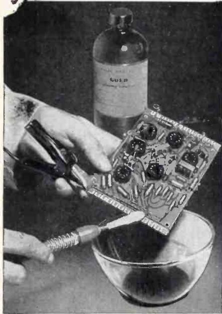
Plating circuit contacts without dismantling electronic components.
