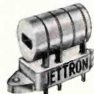
**CAT. 8715**—Ultra-High Temperature Socket for G.E. 7296 Triode can be soldered to printboard or mounted above or below a chassis. High Alumina Insulating material; contacts gold plated Inconel-X. For continuous operation at 1000° F (538° C).
