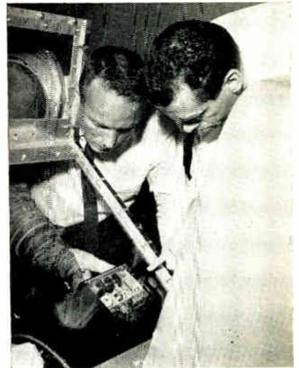
Astronaut M. Scott Carpenter (left) tests communication controls for Project Mercury. Controls, supplied by Collins Radio Co., Dallas, Tex., are in a pressure suit simulator (arm and glove section only).
