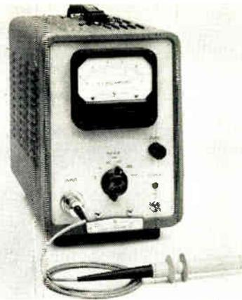
*The slow, inconvenient, and often inaccurate methods of measuring dc using voltage-resistance measurements spurred the development of a clip-on type of milliammeter. The instrument used the fluxgate principle. The principle is now being extended to other applications including the measurement of ac fields, varying dc, and in a Magnetic Ink Tester.*
