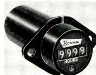
1440 indicator presents 4 white 0.109 in. numerals on a dull black counter drum. The counter provides readings from 0000 to 9999 hrs. with return to 0000. Bowmar Instrument Corp. Booth 765.
