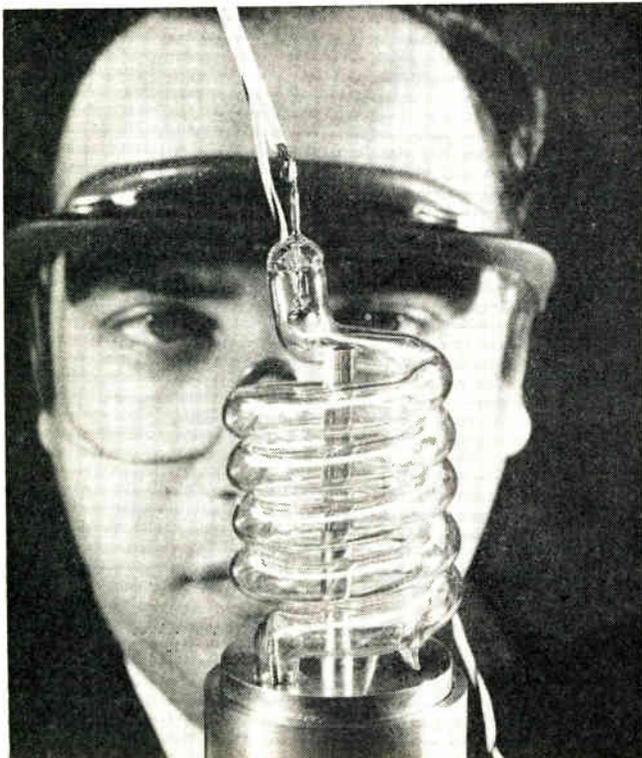
Fig. 1: The laser's main parts are a light source surrounding a rod of synthetic ruby crystal through which excited atoms generate the intense beam.
