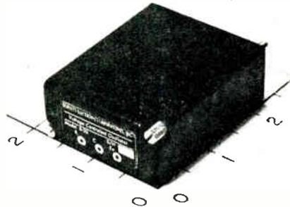
minum configuration that features a captive screw hold down and a removal device. Package measuring 2.25 x 1.875 x 0.875 in. is smallest of 3 packaging modules in the series of telemetering hardware. Adjustment controls for centering, deviation sensitivity, and output provided at top of unit. Available in standard IRC channels with inputs of either 0 to 5 v., or  $-2\frac{1}{2}$  v. to  $+2\frac{1}{2}$  v. Dorsett Electronics Laboratories, Inc., 119 W. Boyd, Norman, Okla.
