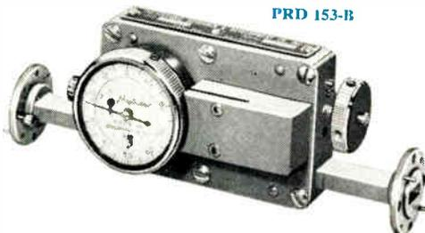
ing it into the waveguide through a slot, as in the PRD 153-B, known as a "flap" type (Freq. range 18.0 to 26.5 KMC; Attenuation to 35 db; Max. VSWR 1.10; Max. insertion loss 0.5 db; Calibration accuracy  $\pm 0.2$ ); or (2) by moving the lossy element from the side wall toward the center of the waveguide
