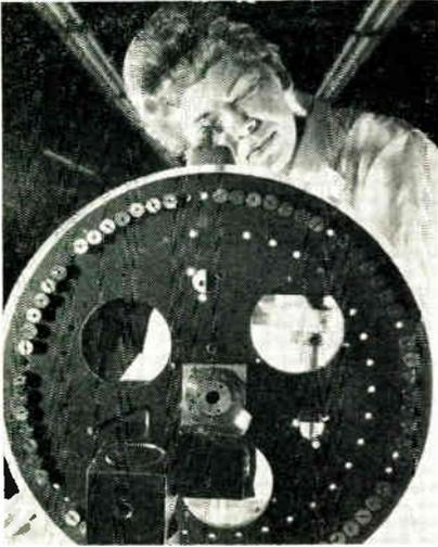
Joan Shave "eyes" some of the 60 ultra-thin wires on "spinning wheel" used in making grids for RCA new nuvistor-RCA-6CW4.
