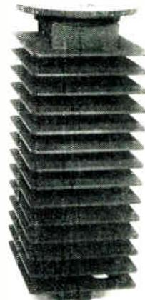
erating from 2600 to 3950 MC to dissipate energy when the radar is not transmitting. Use of inert, high-temperature silicon carbide as the absorptive element minimizes water absorption, increases stability, and lengthens trouble-free life. Liquid-cooled versions also available. Smaller and lighter models of dummy loads for lower power were previously introduced. Airtron-Pacific, 5873 Rodeo Rd., Los Angeles 16, Calif.
