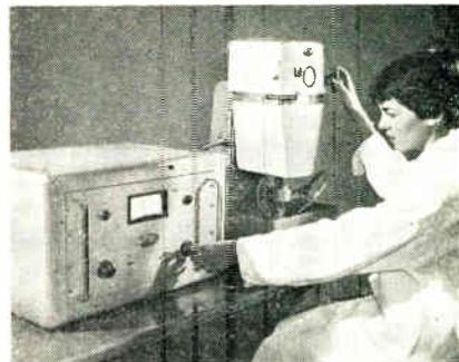
cluding cleaning and soldering. It features an air-cooled, 300-w magnetostrictive transducer and eliminates bothersome plumbing arrangements. The magnetostrictive transducer provides continuous operation, eliminating down-time for cooling often necessary with ceramic transducers. Transducer is an insert-type. Either coil or transducer can be removed without disturbing the other. Commercial Apparatus & Systems Div., Raytheon Co., 1415 Providence Tpke., Norwood, Mass.
