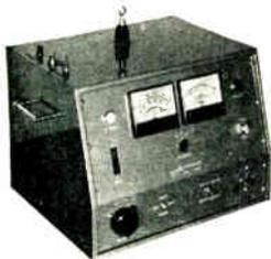
Model 424 HYPOT provides 0-5000 v d-c for testing cables, condensers, coils, transformers and assemblies. Measures leakage 0.1 to 100 microamperes over four scale ranges. Rapid charging of capacitors with 5 ma. output. Self-contained power supply. Complete \$497.00.
