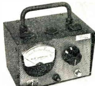
single control, it provides a current range from 60 to 125 ma dc for any tube with an operating voltage from 30 to 100 v. and lower currents for tubes with higher operating voltages. Max. ripple voltage under load is 4 vac. Characteristics: Input, 115 vac at 115 vac at ¼ aac; Output, Unloaded Supply Voltage, 350 vdc, nom; Loaded Supply Voltage, 230-275 vdc; Current 125 ma dc, max.; Size 4½ x 6¾ x 5¾ in. The Bendix Corp., Red Bank Div., Eatontown, N. J.
