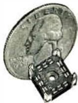
**CO-7140** — Printboard Application Socket for R.C.A. Micromodule. Measures only .400 maximum square by .094 high. Insulation resistance greater than 50,000 megohms. Employs silver plated beryllium copper contacts and DIALL FS-5 insulating material.
