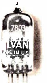
**SYLVANIA-7803**... a miniature double-triode, it offers high  $g_m$  of 12,500  $\mu$ mhos per unit and low capacitance. 7803 uses the Sylvania-developed, rugged strap frame grid—enabling use of fine grid wire, high T. P. I.
