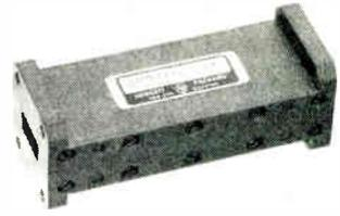
N362A in order): Pass band, 10 to 15.5 KMC-15 to 21 KMC; Standing wave ratio (pass band), 1.5:1-1.5:1; Insertion loss (pass band), less than 1 db-less than 1 db; Stop band, 19 to 47 KMC-28 to 63 KMC; Rejection (stop band), at least 40 db-at least 40 db; Waveguide size WR 75-WR 51; Flange, flat cover-flat cover; Length, 4 15/32 in.-3 1/32 in.; Weight, net 9 oz.-net 5 oz. Hewlett-Packard Co., 1501 Page Mill Rd., Palo Alto, Calif.
