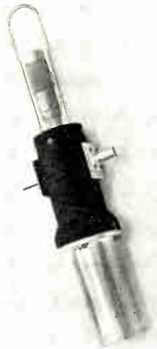
The micrometer is readable to 0.0001 in. and a calibration chart is furnished. Radar Design Corporation, Microwave Components, Pickard Drive, Syracuse 11, New York.
