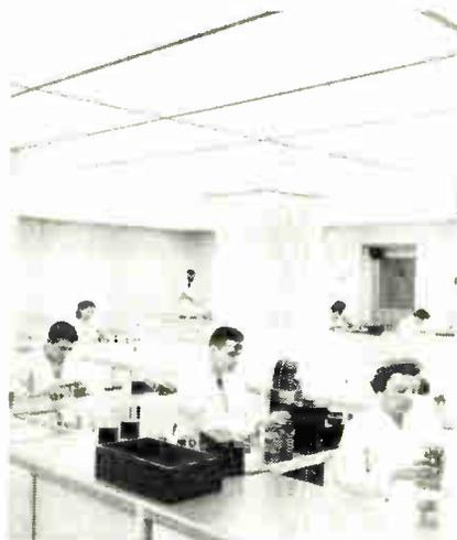
Meter assembly "White Room" has luminous ceiling which features a lighting level of 300 footcandles at Hickok Electric Instrument Co. in Cleveland, Ohio. This has boosted quality levels 100%, output 50% and cut production costs 20%.
