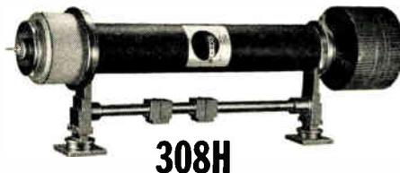
**308H** Control grid  $\mu = 55$ . 15 kw peak power output (150 watt average), 8.6—9.9 kmc frequency range, 53 db saturation gain, 1% maximum duty cycle, beam voltage = 24 kv, 14 lbs. total weight of tube and magnet.
