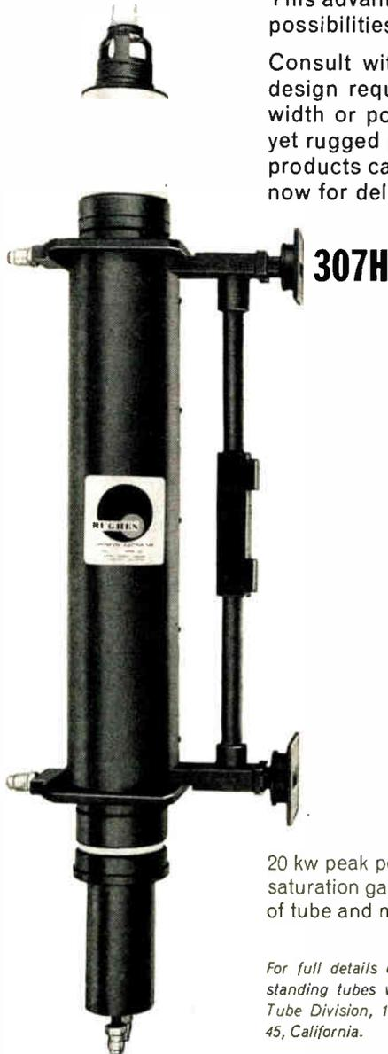
**307H** LEFT: 100 kw peak power output (500 watt average), 8.5—9.5 kmc frequency range, 54 db saturation gain, 1% maximum duty cycle, beam voltage = 38 kv, 21 lbs. total weight of tube and magnet.
