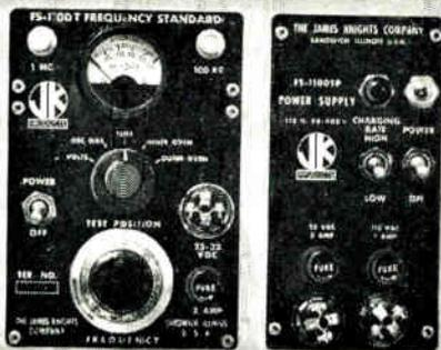
A JK-SULZER FS1100T currently serves as the basic quartz crystal Frequency Standard employed by WWVL (Bureau of Standards, Boulder, Colorado) to provide a 20kc reference signal having a stability of  $1 \times 10^{-10}$ /Day.
