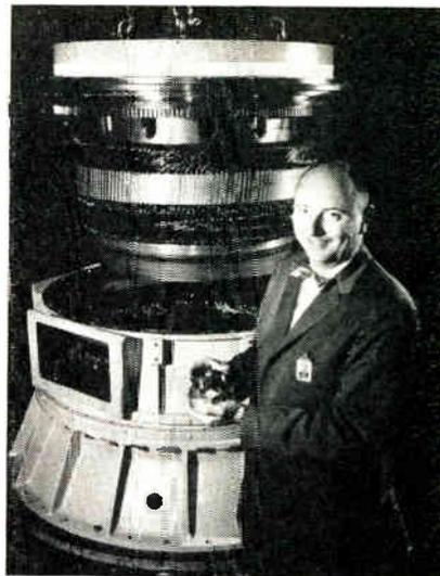
Small drive motor used in Polaris Missile Inertial Guidance System is contrasted with new Fire Control Director, MK 73. Used with the AN/SPG-51 Radar to track and illuminate enemy aircraft traveling at supersonic speeds, the gearless power drive is displayed by co-inventor, E. B. Canfield, Advanced Control Engineer, G. E. Ordnance Dept., Pittsfield, Mass.
