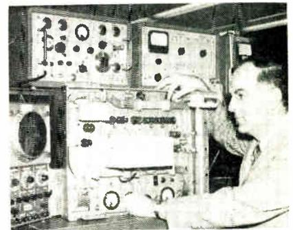
Production model of GE's new parametric up-converter is checked out by Dr. Harry Pappiatt. An incoming signal of 400 MC is converted up to 10,000 MC, and then down to an intermediate frequency, with low noise gain.
