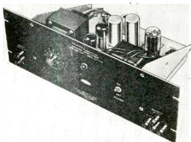
0.5 v. input. Features low distortion, wide frequency range (12 cps to 60 kc), and low internal noise and hum. H. H. Scott, Inc., Instrument Div., Dept. P, 111 Powdermill Rd., Maynard, Mass.
