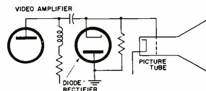
Fig. 3: Video amplifier AC coupled to the picture tube. This circuit represents present day practice—no DC restoration.
