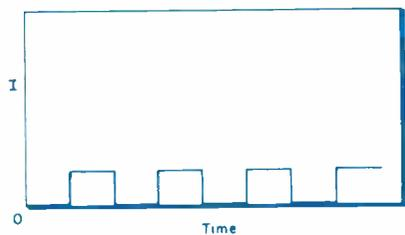
Fig. 17 (left): Pattern of square wave pulses used in measuring resistance. (top) zero biased low current pulses for initial measurement of forward voltage drop; (bottom) pulse pattern for diode self heating.
