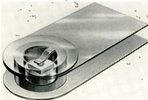
No larger than the head of a match, tunnel diode in RCA developed low-inductance case with integral ribbon measures less than  $\frac{1}{4}$  in. in overall length and has a height of about  $\frac{1}{16}$  in. Cylindrical ceramic case and ribbon lead-and-tab construction provide an inductance of only 0.4 millimicrohenry. The tiny component is now being offered on a sampling basis by the RCA Semiconductor and Materials Division for engineering evaluation.
