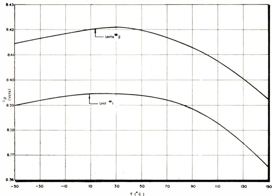
is also a strong function of temperature.<sup>19</sup> It is also the parameter most frequently used to measure thermal resistance. Unfortunately, for silicon at room temperature and higher, the temperature dependence of the reverse current is complicated by space charge generated currents.
