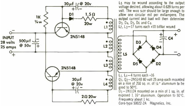
$L_s$  may be wound according to the output voltage desired, allowing about 0.639 turns per volt. The wire size should be large enough to allow one circular mil per millampere. The output current and load will then determine  $D_3, D_4, D_5, D_6$  and  $C_4$ .
