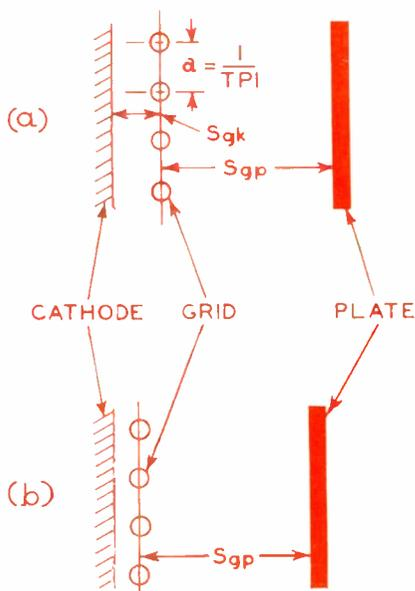
Fig. 1: When the plate and grid No. 1 of the triode with given dimensions (a) are moved closer to the cathode (b), contrary to expectations the  $g_m/I_b$  ratio changes.
