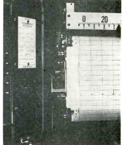
the chart. It can be field mounted directly on change gear hubs. Two standard models of the multi-speed chart drive, having overall ratios to 16:1 and 32:1 are available for every different chart drive gear train used in the standard Dynamaster recorder. Inasco Co., Div. of Barry Controls Inc., Groton, Mass.
