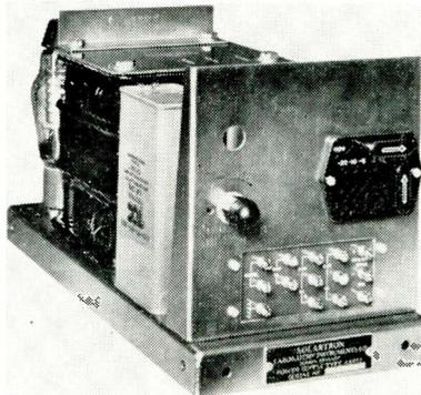
955, 956, 957) output voltages covering from 100 to 400 v. Output voltage can be varied over  $\pm 50$  v. from nominal. Solartron Electronic Group Ltd., 45 Thames St., Kingston, Surrey, England.
