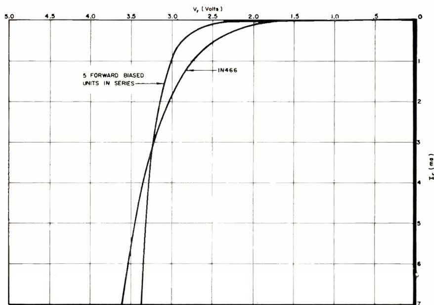
Fig. 13 (above): Comparison of the breakdown characteristic of a low voltage reverse biased diode with that for a series string of five forward biased units.
