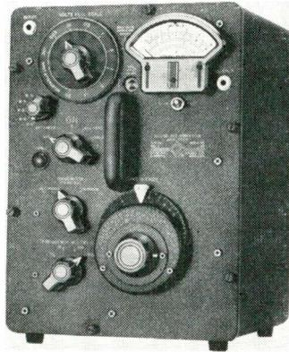
quency) and all-pass response. It is a tunable voltmeter whose bandwidth is a constant percentage of the center frequency. Narrow-band max. response is flat  $\pm 2$  db over the tuning range;  $\frac{1}{2}$ -octave max. response is flat  $\pm 4$  db over range; and the all-pass response is flat from 2.5 to 25,000 CPS  $\pm 2$  db. General Radio Co., West Concord, Mass.
