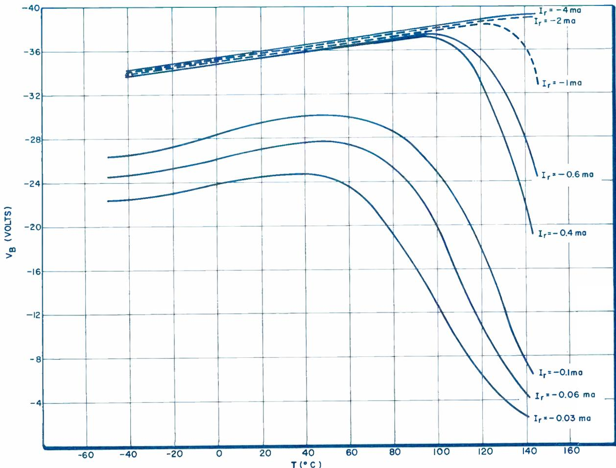
Fig. 16 (right): Change in nominal output voltage versus time for some 1N430 diodes under various operating conditions.
