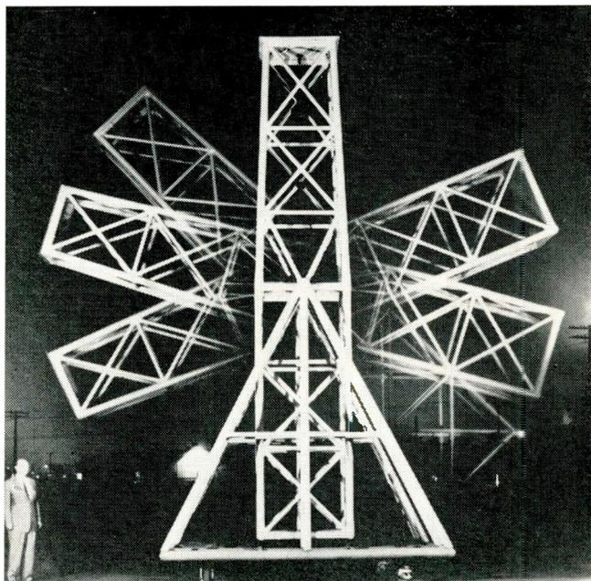
position not only mock-ups, models and missiles up to 500 lbs. in weight, but also two-axis azimuth/elevation positioners which themselves may weight some quarter of a ton.
