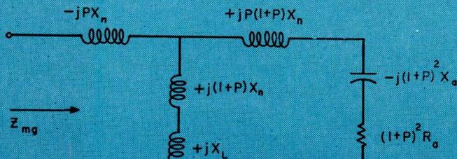
Fig. 2: Folded-unipole equivalent circuit (Poté)
