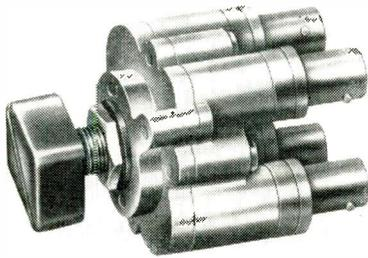
500 MC and 1.2 up to 1000 MC. It is a four terminal, two position transfer switch, coaxially mounted in a die cast metal frame. Insertion loss is less than 1/10 db to 1000 MC. Isolation between the open and closed circuit is 58 db at 100 MC and 40 db at 1000 MC. Jerrold Electronics Corporation, 15th and Lehigh Avenue, Philadelphia 32, Pa.
