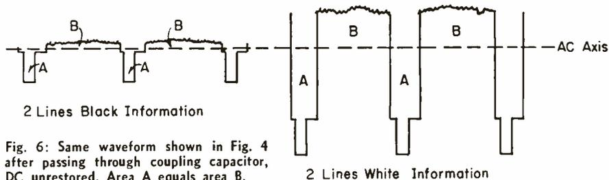
Fig. 6: Same waveform shown in Fig. 4 after passing through coupling capacitor, DC unrestored. Area A equals area B.
