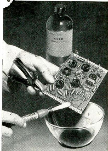
Plating circuit contacts without dismantling electronic components.
