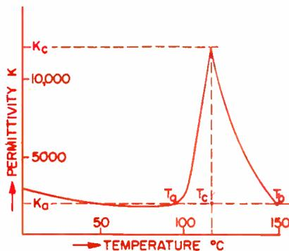
Fig. 1 Permittivity of a dielectric, barium titanate, around Curie temperature.
