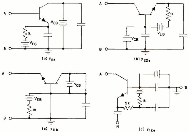
Fig. 3: Circuits for measuring  $y_{11e}$ ,  $y_{22e}$ ,  $y_{11b}$  and  $y_{12e}$
