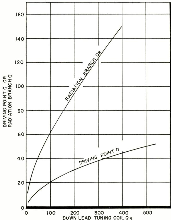
Fig. 8: Plots of radiation branch  $Q$  and driving point  $Q$  are shown as a function of the tuning coil  $Q$
