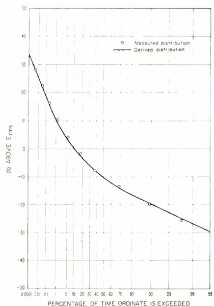
Fig. 2: Graph illustrating the effectiveness of a graphical method for obtaining the amplitude-probability distribution of atmospheric noise.
