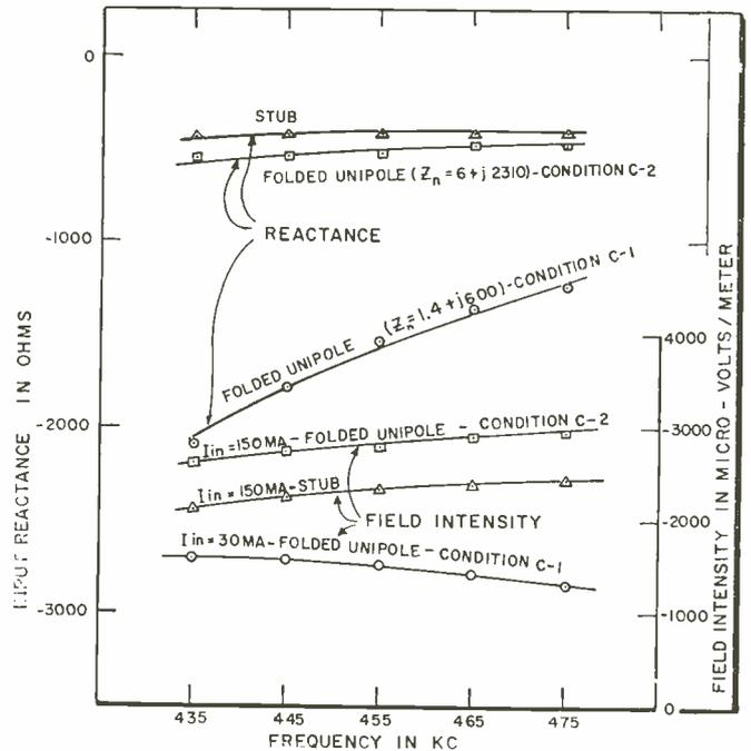
Fig. 9 (right): Input reactance and field intensity vs. frequency
