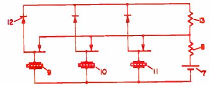
Fig. 4: Another method of eliminating power is the multiple capacitor converter.
