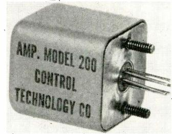
may be adjusted by external resistor. Gain stability is 2 db over temp. range. Internal limiting prevents overdrive or phase shift for high input signals. Operates on 28 vdc. Low output impedance gives good servo response. Will operate under MIL E5272A environmentals. Control Technology Co., 1186 Broadway, New York 1, N. Y.
