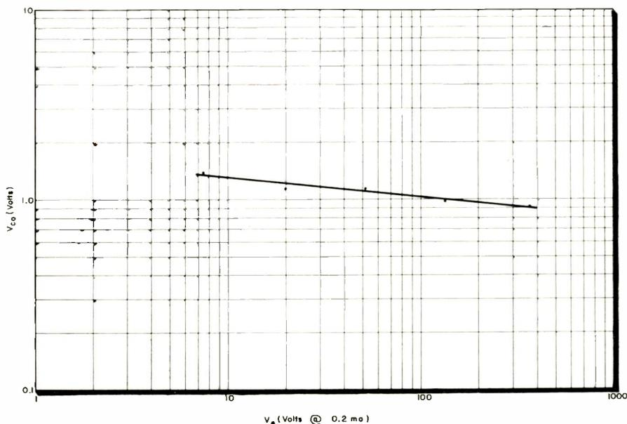
Since the forward impedance of the diodes would be additive, one might expect the series string to be a poorer regulator than a single reverse biased diode of the same voltage. However, the reverse characteristic of the diodes (Hoffman IN465 through IN470) becomes softer as one goes down in zener voltage.
