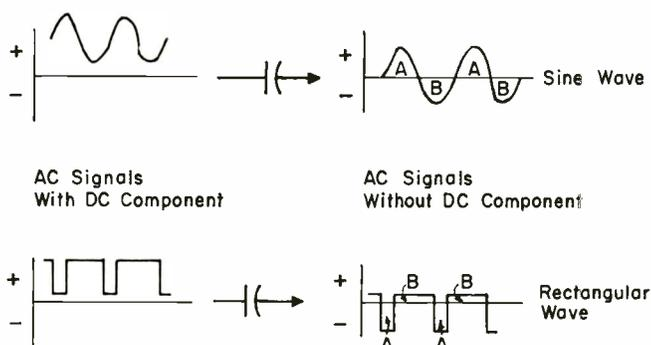
Fig. 5: The effect on waveforms when the DC component is removed by interstage coupling capacitors. Area A equals area B.
