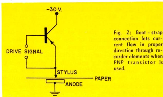
Fig. 2: Boot-strap connection lets current flow in proper direction through recorder elements when PNP transistor is used.
