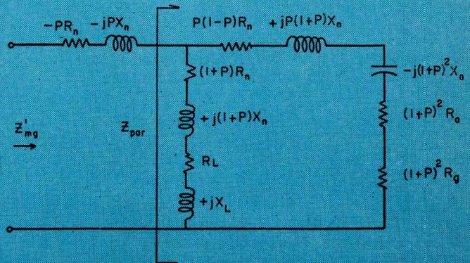
Fig. 3: Equivalent circuit for folded-unipole (losses included)
