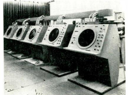
Airborne Tactical Data System consoles are set-up for preshipping tests.
