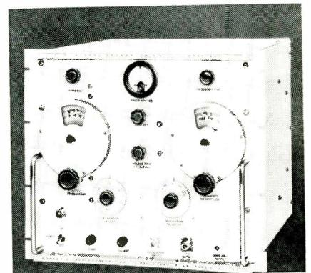
peak is produced by external modulation signals having an amplitude of 1.0 v. peak to peak. R-f output is continuously variable from 0 dbm to -110. Sierra Electronic Corp., 3885 Bohannon Drive, Menlo Park, Calif.
