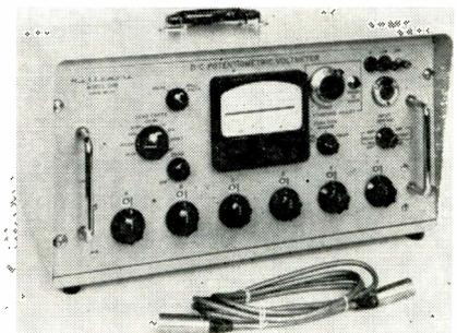
$\mu v$ ). The resistor network is controlled by 6 decade switches covering voltage ranges from  $\pm 10 \mu v$  to  $\pm 10$  volts. Hallamore Electronics Company, 714 N. Brookhurst Street, Anaheim, Calif.
