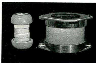
A size reduction is dramatically illustrated when comparing an HPD rated at 25 amps with a conventional CM85 mica capacitor.
