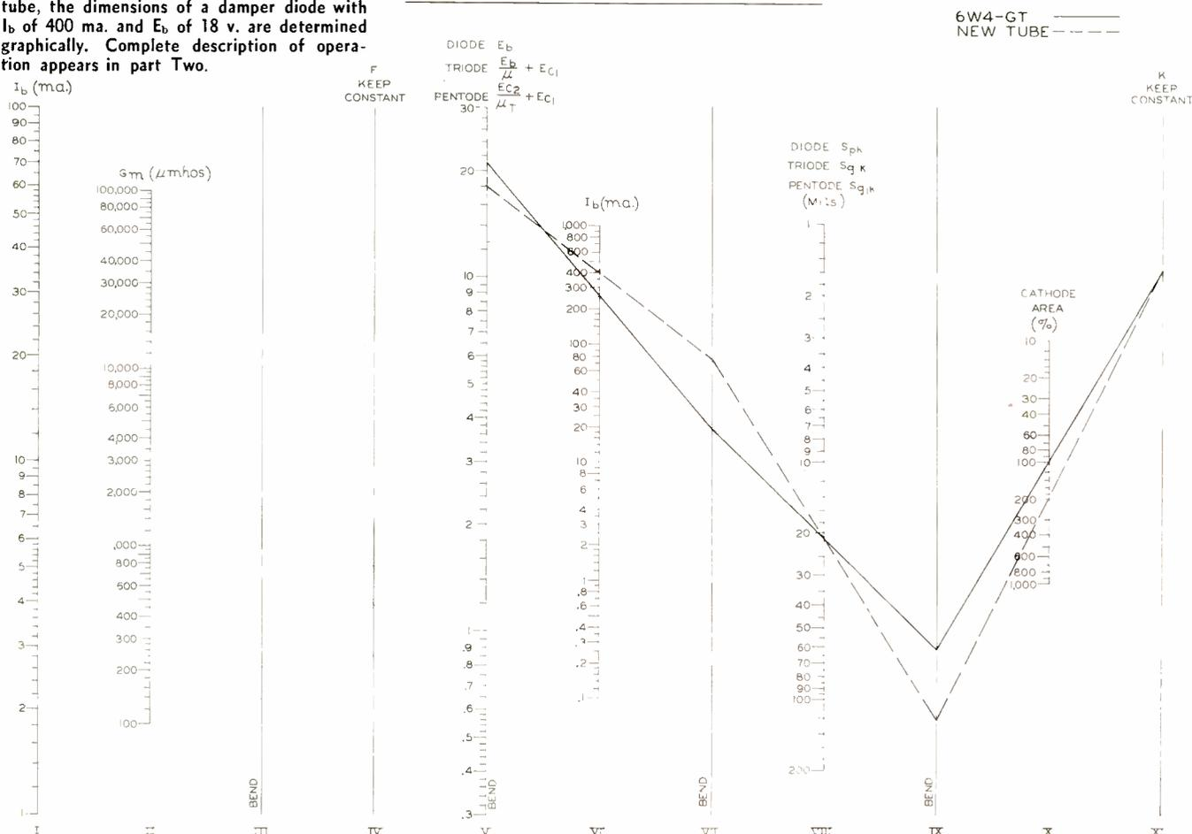
$$I_b = K' \frac{A_k}{S_{g1k}^2} \left( \frac{E_{c2}}{\mu_T} + E_{c1} \right)^{3/2} \quad (6)$$
