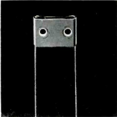
to 8.0 $\mu$ , peak response 6.0 to 6.5 $\mu$ . Sensitivity measured with 2 $\mu$ W radiation on sensitive area and 50ma dc applied to cell. With this, signal to noise ratio at 6 $\mu$  is more than 72 and noise equivalent power at 6 $\mu$  is 4 x 10<sup>-9</sup>w. Cell is low impedance in the order of 75 ohms. The max. dc value is 100ma and the max. case temp. 70°C. International Electronics Corp., 81 Spring St., New York 12, N. Y.
