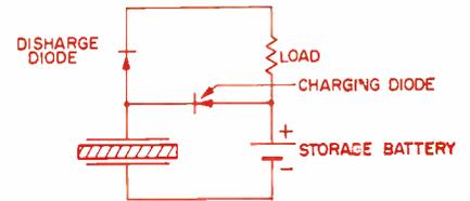
Fig. 3: Ferroelectric energy converter circuit requiring no primary battery power
