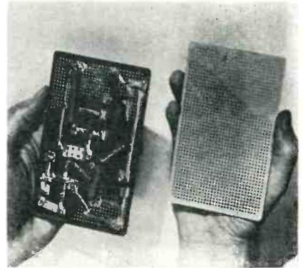
persulfate are used for removing excess copper. Boards are 1/16 in. thick and available in 3 sizes: 3 x 5, 6 x 8 and 9 x 12 in. Components can be soldered to the board more than 50 times without circuit run failure. Fotoceram, a glass-ceramic with high strength, high temp. resistance, and zero water absorption, is non-flammable and dimensionally stable. Electronic Components Dept., Corning Glass Works, Bradford, Pa.
