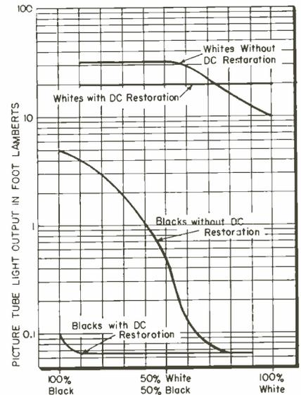
Fig. 8: Actual light output from the face of a picture tube under both restored and unrestored conditions. White and black input signals held constant. Percentage of white and black areas in picture indicated along the abscissa.
