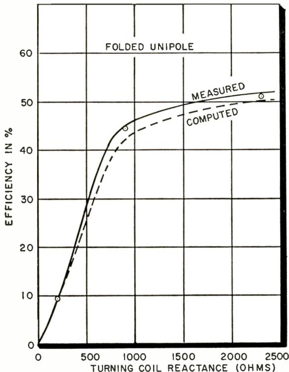
Fig. 7: Radiation efficiency (ant. only) vs. tuning coil reactance
