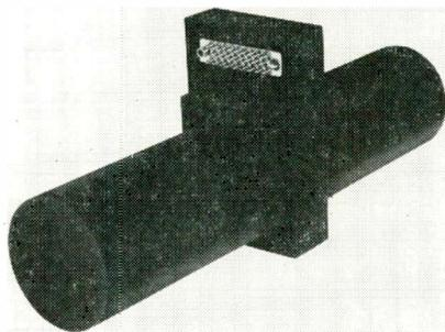
package. Each individual potentiometer can be supplied with its own independent function so that simultaneous control, feedback and telemetry signal can be provided. Specs are: linearity,  $\pm 0.1\%$ ; resistances, 1000 to 100,000 ohms; resolution, as low as 0.03%; power rating, 1.5 w per element; temp. range  $-65$  to  $+200^\circ\text{F}$ . Bourns, Inc., P.O. Box 2112, Riverside, Calif.
