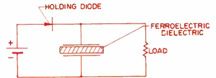
Fig. 2: Basic circuit of the ferroelectric energy converter aids understanding.
