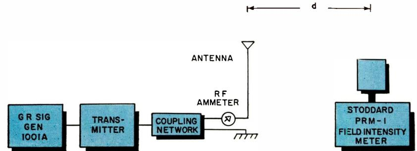
Fig. 5: Radiated field intensity measurements setup
