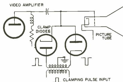
Fig. 10: A keyed clamp DC restorer circuit.
