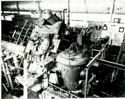
A 5000 lb. high vacuum induction furnace, the only unit of its kind and the world's largest, has been installed by the Metals Div., Kelsey-Hayes, Co., Hartford, N. Y. The entire melting chamber of the furnace, designed and built by ASEA, Vasteras, Sweden, tilts to pour. Vacuum is as low as one micron. Ingot size can range from 200 to 5000 lb.
