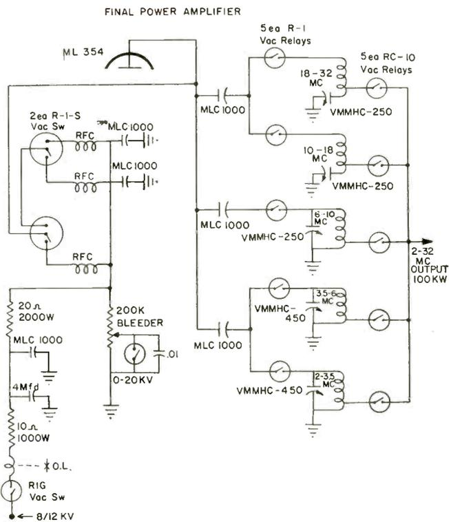
Normal operating conditions for the final amplifier tube are as follows: plateloading is 1666 ohms with a capacitive reactance. The
