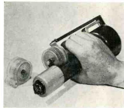
miniatures. Contacts are in disposable plastic cartridges. Crimping action is that of the Deutsch manual crimping tool, providing 2 series of 4 indents. Locking action is built in. In case of air failure or intermittent pressure, the tool will jam. The Deutsch Co., Electronic Components Div., Municipal Airport, Banning, Calif.
