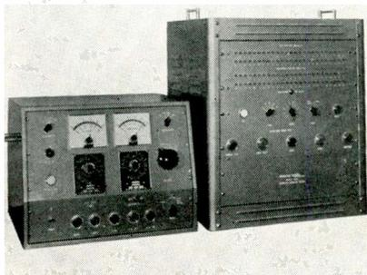
Model 8514 HYPOT<sup>®</sup> high voltage test set used with the tester. The rate of rise for this test potential and the length of time it is applied to each unit (up to 15 min.) is adjustable. All units, when not under test, are short circuited. Leakage current metering circuits have ranges of 0-10/25/100/250 ma. Automatic reject controls are adjustable from a min. of 0.5  $\mu$ a to a max. of 250 ma. Associated Research, Inc., 3777 W. Belmont Ave., Chicago 18, Ill.
