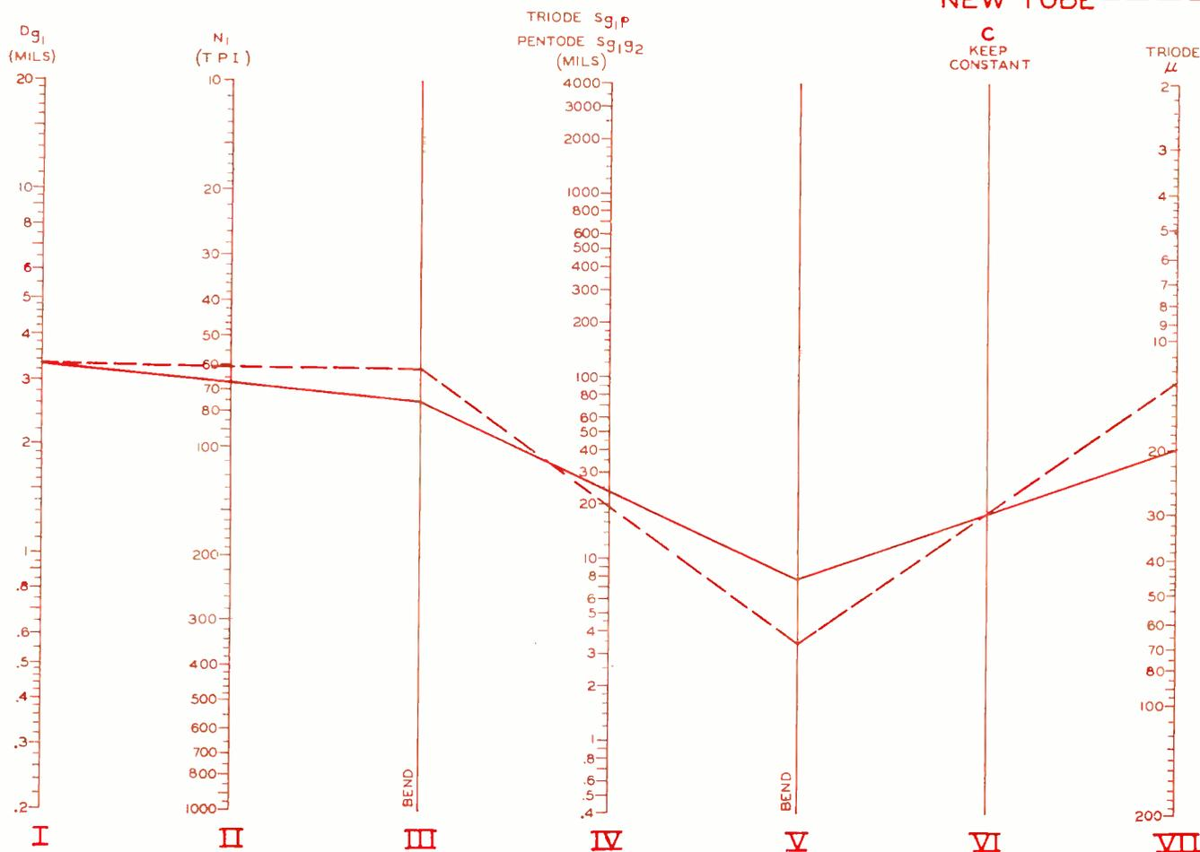
Fig. 7: The parameters of the new tube, which used the 6SN7-GTB as an original, can be determined by working back on this nomograph.
