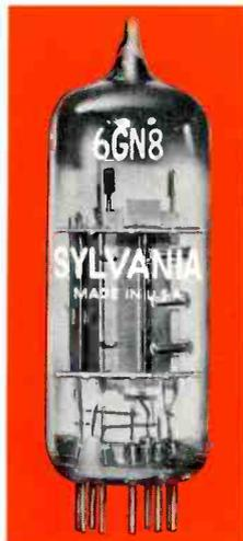
**6GN8** . . . a 9-pin miniature with a *triode section* for general-purpose use as a voltage amplifier or for service as a sync-separator, and a *pentode section* for video-output service. The *pentode section* is equipped with a cathode especially designed to provide "cool" operation with resultant extended life and reliability.
