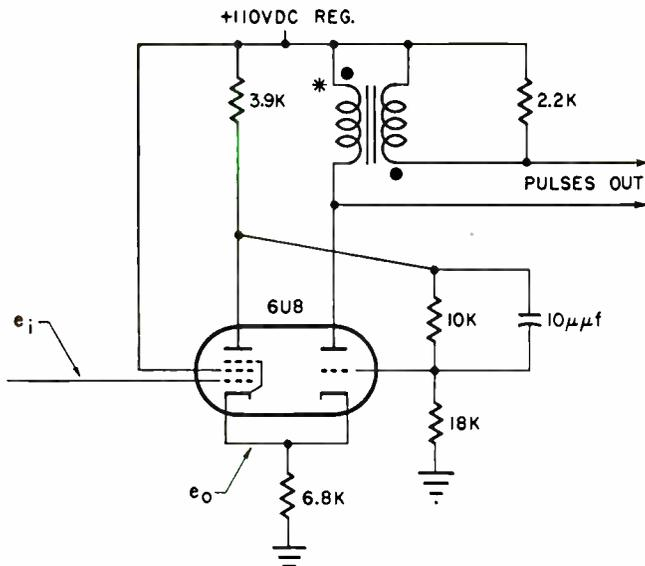
Fig. 7: Actual Schmitt Trigger circuit used in "7000 Series". Amplification occurs in the pentode circuit. The second stage (triode) operates as a cathode follower to provide a low-impedance feedback signal which is direct-coupled to cathode of the pentode. A pulse transformer in the plate circuit of the triode differentiates plate current changes to create output pulses.
