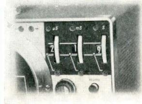
Direct, digital ReadOut of measurement parameters—reducing errors due to interpolations.
