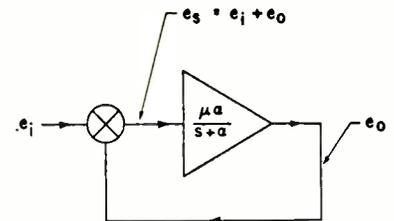
Fig. 4: Block diagram of trigger circuit
