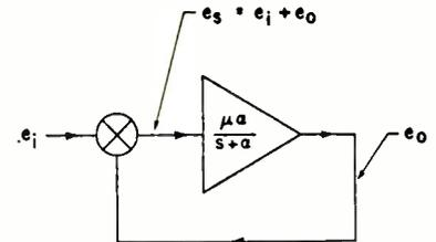
Fig. 4: Block diagram of trigger circuit
