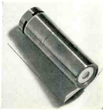
microns; detector area, 3.5 x 3.5 mm.; impedance, 50,000 ohms to 1 megohm; acceptance angle, approx. 100°; response, measured with a blackbody at 500°K at 800 CPS and referred to 1 cycle bandwidth. NEP = 7 x 10<sup>-10</sup> to 7 x 10<sup>-11</sup> w; D\* = 5 x 10<sup>8</sup> to 5 x 10<sup>9</sup> cm/w; time constant, less than 1 microsecond. Applications Engineering Dept., Raytheon Co., Waltham, Mass.
