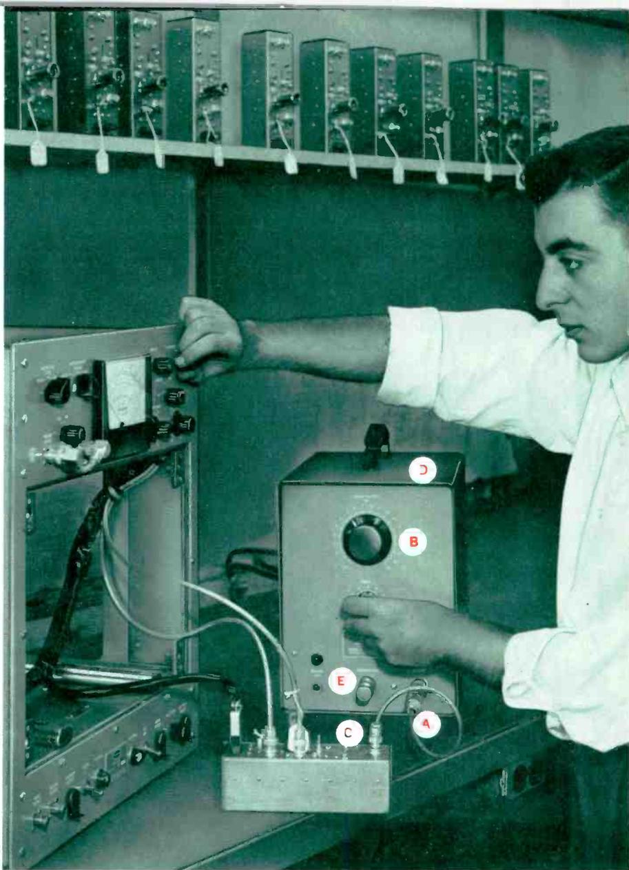
Production line noise figure measurements, made rapidly and accurately with Polarad Model N-1.
