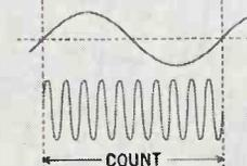
Frequency ratio measurements
