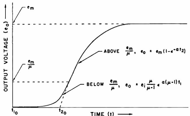
Fig. 6: Curve shows switching action of trigger circuit when input voltage is raised to a point infinitesimally above the trigger level at time  $t_0$  and held constant.
