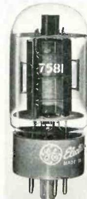
rounded-top envelope for "rattle control" which reduces microphonic action under vibration. Zero-bias characteristics: plate, 70 v.; screen, 300 v.; control grid voltage, zero; plate current, 210 ma.; and screen, 25 ma. Max. ratings: 500 v plate, 450 v screen, 30 w plate dissipation, and 5 w screen dissipation. General Electric Co., Receiving Tube Dept., Owensboro, Ky.
