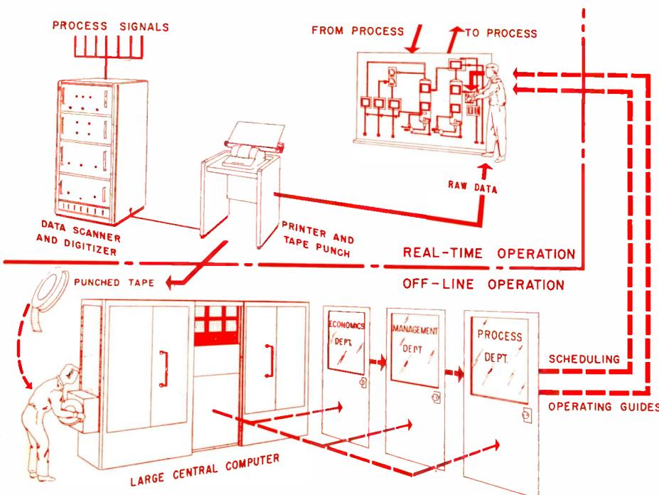
Fig. 2: The information flow when using a small digital computer is illustrated.
