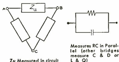
Wayne Kerr Universal Bridge, Type B-221 is a highly accurate transformer ratio arm bridge providing 2, 3 or 4-terminal measurement of impedance or transfer admittance over an extremely wide range. An impedance between any two terminals may be easily measured regardless of other impedances from either or both terminals and a third point. Measurement is unaffected by impedance of test leads.
