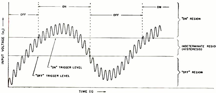
Fig. 3: Diagram showing how hysteresis of trigger circuit discriminates against noise.
