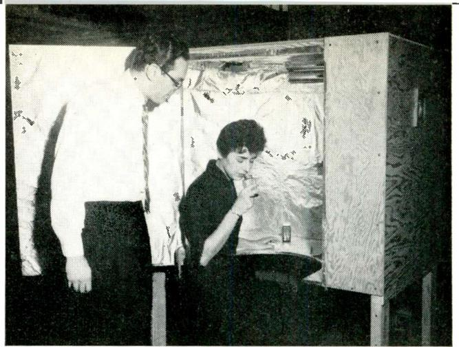
Fig. 14: Battelle Memorial Institute built this booth for conducting experiments to determine the relation between physical characteristics of odorants and their subjective odor properties. They are studying this and others as possible alternate inputs to the man-machine system.
