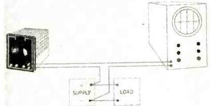
istics of dc power supplies by removing the dc component and utilizing the scope to its max. capabilities. Voltage adjustment is in 75 v. steps for coarse adjustment, with fine adjustment potentiometer 0.25 v./degree; ripple is less than 1 mv RMS. The unit has current limiting and short circuit protection. Acme Electric Corp., Cuba, N. Y.
