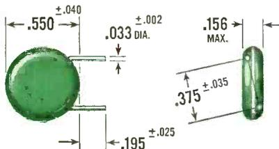
Allen-Bradley Type A capacitors are available in the most frequently used types and capacitance values.
