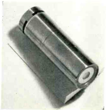
microns; detector area, 3.5 x 3.5 mm.; impedance, 50,000 ohms to 1 megohm; acceptance angle, approx. 100°; response, measured with a blackbody at 500°K at 800 CPS and referred to 1 cycle bandwidth.  $NEP = 7 \times 10^{-10}$  to  $7 \times 10^{-11}$  w;  $D^* = 5 \times 10^8$  to  $5 \times 10^9$  cm/w; time constant, less than 1 microsecond. Applications Engineering Dept., Raytheon Co., Waltham, Mass.
