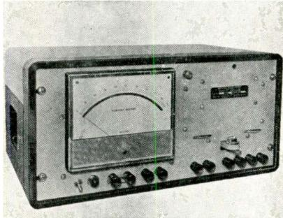
temp. to compensate for decreased current in the moving coil. Coils can be overloaded 400% without degrading accuracy due to heating effects. Ranges are 250/500/1000 w. Input (current) is 5 a. nor. and 10 a. max.; (potential) 50/100/200 v. nor. and 75/150/300 v. max., and outputs of 1 ma in a max. output burden of 5000 ohms (5 v). Frequencies are 40 to 1000 cps. Daystrom-Weston Sales Div., Daystrom, Inc., 614 Frelinghuysen Ave., Newark 12, N. J.
