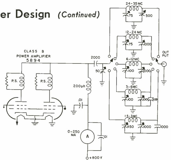
Fig. 3: Pi networks were used to match buffer output to grid of first P.A.
