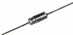
capacitors provide low leakage current, low power factor (or equivalent series resistance) and good temp. coefficient characteristics. They can be supplied in close tolerances. Their stability in performance or in storage is unexcelled and they are designed to withstand extraordinary conditions of high frequency vibration, shock and acceleration. Ohmite Mfg. Co., 3667 W. Howard St., Skokie, Ill.
