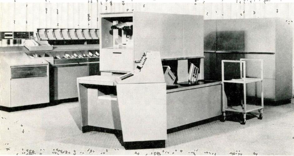
From these stages (above and below) is developed an actual artist's concept of the finished product and finally the final machine shown left. This is Burrough's B251 Visible Record Computer, a solid-state electronic data processing system.
