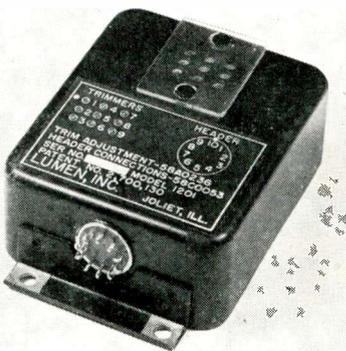
are: amplifier output impedance, 1000 ohms (max.); amplifier output signal, 0-5.0 v.; amplifier output linearity,  $\pm 1\%$  of full scale ( $\pm 50$  mv); amplifier zero shift,  $\pm 1\%$  of full scale ( $\pm 50$  mv); amplifier frequency response, approx. 2 cps; excitation voltage, 28 vdc  $\pm 5\%$ ; amplifier input impedance, 100 ohms per 1 mv input signal. Lumen, Inc., Moen Ave., P.O. Box 905, Joliet, Ill.
