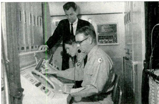
**"Vest Pocket Air Defense System"**—Hughes mobile digital computer and display unit, linked to a Hughes 3-D scanning radar antenna, assigns enemy targets to missile batteries.
