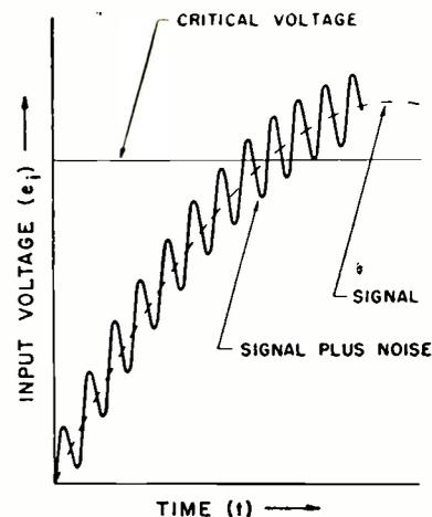
Fig. 2: Noise may cause input voltage to intersect critical value more often than a pure signal would
