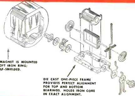
ALNICO MAGNET IS MOUNTED INSIDE SOFT IRON RING; FULLY SELF-SHIELDED.
