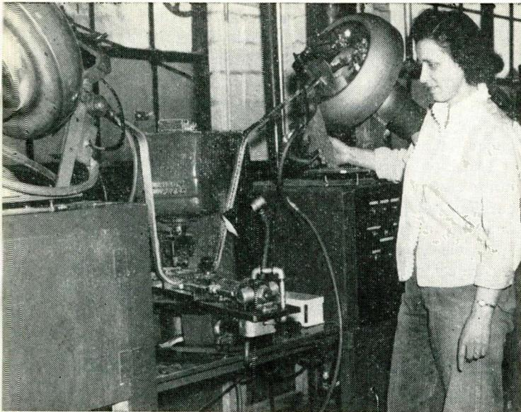
Multipress method using hopper feeds to handle and position component parts for assembly of terminal posts.
