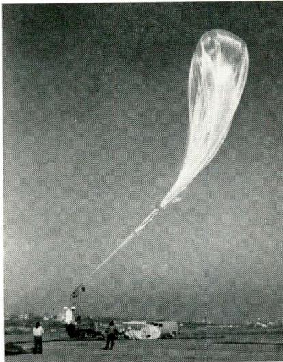
Radar and aerial cameras carried by this huge, 2 million ft<sup>3</sup> balloon photographed the earth's surface from over 100,000 ft. The flight, conducted by Goodyear Aircraft Corp., assisted by General Mills technicians, was part of an Air Research and Development Command research program. Engineers will study the aerial radar photographs in evaluating the characteristics of radar at stratospheric altitudes.
