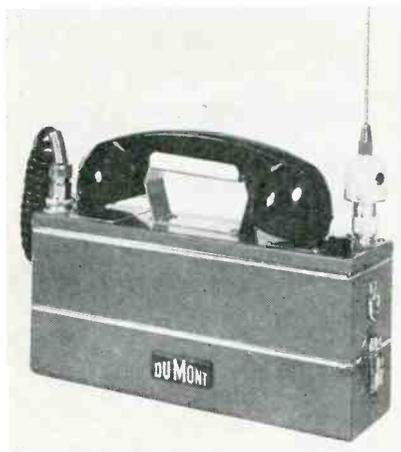
less than 12 in. in length. It includes a handset, FM receiver, 1 or 2 channel FM transmitter, demountable whip antenna, battery pack, and carrying strap. Available with loud-speaker and palm microphone and for use on the 25-54 mc frequencies or 144-174 mc band. Power output in excess of 1 w on lower frequencies. Allen B. Du Mont Laboratories, Inc., Clifton, N. J.
