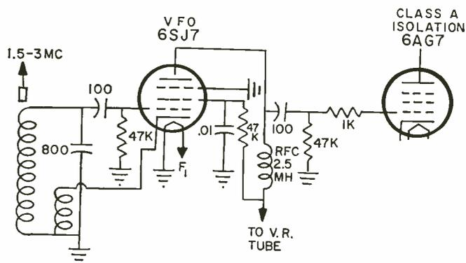
Fig. 2: A stable VFO was chosen instead of a crystal control oscillator because of the need for many different operating frequencies.
