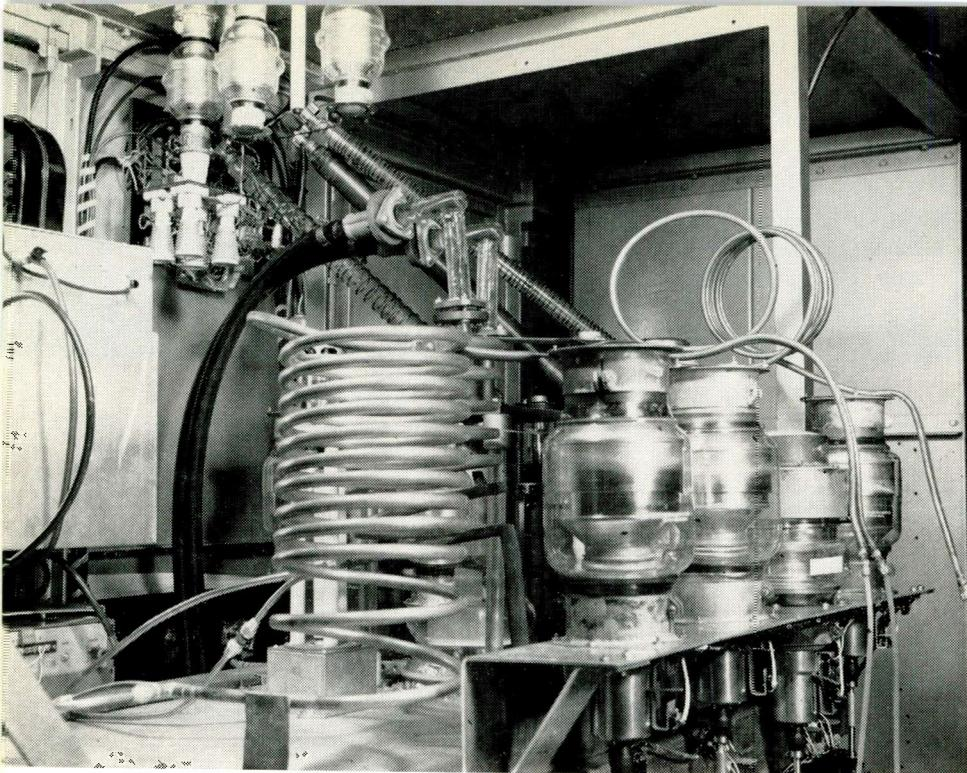
Fig. 1: Final amplifier plate circuits and r-f chokes utilizing motor operated vacuum variable capacitors are shown.
