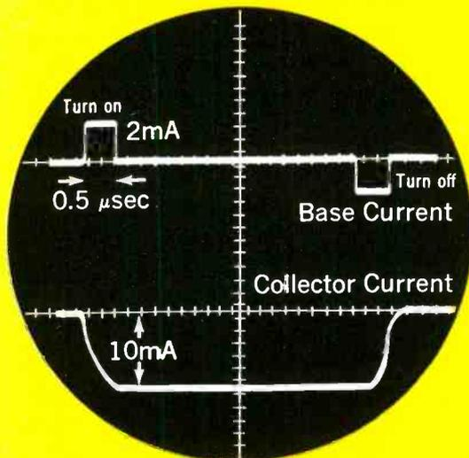
The TRANSWITCH is a new bistable silicon device that can be **TURNUED OFF** with gate current.
