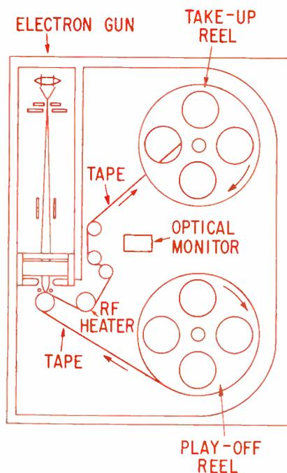
Fig. 2 (right): The film in this TPR machine is handled in a vacuum. Vacuum is obtained in about one minute.
