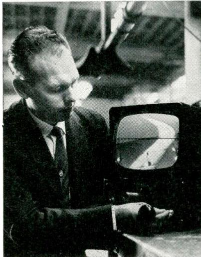
Fig. 15: George H. Balding, Kaiser Aircraft & Electronics, operates the company's Contact Analog Display System. The system will show the pilot at a glance the basic information needed for flight control.
