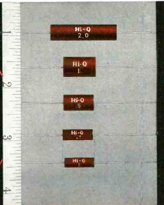
New from Hi-Q . . . a major breakthrough in the design and construction of ceramic capacitors that provides extremely high capacity ceramic units in ranges previously unattainable. CEROL capacitors are rolled ceramic capacitors in the high capacitance range of paper and plastic film dielectrics but in much smaller physical sizes and with superior electrical characteristics.
