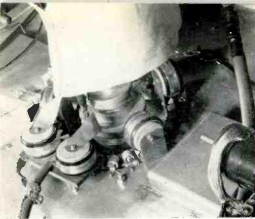
Fig. 6 (left): Final P.A. tube is shown with radially mounted ceramic capacitors. Cloth over tube is air duct.
