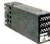
The finished package weighs only 20 lbs.; measures 5" x 8" x 20 3/8". Unit generates 14-digit Point Mugu code, modulating a 1 kc carrier plus a dc time code. Three sine wave and four pulse outputs are also provided, all with only 96 T-Series circuits and 77 watts of input power.
