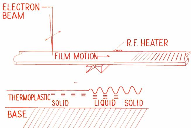
Fig. 1 (left): The melted thermoplastic coating is deformed by the charges. The ripples are then frozen in place.
