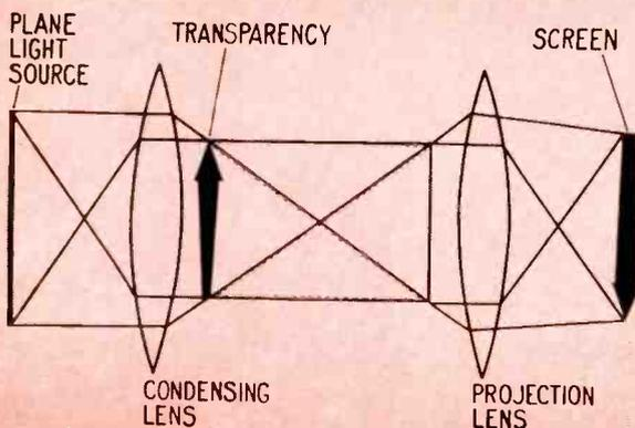
Fig. 4: TPR projector uses line light sources. Bar system acts like a shutter.
