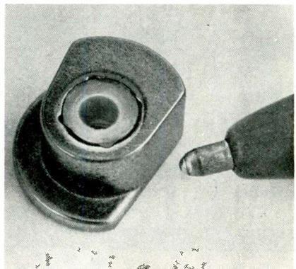
aligning, self-locking and withstand extreme environmental conditions. Self-alignment is quickly and easily accomplished because of a nylon insert. When the screw is tightened, the nylon insert is stripped which allows the clamp to self-align perfectly. The more the screw is turned the tighter the clamp seats. Timber-Top, Inc., 36 Brooklyn Ave., Freeport 8, L. I., N. Y.
