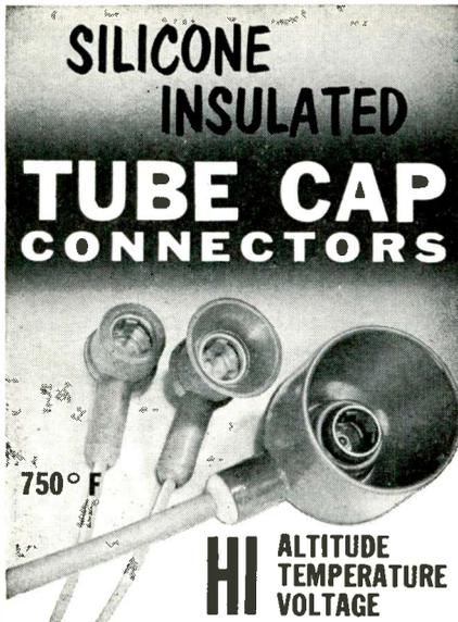
This is a new series of Tube Cap Connectors using special silicone components for high reliability applications. They provide the highest degree of resistance to temperature extremes and are virtually unaffected by ozone and corona. The excellent dielectric characteristics make them ideal for high voltage. Skirts and sealed-in leads guard against flashover at high altitudes. Additional features include anti-corona cup and long-life spring contacts.
