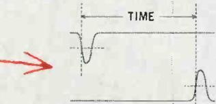
2-channel time interval measurements
