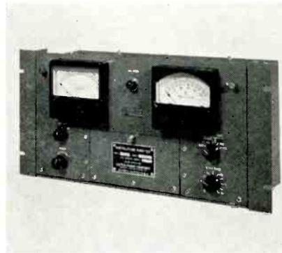
mately 50 msec and will measure the true peak amplitude of program or tone regardless of the wave forms. It can be located at the transmitter and operated by remote control, with compensating adjustments in the monitor for imperfect telephone lines. Gates Radio Co., Quincy, Ill.
