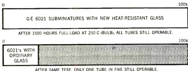
Type 6021 is a key tube in Hoffman's TACAN circuit. Glass electrolysis—cause of 90% of tube failures at high temperatures—has virtually been eliminated by General Electric in the 6021 and other subminiature receiving tubes.
