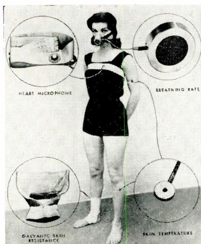
Fig. 6: The well-dressed space pilot will wear many of these medical instruments (designed by Gulton Industries, Inc.). They will measure heart reactions, breathing, temperature, and resistance to shock and stimuli. The breathing rate apparatus, can even tell if he is alive or unconscious.
