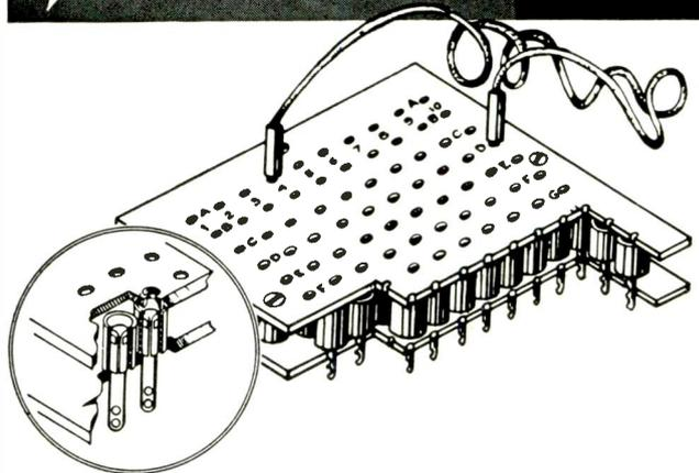
Vector Patch-Boards provide simple, economical units for multiple-connection, single conductor patching. Useful for low cost computers, test boards and a multitude of connecting applications. Receptacles are 0.265" on centers and take .087-.091 diameter plugs. Patch cords also available. Standard boards available or readily made to size required.
