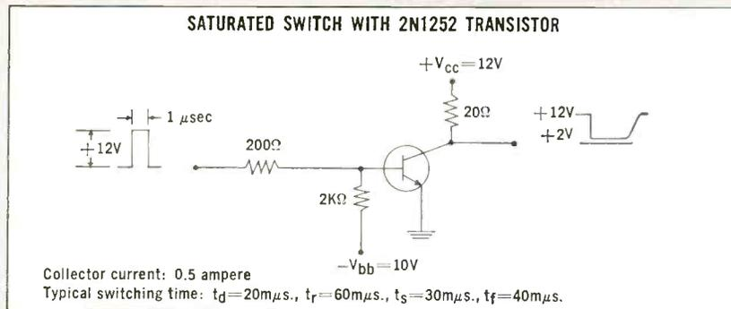
**HOW?** — By using Fairchild's 2N1252 or 2N1253 lowstorage silicon mesa transistors. The guaranteed low storage characteristic permits a simple saturating circuit to achieve switching speeds that previously required complex non-saturating circuits.
