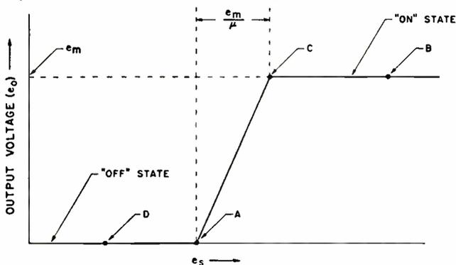
the first phase ( $e_o = 0$  to  $e_o = e_m/\mu$ ) when the output is dependent on the input voltage and, consequently, that output pulses would not be the same shape for all input waveforms. For these reasons the hysteresis (which is equivalent to the peak-to-peak sensitivity of the trigger circuit) must be 6v or more.
