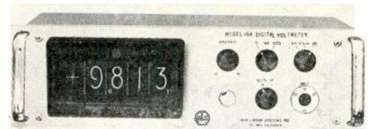
(0.01%) resolution, high input impedance and an average measuring time of 0.75 sec. per reading. It is 5¼ in. high by 15¼ in. deep for mounting in a standard 19-in. rack. Its range without accessories is 500 vdc in steps of ±9.999/99.99/500. Non-Linear Systems, Inc., Del Mar, Calif.
