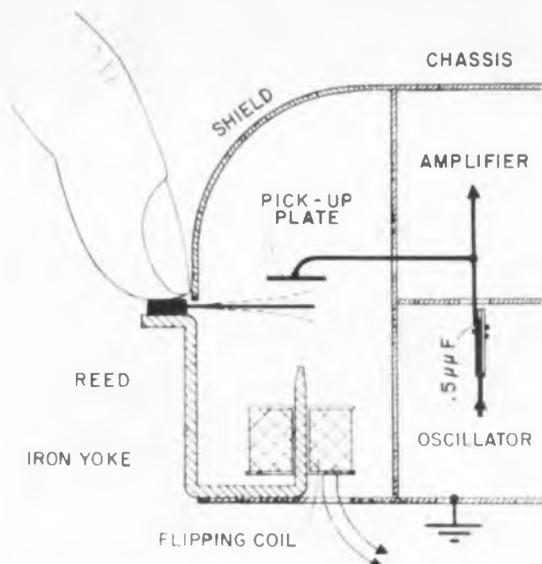
Fig. 1: Varying capacity between reed and pick-up plate modulates r-f carrier.
