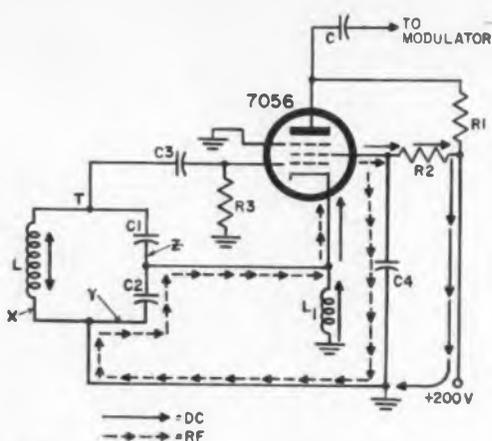
Fig. 1: Oscillator uses series-resonant overtone crystal.
