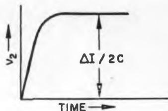
Fig. 8 (right): Waveform of the output voltage.
