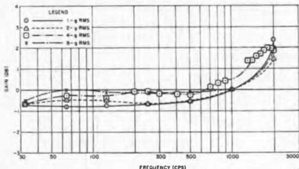
Fig. 8: Response of triangular-shaped transducer configuration.
