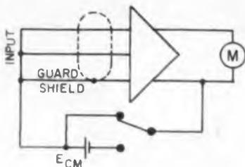
Fig. 9: Setup to be used for ac and dc common mode rejection.
