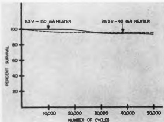
Typical test results for the Sylvania 26.5 volt heater compare very favorably with a 6.3 volt heater of known high reliability. Testing for both types was performed at 120% of rated heater voltage.
