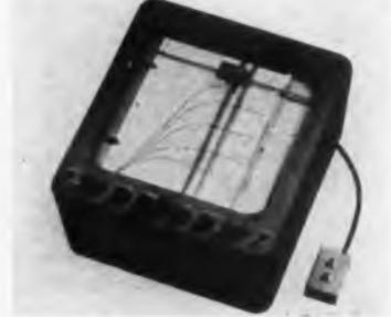
loading, the pen is held so that no trace appears when indexing back to the original position. Accuracy is 1/2% with 7 1/2 in/sec. pen speed on both axes. Houston Instrument Corp., P. O. Box 22234, Houston 27, Texas.
