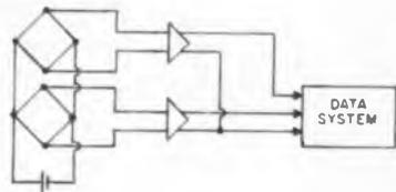
Fig. 2: Strain gages using a common power supply also require isolated amplifiers.
