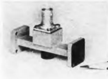
an insertion loss of 2 db. Although designed for K-band, other bands are available with very little change in specs except size. ( $2\frac{1}{2}$  x  $1\frac{3}{4}$  x  $\frac{3}{8}$  in. for K-band unit). If a greater on-off ratio is required, these units can be cascaded in series. A dual unit is available with the same dimensions which had an on-off ratio of 40 db with an insertion loss of only 4 db. The Bendix Corp., York Div., York, Pa.
