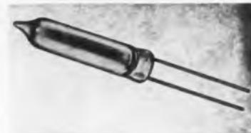
of a pentode which employs high plate voltage. Operation is from -55° to 75°C with min. life over 1000 hrs at recommended operating current. The Victoreen Instrument Co., 5806 Hough Ave., Cleveland 3, Ohio.
