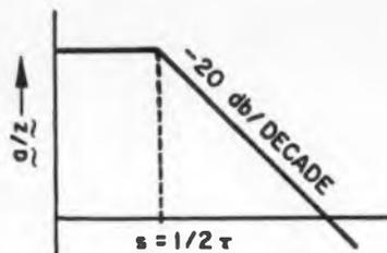
Fig. 7 (left): Subtracting curve  $z$  from  $a$  of Table 4 gives the frequency response.
