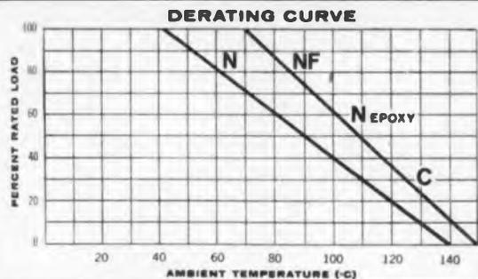
For quantities of less than 1000, contact the nearest distributor serviced by Erie Distributor Division. For data sheets on Corning Type NF, N, N-EPOXY or C resistors, write CORNING GLASS WORKS, 546 High St., Bradford, Pa.
