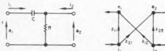
Fig. 1: The first R-C network z-parameters are the open-circuit type.
