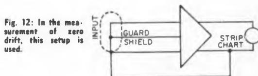
Fig. 12: In the measurement of zero drift, this setup is used.
