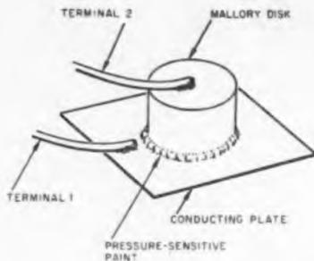
Fig. 1: Application using a weight on pressure-sensitive paint during vibration.
