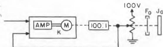
Fig. 3: Wire-wound pot has a 0.05v difference between turns.
