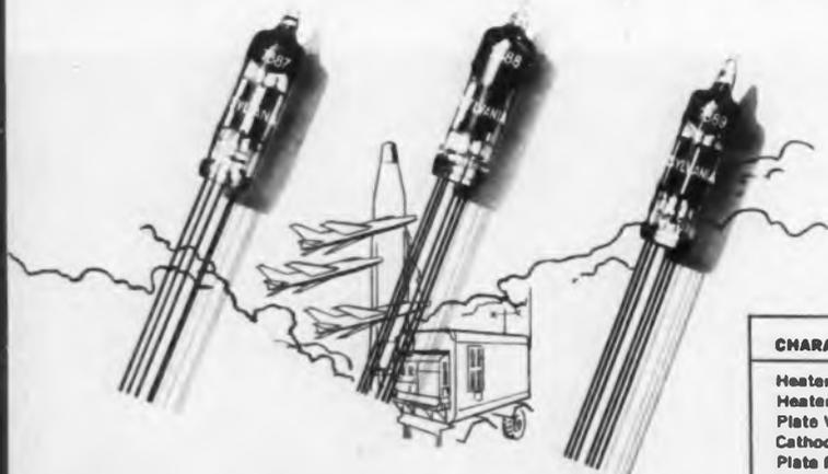
**SYLVANIA-7887.** Medium- $\mu$  double triode; 26.5V, 90mA heater with 100V Eb; designed for oscillator, amplifier and low-power servo circuits.
