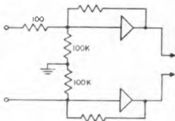
Fig. 5: Common mode rejection ratios of direct coupled differential amplifiers depend on input balance.
