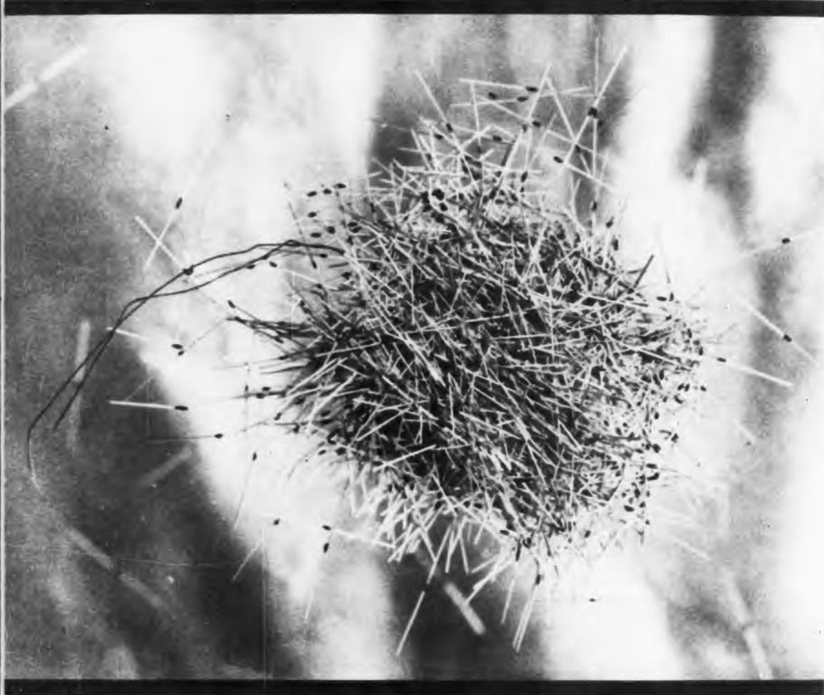
Here's reliability so big you can barely see it. A needle and red thread almost concealed among thousands of silicon diodes demonstrate the super-miniaturization of PSI Micro-Diodes. These are the smallest known semiconductor devices, with reliability equal to or greater than conventional diodes.
