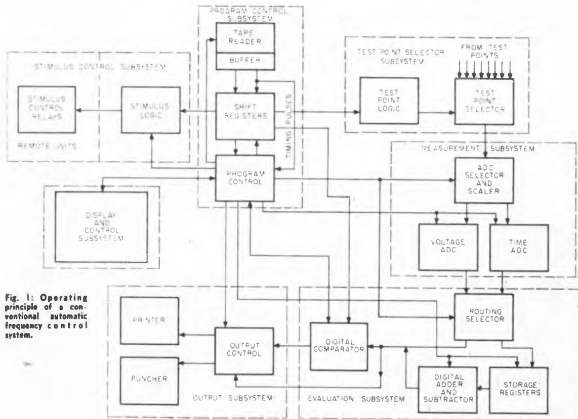
Fig. 1: Operating principle of a conventional automatic frequency control system.
