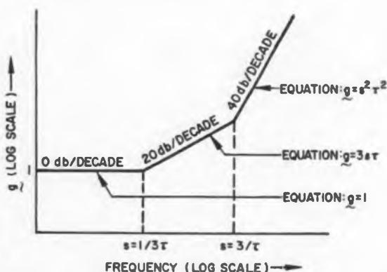
Fig. 5: Plot of individual portions of the curve for  $g$  in Table 4.
