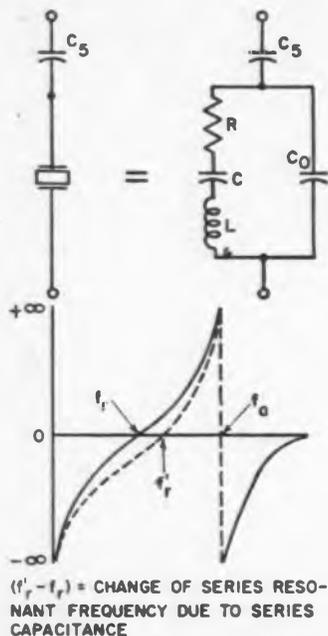
Fig. 5: Effect of adding series capacitance.
