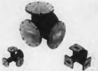
tees are equipped with appropriate iris or ramp matching devices. Design and fabrication techniques result in excellent reduction of VSWR values relatively wide bandwidths. Also isolation between the shunt and series arm is greater than 35 db over the applicable freq. range. Units are constructed of silver brazed brass which is silver plated and finished in instrument grey enamel and all arms are provided with standard waveguide cover flange connectors. Wave-line Inc., Caldwell, N. J.
