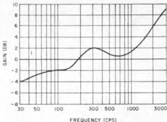
Fig. 7: Freq. response of transducer (see Fig. 6e).
