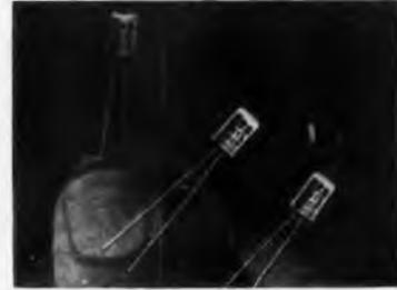
tion, computer and other data processing equipment where precise low voltage regulation is required. Diodes may be used in series for higher reference levels. Rated at 200 mw power dissipation at 25°C, it has a max. dynamic impedance of 20 ohms at 7.5 ma, and a power derating factor of 1 mw/°C. Units measure 0.330 x 0.230 in. (dia) max. International Rectifier Corp., 1521 E. Grand Ave., El Segundo, Calif.
