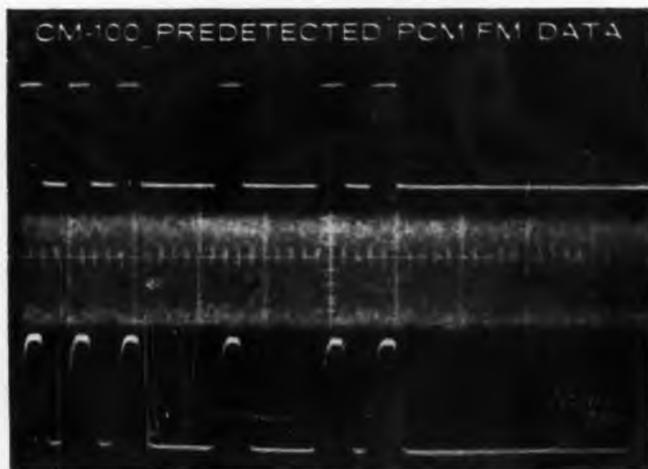
5.0-mc IF carrier heterodyned down to 750 kc. Random-spaced pulses.
