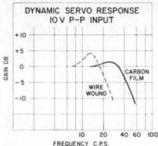
Fig. 5: Servo response curves show one advantage of carbon pots.
