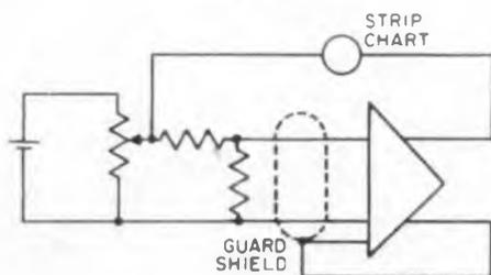
Fig. 11: In the measurement of high gain stability use this setup.
