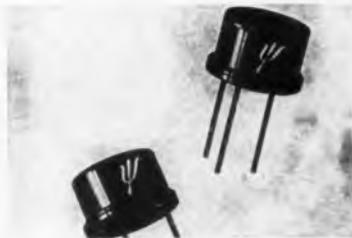
to emitter voltage drop of the 2N697. Additionally, the 2N1837 has nearly three times the small signal beta, half the collector capacitance and half the leakage current. All other characteristics are equal to or better than the 2N697. Pacific Semiconductors, Inc., 12955 Chadron Ave., Hawthorne, Calif.
