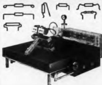
**AUTO FORMER, Model UF2RL**, with optional handy hopper feed attachment, automatically cuts and forms pig tails (leads of resistors, capacitors, etc.) up to 5000 per hour. This versatile machine will cut and shape any conceivable lead form on any component body with coaxial leads. Handles short-run production economically. Pays for itself quickly in time saved and quality of work.
