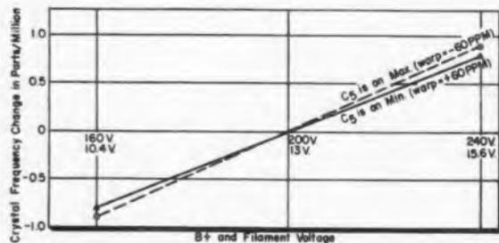
Fig. 6: Crystal oscillator stability over the total warp range vs. B+ and filament voltage.
