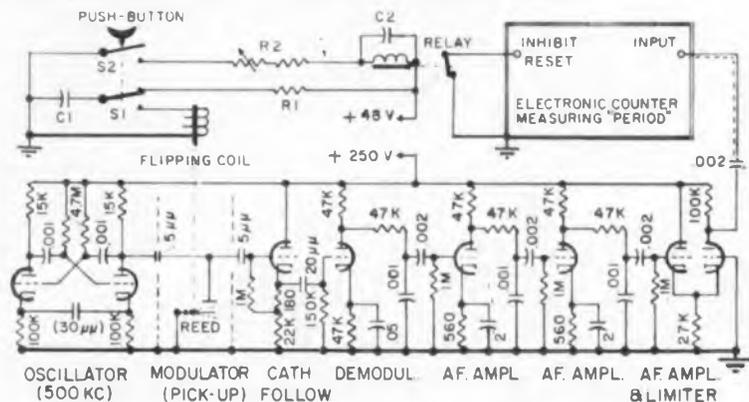
Fig. 2: Counter is held inoperative with "Inhibit Reset" line grounded through relay contact.
