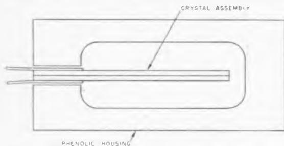
Fig. 5: Transducer assembly.
