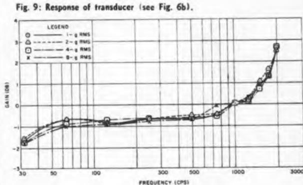
Fig. 9: Response of transducer (see Fig. 6b).
