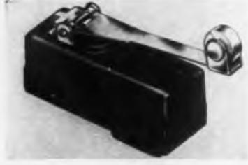
vironmental conditions. It is listed by Underwriters' Labs., Inc. for single-pole, double-throw operation at 2 hp 250 vac, 1 hp 125 vac, 20 a 125 vac. Basic switch is 11/16 in. wide, 1-15/16 in. long, 13/16 in. high and has 2 mounting holes on 1-in. centers. Series also includes leaf, roller-leaf, and hinged-lever actuator styles. Switches can be furnished with solder-lug, screw-type, or snap-on terminals. UNIMAX Switch Div., The W. L. Maxson Corp., Ives Rd., Wallingford, Conn.
