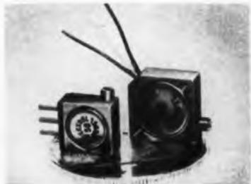
and MIL-E-5272C, Procedure I. Model 50 is available from 50 to 20K ohms and Model 60 from 50 to 50K ohms. Model 50, weighs 1 gm, is rated at 1 w at 50°C and Model 60, weighs 2 gm, rated at 2 w at 40°C. The 25 turn units meet all applicable military specifications for altitude, fungus, salt spray, humidity, sand and dust, temperature cycling, shock and vibration. Spectrol Electronics Corp., 1704 S. Del Mar Ave., San Gabriel, Calif.
