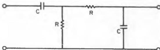
Fig. 3: The networks of Figs. 1 and 2, in series, form this circuit. The Jacobians for this composite circuit are shown in Table 3.
