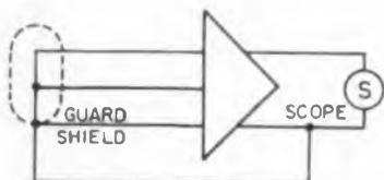
Fig. 10: Test setup for amplifier noise.
