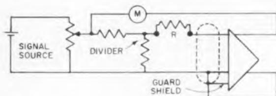
Fig. 8: Setup to be used for input and output impedance measurements.
