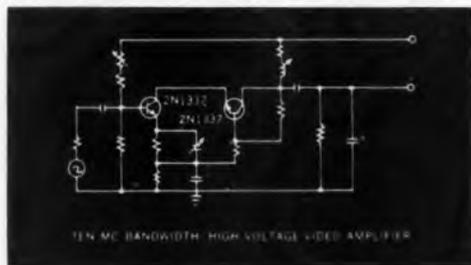
The higher power dissipation, faster rise time and lower collector capacitance of the 2N1337, for example, makes this transistor an unusually fine performer in advanced video amplifier circuits.
