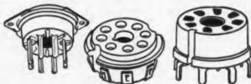
Bottom mounting molded octal sockets for one inch chassis holes and mounting holes 1 5/16 in. apart. This socket has the wire-wrap type tails and is available from Elco Corp.
