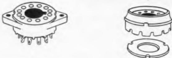
Duodecal C.R. tube sockets with twelve contacts for use on television sets have bodies of general purpose phenolic or mica-filled low-loss phenolic. These sockets fit on the neck of the tube and have no other means of fastening except by its contacts to the pins of the tube. The contacts are of hot solder coated brass and are available from Hugh H. Eby Inc., Cinch Mfg. Corp., and several others.
