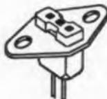
Sockets can be swaged or cemented into chassis or mounted with rings. The bodies are low-loss mica-filled phenolic, or general purpose phenolic. Contacts are available silver plated or silver plated with gold flash. Available from Cinch Mfg. Corp.
