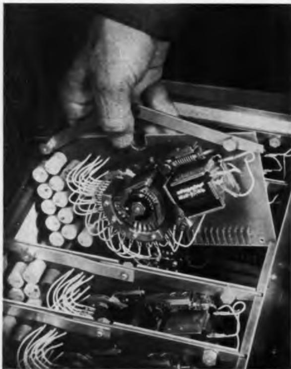
*Plug-in stepping switches in the digital voltmeter section of the RS2 permit replacement of all switches and decade resistors in minutes instead of days. The plug-in feature allows almost instant troubleshooting by the substitution method.*
