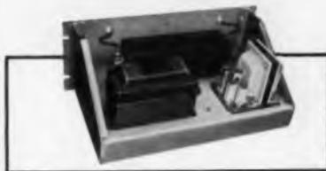
Useful in Radar systems requiring extremely wide bandwidths such as countermeasures, surveillance, high resolution and special communications equipment. Standard units available in octave bands from 40 to 600mc. Broad band units are available to 1000mc on request.
