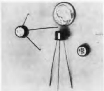
for Nixie tubes, indicator and neon bulb applications. The device is also rated for 200 ma. collector current. Housed in a standard TO-5 package, it has a 4-point mounting internal substructure with 2 connections for the base tab rather than the customary single connection. Motorola Semiconductor Products Inc., 5005 E. McDowell Rd., Phoenix, Ariz.
