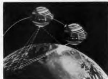
Transit IIIB satellite will carry a 7-lb. transmitter-receiver which will give accurate data on the relative locations of continents, cities, islands, and other landmarks around the globe. Cubic Corp. makes the transponder.
