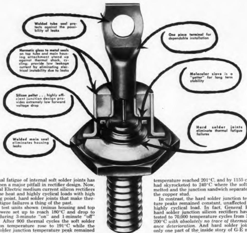
Thermal fatigue of internal soft solder joints has long been a major pitfall in rectifier design. Now, General Electric medium current silicon rectifiers beat the heat and highly cyclical loads with high melting point, hard solder joints that make thermal fatigue failures a thing of the past.
