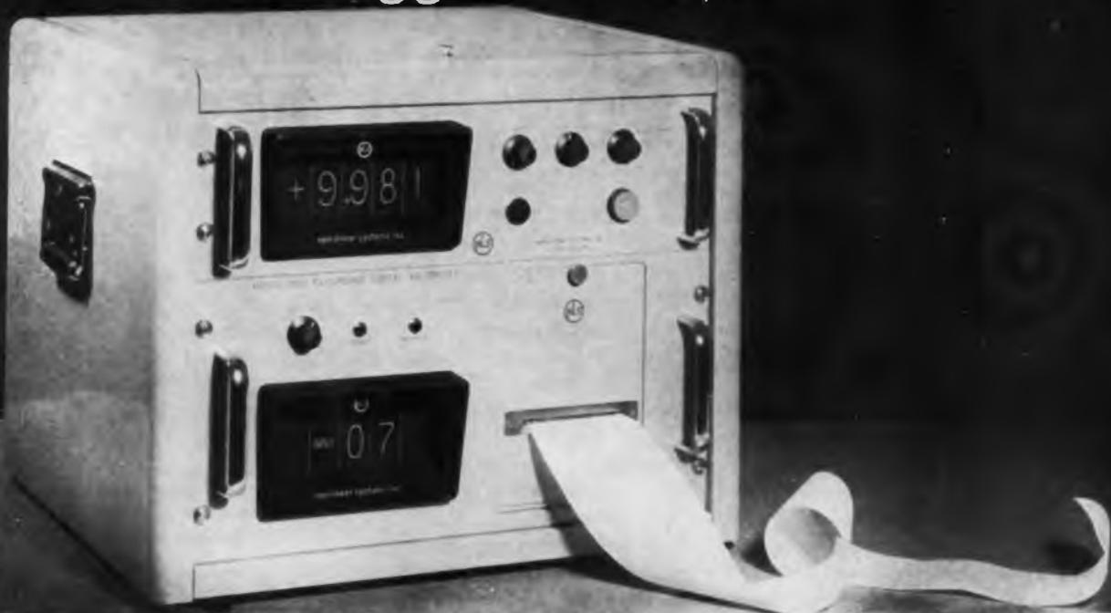
*The RS2 Recording Digital Voltmeter — now in volume production at Non-Linear Systems, Inc. — scans up to 20 double-pole input channels . . . measures DC voltage from  $\pm 0.001$  to  $\pm 999.9$  with  $\pm 0.01\%$  accuracy . . . and records input channel number and the 4-digit voltage measurement. Uses include research and development, quality control, environmental and reliability testing.*
