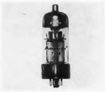
lower, and as an output tube in Class B push-pull circuits. The tube features high transconductance of 25,000 micromhos, low screen grid current (4 ma), and a peak voltage of 6 kv. The cathode current is 300 ma. It has a low distortion for 60w. output in push-pull class B circuits. Amperex Electronic Corp., 230 Duffy Ave., Hicksville, L. I., N. Y.
