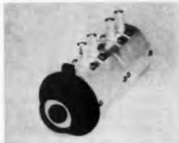
The complete units can be used to operate 2 separate r-f circuits or can be wired in series to double or triple the range of a single attenuator. The Model TAA 50 consists of two 0-50 db attenuators with 10 db steps. It can provide up to 50 db attenuator to each of 12 circuits or 100 db in 20 db steps to a single circuit. Telonic Industries, Inc., Beech Grove, Ind.
