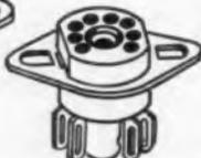
lium copper or silver plated brass and are of the "tuning fork" type. To prevent moisture trap, Sylastic Sealer is applied inside the laminated phenolic washer which holds the contacts in place. These sockets are available with or without center shield from Cinch Mfg. Corp.
