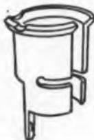
These sockets are used with pencil tubes 5675, 5676, 5893, 6173, 6263 and 6264. Insulating bodies are of general purpose phenolic or mica filled low loss phenolic. Contacts are silver plated beryllium copper with twisted tails. The clip connects to cathode of tube and is made of silver plated beryllium copper. Available from Cinch Mfg. Corp.
