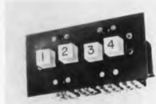
button to return to normal or "at rest" position. Circuitry is dpdt; electrical ratings 5 a @ 125/250 vdc; 5 a (res.) @ 30 vdc; 2.5 a (ind.) @ 30 vdc. Overall length is 3 3/8 in. WC 1730 is designed to meet Mil-S-6743, Mil-S-6744 and Mil-E-5272 as applicable. Control Switch Div., Controls Co. of America, Folcroft, Pa.
