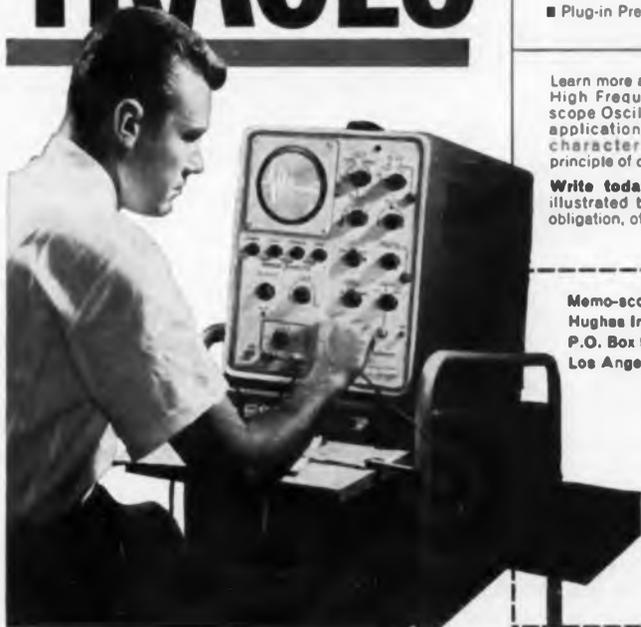
The all-new Hughes High Frequency Memo-scope® Oscilloscope saves you time and money in transient analysis. With its 10 mc bandpass and one million inches per second writing speed, it can store fleeting phenomena for an indefinite period of time. It displays these non-recurring transients for thorough study until intentionally erased. In this way, you can eliminate expensive "hit or miss" methods of transient analysis.
