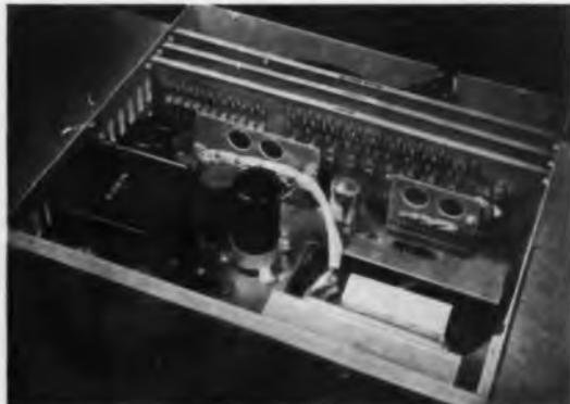
*Note the compact, plug-in modular design of the scanner-printer section of the RS2.*
