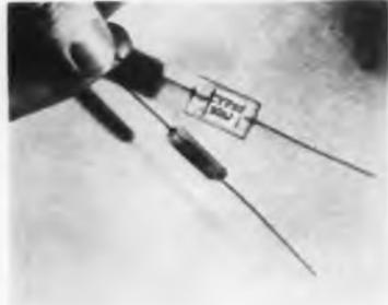
the range of  $-55^\circ\text{C}$  to  $125^\circ\text{C}$ . They are available at 500 wvdc at capacitances between 560 and 3600 pf and at 300 wvdc between 3600 and 5100 pf. Corning Glass Works, Corning, N. Y.
