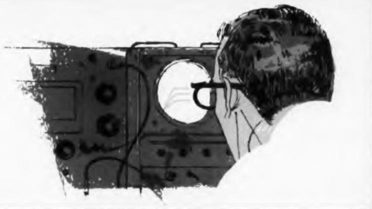
Other factors which are used to insure reliability of Hughes are: a. Rigid visual inspection b. Mechanical vibration under operating conditions c. Mechanical shock under operating conditions d. Thermal shock (temperature cycling) e. Moisture resistance (temperature-humidity cycling) f. Operating and storage life tests at specific temperatures g. In each case, test levels are equal to or greater than the rated values for any given transistor design. Specific failure mech-
