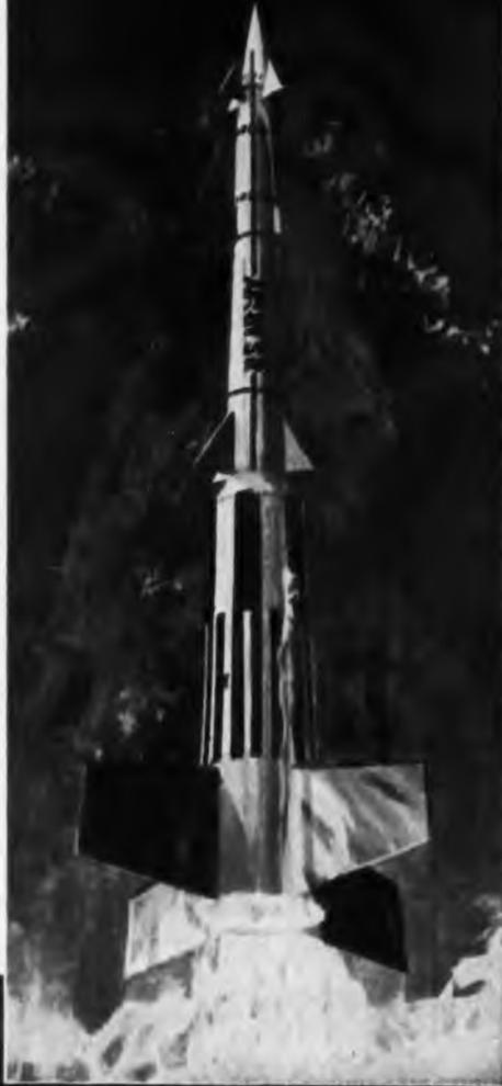
The U. S. Army's NIKE-ZEUS is the only anti-missile missile system under advanced development. It is designed to meet the threat of enemy Inter Continental Ballistic Missiles. Developing a gigantic 450,000 lbs. of thrust at launch, the NIKE-ZEUS missile rises almost instantly to intercept enemy ICBMs traveling faster than 20 times the speed of sound.
