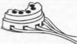
This is an abbreviated duodecal C.R. molded tube socket, developed as a cost reduced type where only five contacts are used. The body is of general purpose phenolic or mica-filled low-
