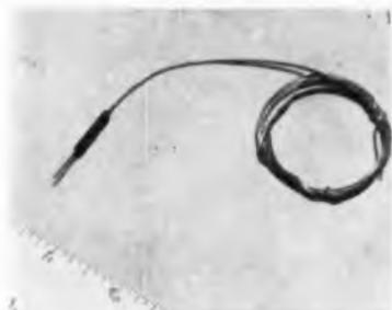
It is a 27 gauge hypodermic needle, made of stainless steel, and has a diameter of 0.022 in. It will accommodate a variety of different thermistors and is useful as a fast time-constant temperature probe. Fenwal Electronics, Inc., 51 Mellen St., Framingham, Mass.
