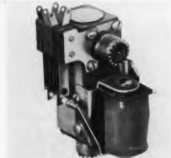
Low VSWR permits use at freqs. up to 300 mc. Relays are ac or dc operated with SPDT internal contacts and up to DPDT auxiliary external contacts. Easy access to internal contacts is provided by a port in the housing. Both military and commercial connectors are available. Specs. are: Pull-in power: dc relay, 2 w; ac relay, 8-10 va. Contact rating: 5 a. res, 2 a. ind @ 28.5 vdc or 115 vac. Duty cycle: continuous. Elgin Advance Relays, Electronics Div., 2435 N. Naomi St., Burbank, Calif.
