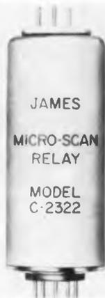
Driving voltage is a nominal 20 v. They have polarized driving systems with center tapped driving coils. Switching circuits are for dry to 10 v. levels with 100 million operations reliability. Models include DPDT and SPDT. Normally open and normally closed circuits are available. James Electronics Inc., 4050 N. Rockwell St., Chicago 18, Ill.
