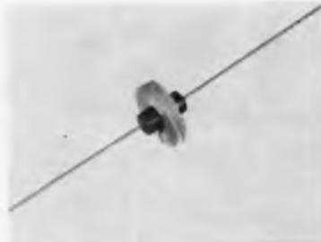
The 1300 series is comprised of 26 video peaking coils designed to assure proper bandwidth and wave shape in high freq. equipment. These coils range in inductance from 20.  $\mu$ h to 950  $\mu$ h. All but 3 of the 26 coils are wound on 0.187 diameter x 3/8 in. long Phenolic form. Numbers 1307 and 1313 are on 22 K resistor form and 1310 on 30 K resistor form. Where resistors are required Mil-R-11 resistors are used. Delta Coils, Inc., 1128 Madison Ave., Paterson 3, N. J.
