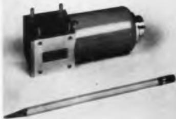
The MA-1064 switches may be pressurized to 45 psi. A low insertion loss of 0.15 db and a max. VSWR of 1.10 over the entire waveguide band are featured. Isolation in excess of 35 db is achieved by design of internal chokes and precision machining. Low holding current of 150 MA is achieved without using dropping resistors. This low holding power minimizes heating allowing operation at ambient temps up to 125°C. Waveguide Systems Div., Microwave Associates, Inc., Burlington, Mass.
