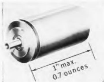
Type 5351-01 is 1 in. long, weighs 0.7 oz., has 0.12 oz. in. torque at stall and 47,000 rad./sec.<sup>2</sup> torque to inertia ratio. The unit can operate continuously at -55°C to +125°C temp. range. No load speed is 9,500 RPM min., rotor moment of inertia 0.18 gm.cm<sup>2</sup>, time constant 0.020 sec. and reversing time 0.034 sec. Rated voltage at 400 CPS is 26 v. (can be available in 18 v. or 33 v.). John Oster Mfg. Co., Avionic Div., Racine, Wis.
