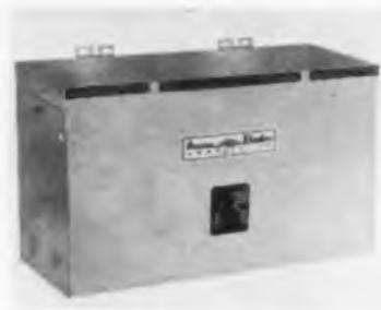
This type of transformer is a code requirement for Class I div. 1 locations in which hazardous concentrations of flammable gases or vapors exist continuously, intermittently or periodically, under normal conditions, during maintenance, because of leakage or during breakdown or as a result of faulty equipment. The line includes ratings from 100 w. to 50 kva, 120 v. input, 120 v. output. Acme Electric Corp., Cuba, N. Y.
