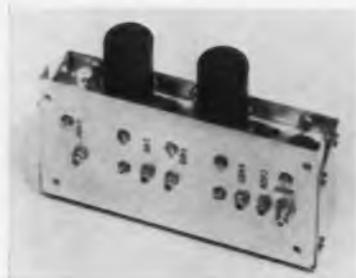
The RF75 is a wide-band r-f pre-amplifier with sufficient gain (over 15 db) to overcome the noise contribution of a following main amplifier. Typical specifications are: center frequency 160 MC, bandwidth greater than 75 MC  $\pm 1$  db, gain greater than 15 db, noise figure less than 6 db, input and output impedance 50  $\Omega$ . LEL, Inc., 75 Akron St., Copiague, N. Y.
