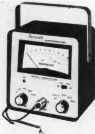
This battery-powered instrument is for measuring surface finishes on metals, plastics, ceramics and organic materials. Model MS 1000 Surfindicator has a rugged pickup stylus that can detect variations of  $\frac{1}{2}$   $\mu$  inch within the measurement range. Three cut-off wavelengths to avoid errors resulting from surface waviness are provided for different ranges of work: 0.030, 0.010 and 0.003 in. Brush Instruments, Div. of Clevite Corp., 37th & Perkins, Cleveland 14, Ohio.
