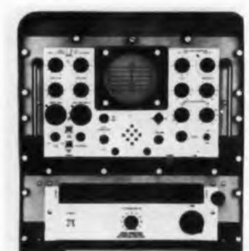
Covers the most widely used communication freqs. for uses including spurious response evaluation, spectrum monitoring, and filter network evaluation. Features are: an operating freq. range of 10 to 1180 mc. Signal sensitivity is 90 dbm from 10 mc to 680 mc, with slightly reduced sensitivity to 1180 mc. 100 kc and 1 mc crystal controlled calibrator gives precise markers for calibration of viewing screen at any spectrum width setting. Lavoie Laboratories, Inc., Morganville, N. J.
