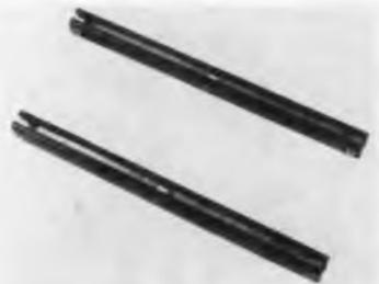
High voltage selenium "channel" cartridge rectifiers are designed for high tension applications such as X-ray, beam welders, precipitators and test equipment. The rectifiers derive their name from the novel channel construction which makes them especially suitable for applications in oil. Dimensions range from 4 1/2 in. long with a cross section 1/2 in. sq. to 8 1/2 in. long with a 3/8 in. sq. cross section. Selenium Div., Radio Receptor Co., Inc., 240 Wythe Ave., Brooklyn 11, N. Y.
