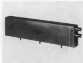
Typical applications are in radar and communication i-f amplifiers. The delay lines are available in various combinations of operation freqs. and time delays generally restricted to ultrasonic type delay lines. Typical time delay values of 0.22  $\mu$ sec, at an operating freq. of 60 MC and a bandwidth of 10 MC are attainable in a unit measuring only 1 x 2 x 10 in. Insertion loss is 3 db. PCA Electronics, Inc., 16799 Schoenborn St., Sepulveda, Calif.
