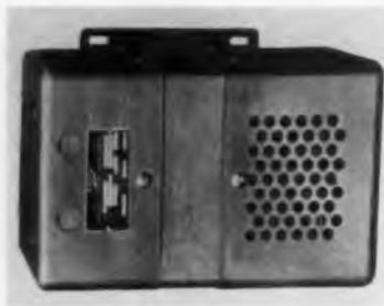
The Sola Standard Sinusoidal Constant Voltage Transformer is completely automatic with continuous regulation. It has a response time of 1 1/2 cps or 25 millisecc. at 60 cps. With no moving parts, manual adjustment or maintenance is unnecessary. The cvs is self-protecting against short circuits on output or load circuit. Available in 29 primary-secondary voltage combinations; 60 to 7500 va. Sola Electric Co., Elk Grove Village, Ill.
