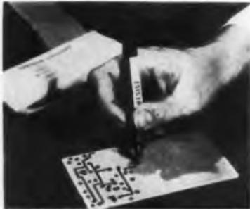
Using the kit's copper-clad Foto-ceram grid boards, resist materials to lay out circuit patterns, and etching materials to etch away copper beyond the circuit runs, a designer can produce a printed circuit on glass-ceramic substrate in 15 minutes, without leaving his desk. Corning Glass Works, Corning, N. Y.
