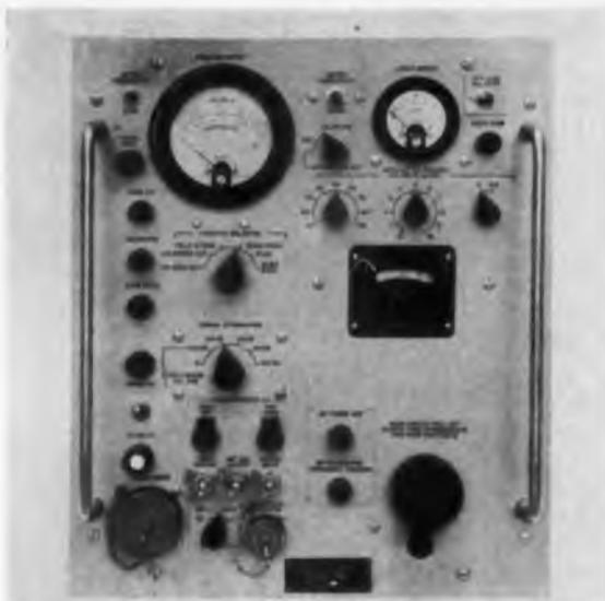
Radio interference set covers from 0.15 to 25 mc. Several types of measurements are available by front panel selection.
