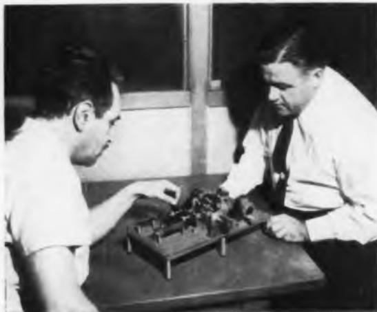
Breadboard parts are assembled according to design drawing. Design can be easily changed if system does not operate as desired.
