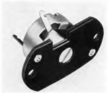
This 3/4 in. dia. reliable preset wire-wound variable resistor has a mounting plate which insulates the control when mounted on a metal chassis. Connection through the cover to the rotating contact is provided by a solder lug. Rating is 1 1/4 w at 40 C derated to no load at 105 C. Three embossed points on the contactor provide continuous contact between contactor, rotor and cover. CTS Corp., Elkhart, Ind.
