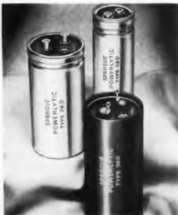
Powerlytic® Aluminum Electrolytics find wide use in power supplies for digital computers, industrial controls, and allied equipment. Ratings to 150,000  $\mu\text{f}$  at 3 v. or 1000  $\mu\text{f}$  at 450 v. are in a standard case size of only 3 in. dia. x 4 1/2 in. high. Standard ratings in working voltages from 3 to 450 vdc at 65°C max. ambient temp. are available. Sprague Electric Co., 233 Marshall St., N. Adams, Mass.
