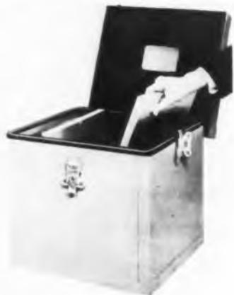
The container is constructed of stress reinforced Netic S-3 magnetic shielding alloy, meeting Mil. drop and environmental specs. Shock absorbing liner allows simple positioning of 1/4 to 2 in. wide tapes in any combination. Rubber gasket, pressure seals upon locking, make the container virtually moisture proof. Containers are currently available for 14 in. reels; other sizes can be fabricated. Magnetic Shield Div., Perfection Mica Co., 1322 N. Elston Ave., Chicago 22, Ill.
