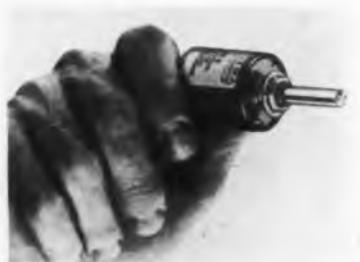
Printed circuit types enable circuit arrangement to provide up to 20 steps of attenuation. Accurate composition 1/2 w resistors are featured in these units with wire-wounds available. Attenuation is increased with counter clockwise rotation. These units are available in the ladder and potentiometer. Specific requirements and performance are the same as the standard type specifications. Cinema Engineering Div. of Aerovox Corp., 1100 Chestnut St., Burbank, Calif.
