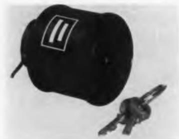
Vaneaxial blower, VAX-3-GN, operates on 115 vac, 60 cps or 115 vdc delivering 85 cfm of air at 1.5 in. static pressure. The unit weighs 1 lb. Diameter is 3 in.; length 3 3/4 in. Mounting is made by clamping to servo rim at either end of the blower. Integral propeller shroud and motor housing is a black anodized aluminum precision casting and the unit is designed to meet pertinent MIL specs. Globe Industries, Inc., 1784 Stanley Ave., Dayton 4, Ohio.
