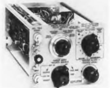
Model 166D Sweep Delay Generator, delays the main sweep of the Hewlett-Packard 160B and 170A o-scopes for detailed examination of a complex signal or pulse train. It offers a new mixed sweep feature to show an expanded waveform segment while still retaining a presentation of earlier portions of the waveform. Thus, both low speed and high speed phenomena can be observed on the same trace. Model 166D's delay time is 1  $\mu$ sec to 10 sec. Hewlett-Packard Co., 1501 Page Mill Rd., Palo Alto, Calif.
