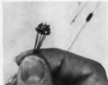
Silicon transistor-diode logic pacs with fan outs up to 5 diodes are available in engineering samples. Diodes are very fast switching silicon computer devices. The transistor used is a 2N1472, having a beta ( $h_{FE}$ ) of typically 35, saturation voltage typically 0.1 v. at 10 ma and a gain bandwidth product ( $f_t$ ) of 175 MC. Philco Corp., Lansdale Div., Lansdale, Pa.
