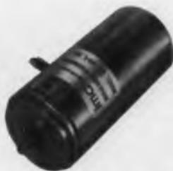
Model BT1004MA measures 1.250 in. long. Designed to operate with transistorized circuitry the unit can also be supplied with any required gear train. Input to the motor is 115 v., 400 cps fixed phase, 20 v. control phase, center tapped. Tachometer input is 26 v. The output voltage of the unit is 0.24 v./1000 RPM. Total weight of unit is 3.2 oz. Standard operating temp. range is -55°C to +125°C. IMC Magnetics Corp., Eastern Div., 570 Main St., Westbury, L. I., N. Y.
