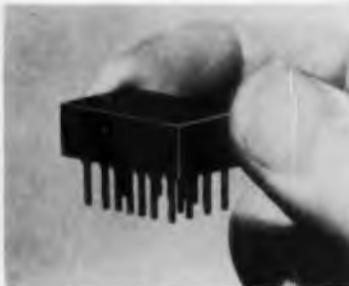
The first BIPCO® module offered is a Binary Coded Decimal-to-Decimal Converter using the 4-2-2-1 code. This device contains 40 silicon diodes and is designed to drive a Nixie® indicator tube directly from inputs encoded in the binary coded decimal form. Typical specs. for the individual diodes are: minimum forward current at 1 v. = 10 ma; max. inverse current at 100 v., 25°C = 5  $\mu$  amps; PIV = 200 v. Burroughs Corp., Electronic Tube Div., P.O. Box 1226, Plainfield, N. J.
