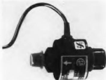
Available in 6 to 64 vdc, 6, 12, 24 and 110-220 v., 60 CPS ac and 110 v., 400 CPS ac models, this valve operates in any position with a max. rate of 1000 CPM at 100 psi. It is also available in water proof and fungus proof models. Using from 1 to 3 w, it will serve under pressures up to 200 psi in temp. from -65°F to +350°F. General Magnetics, Inc., 2641 S. Louisiana Ave., Minneapolis 26, Minn.
