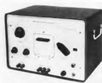
Sine, triangle and arbitrarily modulated suppressed carrier signals of any carrier freq. to 5 kc are available. Applications are: ac or dc servo testing; vibration machine programming; and process control testing. Specs are: freq. range, 0.001 to 10 cps in 4 ranges at  $\pm 3\%$  of set freq.; output voltage, 20 v. max. peak to peak adjustable; load requirements: min. of 10K; output function: cams supplied are for sine and triangle waveforms. Tensor Electric Development Co., Brooklyn, N. Y.
