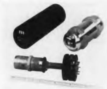
Mercury thermal switch Crystal Oven permits use of a wider range of crystals in both size and freq. The Manson RD-135 Crystal Oven has typical mounting bases: T5½, HC-C/U, HC-13. The unit employs a precision mercury thermal switch, in the form of a miniature thermometer, to provide a constant drift-free reference for close oven control. The heater control circuit is transistorized. The internal structure is completely housed in a thermal bottle. Manson Laboratories, Inc., Stamford, Conn.
