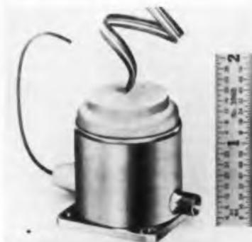
Model LKC-5 is a single cavity oscillator with high efficiency, light weight and no magnetic field requirements. For operation at freqs. from 800 to 13,000 MC, these tubes require only one adjustment to fix oscillation freq. Characteristics are: power output, 5 w cw; beam voltage, 1200 ± 50 vdc; control electrode voltage, 60 v. max.; beam current, 60 ma. max.; half power bandwidth, 7.5 MC. Lewis and Kaufman Electronics Corp., Tube Div., P. O. Box 337, Los Gatos, Calif.
