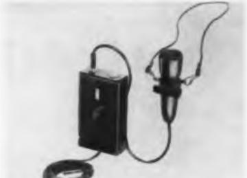
The device consists of a small microphone and a transistorized 10 oz. transmitter. A fixed freq. FM receiver which picks up the transmission can be linked into broadcast or public address systems. The transmitter contains a crystal controlled oscillator operating at high freq. which is directly freq. modulated. It may be used with existing military operations, telemetering, and news and sports events. It covers 20 to 15,000 CFS. The Victoreen Instruments Co., 5806 Hough Ave., Cleveland, Ohio.
