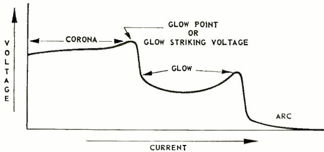
Fig. 5: Curve shows the volt-ampere characteristics of a Corotron.
