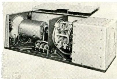
Applying forward current and PIV to the diodes for more than 170°/half cycle, without the large power consumption usually required, is possible with the Daven Model 902 precision motor-driven synchronous switch. Internally protected against overload and overheating, the Model 902 is rated at 200a average forward current and 5000v PIV. Power consumption at this rating is less than 3kw. It will operate unattended for 5000 hrs. The Daven Co., 530 W. Mt. Pleasant Ave., Livingston, N. J.
