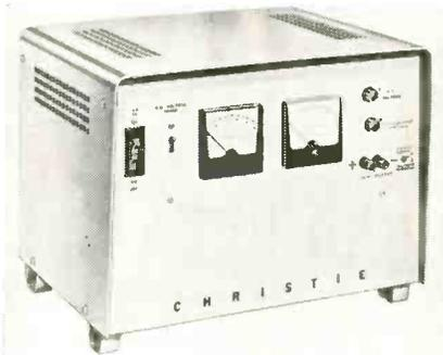
Six models offer a continuous voltage adjustment range of 1 to 145vdc and up to 50a. Standard ac supply source required is 115v, 1  $\phi$  60cps. Unit available for 230v, 1  $\phi$ , for 50, 60, or 400cps and even for all 3 freqs. combined. All models are regulated against line and load variations and have an adjustable automatic battery charging and other constant voltage or constant current uses. Christie Electric Corp., 3410 W. 67th St., Los Angeles 43, Calif.
