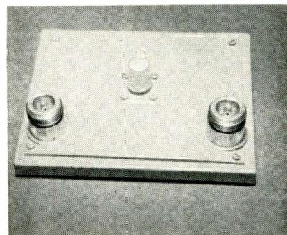
These switches are for receiver protection. Designed for uses from 100 to 2000MC, these reactive coaxial transmission line units handle more than 10kw peak power in the isolating state. Operating temperature is  $-55^\circ$  to  $+65^\circ\text{C}$ . A typical unit, Model SL5, operates over the band 1250-1350MC and has a minimum of 25db isolation in the forward bias state and a maximum of  $0.5\text{db}$  loss in the back bias state. Hyletronics Corp., 185 Cambridge St., Burlington, Mass.
