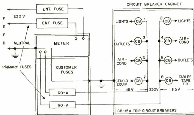
Fig. 1: Typical three-wire 230/115 volt power distribution.
