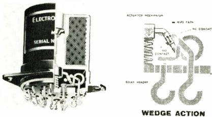
The Type 1000 relay using “Wedge Action,” has a powerful plunger type solenoid to actuate 6 moving contacts. These movable contacts are positioned between 2 rigidly mounted stationary contacts. In either the energized or de-energized position, contact pressure increases between the moving contact and the fixed contact. Low contact resistance, 0.015Ω is assured by electrodeposited 24K gold over an electrodeposited fine silver base. Electro-Tec Corp., 1 Henderson Dr., W. Caldwell, N. J.
