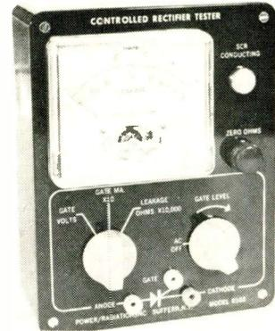
This portable unit determines the gate voltage required to fire the SCR (up to 5v); the gate current required to fire the SCR (up to 50ma); and the anode-cathode or anode-gate leakage (up to 8megs). It comes complete with color coded test leads, and operating instructions. The unit operates from 115v, 60cps. Size is 5 1/4 x 7 x 3 in. Weight is approx. 2 1/2 lbs. Power/Radiation, Inc., Box 616, Suffern, N. Y.
