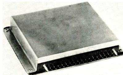
Seven extra inputs are provided for external connection by the user. This or-gate operates from dc to 1Mc. The terminal arrangement is a 35-pin AMP Blade connector. Nominal logic levels are 0 (true) and -5 (false). In the OV condition the signal source must supply up to 1.5ma. Input capacitance is less than 20pf. Voltage shift (output signals) per stage is less than ±0.3v. Model 0-121-DC, DC logic module, will drive 3 or-gates like itself. Digital Design Corp., Box 21, Clay, N. Y.
