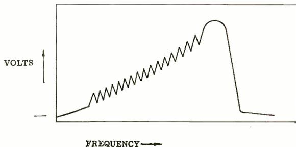
Fig. 4: Relaxation oscillation with r-f sweep generator as driver.
