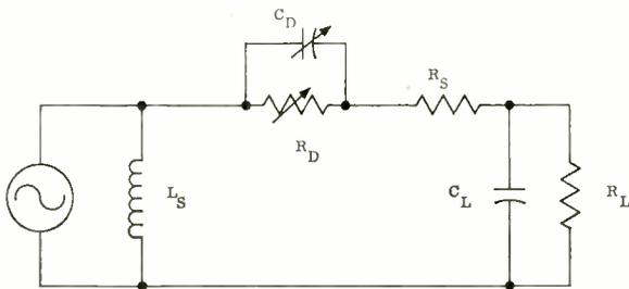
Fig. 2: Equivalent for relaxation oscillation circuit of Fig. 1.
