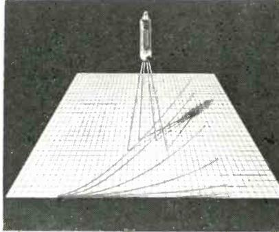
The Type 6977 Indicator Triode is designed for transistor circuits, where its high input impedance will not load the transistors and its small drive requirements are suited to transistor circuit voltages. It can be used to replace neon lamps in electronic computers and data processing systems. The 6977 can be operated from ac or dc supplies and draws 0.03a of heater current at 1.0v. Plate voltage is 50v, and series grid resistance is 100kΩ. Tung-Sol Electric Inc., 1 Summer Ave., Newark 4, N. J.
