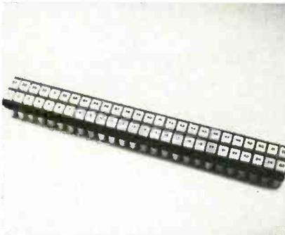
Six basic types offered are: Independent; Momentary Interlocking; Independent Locking and Interlocking; Locking and Interlocking; Locking with Master Release; and Locking and Interlocking with Master Release. Unit shown contains 52 switches mechanically locked and interlocked so that when one button is depressed it remains depressed and releases any other switch previously depressed; no 2 pushbuttons can be depressed simultaneously. Pendar, Inc., 14744 Arminta St., Van Nuys, Calif.
