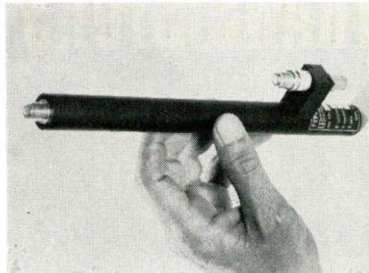
The L-3711 is a metal-ceramic TWT featuring 36db min. small signal gain and high linear saturation characteristics. It is conduction-cooled, measures 12½ in. long and ½ in. in dia. and weighs 21 oz. It operates with temp. compensated periodic focusing and also features high linear power. Helix design and fabrication techniques have raised the saturation gain to within 3db of small signal gain. Litton Industries, Electron Tube Div., San Carlos, Calif.
