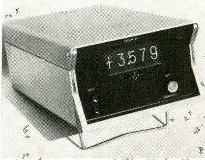
The ASX digital voltmeter measures 5¼ x 8½ x 14 3/16 in. This size allows for internal mounting of such optional equipment as ac/dc converter, battery pack for isolated dc operation, ratiometer, ohmmeter, automatic range and polarity, and printer drive. The voltmeter is in 3 basic models. These consist of completely solid state, reed relay and stepper switch units. Accuracy of each instrument is 0.01% of full scale ±1 digit. American Space Exploration Inc., 3910 S. Kalamath, Englewood, Colo.
