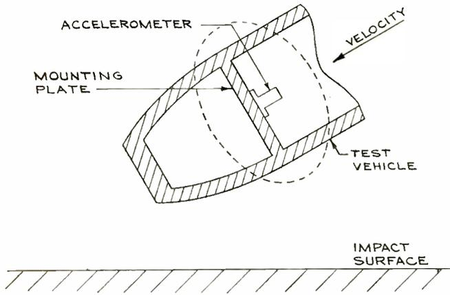
Fig. 2 (l.): Sketch illustrates a typical accelerometer application.
