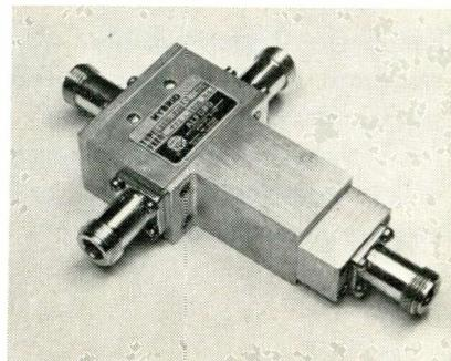
Contained in a rigid, lightweight aluminum housing, it measures 5 27/32 x 4 1/16 x 1 1/8 in. including the 4 Type N connectors. It has a rated min. isolation of 40db over the freq. range of 750 to 1050MC. Max. SWR at the parallel end is 1.3, and at the series end is 1.45. CW power rating is 100w at the parallel end, and 10w at the series end. A complete line, including units operating from 45 to 5000MC and capable of up to 30kw CW, are available. Alford Mfg. Co., 299 Atlantic Ave., Boston, Mass.
