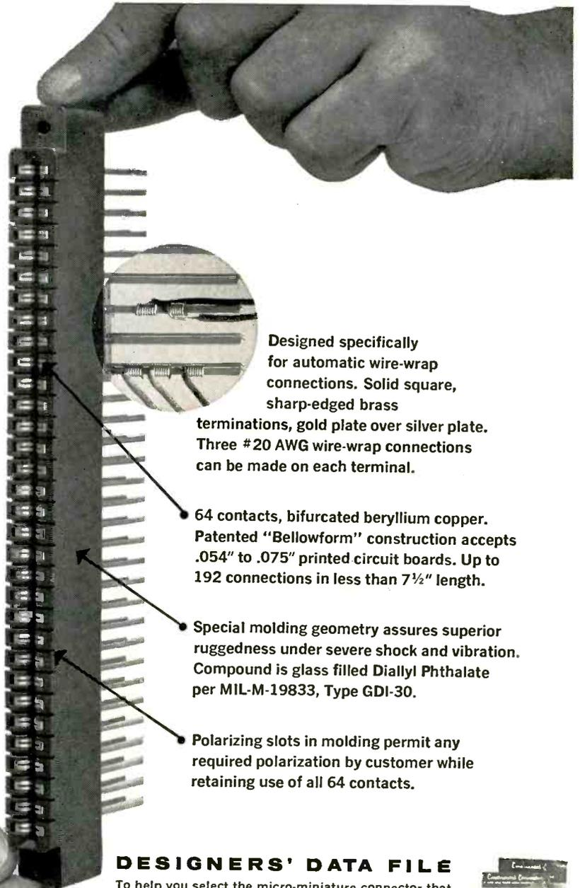
Designed specifically for automatic wire-wrap connections. Solid square, sharp-edged brass terminations, gold plate over silver plate. Three #20 AWG wire-wrap connections can be made on each terminal.
