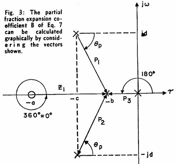
Fig. 3: The partial fraction expansion coefficient  $B$  of Eq. 7 can be calculated graphically by considering the vectors shown.
