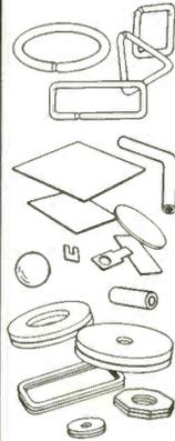
Automatic soldering requires solder preforms of controlled alloy content, size and shape. The right preforms can increase production, guarantee product precision, cut labor costs and provide stronger, smoother joints.
