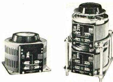
The no-overvoltage version of Ohmite's 20a, VT20, designated "VT20N," delivers just line voltage at max. setting, but the current is 25a. Both the VT20 and VT20N are now available with "B" type enclosure, a basic ventilated metal cover protecting the windings, track and brushes but exposing the transformer's terminal panel. The VT20 and VT20N also available from stock in ganged assemblies of 2 or 3. Larger gangs can be made to order. Ohmite Mfg. Co., 3679 Howard St., Skokie, Ill.
