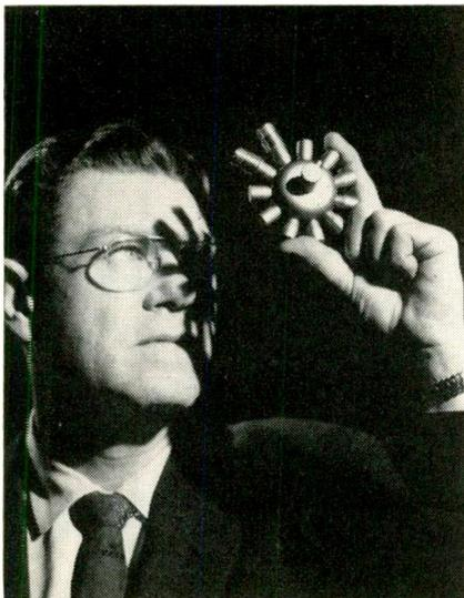
Raytheon Co. space Amplitron delivers more power per pound. Radical design permits use of single small magnet for the tube which delivers 25w, yet weighs only 16 oz. Efficiency of 60%, combined with light weight and compact design make the new Amplitron ideal for space communications systems.
