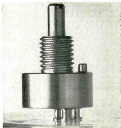
The JP/2 is a panel mount potentiometer, smaller in overall volume than standard  $\frac{1}{2}$  in. miniature pots and considerably lower in cost. It is designed to meet standard military environmental specs. The JP/2 can be interchanged with most  $\frac{1}{2}$  in. pots. It is available in a resistance range from 10 $\Omega$  to 20k $\Omega$ . Waters Manufacturing, Inc., Wayland, Mass.
