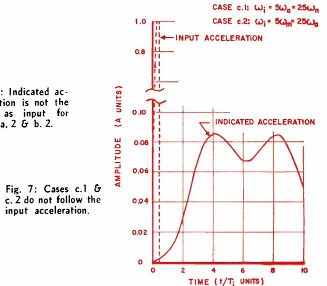
Fig. 7: Cases c.1 & c. 2 do not follow the input acceleration.
