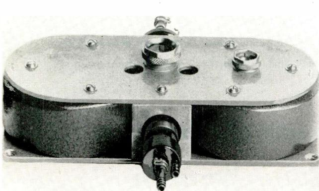
Millimeter wave tubes have found uses as microwave spectroscopy signal sources, maser pumps, power sources for CW or pulsed doppler radars, harmonic generators, local oscillators, in gas plasma experiments, commercial moisture detectors, inter-satellite communication systems, ballistic missile to ground telemetry systems, as well as signal sources for antenna design experiments.
