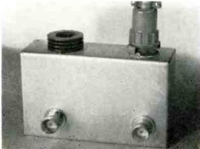
Freq. response is from 20CPS to 50MC flat to  $\pm 0.5$ db, down 3db at 60mc. Gain is 22db nominal. Impedance is  $75\Omega$  in and out with BNC connectors. The compact aluminum chassis measures  $3\frac{1}{4} \times 2 \times 1$  in. and weighs 8 oz. A separate power supply is required to supply 280ma at 30vdc. Other models covering other freq. ranges and having power supplies are available. Community Engineering Corp., 234 East College Ave., State College, Pa.
