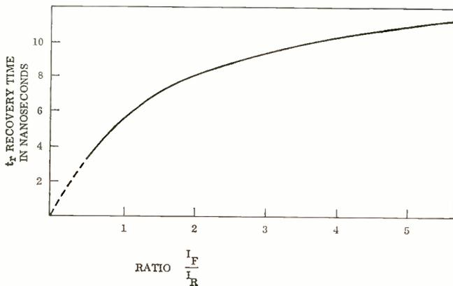
Fig. 8 (above): Typical variation of recovery time with the ratio of maximum forward current to maximum reverse current for a diode.
