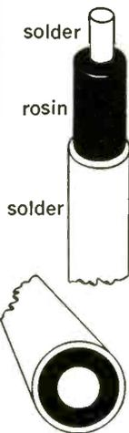
The use of Alpha Cen-Tri-Core® "energized" rosin-filled solder results in more joints per pound as well as higher quality. Here's why:
