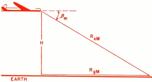
Fig. 1: The Idealized cosecant-squared pattern lies uniformly along the surface of the (flat) earth.
