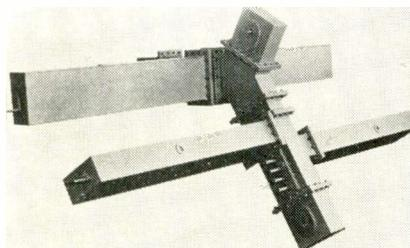
It's tunable over the entire band, can be tuned and locked in just 30 minutes, has a calibration scale which is visible through a pressurized window, and meets all FRC-39 specs. It has an 80db rejection at the center freq., a less than 0.5db pass band insertion loss, and an input VSWR into any terminal of less than 1.2 over  $\pm 3$ MC about the pass band freq. The freq. separation is normally 10%, and power handling capacity is 10kw. Antenna Systems Inc., Hingham, Mass.
