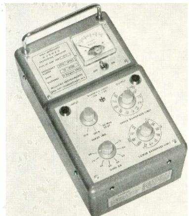
It is a fully transistorized, self-contained, battery-operated amplifier. Noise, with 50meg input, open or shorted, is less than 3 $\mu$ v with a bandwidth of 10kc. Unit has other input impedances of 10 and 100k $\Omega$  for use with lower source resistances. Amplifier has 80db gain with 10db steps. Max. output is 1v RMS on any gain setting. Frequency response is 2cps to 180kc. Millivac Instruments, Inc., P.O. Box 997, 1100 Altamont Ave., Schenectady, N. Y.
