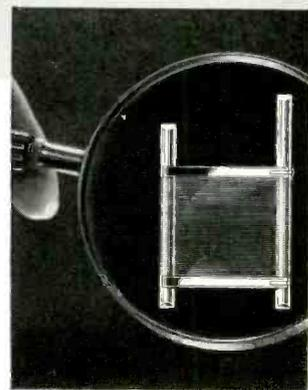
The higher gain bandwidth product and lower noise of Raytheon frame grid tubes mean more reliable performance with fewer tubes. The rigid frame grid design and precision spacing of windings assures minimized spread of characteristics and greater uniformity even under extremely rugged service.
