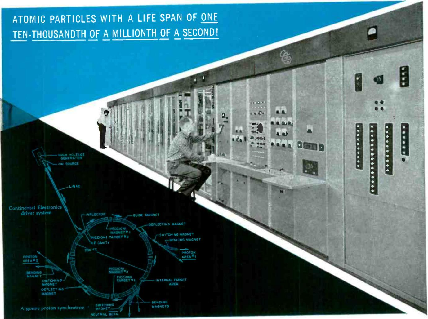
Continental Electronics, specialist in super power electronics equipment, is building the radio frequency driver system for the linear accelerator injector for the proton synchrotron now under construction for the Argonne National Laboratory. This driver system will have a peak power of 5 megawatts, with an average power of 25 kilowatts, operating at a frequency of 200 megacycles with a 500 micro-second pulse.
