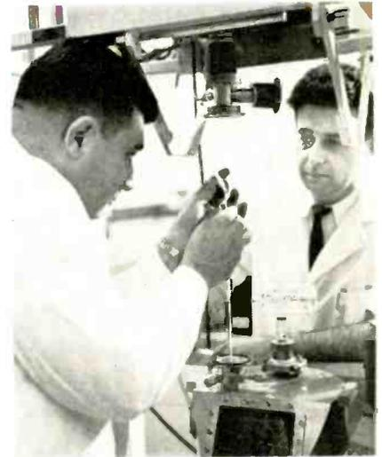
IBM chemists Dr. A. Reisman (l), and M. Berkenblit, who developed a new low-temperature method of synthesizing cadmium selenide directly from the elements, mount a sample in apparatus used in their studies of the Cd-Se system. New method produces ultra-pure, fully reacted CdSe, a compound whose photoconductive properties are of current interest.
