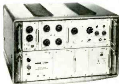
It offers twin-pulse capability as a standard feature. Can be switched in wherever desirable to generate 2 pulses on a common time basis, each pulse having the same width, polarity, and amplitude. Basic instrument specs.: 0 to 10,000 $\mu$ sec. delays; 0.05 to 10,000 $\mu$ sec. widths;  $\pm 50$ v into 50 $\Omega$ ; and better than 15nsec. rise time. Standard modules plug into both front and rear of the rack frames. Servo Corp. of America, 111 New South Rd., Hicksville, N. Y.
