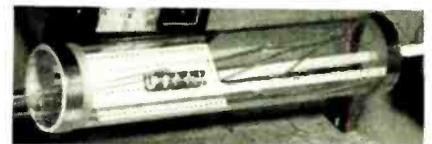
One mounted  $1\frac{1}{2}$ " diam. x 8" long oven, two circuit mounting boards, quartz insulating sleeves, four circuit spacers, connecting wire and ribbon, asbestos tape, thermocouple (Cr-Al), end-plugs, thermal insulating sheet.
