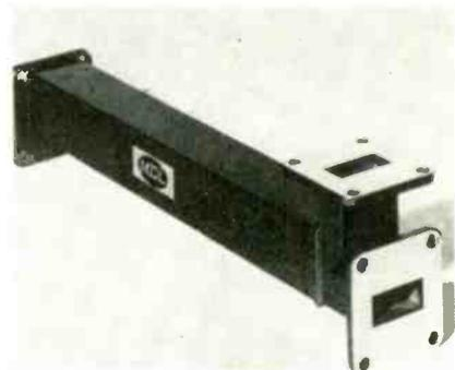
The series is available in EIA WR90 and WR112 waveguide sizes. The line offers 5 coupling ratios of 3, 6, 10, 20 and 30db in each of the 2 overlapping bands covering the freq. range of 7.0 to 12.4gc. New design has allowed a 2:1 reduction in length with little sacrifice in electrical performance. Each coupler is individually calibrated at 5 freqs. over its waveguide band. Microwave Development Laboratories, Inc., 19 Strathmore Rd., Natick Industrial Centre, Natick, Mass.
