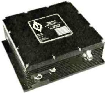
This pressurized VHF Telemetry Power Amplifier has an output of 50w. The anode is mechanically and electrically connected to the housing, providing a thermal connection for vacuum tube cooling. This 6 lb. amplifier, of 115 cu. in., is designed for application in FM Telemetry systems in the 215 to 260MC range. The unit features compactness and overall efficiency is typically 35%, with a power gain of 10db and operates from a standard 28vdc source. Vector Mfg. Co., Inc., Southampton, Pa.
