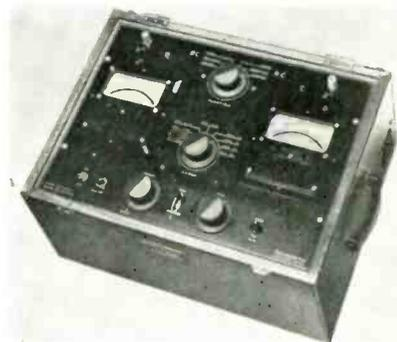
This portable Meter Calibrator supplies accurately metered ac and dc voltage and current for calibration of all kinds of panel and laboratory meters without loading errors. The 54 full-scale ranges cover 20 $\mu$ a to 10adc, 2v to 1000vdc, 20ma to 10a ac and 2mv to 1000vac. AC ranges are compensated and calibrated for 60 and 400 cps; dc supplies are filtered to 0.5% or better. The controls of this instrument are fully interlocked for safety. Twinco Inc., 10 Cheney St., Boston 21, Mass.
