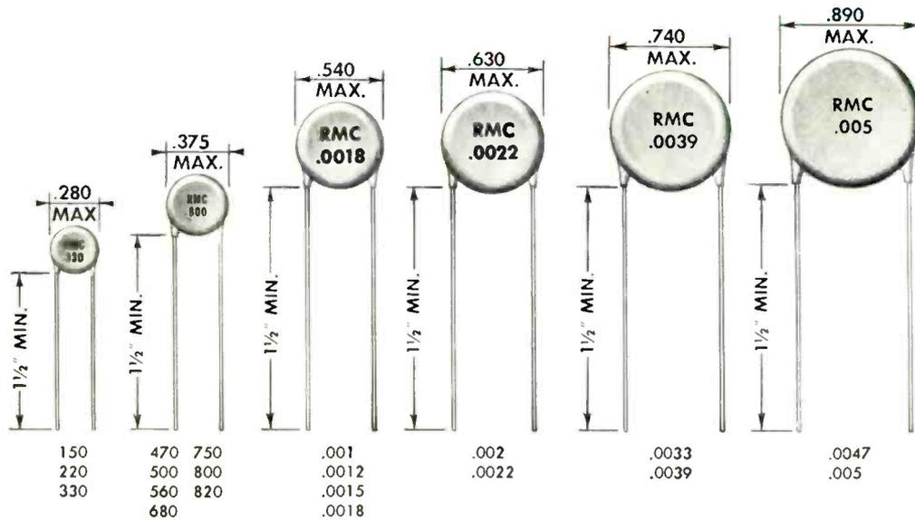
Disc sizes under 1/2" diameter have lead spacing of .250. Discs 1/2" diameter and over have .375 spacing.
