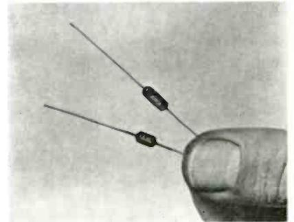
This line of subminiature high voltage silicon rectifiers offers rugged construction, both mechanically and electrically. They are hermetically sealed under pressure and feature high surge ratings. The silicon rectifiers are very reliable under high operating temperatures and require no heat sink. Standard package units are designed for low altitude applications. Semtech Corp., Newbury Park, Calif.
