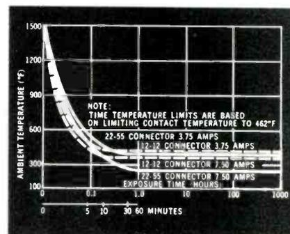
While Amphenol 48 Series Connectors are nominally rated at 200°C, they can also withstand considerably higher short-time temperature exposures.
