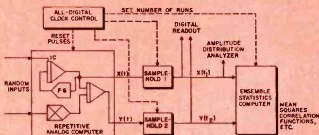
Fig. 1: ASTRAC system operation for random-process studies. Right is block diagram and left illustrates the pulses.
