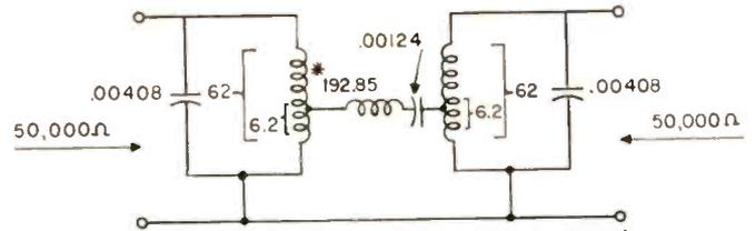
In this configuration, the (192.85 mhy) inductor would have a value of 206.15 mhy to compensate for the mutual inductance in the tapped coils (toroids) L's in Mhys & C's in μfds
