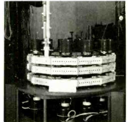
Multiple Beam Klystron
