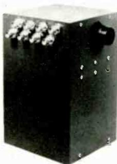
Model CP-10, solid-state diode switch, can be furnished in crossbar-type matrix configurations up to 10 x 10. Its characteristics, over any 20MC band between 0.5 and 60MC are: 1.5db max. insertion loss; 1.1 max. VSWR;  $\pm 0.25$ sec max. differential delay between any 2 circuit paths; 60db min. crosstalk attenuation; and low intermodulation distortion. Sylvania Electric Products, Inc., Sylvania Electronic Systems-West, P.O. Box 188, Mountain View, Calif.
