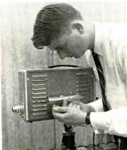
Westinghouse engineer shows new TV camera tube called a slow-scan vidicon, Type 7290, alongside camera in which it is used. Slow-scan system produces one picture every eight seconds. Pictures can be sent over phone lines, stored on a consumer-type tape recorder, or broadcast by radio such as a mobile two-way unit.
