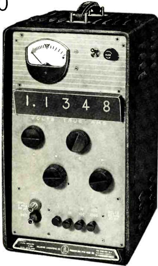
For highly accurate voltage measurements, the uncertainty introduced by waveform distortion limits the use of average and peak-responding instruments. The Model 350 is a 0.25% accurate, true rms-responding instrument designed to overcome this limitation. It provides the engineer with a rugged, reliable and easy-to-use laboratory or production line instrument. It will measure a periodic waveform in which the ratio of peak voltage to rms is not over 2.
