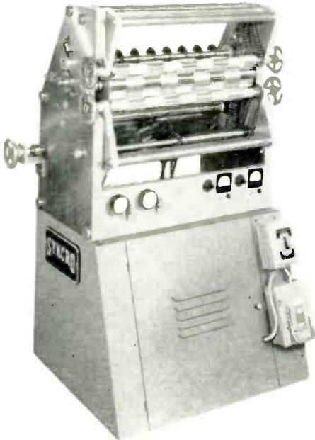
Particularly suited to dead soft strip conductors, these machines are also adaptable to film, fabric, plastic, and paper. Will handle etched, formed, anodized and coated foils without damage. No edge curling or wrinkling; no interleaving, no trimming needed.
