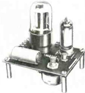
Model DCV-121 is a compactly designed, vacuum tube-transistor power supply. It is designed to provide regulated dc output from an unregulated dc input. The entire circuit is on a printed circuit board provided with threaded standoffs for mounting. It has a typical regulation of 0.02% for both line and load variation. It contains only one vacuum tube, one voltage reference tube, and one transistor. Production Electronics Inc., 525 Lehigh Ave., Union, N. J.
