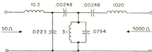
2. Construct a filter with the same characteristics as in problem 1, except that  $R_{in} = R_{out} = 50 \text{ ohms}$ . Using the constant-K values which were calculated for problem 1, it is seen that  $L_{2k}$  and  $C_{2k}$  are very unsatisfactory if one is to get high  $Q$  and small size. A convenient solution is to transform the section by substituting  $\theta = 10$  into Fig. 7. Fig. 21 is thus obtained.
