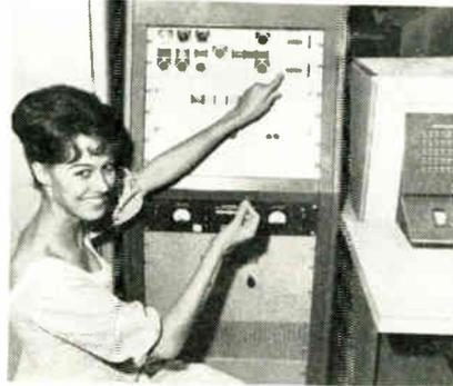
Linda Lee Shryock, a production employee, holds germanium epitaxial mesa transistor which was tested on the Motorola Automatic Sequential Computer Operated Transistor Testing Line at Motorola, Phoenix, Arizona. The system is capable of completely testing, selecting and sorting up to 28,000 transistors per eight-hour shift, or one unit/sec.
