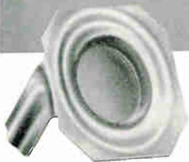
The directional distribution of getter material on the glass envelope is a sure sign of reliable performance of Raytheon tubes. Effective initial tube degassing, directional flash and greater subsequent gas absorption by the efficient Raytheon pressed-pellet getter reduce contamination of tube components for longer, more reliable operation.
