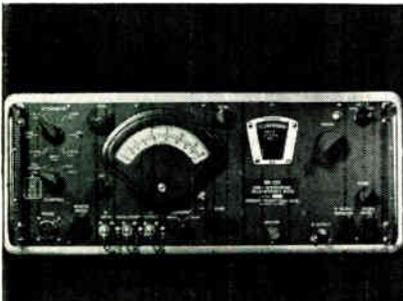
It has built-in capability for data and spectrum signature recording. Both a superheterodyne receiver and a calibrated freq. selective microvoltmeter, the NM-22A features constant gain over the freq. range; 2 selectable 6db bandwidths (3 and 10kc) and analog voltage outputs for freq. vs. amplitude recording. Sensitivity is rated up to  $0.1\mu\text{v}$  and measurement range is 140db. Stoddard Aircraft Radio Co., Inc., 6644 Santa Monica Blvd., Hollywood 38, Calif.
