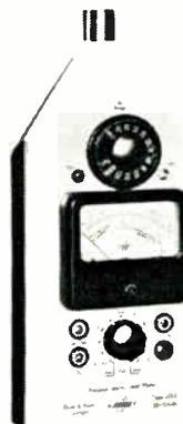
Model 2203, 6 lbs., features a stable accuracy of ±1db from 20cps to 15kc over the range of 31db to 134db. This is obtained through a built-in precision condenser microphone, a case specifically shaped to minimize acoustic reflections, and an RMS detector circuit. Field calibration to 0.2db accuracy is readily performed through use of a Model 4220 Pistonphone Accessory. B & K Instruments, Inc., 3044 W. 106th, Cleveland 11, Ohio.
