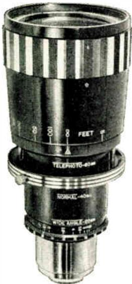
Elgeet offers Vidicon television cameras and 16mm cameras the first Zoom Navitar, a manually-controlled 4:1 zoom with a 20mm to 80mm range— $f:1.8!$  This new lens achievement is optically compensated to hold focus through the entire zoom action. Fourteen elements—covers Vidicon format—resolves 600 lines—linear zoom action by ring—list price: \$400. For information, write for Catalog 2080-CZ18.
