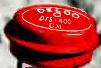
This is the new DTS-400 from Delco Radio . . . one of the highest voltage silicon power transistors available. The DTS-400 offers  $V_{ce0}$ ,  $V_{cbo}$  and  $V_{ces}$  of 400 volts. Because of its high voltage capabilities and its ability to withstand high temperatures, this transistor offers a significant advancement in the art of power conversion.
