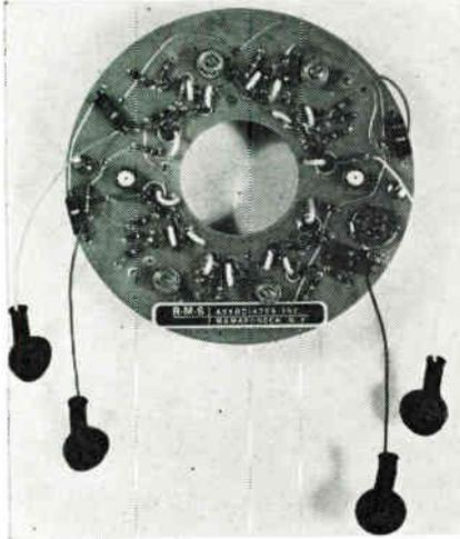
This wide band, fully transistorized deflection amplifier is designed for use with dual deflection CRT's combining electromagnetic and electrostatic deflection, used as output devices for computer generated displays. Type D65701 is packaged on a 5 in. dia. printed circuit board which conserves space and keeps output lead length to a min. Push-pull output/channel is 120v peak-to-peak. Nominal input for full output is 1v across 100Ω. RMS Associates, 805 Mamaroneck Ave., Mamaroneck, N. Y.
