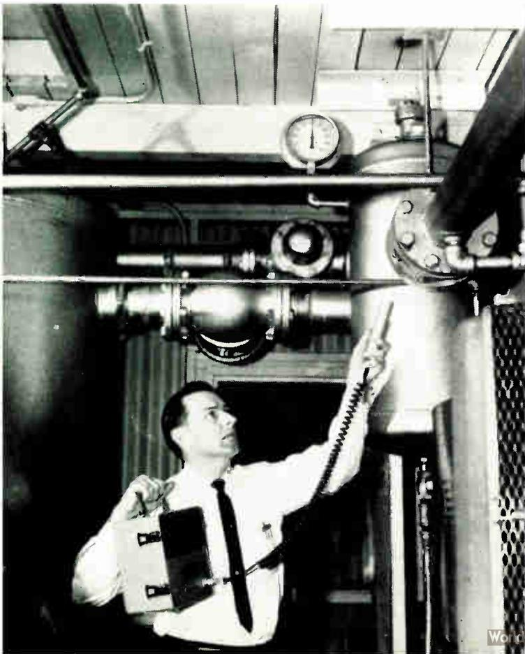
A NEW INSTRUMENT, which can detect and locate air or gas leaks as minute as 0.006 inch in diameter at a distance of 50 ft., has been introduced.
