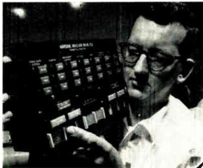
Final GO-NO-GO check of the X-15's adaptive control system is accomplished by this airborne automatic checkout equipment.
