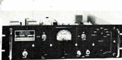
Completely Nuvistorized unit operates with a B+ of 60v. The adapter measures 5¼ x 13½ x 19 in. and weighs 20 lbs. Included is an all-electronic AFC with a correction speed of 50cps/sec. Received carrier is directly compared with a local carrier reference from a crystal oscillator. During severe fades of main and sub-carrier, a RC memory maintains tuning until carrier is restored. Kahn Research Laboratories, Inc., 81 S. Bergen Place, Freeport, L. I., N. Y.
