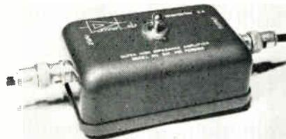
Solid state amplifier has a bandwidth of 3cps to 300kc. Broad-band noise is under  $100\mu\text{v}$  with open input terminals. Model 514A has unity voltage gain. Its output impedance is  $2\text{k}\Omega$ ; adjustable phase shift  $0^{\circ}$  to  $180^{\circ}$ ; detectable signal power is  $10^{-15}\text{w}$ . Denro Lab., 2801 15th St., N.W., Washington 9, D. C.
