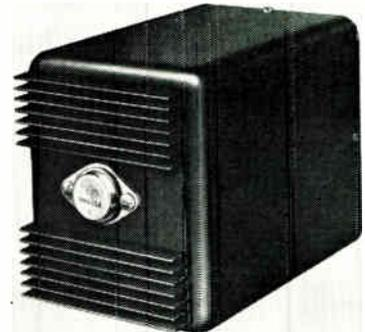
The RVA Series voltage regulated transistorized power supplies are designed to deliver voltage regulated dc power from 105-125vac sources. Input freq. range is 50-400cps. The RVA series is manufactured in 4 constant duty power ratings—15, 30, 60, and 100w. Models from 5vdc to 300vdc are available. The RVA-300-30 (shown) has: input, 105-125 vac; output, 300vdc, 30w; and measures  $4\frac{1}{2} \times 3\frac{3}{8} \times 6$  in. Kupfrian Manufacturing, 160 Prospect Ave., Binghamton, N. Y.
