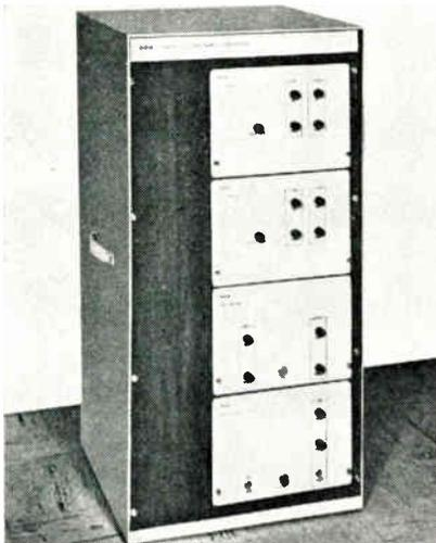
The GEC 6021 Universal Transistorized Scan Converter is designed around a dual gun storage tube and is capable of converting radar PPI data to a bright TV display on an ordinary TV monitor which can be viewed under high ambient light conditions. It is also capable of converting from one TV scan format to another. The entire unit can be rack mounted in less than 37 in. of panel space; weighs 106 lbs. Consumes 175w of power. General Electrodynamics Corp., 4430 Forest Lane, Garland, Tex.
