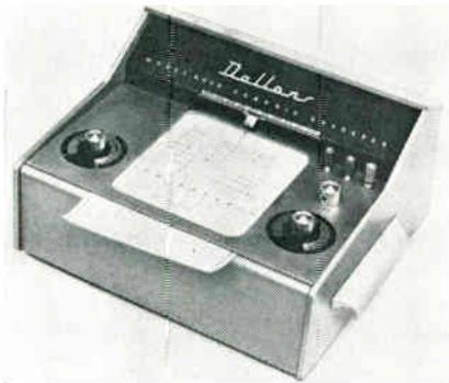
This dual-speed graphic recorder has a 5mv to 50v span. Used in recording dc voltage or current variations vs. time, the Model 5000 provides step selection of ranges from 5mv to 50v by means of a front panel attenuator. It uses a null-balance, servo-type, potentiometric, chopper-stabilized system to eliminate zero-drift problems. Available chart speeds range from 1 in./hr. to 16 in./min. Measures 12½ x 11¾ x 9 in. Dallons Laboratories, Inc., 120 Kansas St., El Segundo, Calif.
