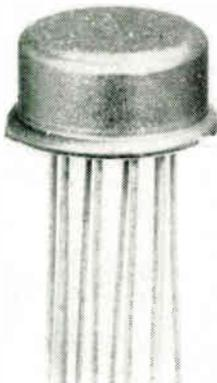
Fig. 1. When network is assembled into a TO-5 type case, it requires about 0.02 in.<sup>3</sup>, not including the leads.
