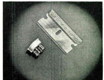
Also accepts other semiconductors using the same 6-pin configuration. Lugs are made of brass, gold flash over silver plate, and are double turreted to accommodate transistor leads and associated circuitry. A seventh hole is for positioning the component. Minor diameter of Teflon body is 0.465 in.; shoulder measures 0.495 in. in diameter. RTC-650-T transistor socket available in white, or any of the standard EIA color codings. Sealectro Corp., 139 Hoyt St., Mamaroneck, N.Y.
