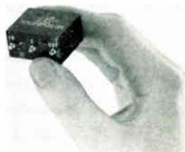
FL-384 through FL-388 subminiature telemetering filters have source and load impedance of  $47K\Omega$ . The units are designed for IRIG channels, A, B, C, D, E, with center freqs. from 22kc to 70kc. Attenuation in pass band ( $F_0 \pm 15\%$ ) is less than 1db. At freqs. below  $0.15 \times F_0$ , the attenuation is over 20db. At freqs. above  $2 \times F_0$ , the attenuation is over 30db. Triad Distributor Div., Litton Industries, 305 N. Briant St., Huntington, Ind. BOOTH 3316.
