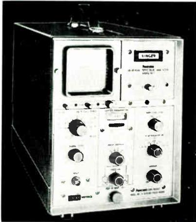
Three plug-in interchangeable modules covering the 20cps to 25Mc range are for use with the portable TA-2 Universal Panoramic spectrum analyzer. Any ac line from 95 to 1000cps will recharge the unit's nickel cadmium batteries. Singer Metrics, 915 Pembroke St., Bridgeport, Conn. BOOTH 2415.
