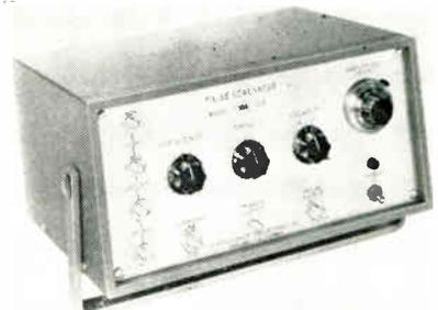
Model 126 uses transistorized circuits and a high-speed coaxially-mounted mercury switch to produce its fast rise times. The fast pulses of calibrated amplitudes make it useful in checking transient response of wide-band systems, fast solid-state switching circuits, computer devices, and nuclear applications. E-H Research Laboratories, Inc., 163 Adeline St., Oakland 20, Calif.
