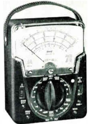
Model 630-PLK has a sensitivity of 20K $\Omega$ /vdc and 5K $\Omega$ /vac. It features  $\pm 3\%$  accuracy on dc and  $\pm 4\%$  on ac. Stray magnetic fields are eliminated by a self-shielding bar-ring movement. It is usable with freqs. through 500kc. The Triplet Electrical Instrument Co., Bluffton, Ohio. BOOTH 3311.
