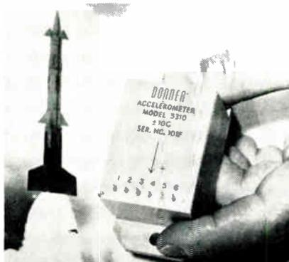
Model 5310 is a servo accelerometer which uses a gravity-sensing system instead of the conventional pivot and jewel suspension system. Designated Flexure Accelerometer, it withstands shock and vibrations up to 500g at 8msec. Systron-Donner Corp., Concord, Calif. BOOTH 2521.
