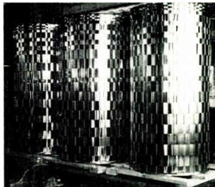
Molybdenum strips, basket-woven to form these cylindrical heat shields create an interesting pattern and form an effective thermal barrier for high-temp. furnace. Molybdenum and other refractory metals for electronic uses are being produced at new General Electric plant near Cleveland.
