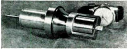
The Model 32-310 is a versatile hermetically-sealed actuator for high-vacuum instrumentation use and feed-through motion transmission. This rotary-to-rotary drive may be manually actuated or motorized. Reduction ratio is 72:1, and servomotors ranging from size 11 to size 18 can be coupled to the input shaft. High-speed input components can be removed to allow bakeout to 400°C. Actuator weight, less motor, is approx. 2 lbs. Harmonic Drive Div., United Shoe Machinery Corp., Beverly, Mass.
