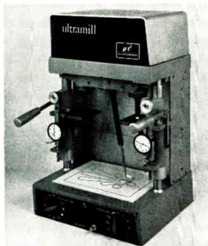
Ultramill is a laboratory tool used for development work in semiconductors and microelectronics. This micro-manipulated machine tool permits direct working from 8½ x 11 in. drawings. Movements traced by a plastic chessman on the drawing are reduced mechanically and transmitted to 2 interchangeable tool housings. The Ultramill machines its own tools. Micro Dynamics Corp., 34118 Pacific Coast Hwy., Dana Point, Calif. BOOTH 4003.
