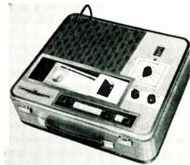
Tracemaster® single-channel portable direct-writing recorder, model 29105, has a timer-event marker to correlate time of data with related events. The marker may be used as a timer or remote timer. The unit has a response from dc to 90cps; is essentially flat at 30mm (P to P amplitude), 3db down at 125cps. Rise time is approx. 5msec. American Optical, Instrument Div., Buffalo 15, N. Y. BOOTH 4525.
