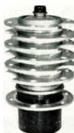
Type RA24A 3-phase vacuum relay operates up to 120 amps each phase and at 115vac (400 cycles). The contacts need only be separated only a few thousandths of an inch to achieve 1000 megohms. Peak test-voltage rating is 2kv. Jennings Radio Mfg. Corp., P. O. Box 1278, San Jose, Calif. BOOTH 1901.
