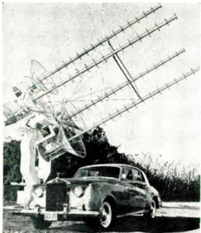
Model 170 antenna pedestal control system is used with ground-based telemetry where the receiving antenna is an end-fire corrugated cylinder surface wave-element array. Control system includes a servo bandwidth adjustment which allows the system to be optimized for any tracking condition. Modifications of existing design are available for mounting parabolic reflectors and multi-element arrays. TEMEC, Inc., 7833 Haskell Ave., Van Nuys, Calif.
