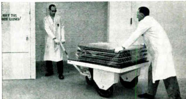
Every precaution is taken to protect the surface. Before leaving the "white rooms" for the laminating presses, copper-clad loads are covered with plastic film to prevent dust or other foreign matter from contaminating the surfaces of the material.
