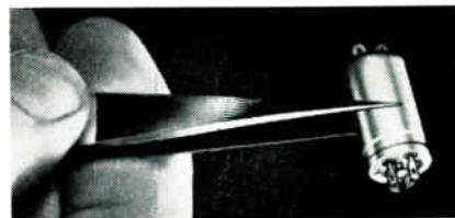
Series F subminiature chopper occupies 0.1 cu. in. and coil requires 160mw when operated at 6.3v., 400cps, and within environmental ratings of: temp., -65° to +125°C; shock, 30Gs; vibration, 0.25 in. D.A. or 20Gs, 5-2000cps. Bristol Co., Waterbury 20, Conn. BOOTH 3409.
