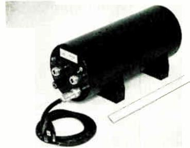
The WJ-269 is completely self-contained, requires only an ac line-voltage input, and is adjustment free. The compact L-band amplifier with its integral power supply weighs less than 17 lbs. Max. noise is 5.5 db from 2.0 to 4.0Gc. Small signal gain is 25 db (min.); saturated power output is nominally -5-dbm. Watkins-Johnson Co., 3333 Hillview Ave., Stanford Industrial Park, Palo Alto, Calif. BOOTH 4505.
