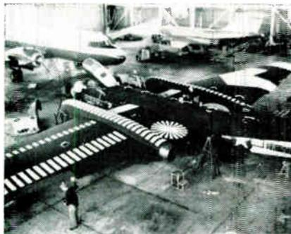
This RB-57D will have its picture taken by remote-control 100,000 ft. above New Mexico desert. Purpose is to test effect of air turbulence on aerial photos. Ground radar ranging unit will track aircraft and balloon holding camera, electronically trigger the camera shutter and film-advance at proper times. Honeywell is conducting tests under \$2.25 million AF Systems Command contract.
