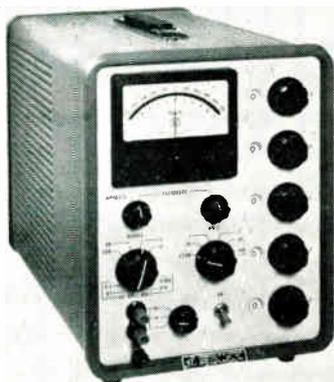
Model 823A has dc voltage measurements of  $\pm 0.01\%$  accuracy and  $\pm 0.1\%$  ac accuracy (infinite at null) over 0 to 500v ranges. It features in-line readout with lighted decimal, dc polarity switch, recorder output, and no zero controls. John Fluke Mfg. Co., Inc., P. O. Box 7428, Seattle 33, Wash. BOOTH 3220.
