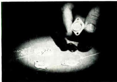
The LDR-25 light-dependent resistor with high power-handling capabilities is now commercially available. In some uses it eliminates the need for high-current-carrying relays. It operates from 110vac and is rated at 200vdc or peak ac. Deleo Radio Div., General Motors Corp., Kokomo, Ind. BOOTH 3814.
