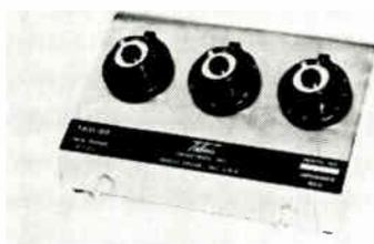
Model TAD-50A is a turret-type decade attenuator designed for r-f signals in the dc to 1000mc range. It contains 3 separate turret attenuators covering 10db in 10 steps, 50db in 5 steps, and 50db in 1 step. Max. error at 900mc is 0.5db for the 1 db-step turret; 0.5db  $\pm 5\%$  for 10 db-step turret, and 3db for the 50 db-step unit. Insertion loss is less than 0.5db and is down below 0.2db at 30mc. Telonic Industries, Inc., 60 N. 1st Ave., Beech Grove, Ind. BOOTH 418.
