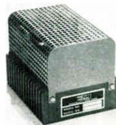
This regulated dc power supply is built with silicon transistors and has a 75°C amb. temp. range. Models are available with output voltages from 6 to 31vdc and current capacities from 600ma to 1.5a. Input range is from 105-125vdc, 47 to 440cps. Consolidated Avionics Corp., 800 Shames Dr., Westbury, L. I., N. Y. BOOTH 4615.
