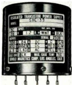
SH series feature input voltages from 12-32vdc ( $\pm 2$ ). Any 3 output voltages may be selected at any combination of amperages up to 60w. They meet the requirements of Mil-E-52721. Units are encapsulated in thermal-conducting epoxy, permitting relatively transient-free operation from  $-54^{\circ}\text{C}$  to  $+71^{\circ}\text{C}$ . Within this range, line and load regulation are maintained to  $\pm 0.5\%$ . Arnold Magnetics Corp., 6050 W. Jefferson Blvd., Los Angeles 16, Calif.
