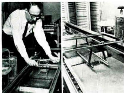
The USWA is an ultrasonically energized wave applicator which allows a straight-line ultrasonic process. The elevated standing wave is 12 in. wide x 12 in. long and is raised  $\frac{3}{4}$  in. above the tank surface. The unit may be used for pickling, bleaching, washing, burnishing and tanning processes. Electrovert Inc., 240 Madison Ave., New York 16, N. Y. BOOTH 4009.
