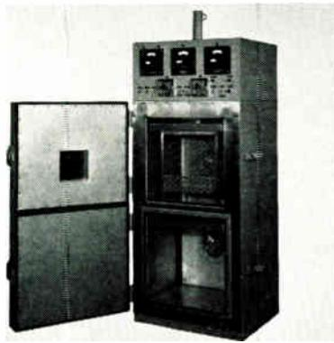
This compact environmental chamber performs the thermal shock portions of Mil-202B, Methods 102A and 107A. It performs between  $-100^\circ\text{F}$  to  $+300^\circ\text{F}$  range. The unit can also be supplied for operating in a range of  $-300^\circ\text{F}$  to  $+1000^\circ\text{F}$ . Operation is completely automatic with cycling timers for each test phase. Interior of the chamber is 16-gauge stainless steel with 16-gauge galvanized exterior. Conrad, Inc., Holland, Mich. BOOTH 1310.
