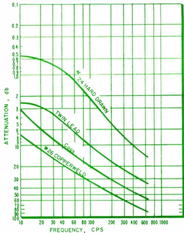
Fig. 2: Attenuation vs frequency characteristics for several lines (when fully dispensed from spools) are plotted here.
