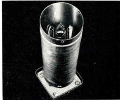
Dimensions of 1½ x 1½ x 4 in., excluding studs and header. Operating temp. is 75°C (±2°C). Stability is ±4°C over an amb. temp. range of -55°C to 65°C. Power requirements: 20w at 110vac. Reeves-Hoffman Div. of Dynamics Corp. of America, Cherry and North Streets, Carlisle, Pa.
