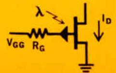
WE PUT THE EYEBALL AND THE LOW NOISE AMPLIFIER IN ONE TO-18 PACKAGE. RESULT: A DETECTIVITY —  $D^*$  — THAT WILL PLEASE STAR-GAZERS. SPECTRAL RESPONSE, HIGH-Z INPUT, AND SPEED MAKE IT IDEAL FOR READERS, COUNTERS, AND OTHER APPLICATIONS. THE THIRD LEAD LETS YOU BIAS IT FOR THRESHOLD CONTROL AND LOW D-C DRIFT. WRITE FOR FILE P-102 AND MORE APPLICATIONS IDEAS.
