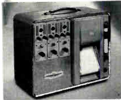
The 290 series consist of single two- and three-channel units. Plug-in amplifiers (Models 292 and 293 multiple-channel units) have a sensitivity range from 5mv-5v./chart div. Input impedance: 2.5 megohms, either side to ground. Power: 115v.  $\pm 10\%$ , 60cps, 125w. Weight: 20 lbs. (single-channel) and 40 lbs. (multiple-channels). Americal Optical Co., Instrument Div., Buffalo 15, N. Y.
