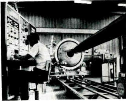
Engineer begins the test cycle of new CEBM (corona, eddy current, beta ray, microwave) Polaris A-3 motor chamber test system. The unit, built by Magnaflux, will test complex glass-epoxy structures. Microwave, beta and corona testing equipment is on end of boom. Eddy current is tested with hand-held probe.
