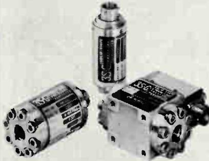
**SILICON SEMICONDUCTOR STRAIN-GAGE PRESSURE TRANSDUCERS.** All solid state • 5 V output with integral amplifier module, 250 mv without amplifier • 0.25% combined linearity and hysteresis • infinite resolution • repeatability 0.05% • operating temperature -65 to +250°F, with internal compensation • pressure ranges to 20,000 psi • internal shunt calibration • responsive to both static and high frequency dynamic pressures • 1000 G shock • 100 G sinusoidal and 8 G<sup>2</sup> random vibration.
