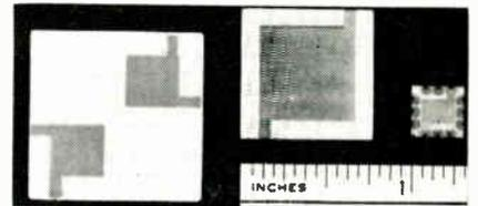
The Cerafer<sup>TM</sup> capacitor has a capacitance range up to 8000pF/single layer. It has constant capacitance and high Q into the mc range. Voltage breakdown exceeds 250vdc and temp. coefficient is less than 300ppm/°C. Rating is 75vdcw; insulation resistance exceeds 100K megohms at 50vdc. Max. capacitance change is 3% in 1000 hrs. life test @ 85°C and 75vdc continuous. Temp. -65° to +125°C. CTS Corp., Elkhart, Ind.
