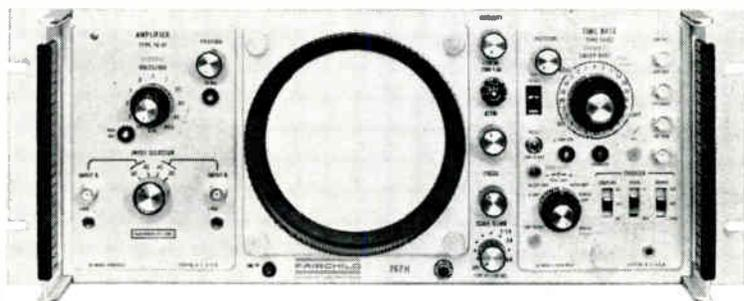
**Type 767**—Rack-mount configuration is standard 19" in width, only 7" high.
