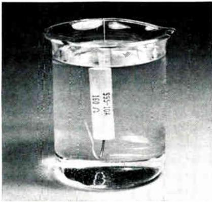
**SOAK IT IN SOLVENT!** Here's another test you can run quickly. Fill a beaker with the most active of organic solvents used in degreasing and flux removal. Drop in a Series 99 molded resistor. Let it soak. Then try to rub off the markings. They're bright as new, because they're part of the ceramic coating. Try this on any other resistor . . . the markings dissolve and can be rubbed off.
