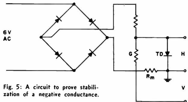
Fig. 5: A circuit to prove stabilization of a negative conductance.
