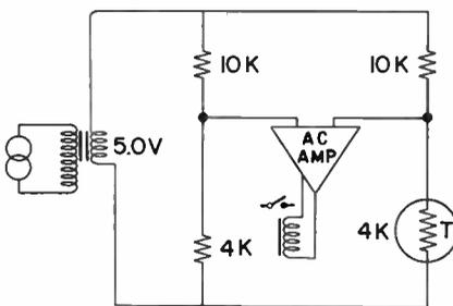
Fig. 3. Typical thermistor temperature control circuit
