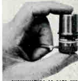
**SUBMINIATURE AC RATE GYROS.** Only  $\frac{1}{8}$ " in diameter by  $1\frac{1}{8}$ " long in its smallest size. Maximum ranges from  $\pm 5^\circ$ /sec. to  $\pm 5000^\circ$ /sec. Threshold rates as low as 0.01 $^\circ$ /sec. for ranges up to 200 $^\circ$ /sec. 0.05% of full scale for higher ranges. Withstand 150 G shock, 8 millisecond duration along any axis standard. Self test is available.
