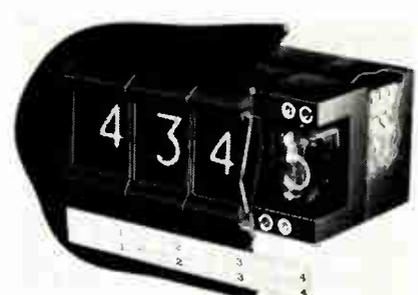
The Tec-Lite TNR-30 series is available in 8 models to handle 8-wire or 4-wire B.C.D. input in 1, 2, 4, 8 code. Supply voltage of +180vdc ( $\pm 10$ vdc) @ 2 to 6ma. is confined to the panel area. Elements of the rectangular neon readout tube are controlled by internal all-transistor decoder components. Numerals are 0.610 high. Life expectancy is 100,000 to 200,000 hrs. Transistor Electronics Corp., P. O. Box 6191, Minneapolis 24, Minn.
