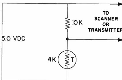
Fig. 2. Typical thermistor telemetry circuit
