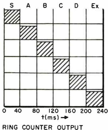
Fig. 4: Timing program. Information pulses during the time intervals A, B, C, and D are sensed by AND gates that use counter and inspection pulses generated by the command word.
