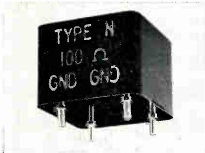
The Series N nsec. lumped constant delay lines are constructed using mica capacitors and iron toroids. Size is  $\frac{5}{8}$  x  $\frac{3}{8}$  x 0.450 in. and it may be mounted on printed-circuit boards. Attenuation is 2% max.; temp. coefficient is 50 parts/million/°C. DC working is 300v.; time delay to rise time ratio is 3.5/1 for 1 unit. Allen Avionics, Inc., 255 E. 2nd St., Mineola, N. Y.
