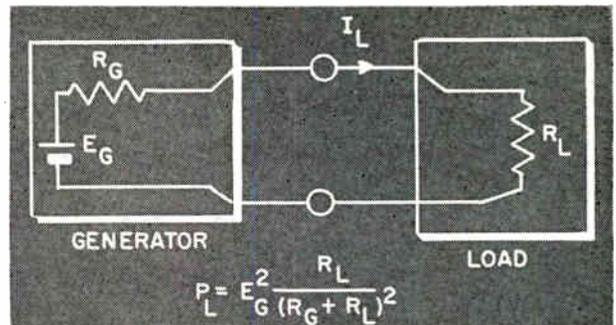
Fig. 11: Matching for maximum power transfer is illustrated.
