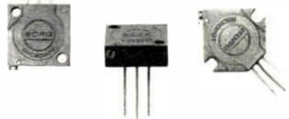
These 3/8 and 1/2 in. sq. wirewound trimming potentiometers are humidity-proof, dust proof, and shock-proof to 100g. They operate from -65°C to +175°C. The 1/2 in. model meets all requirements of MIL-R-27208A, Style RT-22. Resistance ranges for 1/2 in. is 10 to 100KΩ (±5%) and 10 to 50KΩ (±5%) for the 3/8 in. trimmer. Power rating is 1w. at 70°C for 1/2 in., and the 3/8 in. is 1w. at 50°C. Borg Equipment Div., Amphenol-Borg Electronics Corp., Janesville, Wis.
