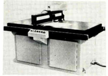
By optically scanning a pencil-line tool path layout drawing, practically any shape that can be drawn with standard drafting instruments can be produced in metal in 2 dimensions (X & Y) with this Master-line Tracer system and method. It is provided with a large vertical special mill equipped with 2 zero-backlash ball-bearing table movement lead screws. Any 2 dimensional contour can be machined to a high degree of accuracy. Andrew Engineering Co., Minneapolis 26, Minn.
