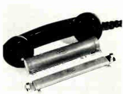
This full-line of silicone-coated HL resistors meet the electrical, environmental and dimensional needs of Mil-R-26C and are interchangeable with the major types of vitreous enamel resistors. Offered are 13 tubular models, ranging in size from 5 to 210w. and 5 flat models ranging in size from 21 to 91w. Resistance capabilities range from 0.1 $\Omega$  to 1.5 megohms ( $\pm 5\%$ ). Tolerances from 0.05% to 10% are available. Dale Electronics, Inc., P. O. Box 488, Columbus, Nebr.
