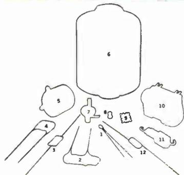
1. 3 V, 0.02 mf ULTRA-KAP<sup>®</sup> micro-miniature capacitor for transistor circuits. Other sizes available in voltages to 20 VDC, capacities to 2.2 mf.
