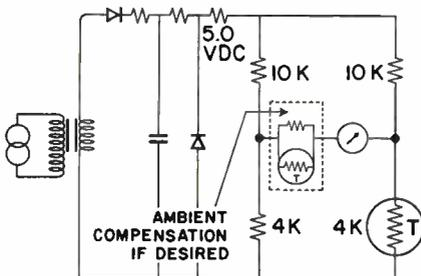
Fig. 1. Typical thermistor temperature indication circuit
