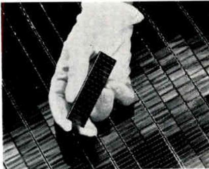
These silicon solar cell panels are capable of optimum operation in environments encountered in space satellites. They incorporate gridded N-on-P or P-on-N cells and use printed circuits to assure optimum conduction from all cells. Flat-mounting replaces shingling of solar cells, making for more rugged panels. International Rectifier Corp., 233 Kansas St., El Segundo, Calif.
