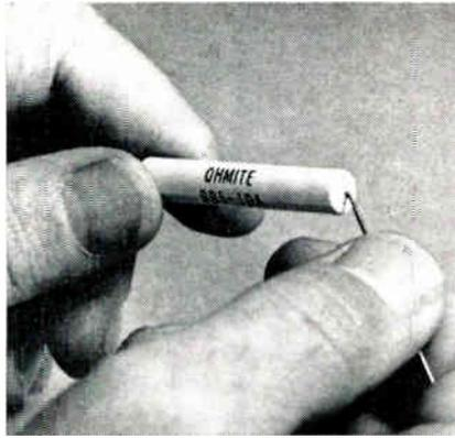
**BEND THE LEAD** where it emerges from the resistor body! You can bend the lead repeatedly at this point without damage. Conventional axial-lead, vitreous-enamelled resistors have a dipped coating which forms a meniscus around the lead where it joins the body of the resistor. Bending the lead ruptures the meniscus and damages the coating. Series 99 resistors are molded and there is no meniscus.
