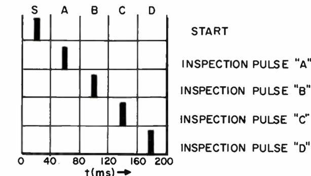
INSPECTION PULSE GENERATOR OUTPUT (ASSUMING 200ms SIGNAL)
