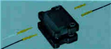
(2) The Tier Block Pin and Socket Connector consists of 10-position male and female blocks that unite firmly without hardware accessories. Normally, blocks are made of general-purpose phenolic, but are available on order in diallyl phthalate. When stacked, male members are locked into position with #10 screws.
