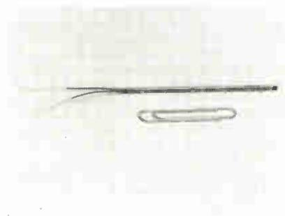
Probe Type SBV-555 has an outer dia. of 0.10 in. which permits magnetic field measurements within small deep bores. They use the basic Hall-effect principle to permit sensing of the magnitude, polarity and direction of magnetic fields. Instrument Systems Corp., 111 Cantiague Rd., Westbury, L. I., N. Y.
