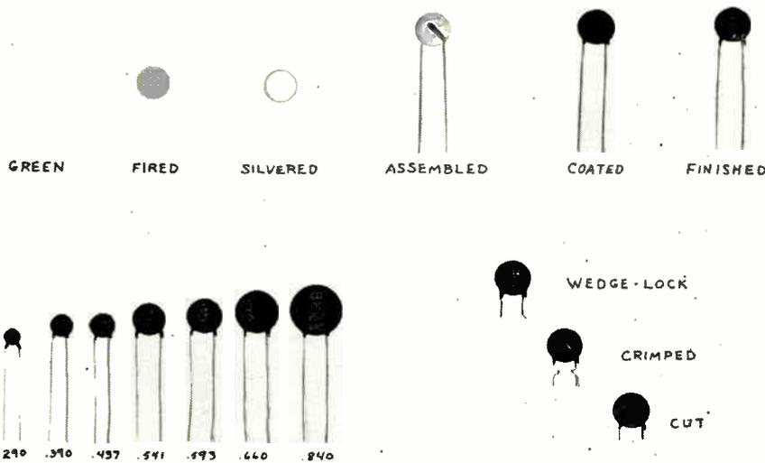
Fig. 2: Typical ceramic capacitor construction. The raw green ceramic piece is made. Then it is fired, silvered, soldered and coated. Available are various lead.
