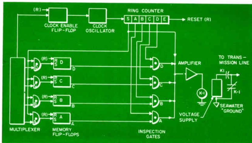
Fig. 7: Command Encoder. A command is generated by manually selecting the desired command on a multiplexer. Approximate volume of the encoder is 25 cubic inches.
