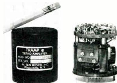
Model 1801-3800 is an 8 1/4 cu. in. servo amplifier which produces 40w. output. Voltage gain is variable from 1 to 1000 through an external resistor in series with the input, and gain stability is ±1/2db over the full temp. range. Output voltage is 36v. rms. M. Ten Bosch, Inc., Pleasantville, N. Y.
