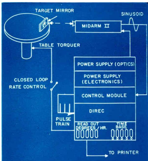
system have less chance to exert their influence as major causes of gyro error. This is important since the rate errors caused by table perturbations show up as drift errors in the output of the gyro. At the same time, genuine drift errors in gyro performance are caused by gyro bearing inequities, pickup drag, air bearing turbine effects, dynamic unbalance, etc. Since both the gyro drift error and the table perturbations occur at the same time they appear as gyro drift errors.
