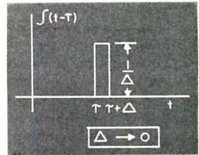
Fig. 14: Graphic representation of unit impulse.
