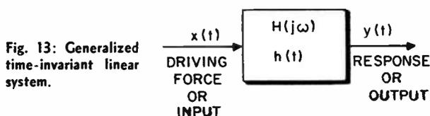
Fig. 13: Generalized time-invariant linear system.
