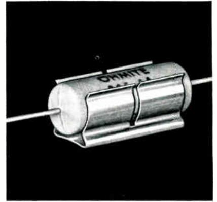
**CLIP IT!** Insert a molded Series 99 resistor into a metal clip. Don't baby it; ram it in. There's no danger of cutting, chipping, or scratching the hard coating which provides 1000 VAC insulation. Notice the snug fit, too. The clip mounting shown is resistant to high shock and vibration. When mounted on a metal chassis, it provides a heat sink which may increase the wattage rating as much as 100%.
