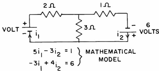
Fig. 9: Simple circuit problem with the mathematical model.
