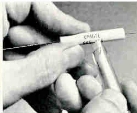
**TORCH IT!** Withstands temperatures of 1500°F without a sign of deformation. No other vitreous-enameled resistor will stand 1500°F without burning, softening, or dripping away. There's absolutely no effect on markings either . . . they are vitreous in nature . . . a ceramic marking fired right into the coating. Markings on all other resistors burn off immediately, or rapidly become illegible.
