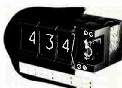
The Tec-Lite TNR-30 series is available in 8 models to handle 8-wire or 4-wire B.C.D. input in 1, 2, 4, 8 code. Supply voltage of +180vdc ( $\pm 10$ vdc) @ 2 to 6ma. is confined to the panel area. Elements of the rectangular neon readout tube are controlled by internal all-transistor decoder components. Numerals are 0.610 high. Life expectancy is 100,000 to 200,000 hrs. Transistor Electronics Corp., P. O. Box 6191, Minneapolis 24, Minn.
