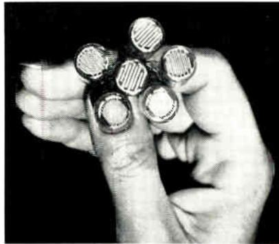
This epitaxial-planer component is a 0.25 in. sq. single-chip microcircuit which effectively replaces 4 diodes, a transistor, and a resistor. The epitaxial NAND gate consists of a 3-input AND gate followed by an inverting stage. The package is a modified TO-5, but other configurations are available. Sylvania Electric Products Inc., 100 Sylvan Rd., Woburn, Mass.
