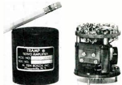
Model 1801-3800 is an 8 1/4 cu. in. servo amplifier which produces 40w. output. Voltage gain is variable from 1 to 1000 through an external resistor in series with the input, and gain stability is  $\pm 1/2$ db over the full temp. range. Output voltage is 36v. rms. M. Ten Bosch, Inc., Pleasantville, N. Y.
