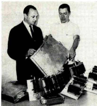
F. H. Guterman (l), Pres., ITT Industrial Products, and R. Hansen, project engineer, examine package of radiation-resistant voltage regulator. It is for AEC's SNAP program (Systems for Nuclear Auxiliary Power), which is to develop power systems for satellite and interplanetary craft.
