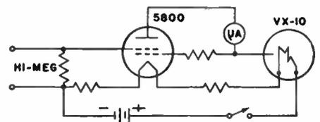
Victoreen has produced two Thermal Time Delay Relays to prevent this destabilization: The VX-10 and VX-69, each of which automatically provides approximately 1 second delay in the application of plate voltages.
