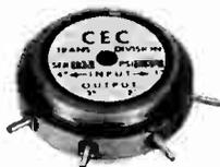
Type 4-325, "small size": Pressure range: 0-10 to 0-100 psia, 0-2 to 0-100 psig,  $\pm 2$  to  $\pm 50$  psi bd. Temperature range:  $-65^{\circ}$  to  $+250^{\circ}$ F.
