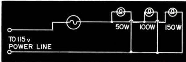
Fig. 1: Elementary circuit theory and mathematics may be used to determine the smallest size fuse that can be used here.
