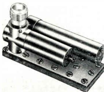
Type 9189, part No. 9189-1000, is an X-band CW microwave oscillator and doubler used as a local oscillator for beacons, altimeters and system ground check-out equipment. Power input requirement 140v. @ 20ma, 6.3v. @ 290ma. The unit weighs 4 oz. and is 2½ x 1 x 1¼ in. It can be modified to other freqs. Trak Microwave Corp., Tampa, Fla.
