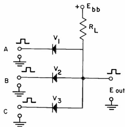
The B leg should be corrected as shown so that the circuit will function as originally intended.
