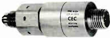
Type 4-326, "universal": Pressure range: 0-10 to 0-10,000 psia, psig. Temperature range:  $-65^{\circ}$  to  $+250^{\circ}$ F.
