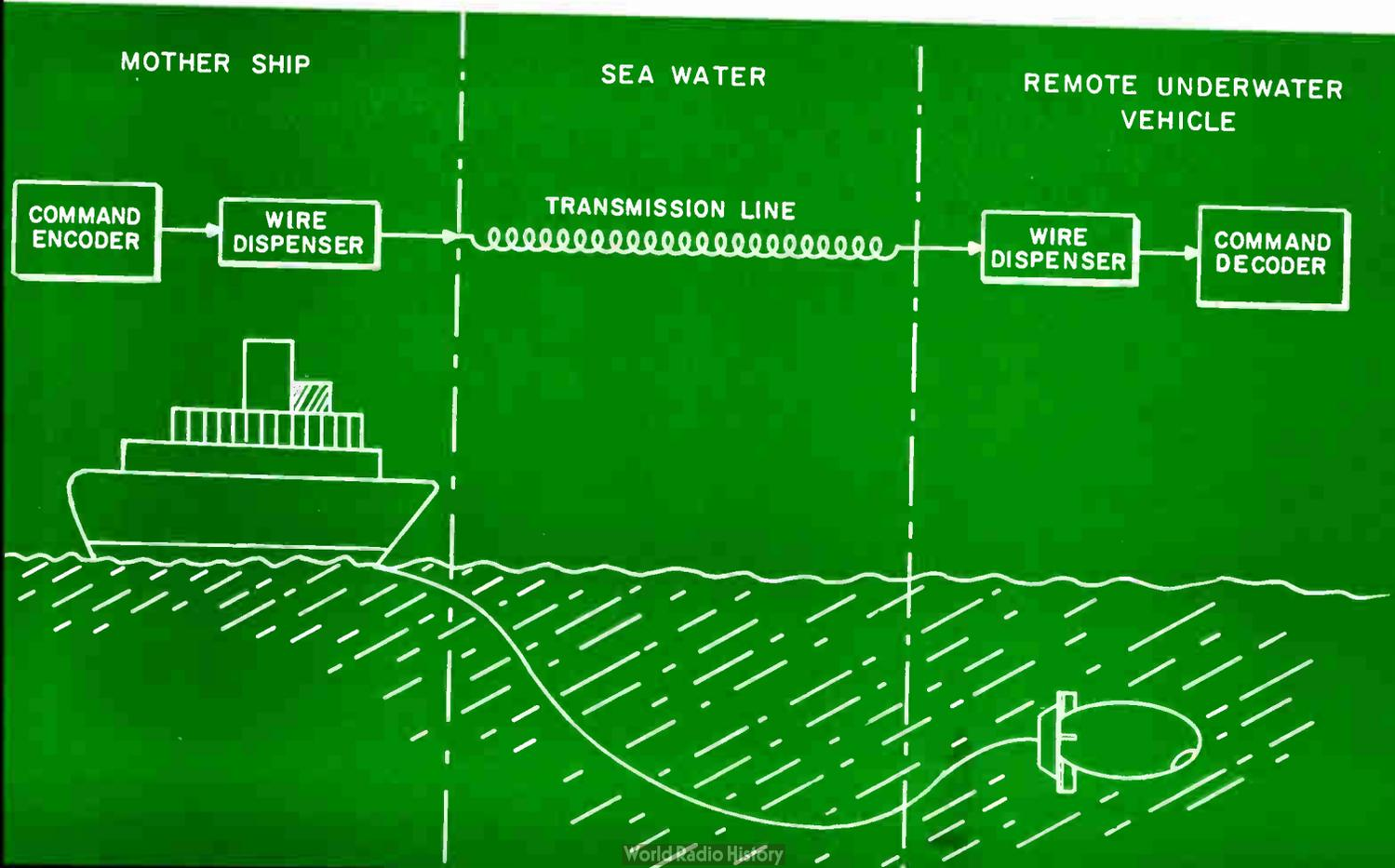
conductor, so that the line is essentially a coaxial cable, with an insulated inner conductor of wire and an outer one consisting of the sea.
