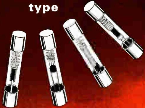
"Slow blowing" fuses for circuits where harmless surges occur. These fuses prevent needless outages by safely holding starting currents or surges, — yet they provide safe, positive protection against short-circuits or continued overloads.
