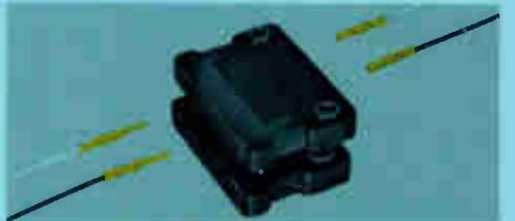
(2) The Tier Block Pin and Socket Connector consists of 10-position male and female blocks that unite firmly without hardware accessories. Normally, blocks are made of general-purpose phenolic, but are available on order in diallyl phthalate. When stacked, male members are locked into position with #10 screws.
