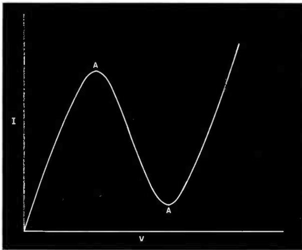
Fig. 1: Curve of a current-voltage relationship of a negative-conductance device
