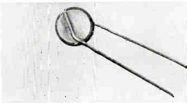
This is a capacitor that failed. The tiny black spot seen on the side of the unit shows where the dielectric broke down during the extended life test.
