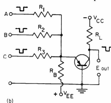
Since these circuits use a combination of resistors (for isolation), and a transistor for the AND action, they are known as *transistor-resistor logic* or *TRL circuits*.
