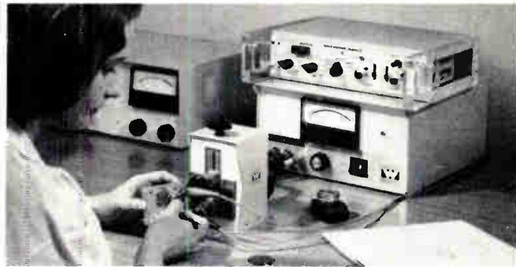
Weld Energy Computer is used as a production monitor to indicate a GO, NO-GO condition in the fabrication of Welded Electronic Modules. Units are built by Weldmatic Div./Unitek.
