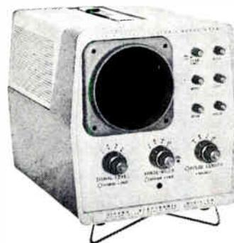
**Step 1.** Assign an operator to scan up to 30 miles of cable through a Sierra 370A Cable Fault Locator.
