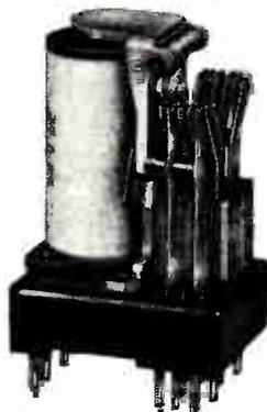
Plug the LS into the socket . . . just as you would a vacuum tube. The relay's tab terminals mate snugly with the socket, will hold the relay in place under normal conditions. When the relay is mounted horizontally, or when vibration is a problem, two banana plugs or two machine screws may be used.
