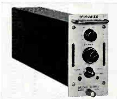
The solid-state Model 6179 bridge supply is a full-floating, triple-shielded, regulated power supply. It has a bridge-balance switch that permits monitoring by external bus of bridge voltage or bridge balance. The unit permits use of 3, 4, 6, or 7 wire connected systems. It supplies 0 to 200ma dc. Dynamics Instrumentation Co., 583 Monterey Pass Rd., Monterey Park, Calif.
