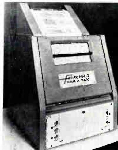
First completely transistorized facsimile transmitting system. The Fairchild Scan-A-Fax uses printed circuitry throughout. The Scan-A-Fax unit (above) accepts all types of copy and visual matter. It has ability to automatically run up received copy to display easel for immediate removal. This feature eliminates four to five minute wait for copy to come from the recorder unit at recording speed.
