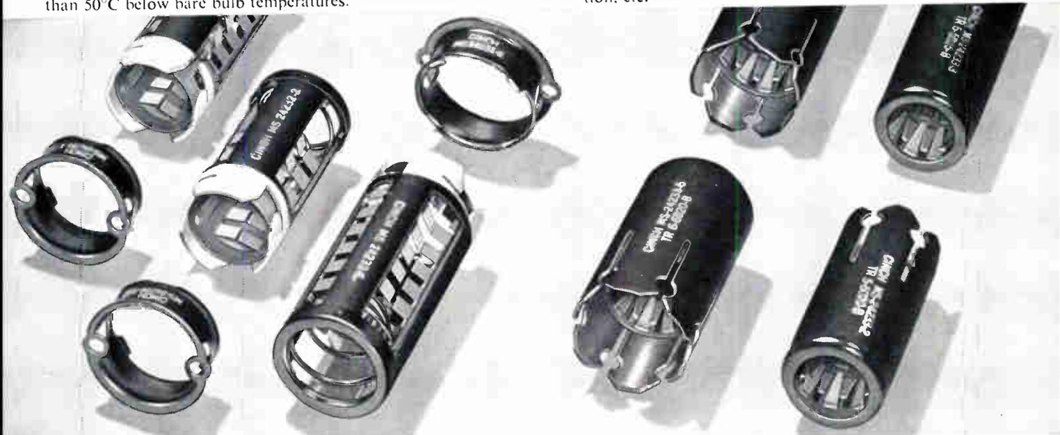
**MILITARY TYPE "B"**—Cinch T5 and T6 Series are designed for new equipment applications. Each shield locks into a flanged base that mounts to the chassis through the tube socket mounting holes. Cinch T5 and T6 Series meet or exceed all physical and environmental specifications of MIL-S-9372C and SCL-6307.2, including for vibration (15 g, 10-2000 cps), heat resistance (200°C), heat dissipation (required 20°C actual 50°C at sea level and 50,000 ft.) and salt spray (50 hour).
