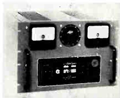
Model KN20 is designed for 208vac, 60 cycle, 3-phase input. The dc output is isolated from the ac line and ground. The unit features a solid-state phase-failure sensor which turns off the power supply if one or more of the 3 input phases opens. It also prevents the supply from starting if the ac source has an open phase. Opad Electric Co., 43 Walker St., New York 13, N. Y.
