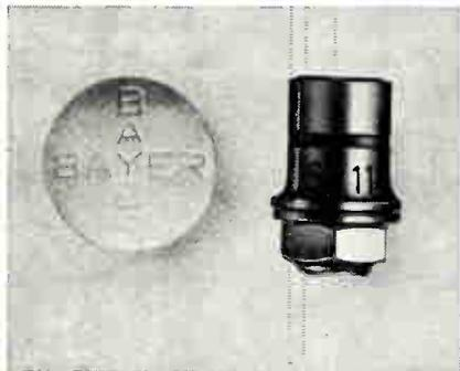
The SG 11054 is a glass dielectric piston-trimmer capacitor. It is 1/4 in. in dia. It has a temp. coefficient of  $0 \pm 50$  PPM/°C; dielectric strength of 1 kvdc at 50% relative humidity and max. rated capacitance; working voltage is 500vdc. Approx. Q: 1000 @ 1mc; 500 @ 50mc; 400 @ 100mc; 350 @ 500mc; etc. Roanwell Corp., 180 Varick St., New York, N. Y.
