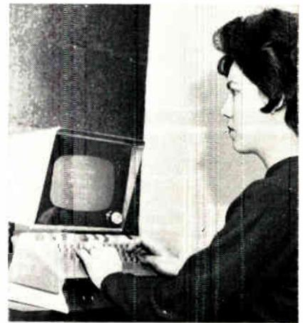
A video typewriter which communicates with high-speed computer systems at rate of 240 characters per second has been demonstrated by The Teleregister Corp. The new electronic input/inquiry device resembles a combination electric typewriter and small TV screen and makes typographical corrections by means of a unique electronic eraser. The unit displays numbers, letters and symbols.
