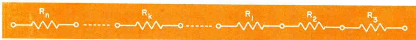
Fig. 1: Central to the Ratiometric method is the string of resistors in series. String is one of the NBS-certifiable standards in the method. In the Julie Standard, resistors have an accuracy of 0.0015% and intercomparison among them permits establishment of ratios of better than 0.00001% accuracy.
