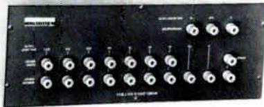
Model 2851 is a 17 lb. instrument for rack mounting or bench use. It has separate working and guard circuits. Input working taps are 3, 7.5, 15, 30, 75, 150, 300, 750 and 1500v.; input guard taps are 15v. and above. Guaranteed error limit for the volt box is  $\pm 0.005\%$ . Calibrated accuracy is  $\pm 0.002\%$ . The instrument is thermally and electrostatically shielded. Honeywell, Denver Div., 4800 E. Dry Creek Rd., Denver, Colo.
