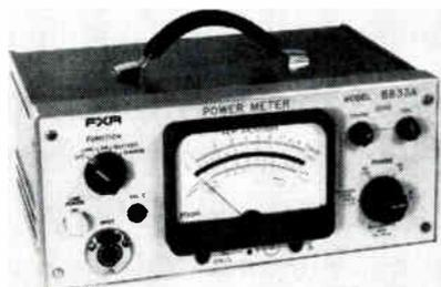
Model B833A uses a dc self-balancing r-f bridge for accuracies of 0.15% @ 10mw or 1.5% @ 1mw. The unit eliminates subtle errors associated with audio power in r-f bridges. Features include: a single zero adjustment; availability of thermistor heads at freqs. from 10mc to 40cc. It is lightweight and portable with optional rechargeable battery. FXR, 25-15 50th St., Woodside, N. Y.
