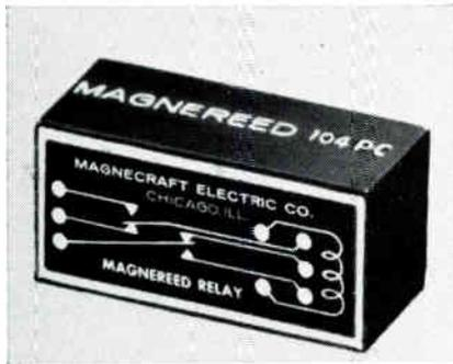
The class 104 encapsulated dry-reed assemblies have preadjusted gold contacts hermetically sealed in inert gas. The spdt units operate in 1msec. and release in 1msec. Contacts are rated 3va @ 0.25a. Life is 10 million cycles. Magneecraft Electric Co., 5575 N. Lynch, Chicago, Ill.
