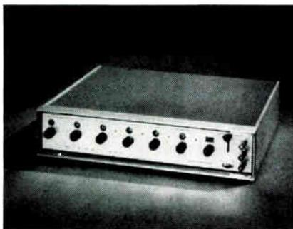
The Vidar 820 digital oscillator with calibrated amplitude control eliminates electronic counter and RMS voltmeter for uses requiring an accurate, calibrated freq. source. It has a 4-digit freq. settable to 0.005%. Amplitude control combines a step attenuator and calibrated vernier, providing  $\pm 1\%$  output voltages over the range of 1mv to 10v. Vidar Corp., 77 Ortega Ave., Mountain View, Calif.
