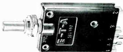
Series 46-400 miniature circuit breaker has 2 auxiliary contacts—NO and NC. The auxiliary contacts can give an indication by light or buzzer, or they can be used to connect or disconnect other components such as relays, solenoids, etc., when the breaker is in the on or off position. Size: 2 x 0.5 x 1.2. E-T-A Products Co. of America, 6284 N. Cicero Ave., Chicago, Ill.
