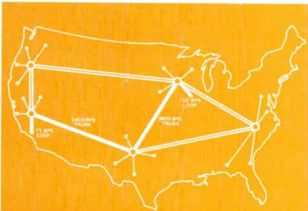
Fig. 1: With message switching, high-speed trunks between switching centers can be used, even where circuits to and from the terminals operate at much slower speeds.
