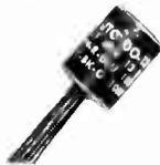
Electrostatically & magnetically shielded output transformer  $\frac{1}{4}$  D. x  $\frac{1}{4}$ " H. Pri. 15K C.T. Sec. 8K C.T.; max. level 50 mw; audio range response. To MIL-T-27B, grade 4.
