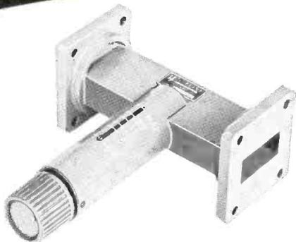
Waveline has developed a series of Power Set Attenuators to provide well shielded, efficient, variable attenuation over a frequency range of 2.6 to 18.0 Gc in six standard models. These variable Power Set Attenuators provide a variable attenuation of from 0.5 to 20.0 db over the full waveguide frequency range with an indication of the approximate attenuation value.
