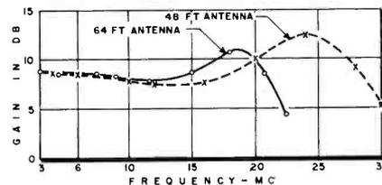
Fig. 3a: Revised h-f Antenna power gain.
