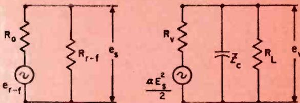
Fig. 5: The circuit in Fig. 4 can be further broken down into equivalent r-f and video circuits as shown here.
