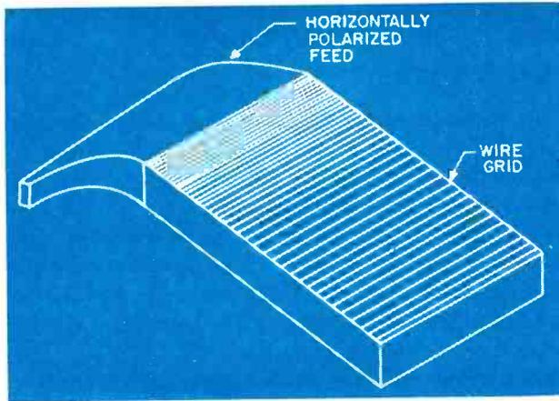
Fig. 1: The inductive-grid leaky-wave antenna consists of parallel wires supported above a metallic plate as shown.
