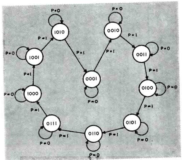
Fig. 11: State diagram shows the first three columns in Table 5.
