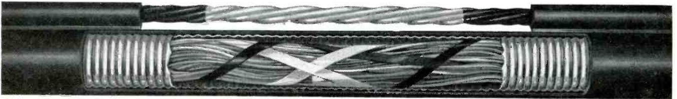
ABOVE: Drawing of new self-supporting cable structure shows "undulated" core of telephone wires encased in aluminum and polyethylene sheath members. Edges of corrugated aluminum sheath are butted along top of cable. Polyethylene sheath extends over steel strand on top to provide built-in cable support. BELOW: Photographs show, left to right, older-type ring-supported cable, present lashed cable, and new self-supporting cable.
