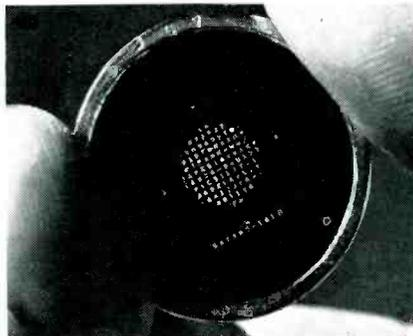
This display uses a Charatron® tube to translate computer codes into understandable data on its face. A newly developed matrix, the key to the Charatron, presents both upper and lower case letters, plus a variety of symbols and Greek letters. The tube also has a spot writing capability, producing a 0.008-in. spot at 4 $\mu$ a. Character size is variable at a ratio of 5-to-1. Stromberg-Carlson, div. of General Dynamics, P. O. Box 127, San Diego 12, Calif.
