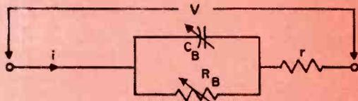
Fig. 3: Low frequency equivalent circuit for the detector diode.
