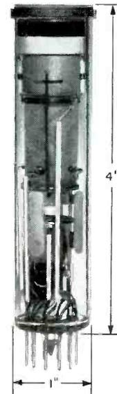
General Electric's new type Z-7845 vidicon tube combines the high resolution performance of all-magnetic vidicons with compact size and light weight.
