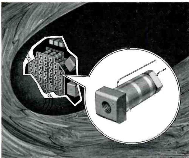
ADVANCED TRANSDUCERS FOR ASW VEHICLES are being developed and produced by Honeywell. The multi-element array shown is a highly directional transducer designed for use in a sonar projector-receiver system.
