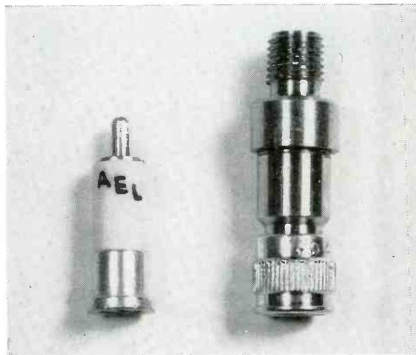
Fig. 8: Miniature integrated mount compared to standard diode.
