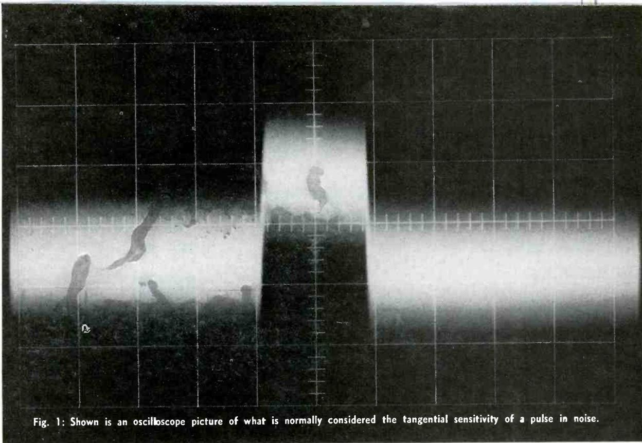
Fig. 1: Shown is an oscilloscope picture of what is normally considered the tangential sensitivity of a pulse in noise.
