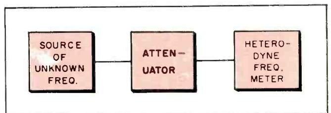
Fig. 6: Measurement of frequency of an active source using a heterodyne frequency meter.
