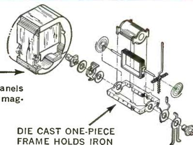
DIE CAST ONE-PIECE FRAME HOLDS IRON CORE IN EXACT ALIGNMENT
