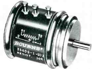
The new Model 3560 is a  $\frac{7}{8}$ -in. dia., 3-turn servo-mount potentiometer. It combines high performance with outstanding resistance to humidity. A Silverweld® termination — a virtually indestructible fused bond between the terminal and resistance wire—eliminates the chief cause of precision potentiometer failure. The unit is rated at 1.5w. @ 70°C. Bourns, Inc., 1200 Columbia Ave., Riverside, Calif.
