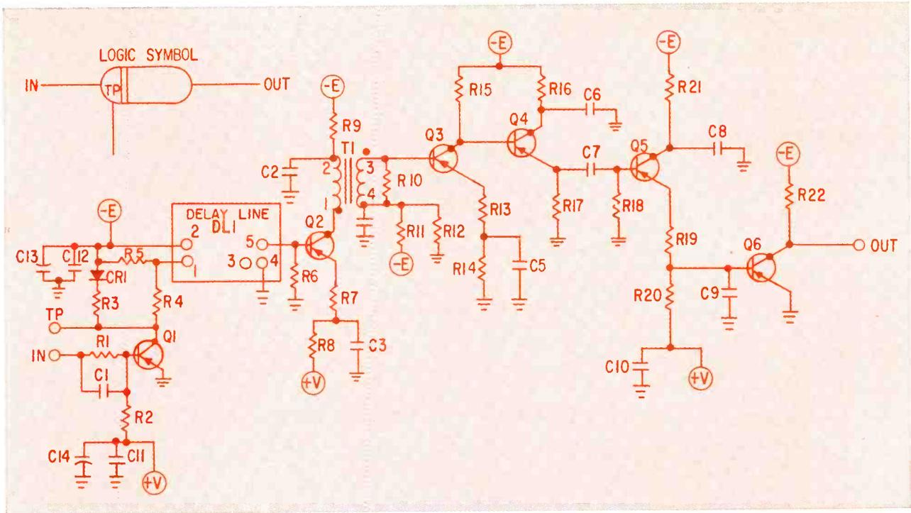
Fig. 1: Delay line circuit diagram and logic symbol.
