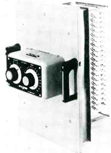
The major feature of the Model 2603 Test Tray is its good electrical and mechanical characteristics over a  $-200^{\circ}\text{F}$  to  $+400^{\circ}\text{F}$  temp. range. It holds 80 axial-lead electronic components for simultaneous electrical and temp. tests. It fits chambers having a test area opening 7-in. high x 16-in. wide. Max. test voltage is 1500v. rms; max. current, 10a. dc. Delta Design, Inc., P. O. Box 728, Del Mar, Calif.
