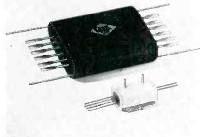
Designed to be more compatible with advanced packaging than round shapes, the new Flat-Pac coils are available with 3, 4, 5 or 6 Form A or Form C reeds (or various combinations with Form B). They are ideal for encapsulation or direct tie-down to a PC board or chassis. Length of coil is 2-in.; thickness, 3/4 in.; and width varies from 1 1/8-in. (with 3 reeds) to 1 3/4-in. (with 6). Available from stock 12, 24, 32, 48 or 110vdc. Coto-Coil Co., 61 Pavilion Ave., Providence, R. I.
