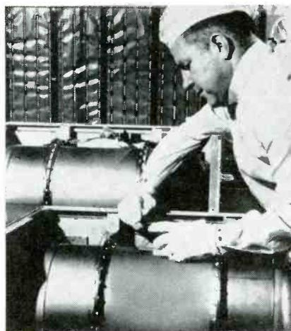
Communications, controls and other equipment in Gemini spacecraft will be powered by this fuel-cell system, which contains two batteries, each containing nearly 100 individual fuel cells in three separate stacks. Two batteries, shown in shipping containers before delivery by General Electric Co., will produce up to 2,000w of power.
