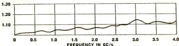
VSWR characteristics of a typical cable assembly with ½ inch Alumifoam cable and a pair of TIMATCH Type N connectors.
