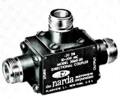
Model 3060-20 has a coupling value of 20db within  $\pm 0.3$ db of nominal value over the 20:1 band. Calibration indications to  $\pm 0.2$ db accuracy at 6 freqs.: 10, 30, 60, 100, 150 and 200mc. The unit's vswr is low, but 1.2 max. over the full octave freq. range. Typical insertion loss for basic input/output is 1.5db; max. is 2.1db. Power ratings are 1w average, and 100w. peak. Narda Microwave Corp., Plainview, L. I., N. Y.
