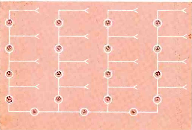
Fig. 5: Eight element multiple beam antenna uses hybrid couplers and fixed phase shifters for isolation and distribution.
