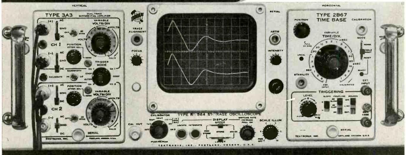
■ presents stored or conventional displays—The Type RM564 presents full-screen stored displays or full-screen conventional displays. Or—with the unique split-screen—stored displays can be presented on either the upper or lower half of the crt with conventional displays on the other half.
