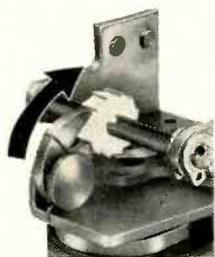
Contact action, except in the case of auxiliary contacts, takes place during the drop-out of the armature. The motive power is the armature's return spring, a constant force providing
