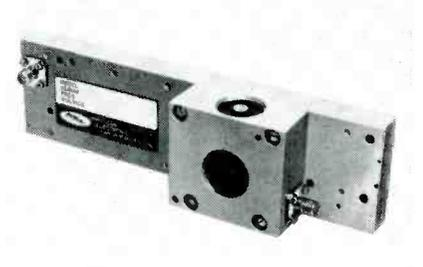
The AEL model MT829A freq. multiplier has a circulator built into the input circuit network to maintain an input vswr of less than 1.5:1. A circulator has been integrated into the output network to provide isolation between mismatched loads in the freq. multiplier. By a careful selection of varactors, conversion efficiencies of 7db are obtainable. Nominal conversion with standard varactors is approx. 9 to 10db. American Electronic Laboratories, Inc., Richardson Rd., Colmar, Pa.
