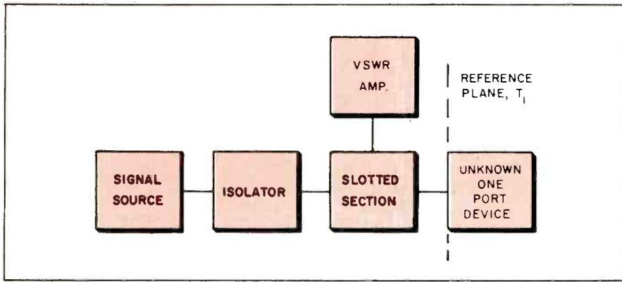
Fig. 4: Setup for measurement of VSWR and Impedance (over the range of 2-10 GC) of a one port device using a slotted section.
