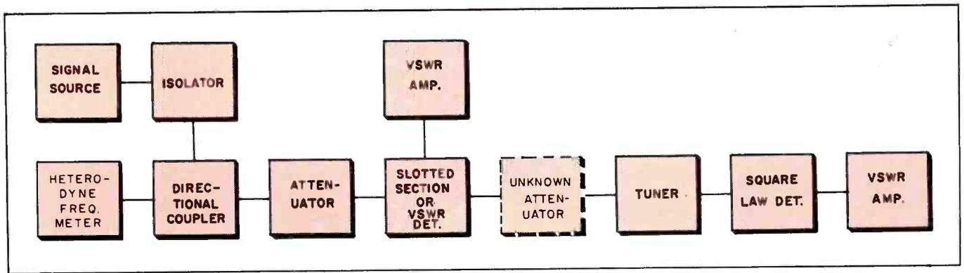
Fig. 1: Voltmeter-bolometer or direct method of calibrating attenuators is simple, fast and accurate over a range of about 40 db.
