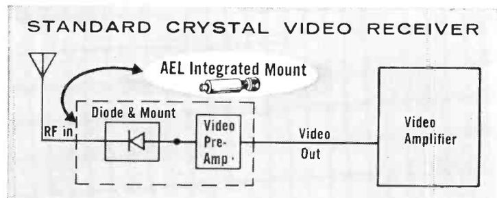
Also available is the triple combination of a miniature bandpass filter and detector-preamplifier in an integrated package, which eliminates the conventional bulky components used in present crystal video systems.
