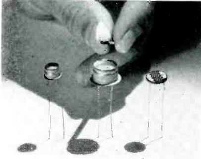
Response time for this new line is approx. 1000-to-1 change in resistance in 10msec. when 25 ft. candles are applied to cells previously held in the dark. The units act as either light-controlled rheostats or relays without contact surfaces. The 1/2-in. type Y-1206 are rated @ 250v. with 250mw dissipation. The 3/8-in. units, type Y-1332, are rated at either 30 or 60v., depending on the max. pattern width. General Electric Co., Tube Dept., Owensboro, Ky.
