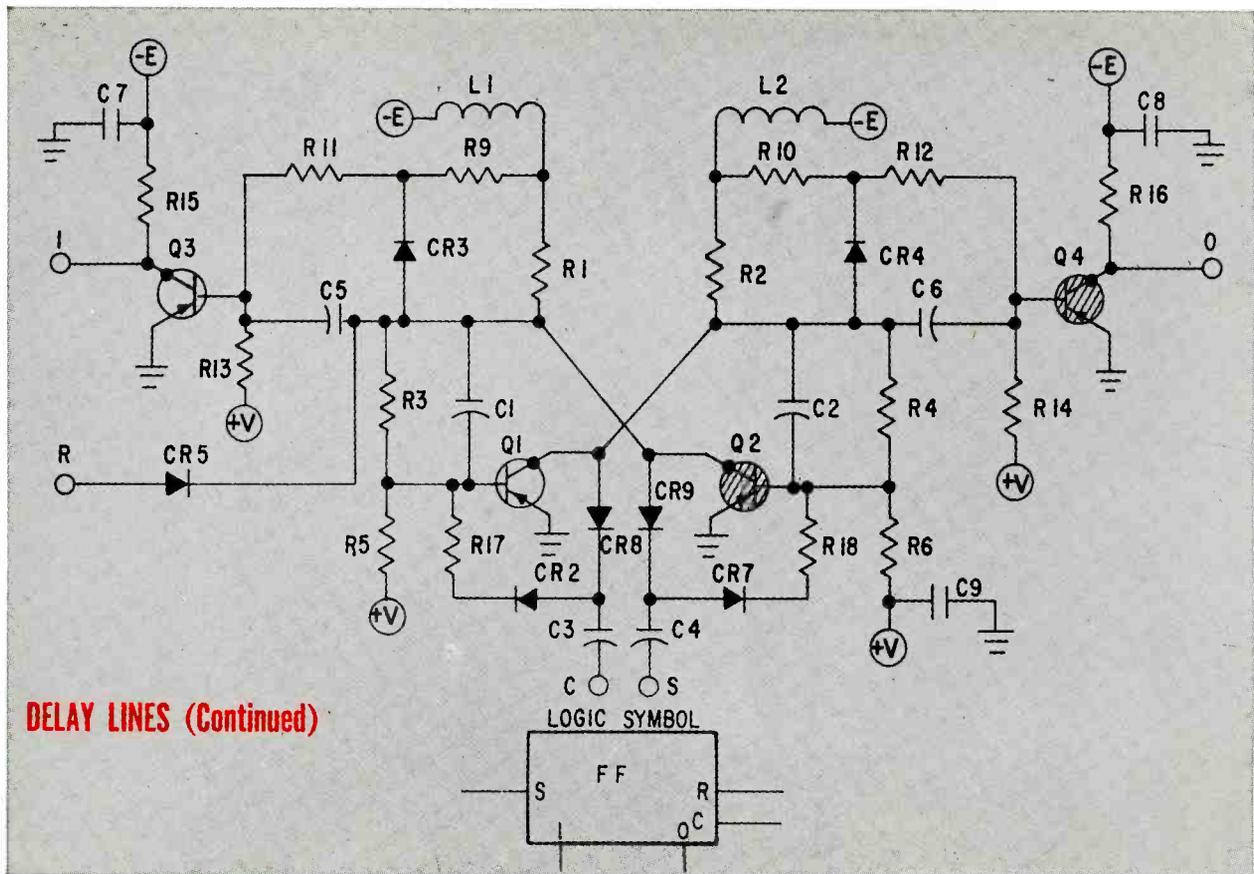
Fig. 2: High power, high speed flip-flop circuit diagram and logic symbol.
