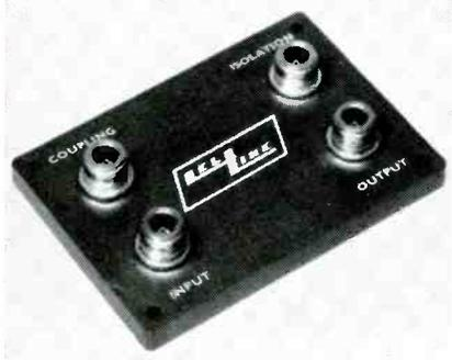
Two octave bandwidth directional couplers are available in coupling values of 6, 10, 15 or 20db. These couplers offer lightweight, small size, rugged encapsulated design with reliable performance over a broad freq. band. Special order couplers are available as narrow band (1 octave), high directivity models, or as extremely broad band (up to 4 octaves) models. LEL, Inc., 75 Akron St., Copiague, N. Y.
