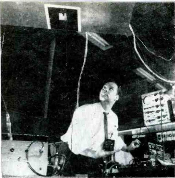
Sperry Gyroscope engineer tests low-level radar altimeter that will allow pilots to maneuver safely at low altitudes once considered impractical because of limited measuring capabilities.
