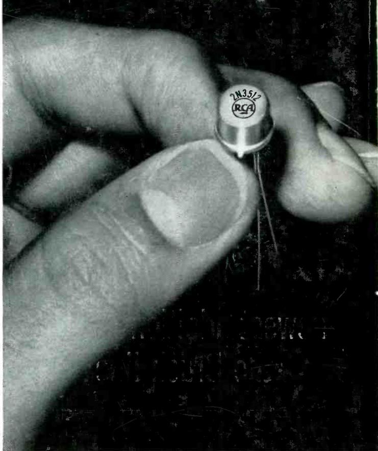
That's right! A 75% boost in collector-to-emitter voltage capability ( $BV_{CEO} = 35$  volts as compared with 20 volts for the popular 2N2476, 2N2477) makes the new RCA 2N3512 ideal for high-voltage, high-speed, high-current switching applications.
