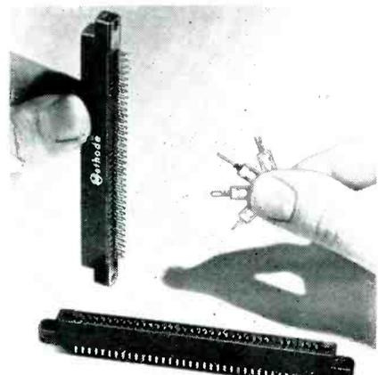
This single-side card receptacle connector, SD836 Series, provides 36 contacts on 0.100 in. centers for microminature uses such as computer circuitry and airborne instrumentation. It accommodates the 36 contacts in the same area normally accommodating only 24 contacts. Flexibility of design permits 4 styles of contacts to be used. Polarizing keys are available for pre-determined polarizing uses. Methode Electronics, Inc., 7447 W. Wilson Ave., Chicago, Ill.
