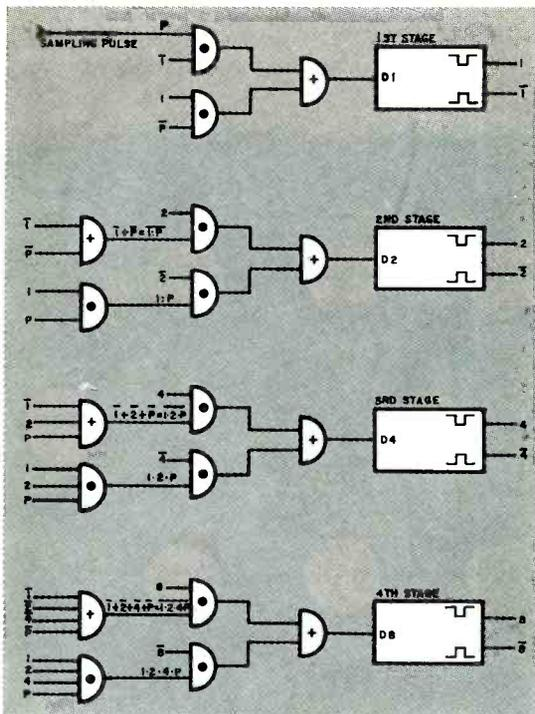
Fig. 5: Standard four-bit delay line counter.
