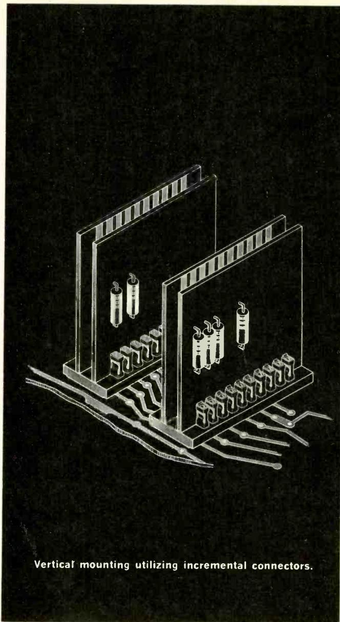
Vertical mounting utilizing incremental connectors.
