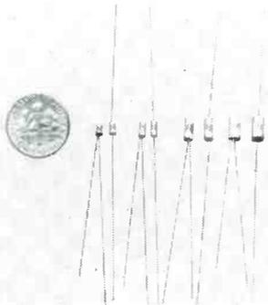
Red Top<sup>TM</sup> capacitors use plastic resin end seal instead of glass-to-metal seal. They are available in both polarized and non-polarized construction with axial-lead or single-ended terminals. The polarized types 162D and 169D have voltage ratings from 2 through 100vdc; capacitances are  $68\mu\text{f}$  to  $0.033\mu\text{f}$ . Non-polarized types 163D and 170D are rated at 2 through 100vdc and  $34\mu\text{f}$  through  $0.016\mu\text{f}$ . Sprague Electric Co., North Adams, Mass.
