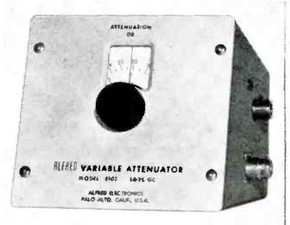
Model E 102 attenuator covers the 1.4 to 2.5gc range. It features low insertion loss, flat response, wide range, and fine resolution. Calibrated attenuation range is 0 to 60db. Freq. sensitivity is less than  $\pm 1/2$ db at min. attenuation, with external terminations possessing a vswr of less than 1.1:1. At midband, calibration is  $\pm 0.2$ db or  $\pm 2\%$ , whichever is greater. Power rating is 100w. Alfred Electronics, 3176 Porter Dr., Palo Alto, Calif.
