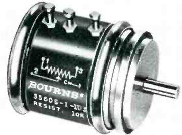
The new Model 3560 is a  $\frac{7}{8}$ -in. dia., 3-turn servo-mount potentiometer. It combines high performance with outstanding resistance to humidity. A Silverweld<sup>®</sup> termination — a virtually indestructible fused bond between the terminal and resistance wire—eliminates the chief cause of precision potentiometer failure. The unit is rated at 1.5w. @ 70°C. Bourns, Inc., 1200 Columbia Ave., Riverside, Calif.
