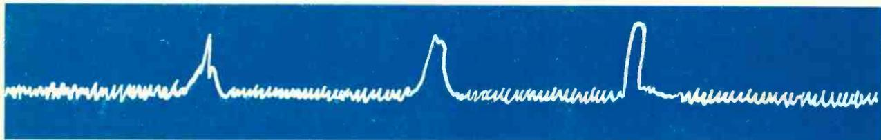
A SPECTRUM ANALYZER provides a calibrated display, usually on a CRT screen, of a rectangular-coordinate plot of signal strength versus frequency. Because all but the simplest unmodulated sinusoidal (CW) signals contain multiple-frequency elements, of differing amplitudes—in other words, a complex spectrum, rather than a single frequency—the spectrum analyzer is an informative, versatile, and accurate tool for design, test, quality control, and troubleshooting.
