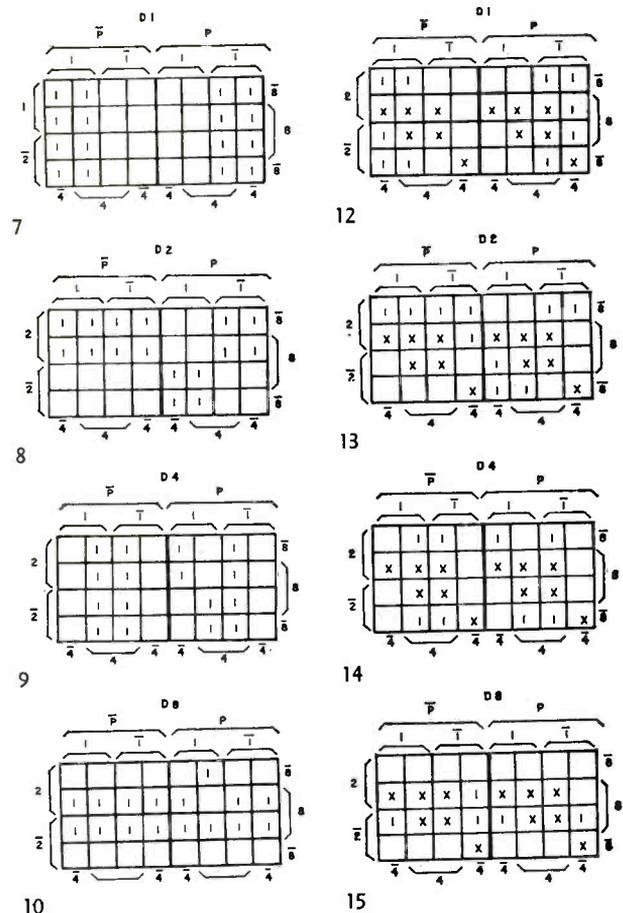
Figs. 7-10 and 12-15: These are Vietch diagrams which are used to simplify Boolean functions. They are referred to in the text.
