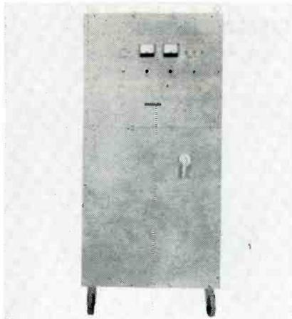
The transistorized Model M3234-1 features voltage programming, series/parallel operation; 0 to 360a. current limiting; dynamic load regulation  $\pm 2v.$  for a 200a. load change;  $-4v., +2v.$  for 300a. load change; dynamic line regulation  $\pm 0.1\%$  for a 5% line step change. Ripple is 100mV RMS max. Input voltage 208/230/460v. 3  $\phi$ , 60 cps. Perkin Electronics Corp., 345 Kansas St., El Segundo, Calif.
