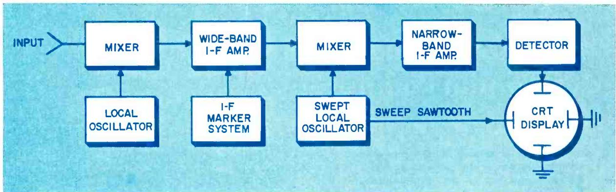
Fig. 2: Swept-IF Spectrum Analyzer Block Diagram. The incoming microwave signal is heterodyned in a crystal mixer assembly with the output of a tunable local oscillator to produce a suitable intermediate frequency, usually of the order of 160 mc. This signal is amplified in the wide-band intermediate-frequency ampli-
