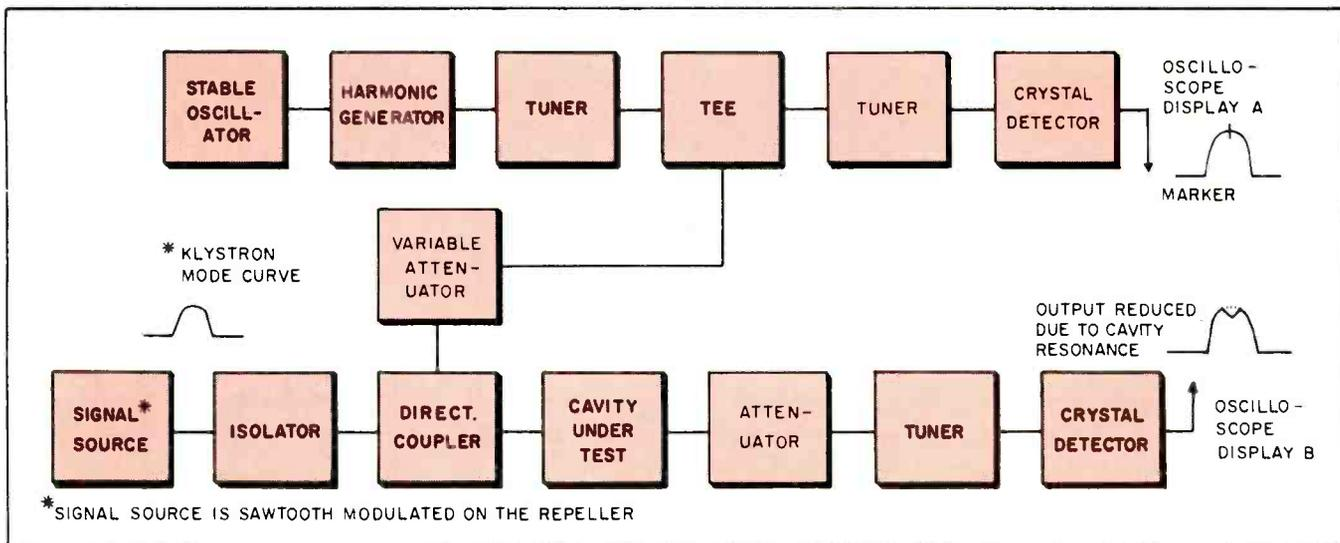
Fig. 7: Diagram for the calibration of a cavity type frequency meter is shown above.
