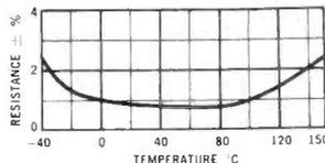
30K Thermistor No. 44008 matches standard curves to these resistance tolerances.
