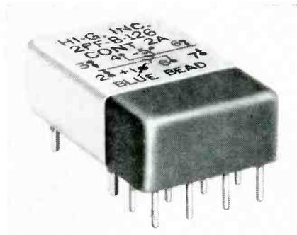
The Side-Step® series are offered in three sensitivities and designed for PC board uses. All three meet the requirements of Mil-R-5757D. The dimensions are: 0.400 x 0.800 x 1.255 in. max. The relays operate without chatter while undergoing shocks as high as 50g and vibrational forces of up to 20g. Hi-G Inc., Spring St. & Route 75, Windsor Locks, Conn.
