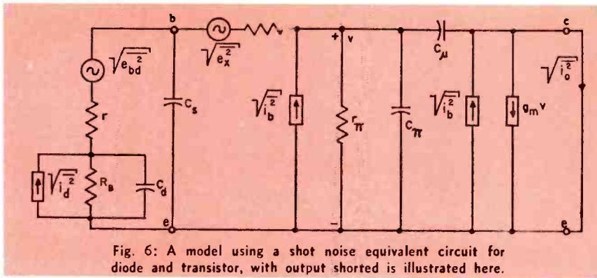
Fig. 6: A model using a shot noise equivalent circuit for diode and transistor, with output shorted is illustrated here.
