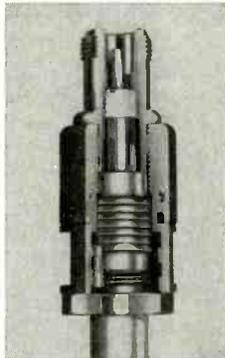
Exclusive COILGRIP Clamp consists of stainless steel coil which is torqued by a torsion collar, thus locking the coil on the collar and locking cable in position.
