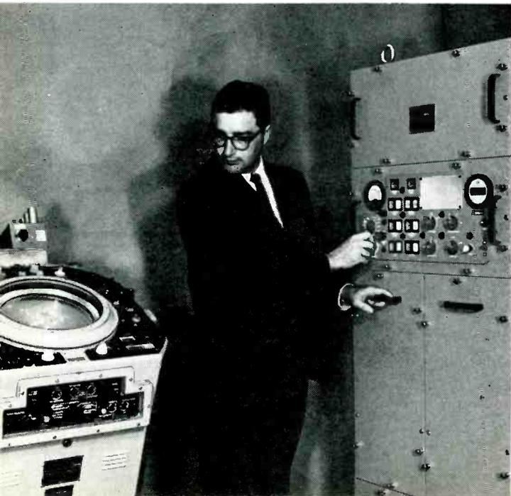
**SEMICONDUCTOR FILMS**, intermetallic, and of a good variety, can be made by the independent evaporation of the separate elements onto a heated substrate, according to engineers at the U. S. Naval Ordnance Lab. They also report good polycrystalline films as well as mixed crystals by this method. "Techniques and Apparatus for Evaporating Compound Semiconductors," (AD 600 676) (50¢).\*
