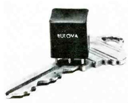
The K-572 is a broadband transformer measuring 0.13 cu.-in. in volume. Applications include balance mixers, balance modulators, ring modulators and the output stages of linear exciters. Power level is 0.3wac. Primary impedance is 170Ω center tapped; secondary is 50Ω. Max. allowable dc current in primary is 250ma. Bulova Watch Co., Inc., 60-20 Woodside Ave., Woodside, N. Y.
