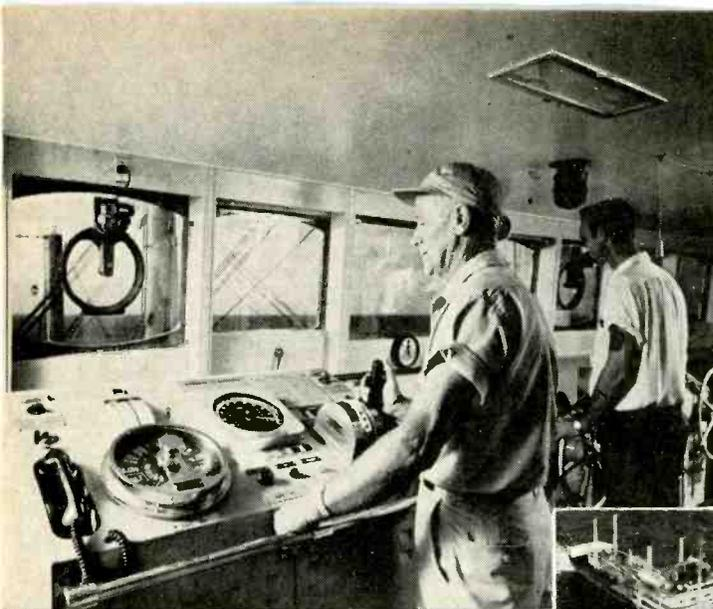
Fig. 1. Automated bridge console permits speed control direct from bridge, no longer requiring tug handling.
