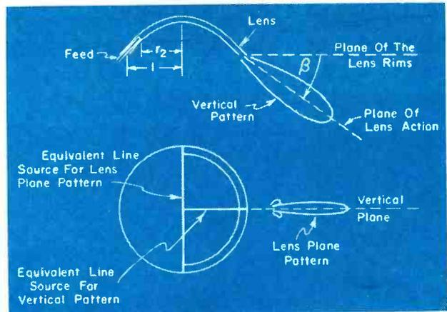
Fig. 2: The geodesic lens antenna focuses the energy by design of the lens contour.
