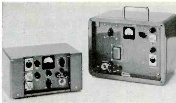
Solid state TV relay 2 GC transmitter (l), and receiver (r).
