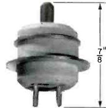
General Electric's new 7911 miniature planar ceramic microwave triode offers advantages in size, weight and performance over previous types. Weight is slashed at least 75%, height reduced to only  $\frac{7}{8}$ ". You get up to 3 times greater tube gain-bandwidth product and transconductance/ma. It is ideally suited for beacons and radar altimeters, and new broadband concepts for DME-TACAN-IFF equipment.
