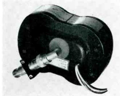
The X-1153 series features noise output of 85db below the carrier. Min. power output is 20mw with typical operation at 40 to 50mw. Applications include receiver local oscillators, sweep signal test equipment, telemetry, radar altimeters, and parametric amplifiers for freq.-agile radars. Eitel-McCullough, Inc., 301 Industrial Way, San Carlos, Calif.
