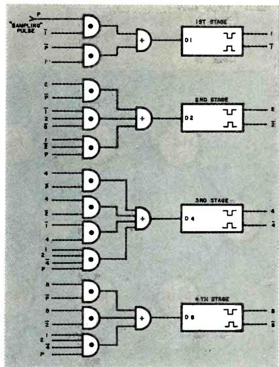
Fig. 6: Standard delay line binary decade.
