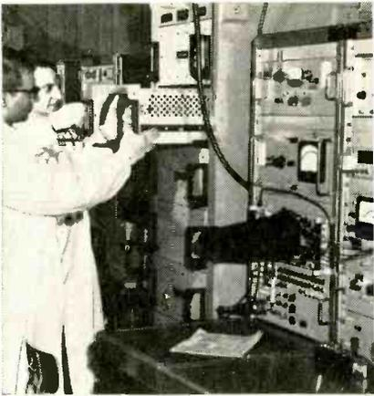
Technicians insert final drawer of equipment for initial radio communication sub-system for the Minuteman ground electronics system. Test console, right, used to check out performance of system, made by Sylvania Electric Products, Inc., before shipment for testing, and then to Air Force. System will provide control and missile data when a regular cable system becomes inoperative.
