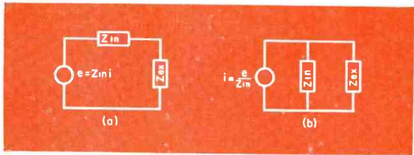
Fig. 2: Equivalent generator forms for voltage (a) and current (b) generators.
