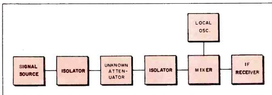
Fig. 2: Measurement of attenuation using the i-f substitution method is shown at left.
