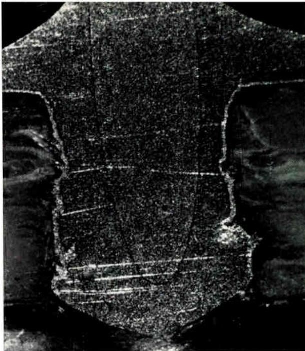
Fig. 1: Typical solder joint in a one-sided CC-4 printed-circuit board, with punched holes that have been plated through.
