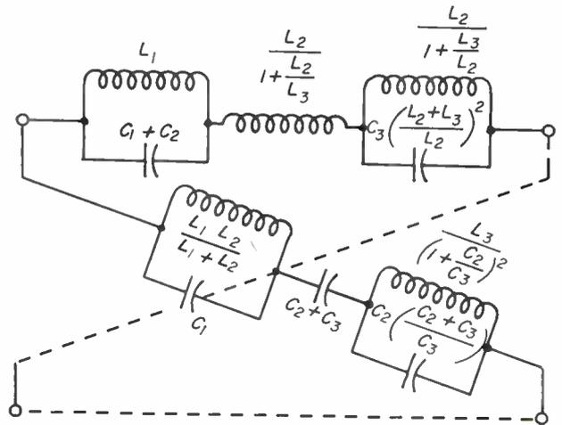
Fig. 7: The dipoles shown in Figure 5 were transformed into the above to facilitate simplification of the circuit.
