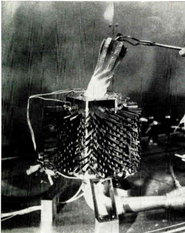
Fig. 8: RCA fossil-fueled thermoelectric test generator.
