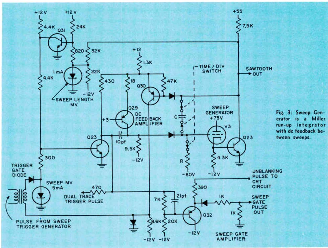
Fig. 3: Sweep Generator is a Miller run-up integrator with dc feedback between sweeps.
