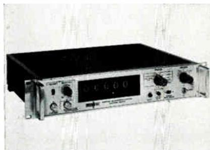
The 600 series feature PC motherboards with plug-in circuit cards. This replaces the basic circuit wiring harnesses. Display time is variable from about 0.2 sec. to 5 sec., and is independent of gate time. Memory or non-memory display mode may be selected by a front panel switch. The count gate may be locally or remotely controlled. Computer Measurements Co., 12970 Bradley Ave., San Fernando, Calif. Circle 246 on Inquiry Card
