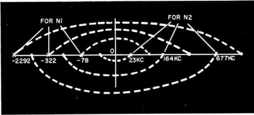
Fig. 3: Poles and zeros location of voltage ratio after synthesis of Fig. 2.
