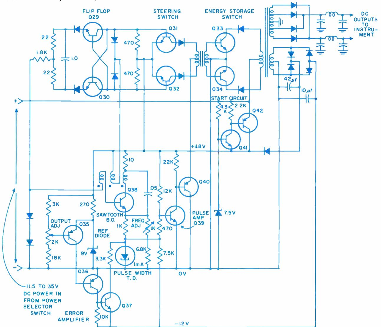
Fig. 4a: In battery supply, a duty cycle regulator and dc-dc converter are combined.
