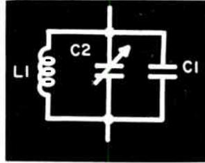
Fig. 2: Practical parallel tuned circuit.
