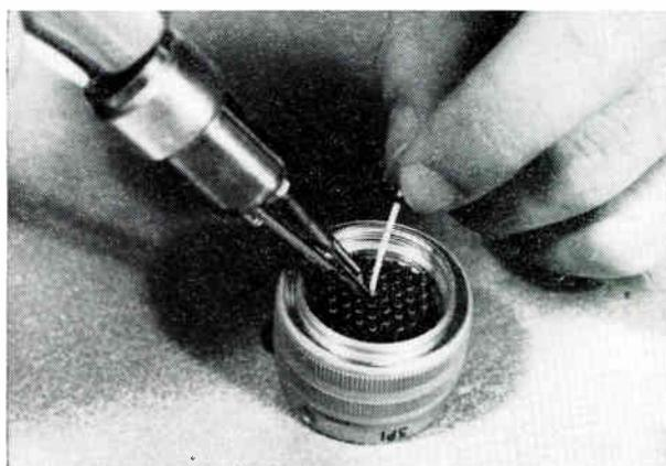
Tip causes heat to be generated only on work surface.
