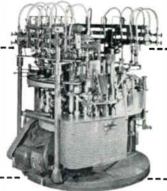
**Assembly Machine No. 3711**—Cat-whisker welder for crystal diode assembly. Automatically welds 3,000 units per hour.
