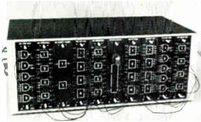
Model DT-2605 Inte-Patch unit is a versatile logic design tool. With it complete systems, including interface with electromechanical devices, can be designed. It uses analog, digital, and hybrid plug-in logic boards which use integrated circuits and discrete components. It also allows integrated circuits to be evaluated. Data Technology Corp., Box 10935, Palo Alto, Calif.
