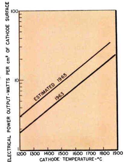
Fig. 12: State-of-the-art performance of thermionic converters.
