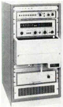
The Vidar 5100 offers microvolt sensitivity on the lowest range. It makes low-level measurements directly without further amplification. The system is floated and guarded from power-line ground with a common mode rejection of 160db at all freqs. The system integrates digital voltmeter, high-speed paper-tape printer, and a system coupler. Channel identification, polarity, 5 digits of data, and range are printed at a max. rate of 600 channels/min. Vidar Corp., Mountain View, Calif.
