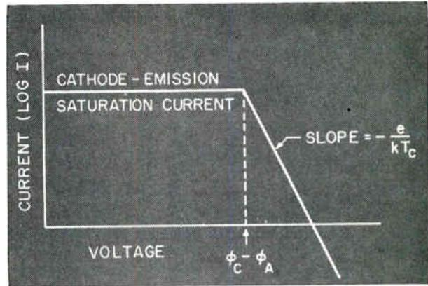
Fig. 11: Idealized V-A characteristic for thermionic converter.
