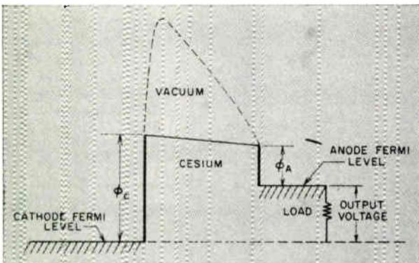
Fig. 9: Potential energy diagram for thermionic converters.
