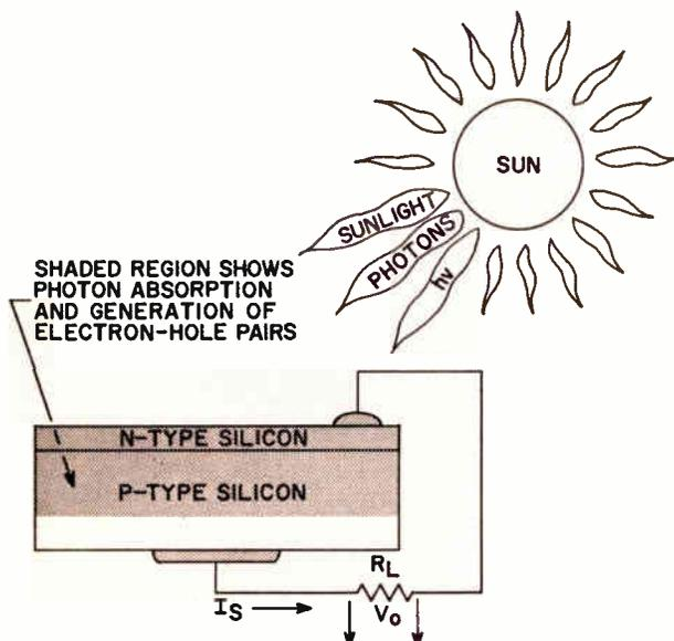
Fig. 2: Basic action of solar cell. Shaded region has intense ionization due to electron-hole pairs generated by light.
