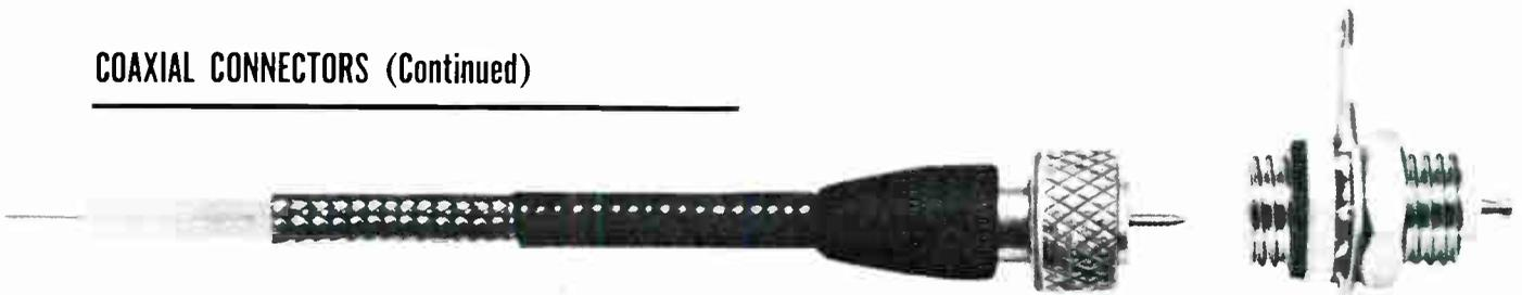
Typical Coaxial Plug and Receptacle
