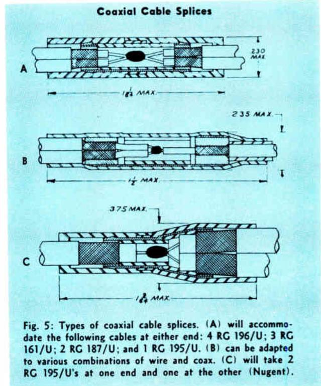
Fig. 5: Types of coaxial cable splices. (A) will accommodate the following cables at either end: 4 RG 196/U; 3 RG 161/U; 2 RG 187/U; and 1 RG 195/U. (B) can be adapted to various combinations of wire and coax. (C) will take 2 RG 195/U's at one end and one at the other (Nugent).
