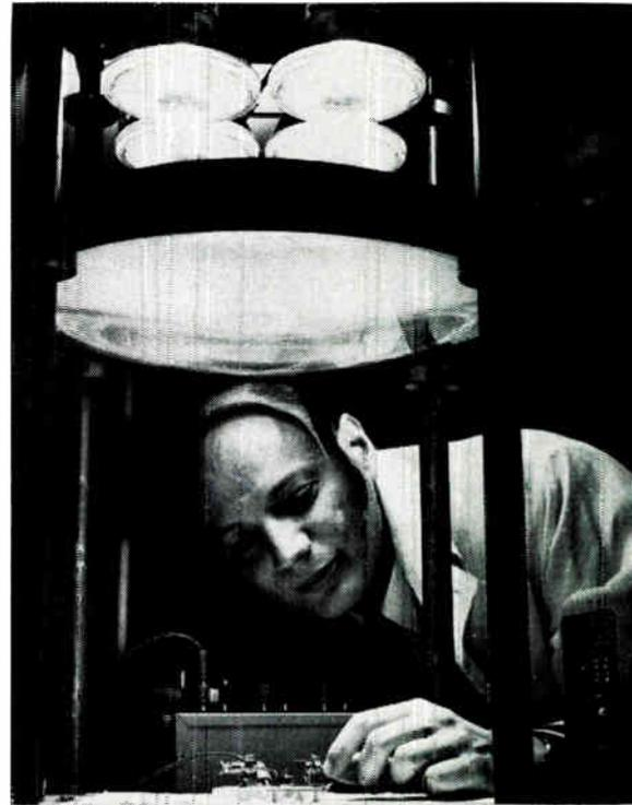
Author P. Rappaport of RCA Labs Technical Staff testing power output of a solar cell under a simulated source of solar energy.
