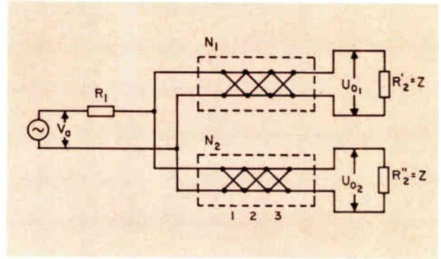
Fig. 2: Principal schematic of phase networks (splitter).
