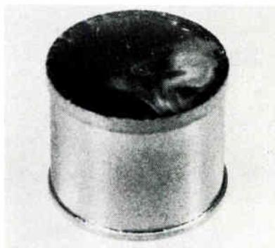
Fig. 5: Si-Ge thermoelement with tungsten contacts.
