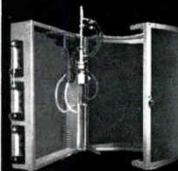
Enclosure for plasma device includes hinged protective shield of tinted plexiglas and flow meters.
