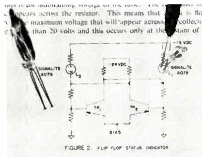
Lamp type A079 is designed to hold its operating characteristics throughout its rated lifetime of 7,500 hrs. Operating characteristics include: max. breakdown voltage, 70vdc; max. maintaining voltage, 58vdc; minimum extinguishing voltage, 47vdc; and design current, 0.3ma. Its operating temp. range is from  $-55^{\circ}\text{C}$  to  $+90^{\circ}\text{C}$ . Signalite, Inc., 1933 Heck Ave., Neptune, N. J.
