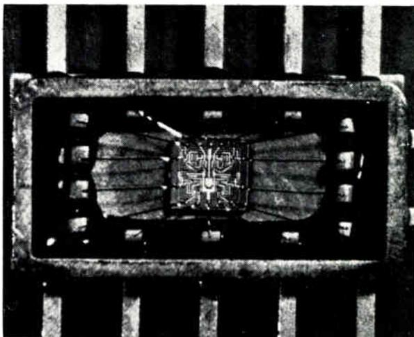
The series uses a multi-function concept—packing up to 4 circuit functions into one monolithic bar of silicon.
