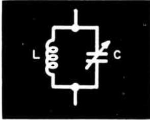
Fig. 1: Practicable parallel tuned circuit.
