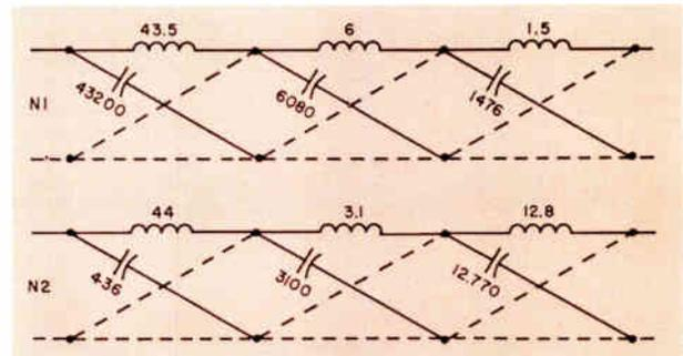
Fig. 4 (below): The elements of six pole networks according to the pole and zero distribution that is shown in Fig. 3 above.
