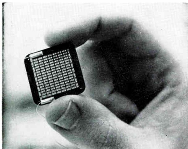
the ferrite powder using a 256-pin die. The perforated sheet is then sintered at a high temperature, using a controlled atmosphere to develop suitable magnetic properties. A copper circuit pattern with attached leads is then applied to the sheet and it is then wired by passing fine wires through each hole.
