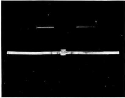
Uniceram Hi Q UY01 capacitors offer a choice of tolerances for each size—from  $\pm 0.25$  to  $\pm 0.50$ pf at the low C end of the line to from  $\pm 1$  to  $\pm 10\%$  at the high end. All units have a guaranteed min. Q of 3000. The 7/64-in. sq. and  $\pm 1/16$ -in. thick units have ceramic dielectric layers fused into a monolithic structure and encapsulated in solid glass. JFD Electronics Corp., 1462 62nd St., Brooklyn, N. Y.
