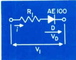
Fig. 1: Basic circuit of a tunnel diode in series with a resistor connected to dc.
