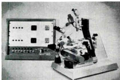
Model XY-540 is an automatically controlled production machine. It contacts components in the slice form prior to the scribing or dicing operations. Up to 16 probes and inkers can be set within a 0.015 x 0.015 in. area. Each probe is adjustable in X, Y, and Z-planes. The probes are stationary while the micro-circuit slice is reciprocating up and down to contact the probes. Cycling speed of machine is 10K/hr. Transistor Automation Corp., 18 Moulton St., Cambridge, Mass.
