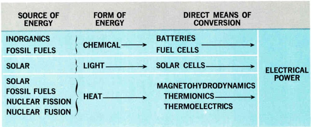
Fig. 1: Direct-energy-conversion technologies
