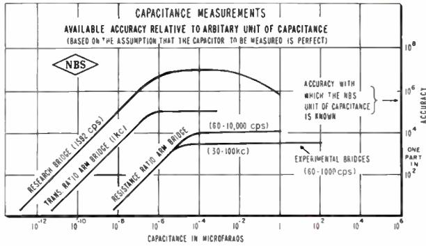
Fig. 2: Accuracies of measurement, based on NBS standards.
