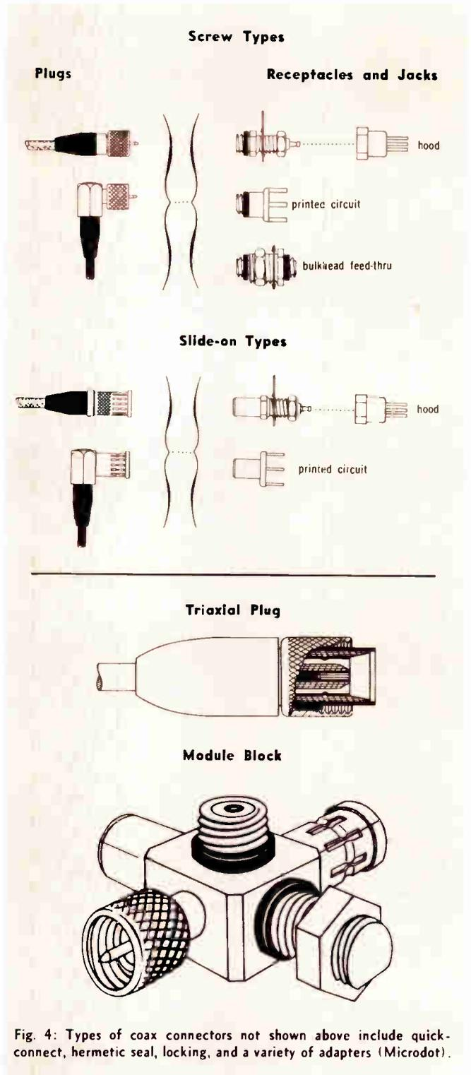
Fig. 4: Types of coax connectors not shown above include quick-connect, hermetic seal, locking, and a variety of adapters (Microdot).
