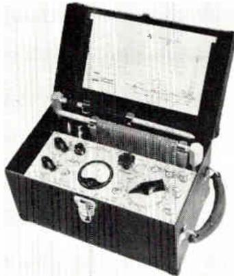
The type A Groundometer features a transistor operated 1-f bridge power source. It uses a synchronous meter detector to eliminate stray ac and dc ground currents. Full scale ranges are 1-10-100-1K and 10KΩ. It is used for measuring the resistance path of grounding electrodes for lightning arrestors, transformers, relays, transmission line towers, telephone and telegraph equipment, etc. Industrial Instruments Inc., Borden Engineering Div., 89 Commerce Rd., Cedar Grove, N. J.
