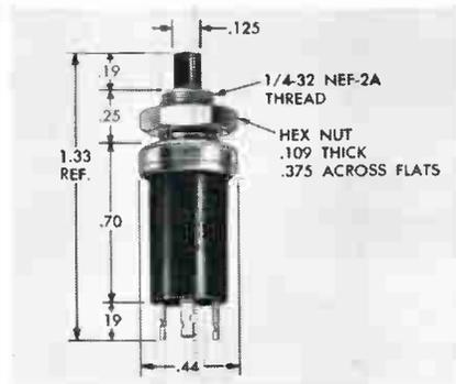
Contact resistance of series 46 after 250,000 operations is 0.010Ω typical, 0.020Ω max. Voltage breakdown is 1500vac and life expectancy is 250,000 operations at rated load. Actuating force is 16 oz. to bottom. The mounting nut and cover bushing are cadmium plated brass; contact terminals and shorting bars are silver-plated phosphor bronze. Grayhill, Inc., 561 Hillgrove Ave., La Grange, Ill.
