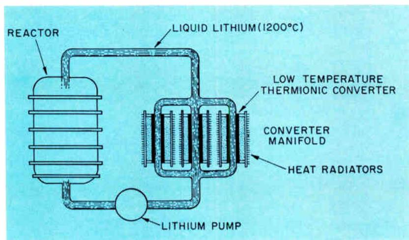
Fig. 15 (left): Reactor thermionic system using liquid lithium.
