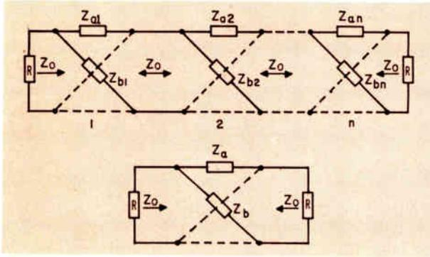
Fig. 1: A chain of lattices and its substitute lattice.
