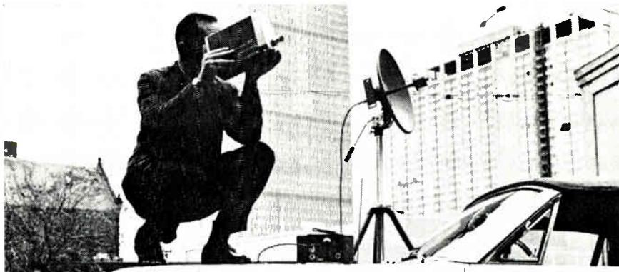
All-solid-state portable TV system introduced by Microwave Associates works from auto cigaret lighter. Works from 1.9 to 2.1 gc and mobile relay band. Applications include high-speed data sending, radar, telemetry, multi-channel TV. Usable to 50-mile radius.
