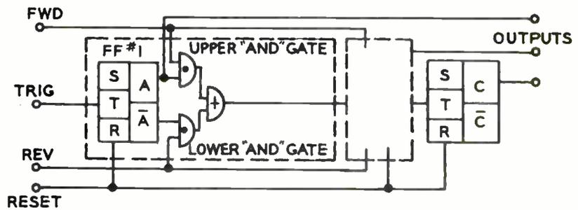
Fig. 3: The 3-stage reversible counter logic diagram.
