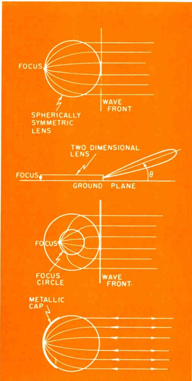
Fig. 7: Luneberg lens is a spherical lens of dielectric material.
