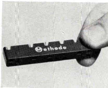
Model TB-809 WS is a 9-contact bussing connector. It is expected to be used in communications, data acquisition and transmission equipment. The connector mounts through 0.051 dia. holes. Jumper bars are available for bussing between any pair of contacts. Insulation is glass-filled diallyl phthalate. Connector measures 2 3/8 x 0.340 x 7/16 in., not including terminals. Methode Electronics, Inc., 7447 W. Wilson Ave., Chicago, Ill.
