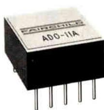
**Differential Amplifier—ADO-11** Voltage Drift =  $3\mu V/^\circ C$  (max.). Gain Bandwidth Product = 1.6Mc (min.). Temperature range =  $-55^\circ C$  to  $+125^\circ C$ . Full compliance with MIL-D-16400 and MIL-E-5400. (Specify part number ADO-11M for 12V/ $\mu$ sec slewing rate.) Dimensions:  $1'' \times 1\frac{1}{8}'' \times \frac{1}{2}''$ . Price: \$150.
