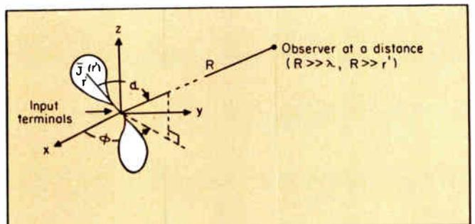
Fig. 2: Receiving ant. in field of elliptically polarized wave.
