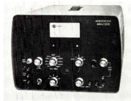
This solid-state unit consistently portrays 5 different parameters on visual hysteresis plots, plus 3 additional measurements which can be calculated. It offers integration ratios from 10:1 to  $10^6:1$  and an integration amplification of 50db gain to each axis. Range is 50 cps to  $50\text{kc}$ ; noise and hum level is  $50\mu\text{v}$ . Power output is  $50\text{w}$ .; power input is from 105 to  $125\text{v}$ . RMS at 150 cps to 400 cps. Emco Systems Inc., 922 S. Lyon Ave., Santa Ana, Calif.
