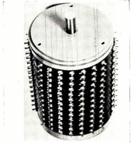
Model 205S contains 13 pot gangs. This film potentiometer functions as a precision voltage divider with multi-increment fixed voltage taps. The same pot can also be used to custom shape non-linear functions (experimentally) until the precise, desired function is obtained. With excitation applied to the wiper, it provides multiple gating signals. Terminal resistance is 120KΩ. Computer Instruments Corp., 92 Madison Ave., Hempstead, L. I., N. Y.
