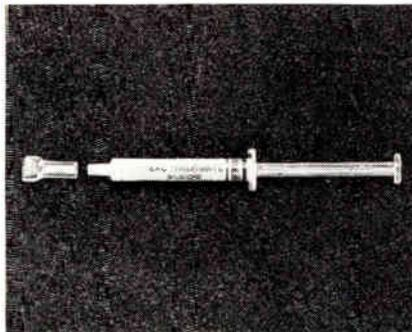
Ther-Mate is a compound of improved silicone grease. It is contained in a dispenser. In use, the dispenser provides easy application to thermal interfaces such as mounting a transistor to a heat sink. The compound is heavily loaded with metal oxides to increase thermal conductivity. It will not harden, soften or run within a temp. range of  $-65$  to  $200^{\circ}\text{C}$  in continuous use. International Electronic Research Corp., 135 W. Magnolia Blvd., Burbank, Calif.
