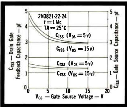
Figure 2. Important capacitance curves for 2N3821, 22, 24 transistors
