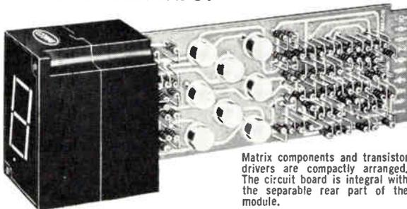
Matrix components and transistor drivers are compactly arranged. The circuit board is integral with the separable rear part of the module.
