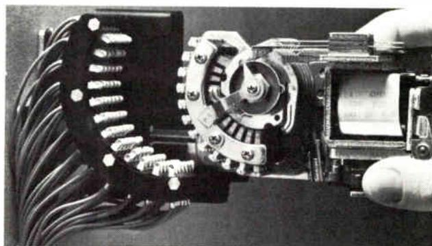
New AMP Inc. connector converts stepping switch into plug-in component. Crimp-on, snap-in contacts permit easy insertion of leads.
