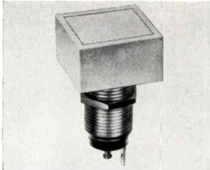
The Contempo 300 Series Square Lens indicator lights are two terminal devices. Series 301 features a  $\frac{3}{4}$  in. sq. lens, and mounts in a  $\frac{7}{16}$  in. dia. hole. It is 1-11/32 in. long. Unique feature of this series is its "push-pull" lens. The lens is "pulled" to remove, and "pushed" to install. Lens colors available are red, white, blue, green, and amber. The Sloan Co., P. O. Box 367, Sun Valley, Calif.
