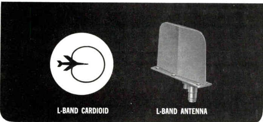
**L-BAND FEATURES** — Frequency - 950 to 1220 MC, VSWR - less than 1.8:1, Weight - less than 1 lb., Size 3.75 x 6.0 x 5 inches.
