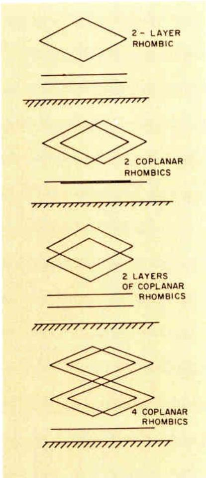
Fig. 5 (right): Basic configuration of single-wire double-rhomboid antenna for gain increase and sidelobe reduction.
