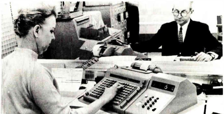
Desk digital computer, developed by Digital Electronics, Inc., instantly checks authenticity of messages in inter-bank activity, now in use at Chase Manhattan Bank, New York. Each computer can index up to 999 identity numbers for member or corresponding banks.
