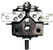
shipment from authorized P&B distributors. Tests show mechanical life will exceed one million operations . . . and the twin contacts are rated at 20 amperes at 115V AC, 60 cycles resistive or 28V DC, 1 HP 115/230V 60 cycles.
