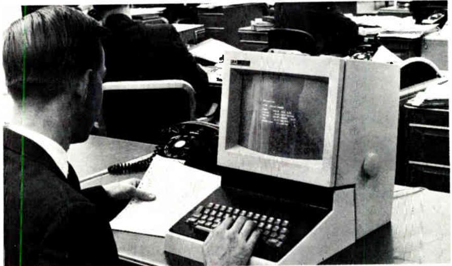
New IBM table-top device provides visual image of computer-stored information, and can help management of small and large firms maintain tight control over business activity. The 2260 can display insurance records, logs of customer calls, inventory-shipping data.
