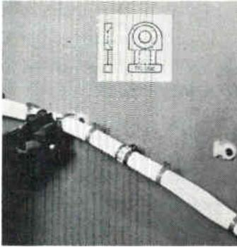
High density electronic packaging and appearance problems are solved with the TY-RAP miniature mount. Harnesses and cables can be tied to these pre-mountable bases with standard TY-RAP ties. The mounts are available in various sizes and accommodate different cable bundle diameters, holding strength up to 50 lbs. Available with screw holes, the mount is easily fastened to chassis. Clamping Section of T&B catalog T66 illustrates over 30 catalog numbers with complete details.
