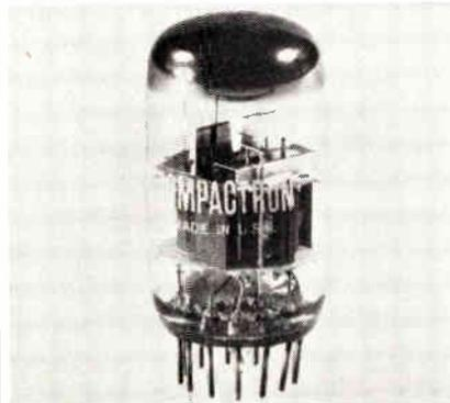
The 9BJ11 Compactron offers sensitivity equal to some 3-stage amplifiers. It can lower costs, improve performance levels, and conserve space in the manufacture of monochrome TV receivers. Construction features of the input section eliminate the need for a gain-robbing un-bypassed cathode resistor. It provides high transductance and low capacitance in each section. High-input impedance unloads the mixer stage for improved tuner gain. General Electric Co., 3800 N. Milwaukee Ave., Chicago, Ill.
