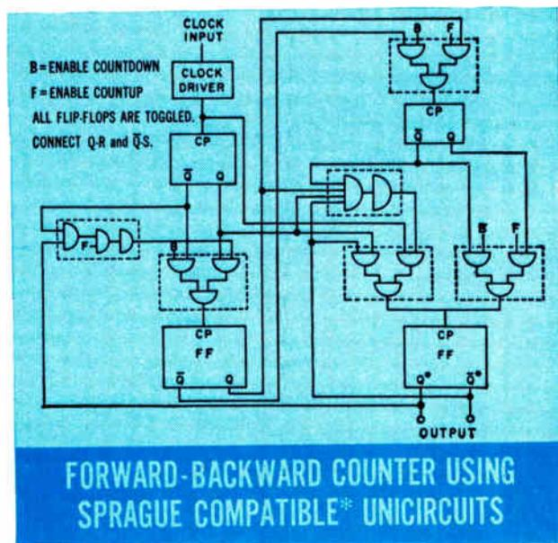
**\*Series US-0100 Unicircuits now provide the electronic industry with two major sources for low-power RCTL circuits.**
