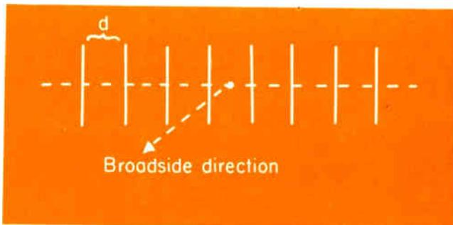
Fig. 6: Broadside array of parallel dipoles is illustrated.
