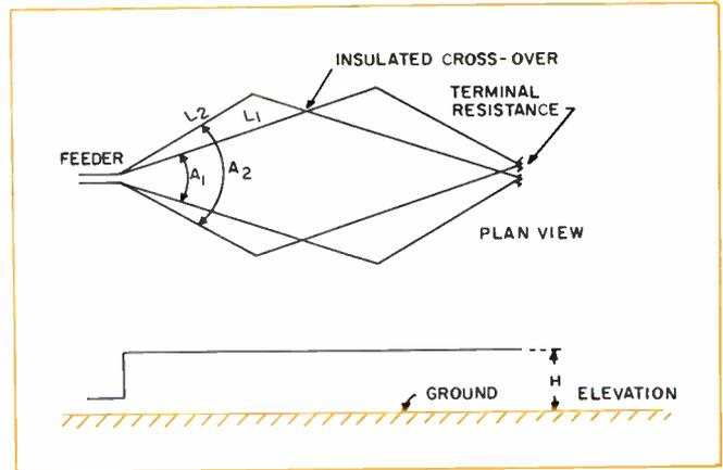
Fig. 4 (left): Plan and elevation views of methods for arraying rhombic units for sidelobe reduction and gain improvement.
