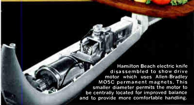
Hamilton Beach electric knife disassembled to show drive motor which uses Allen-Bradley MO5C permanent magnets. This smaller diameter permits the motor to be centrally located for improved balance and to provide more comfortable handling.
