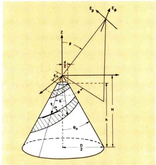
Fig. 6: The basic parameters of the 2 arm balanced conical.
