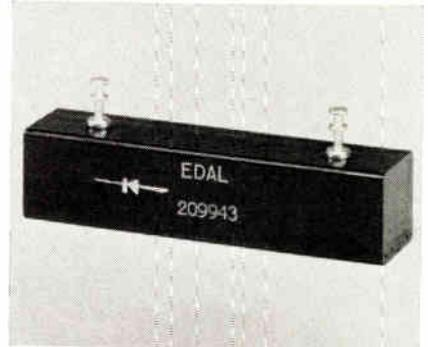
The Series N cold case silicon packages eliminate soldering many diodes to achieve equivalent circuitry. Available in full-wave, half-wave, doubler, center tap, open bridge and 3 phase types. Units consist of matched, pre-tested, pre-selected, double diffused avalanche rectifiers, self-protected against voltage transients. Standard types offer voltage ratings from 1500 to 30Kv PIV, with currents from 20ma to 6a. Edal Industries, Inc., 4 Short Beach Rd., East Haven, Conn.
