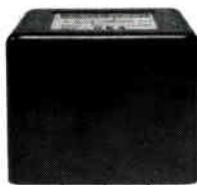
**Differential Amplifier—ADF-1** Drift= $1\mu\text{V}/^\circ\text{C}$ . from  $0^\circ\text{C}$ . to  $+60^\circ\text{C}$ . Noise less than  $5\mu\text{V}/\text{p-p}$ . Common mode rejection = 90 db @ 60 cps; 100 db @ DC. Fixed gain = 1000. Size =  $1\frac{1}{2}'' \times 1\frac{1}{2}'' \times 1\frac{1}{2}''$ . Output =  $20\text{V}/\text{p-p}$  @ 1mA. Pre-aged—100 hour operational test. Prices: 1-4, \$190; 5-9, \$177; 10-24, \$167; 25-99, \$160.
