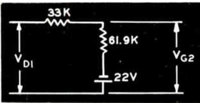
Fig. 2: Equivalent circuit for on-off condition.
