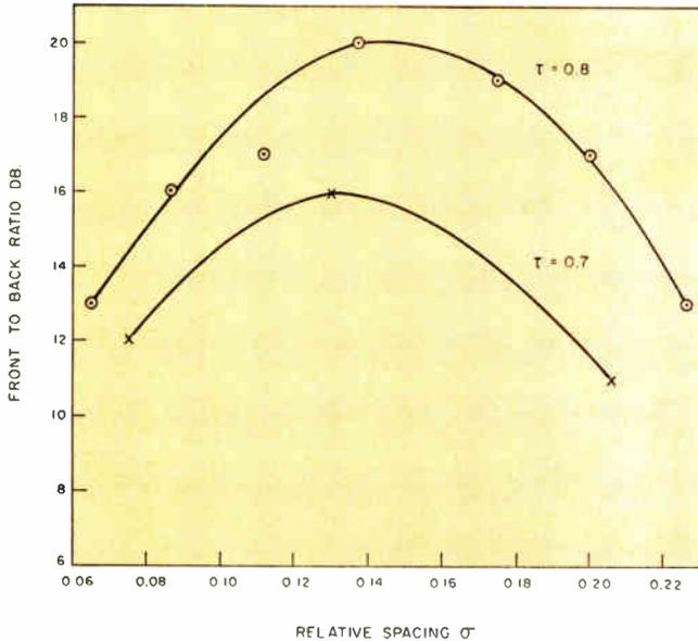
Fig. 5: Computed LP pattern front-to-back ratio vs.  $\tau$  and  $\sigma$ .
