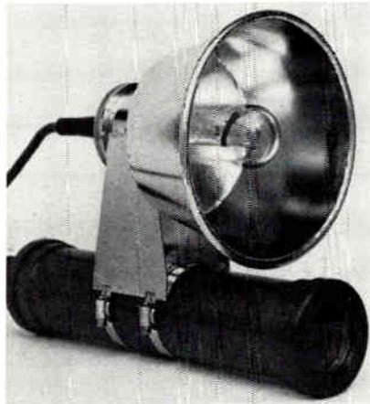
A complete underwater TV system workable down to 1300 ft. in fresh or salt water developed by Cohu Electronics, Inc., includes Cohu 2000 series miniature TV camera (above), 12" long, 3" wide, with special underwater housing. Camera has fixed-focus half-inch lens with remote focus control, plus standard vidicon. Attached is mercury vapor lamp (400w.) that can stand 5000 psi.
