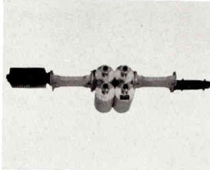
Model S4798B high-power band-pass filter is suited for radar uses where r-f interference is a problem. By preventing unwanted spurious emissions, it effectively eliminates any possible interference with neighboring radar systems. The filter displays a bandwidth ratio of less than 6 to 1 @ 60db. Freq. range is 2700-2900mc and ripple is 0.3db max. Power capability is 1.2 megawatts peak, 4.2kw average. vswr is 1.4:1 max. Aircraft Armaments, Inc., Cockeysville, Md.
