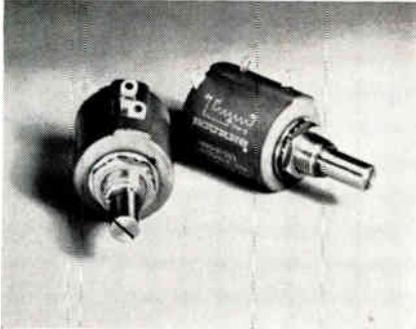
Model 3500 is 7/8 in. dia., bushing mount 10-turn unit. All-sealed construction ensures Mil-spec resistance to humidity. Silverweld® terminations, a fused bond between the terminal and resistance wire, eliminates fragile, single-wire termination. Resistance tolerance is ±3%; linearity is ±0.20%. Withstands vibration of 20G and shock of 100G. Bourns, Inc., 1200 Columbia Ave., Riverside, Calif.
