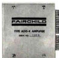
**Operational Amplifier—A00-4** Solid state, chopper stabilized. DC gain over  $5 \times 10^6$ . Gain Bandwidth Product = 2 megacycles. Output =  $\pm 20\text{V}$  @ 2mA;  $\pm 10\text{V}$  @ 7mA. Drift less than  $10\mu\text{V}/^\circ\text{C}$ . from  $-20^\circ\text{C}$ . to  $+85^\circ\text{C}$ . Plug-in case  $4'' \times 5'' \times 1''$ . P.C. edge connector. No chopper drive required. Prices: 1-4, \$92; 5-9, \$86; 10-24, \$81; 25-99, \$77.
