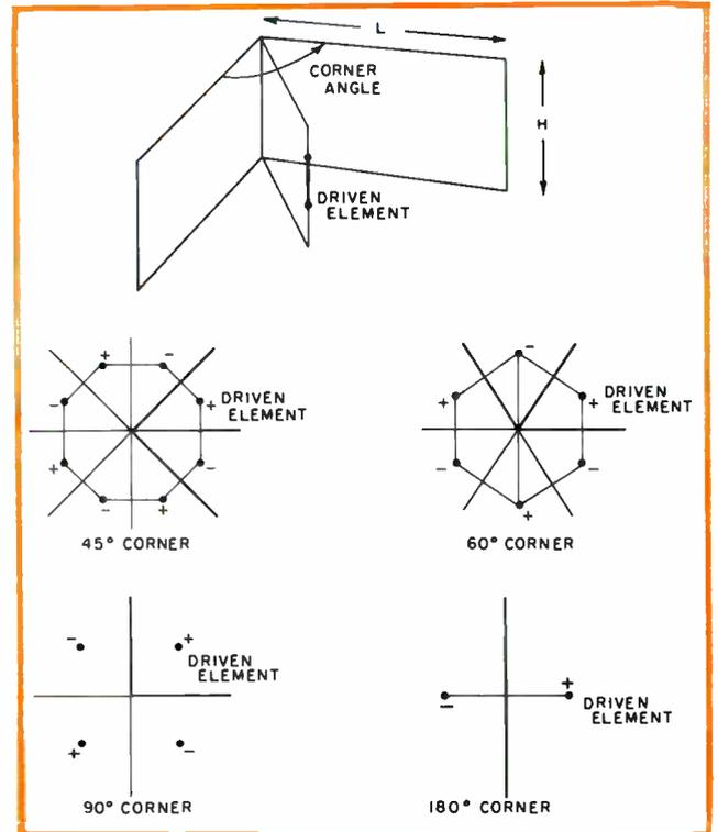
Fig. 5: Corner reflectors are a special case of reflector ant.
