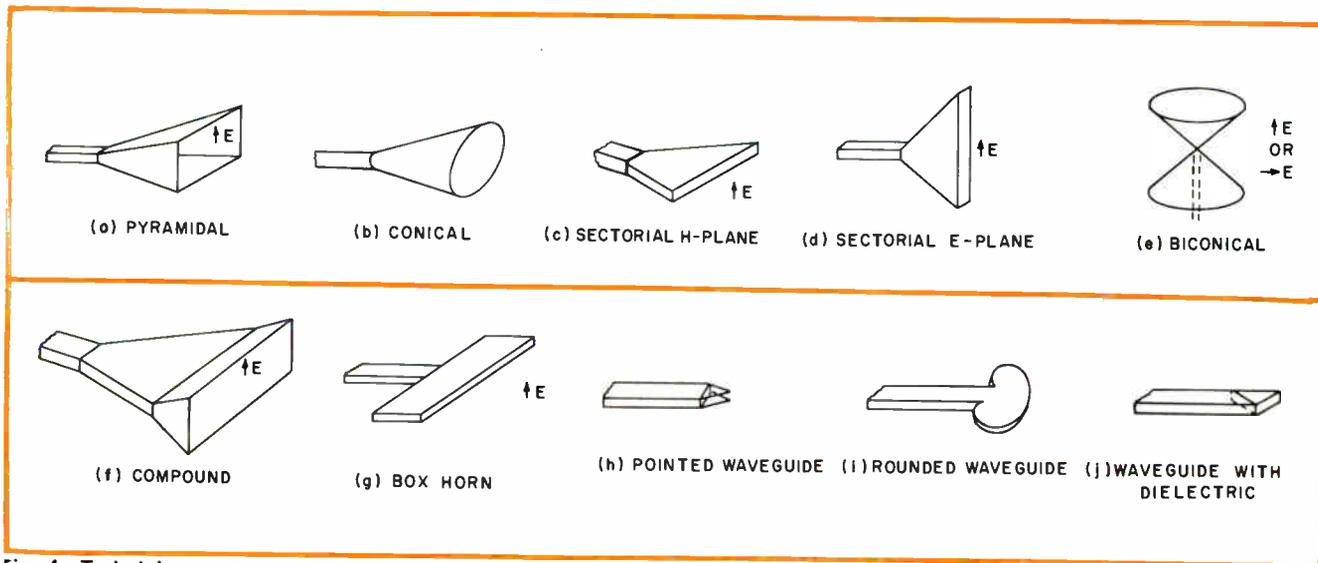
Fig. 4: Typical horn antennas. They are widely used because their dimensions are generally non-critical.
