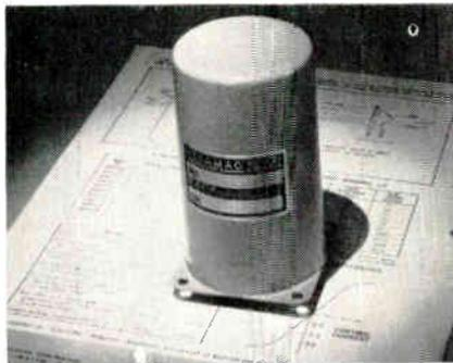
The Ultamag® 100 solid state magnetic amplifiers have high resistance to radiation. Available in either 50 or 60 cps. They can be used in almost any application where vacuum tubes or transistors are required. Life is 10 yrs. The units provide up to 43db polarity reversible gain with 0 stability better than 1%. Power requirements are 115vac  $\pm$ 10%, 50 or 60 cps. Military & Computer Electronics Corp., 900 N.E. 13th St., Ft. Lauderdale, Fla.
