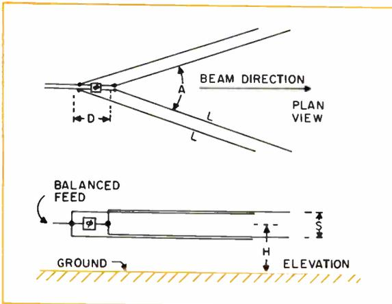
Fig. 3: Basic single-unit horizontal rhombic antenna.
