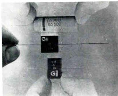
The CN series miniature monolithic ceramic capacitors have a range to 5.0 $\mu$ f. Packaged in transfer-molded plastic cases with non-polar operation, the units can be used over a temp. range of  $-55^{\circ}\text{C}$  to  $+125^{\circ}\text{C}$  without voltage derating. Capacitance will not change more than  $\pm 15\%$  over the temp. range. Gulton Industries, 212 Durham Ave., Metuchen, N.J.
