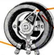
Rounded pivot gives metal-graphite contact brush flush-floating contact with wire.
