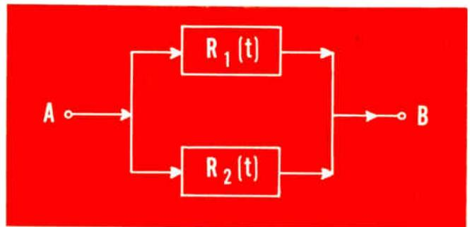
Fig. 1: Redundant path in which either block can successfully transfer signal  $A$  to output  $B$ , independent of one another.
