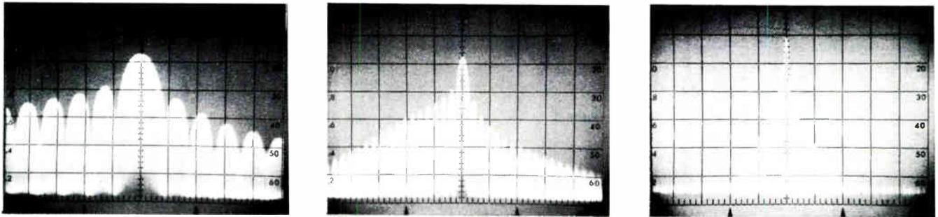
Fig. 5: Pulse spectrum with dispersion (a) of approximately  $1/T$  MC/cm; (b) approximately  $4/T$  MC/cm; (c) approximately  $10/T$  MC/cm.
