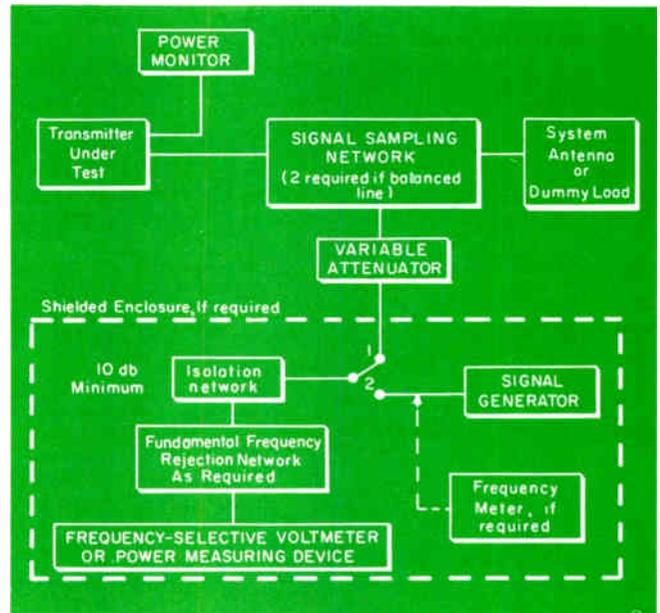
Fig. 1: Typical closed-system (non-radiated) measurement setup.
