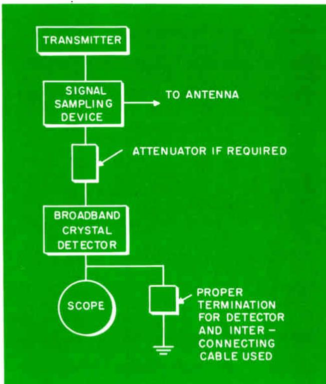
Fig. 6: Pulsed closed-system test setup for measurement of modulation characteristics.
