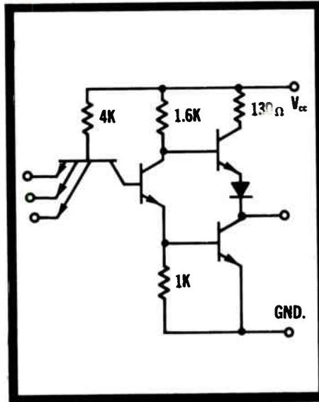
Figure 4. Circuit diagram for basic Series 54 NAND gate
