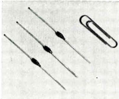
This zener is 0.145 in. in dia. and has a continuous rating of 5w. It can substitute for stud-mounted types many times its size. Voltages available are 6.8 to 400v. It features low dynamic impedances for all voltage ratings combined with extremely sharp knees. These zeners remain completely stable in electrical characteristics, even after overload or exposure to extreme environments. Unitorde Corp., 580 Pleasant St., Watertown, Mass.
