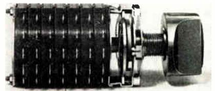
The series 1 switch line have independently sprung, dual, balanced moving contacts. Improved switching action reduces cross tracking between contact and insulation materials. The stators are keyed and nested for positive deck alignment. Other features include: adjustable stops (with 25 in./lb. stop strength ratings), identified terminals, silver or gold plated current carrying parts, and integral molded in terminals and contacts. Voltage breakdown is 1000v. rms. Shallcross Mfg. Co., Selma, N. C.
