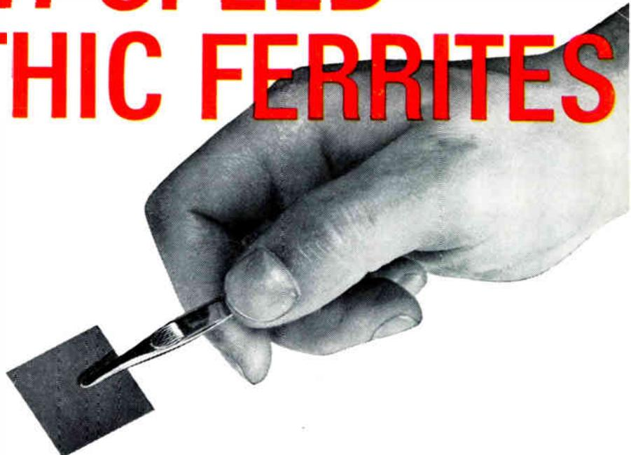
Each monolithic array contains 4096 "virtual cores" with an effective diameter of only 5 mils within a single, solid, sintered ferrite wafer only 1 in. by 1 in. by 0.005 in.
