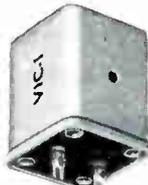
Nominal inductance values of 22 stock items in this series range from .0085 Hy to 130 Hys. Mean inductance may be varied  $+85\%$ ,  $-45\%$  through 60° rotation of adjustment screw in side of case. Rugged die cast case: 1-11/13" long, 1 1/4" wide, 1-7/16" high; weight 5 1/2 ounces.
