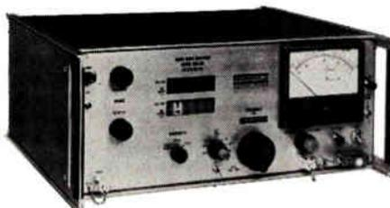
Front-end overload against off-frequency signals, and full capability for electronic frequency control and scanning, internally, or from a remote location, are typical of the unique features found in Audio Wave Analyzer Model EWA-88.
