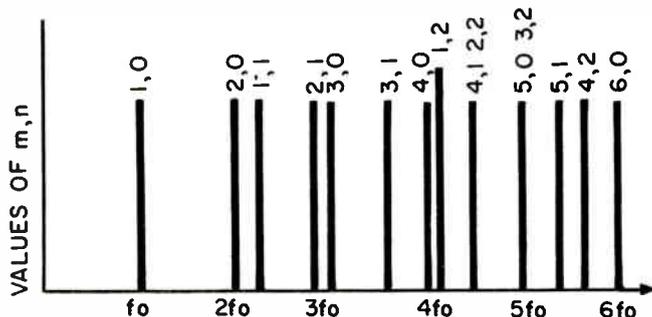
Fig. 3: Frequencies above which various  $TE_{mn}$  and  $TM_{mn}$  modes can propagate.
