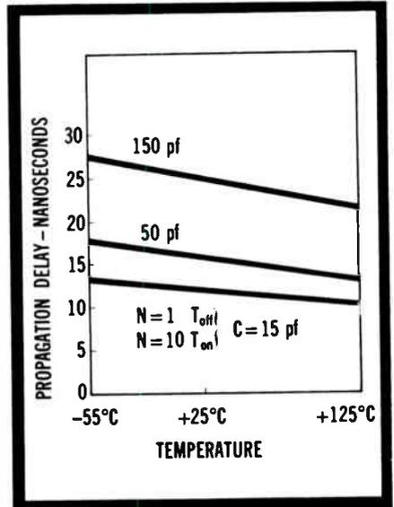
Figure 5. Typical propagation delay vs temperature
