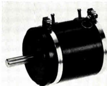
The D20-09 unit is 1.460 in. long. Available in resistances from 1K-200K, standard resolution runs to 0.0003%; absolute linearity of the units is to 0.01%. Total equivalent noise resistance level is 1000Ω max. Up to 4 cups can be ganged on the same shaft, each cup after the first adding 1.235 in. to the length. Technology Instrument Corp. of Calif., subs. of Bomar Instrument Corp., 850 Lawrence Dr., Newbury Park, Calif.
