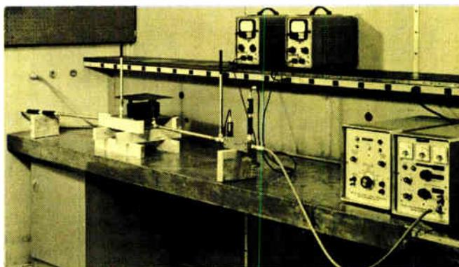
sensor and recorder system and a special field-intensity meter for use in intense fields very near a large radiator.
