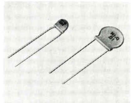
Flat bottom disk capacitors prevent rock or roll on PC boards because they seat perfectly every time. They eliminate electrode exposure normally encountered with bare bottom disks. The new configuration permits lower circuit board height without kinked leads, as well as complete control of Durez on wire leads. They may be used in applications up to and including 500v. Hi-Q Div., Aerovox Corp., Myrtle Beach, S.C.
