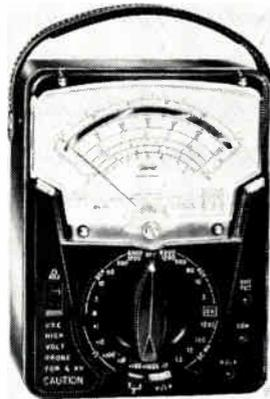
The Model 630-M features 20K $\Omega$ /vac sensitivity, one million  $\Omega$ /vdc sensitivity, and  $\pm 3\%$  ac accuracy. Sensitivity is derived from the singular achievement of its basic 0-1 dc  $\mu$ a suspension movement. The unit has no amplifiers, no zero drift, no warm-up, and no power requirements. It makes current measurements from 20na and voltage measurements from 5mv. The Triplett Electrical Instrument Co., Bluffton, Ohio.
