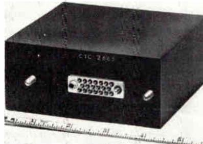
The CTC-2665 plug-in type transponder delay line has an impedance of 300 $\Omega$  ( $\pm 10\%$ ). Accuracy of each tap referred to input is  $\pm 30$ nsec.; figure of merit is 70; temp. excursion: operational -55°C to 125°C; storage, -65°C to 150°C; temp. coefficient of delay: 50 ppm/°C; attenuation is -3db. Columbia Technical Corp., Woodside, N. Y.
