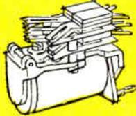
A general purpose relay whose consistent performance has been demonstrated in thousands of applications. It is available unenclosed, in dust covers, or hermetically sealed. Solder, taper-tab or direct plug-in terminals are provided for wired assembly mounting.
