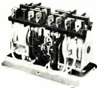
With the 25BL, momentary impulse on the unlatched coil causes the contacts to close and remain latched until the other coil is pulsed. Mechanical life exceeds 20 million operations. Electrical life depends on load characteristics. Pull-in voltages: dc, 75% nominal voltage; ac, 78% of nominal voltage. Designed for heavy duty, 2PDT, 4PDT, or 6PDT switching on ac or dc inputs, it is rated at loads of 5 or 10a. @ 115vac. Weight is 4.5 oz. E. W. Bliss Co., Eagle Signal Div., Davenport, Ia.
