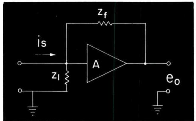
Fig. 5: Operational amplifier operating from a voltage source.
