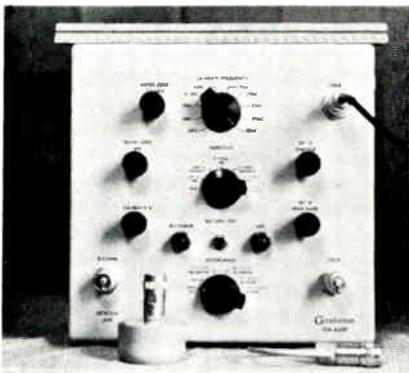
Probe unit of a near field-field intensity meter that is made by Genistron, Inc.
