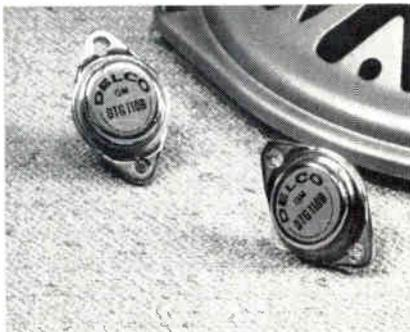
The DTG-110B has such high power handling capabilities that only 2 instead of 4 are needed to handle up to 100w. RMS power in class AB audio power output applications. It offers low distortion at high power levels. Linear gain (typically 125 at  $I_c$  of 5a.) and trans-conductance characteristics provide for very low amplifier distortion. Delco Radio Div., General Motors Corp., Kokomo, Ind.
