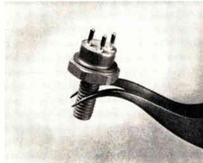
The 2N3818 VHF, NPN silicon power amplifier transistor is designed for Class C amplification from 25v. supplies. Uses include drivers for high-power varactor multiplier chains, and a single sideband amplifier for freqs. through the 74mc band. It is rated at 2a. continuous collector current and 80v. minimum pulse-breakdown voltage. Transistor is packaged in the TO-60 can and uses an interdigitated-type geometry. Motorola Semiconductor Products Inc., P.O. Box 955, Phoenix, Ariz.
