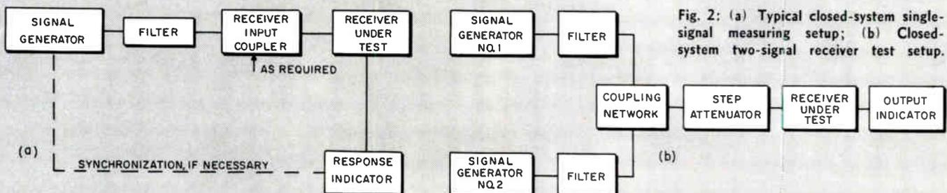
Fig. 2: (a) Typical closed-system single-signal measuring setup; (b) Closed-system two-signal receiver test setup.
