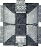
□ **High output voltage.** Equal to conventional cores. Trace indicates over 50 mv each for differential 1 and 0 output. Compare this with other bulk-fabricated systems having output voltages of only 1 or 2 mv.
