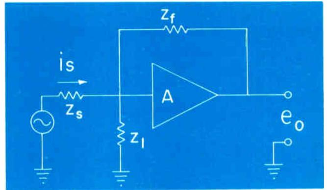
Fig. 1: Conventional feedback amplifier (above left).
