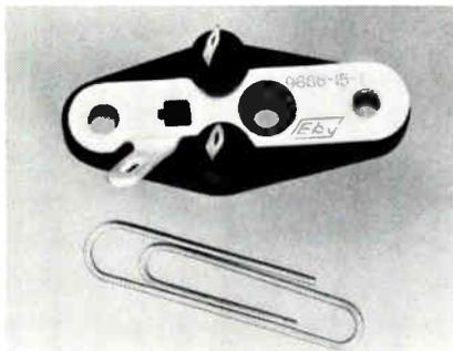
Fig. 9. Explosion proof connectors incorporate arc quenching contact inserts, a snap action coupling device and safe breaking of 200 amp loads (Pyle-National).
