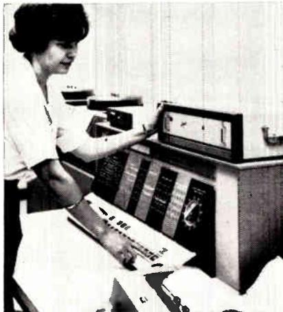
High-speed data sending system—"smaller and more reliable and economical"—introduced by GT&E. The system, Lenkurt 26C Duobinary-Datatel™ data set, transmits digital signals over conventional voice channels at fixed speeds of 2,400 and 1,200 bits/sec. The unit (atop the console above) includes integrated circuitry; is only 3½ inches high.
