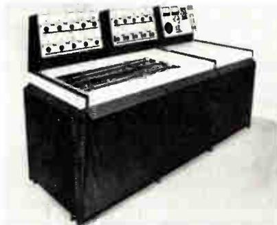
The Jet Plater deposits gold uniformly despite differences in surface areas. It eliminates the need for building up too thick a deposit of gold on one surface in order to accomplish the minimum thickness on the other side. It can also be used for the simultaneous plating of equal thickness deposits on internal and external surfaces of special parts where the current required for plating the separate areas varies. The Meaker Co., subs. of Sel-Rex Corp., 75 River Rd., Nutley, N.J.
