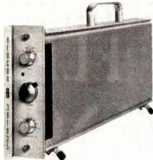
The 391 Series Low Level DC Differential Amplifier has a single gain between 10 and 1000 and a single bandwidth of 100kc. The 5 options are: 7 switched gains; 5 switched gains with full interpolating vernier; dual output; 8 switched bandwidth; triple output — high level multiplex switch for remote switching of 2nd output. Redcor Corp., 7800 Deering Ave., P. O. Box 1031, Canoga Park, Calif.
