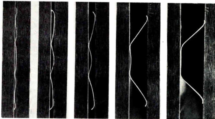
Fig. 3: The development of multiple lines of contact during compression of a single RFI floating finger strip for doors.
