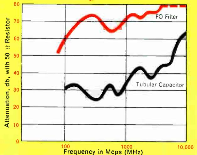
■ This new line of FO type subminiature low pass filters is designed to provide maximum reduction of RFI *in a minimum of space*—attenuation is greater than 50DB over the frequency range from 100 MHz to 10 GHz.
