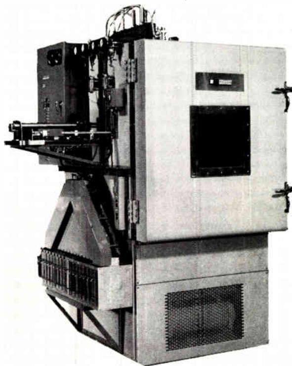
Test chamber automatically feeds and unloads 1500 devices/hr.
