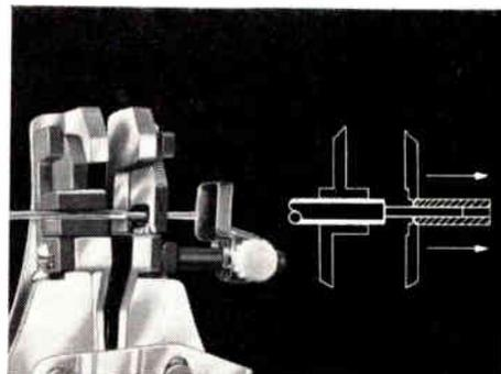
Die severs insulation and strips slug. Never touches conductor, can't nick or scrape.
