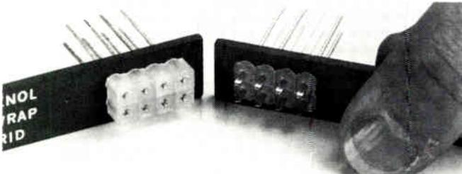
Fig. 2. Male and female connectors for patchboard use. Contacts are inserted into nylon bushings that are snapped into punched holes in a base plate (Amphenol).
