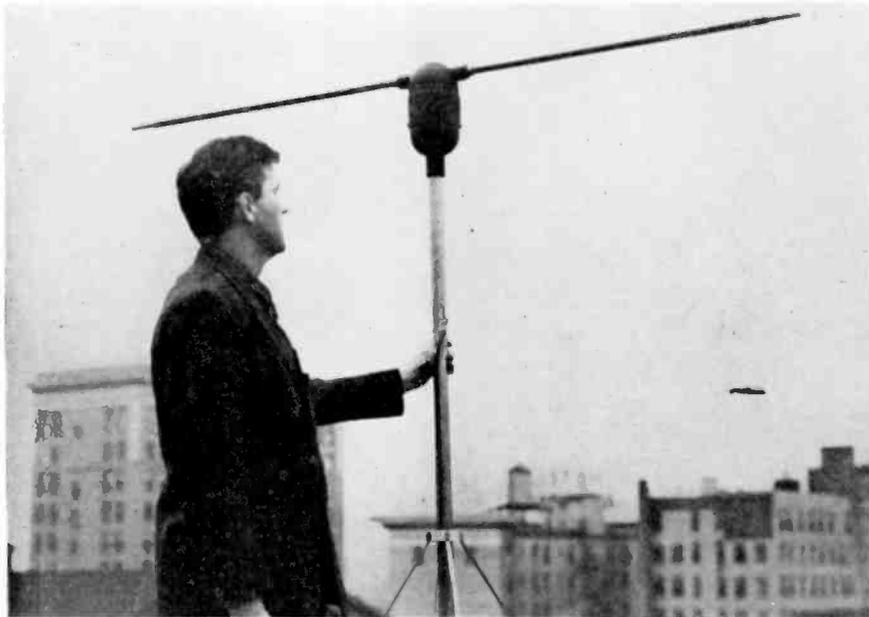
Farnsworth antenna, above, can be rotated clockwise and counterclockwise and has members which are extensible, allowing for proper orientation and tuning.
