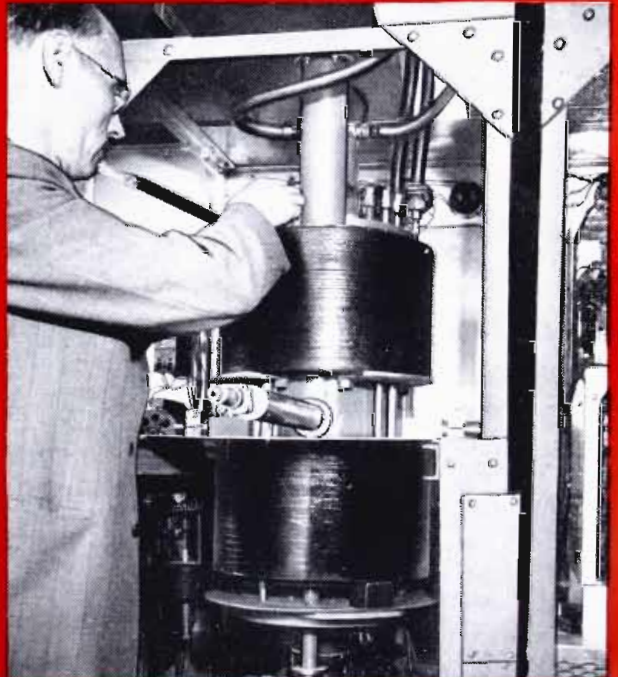
High-Power UHF Klystron Tube. A successful solution to the difficult problem of high power at UHF. Designed and built to G-E specifications, this tube's remarkable amplification and extreme stability actually make high-power UHF television a reality.
