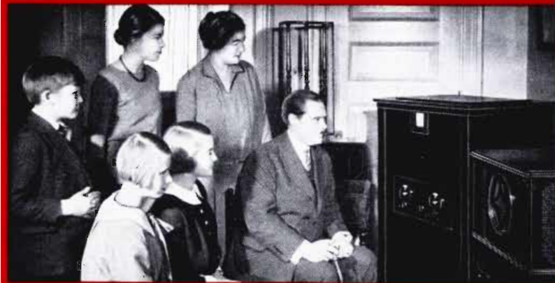
First Home TV Receiver, in 1927, at Schenectady. Dr. Alexanderson reveals his console model with a tiny 3" screen. The receiver used a rotating perforated disc to scan the image. Sound was received on a different wave length through speaker at right.
