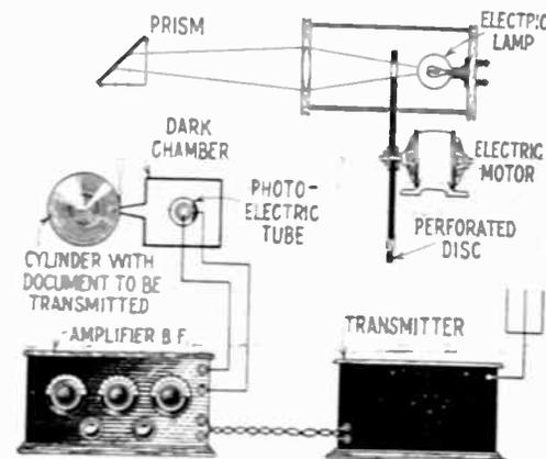
The above illustration shows clearly the arrangement of the apparatus and how it is coupled to the radio transmitter.
