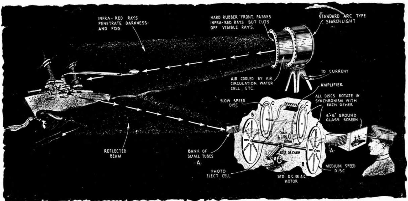
The apparatus used to receive the view illuminated by the invisible beam of the infra-red searchlight and render it visible to the eye of the operator, is shown in the above illustration. The infra-red rays have the property of penetrating darkness and fog and thus lend themselves to use during war time and also in locating ships lost at sea during a storm.
