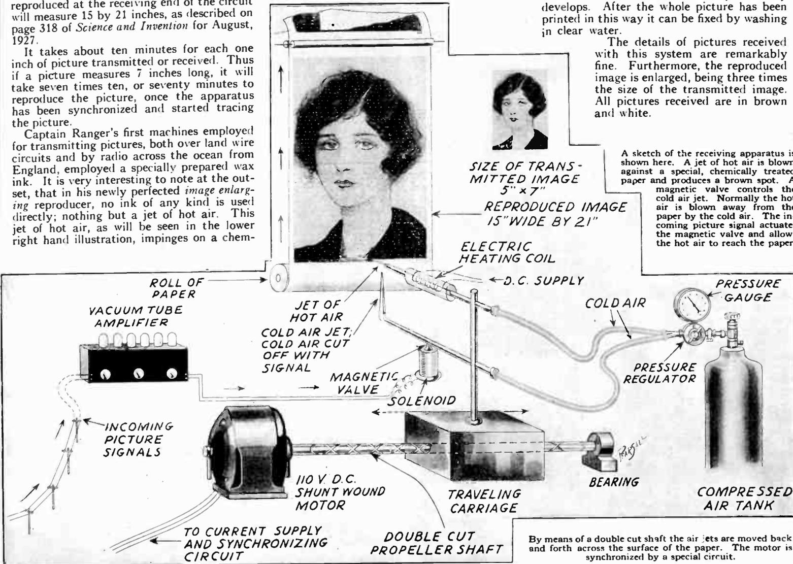
By means of a double cut shaft the air jets are moved back and forth across the surface of the paper. The motor is synchronized by a special circuit.
