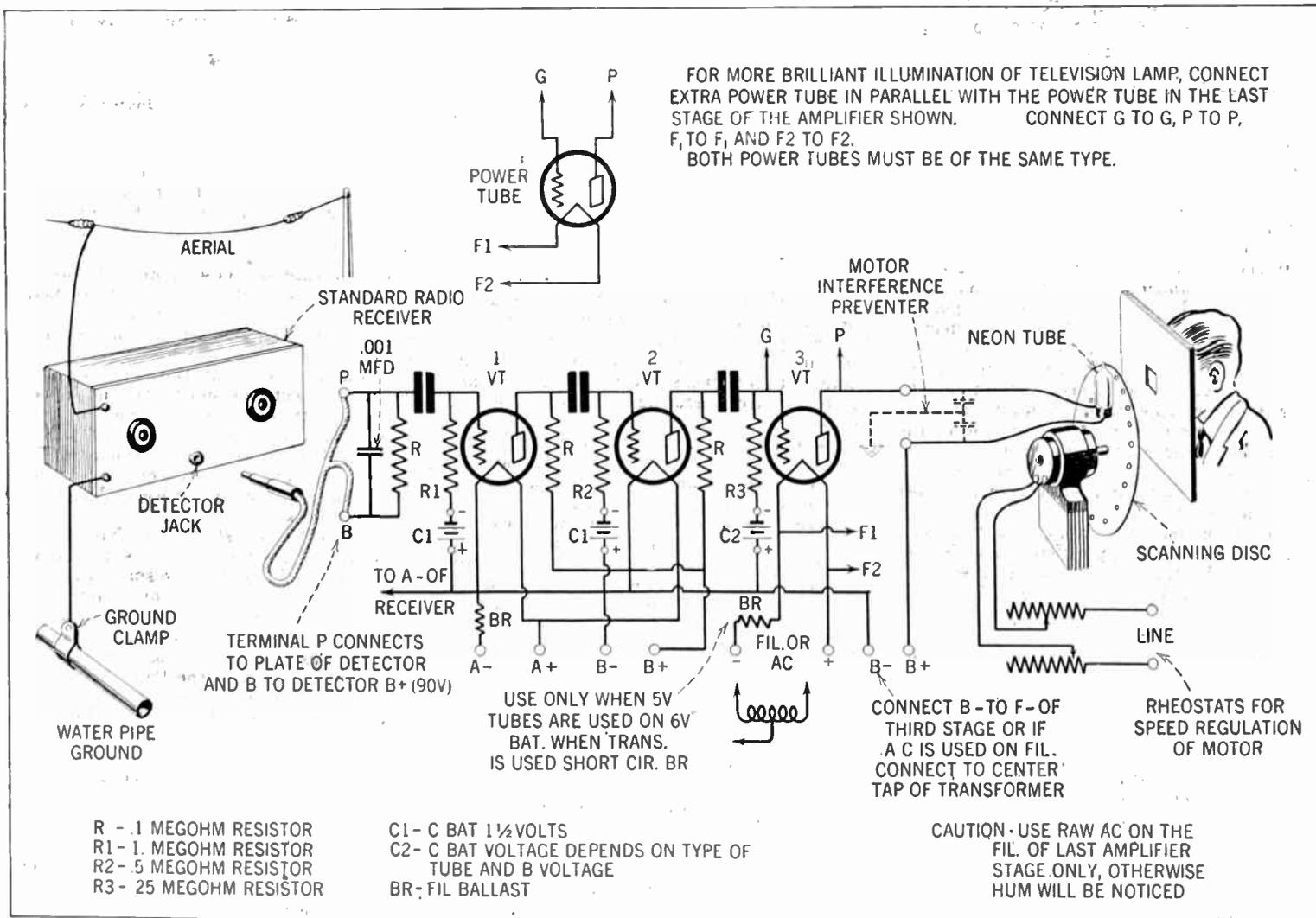
One of the best practical receiving circuits for television so far brought out is that shown above. As will be seen, three stages of resistance coupled amplification are connected, by means of a plug, into the detector jack of any standard radio receiving set. The last stage of the resistance coupled amplifier should be supplied with a power tube and at least 350 volts, supplied preferably from "B" batteries, or else
