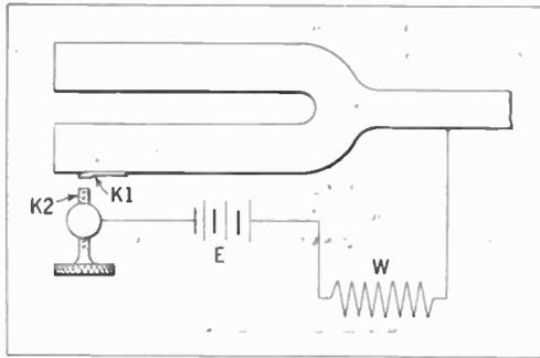
Diagram showing the principle of tuning-fork control.
