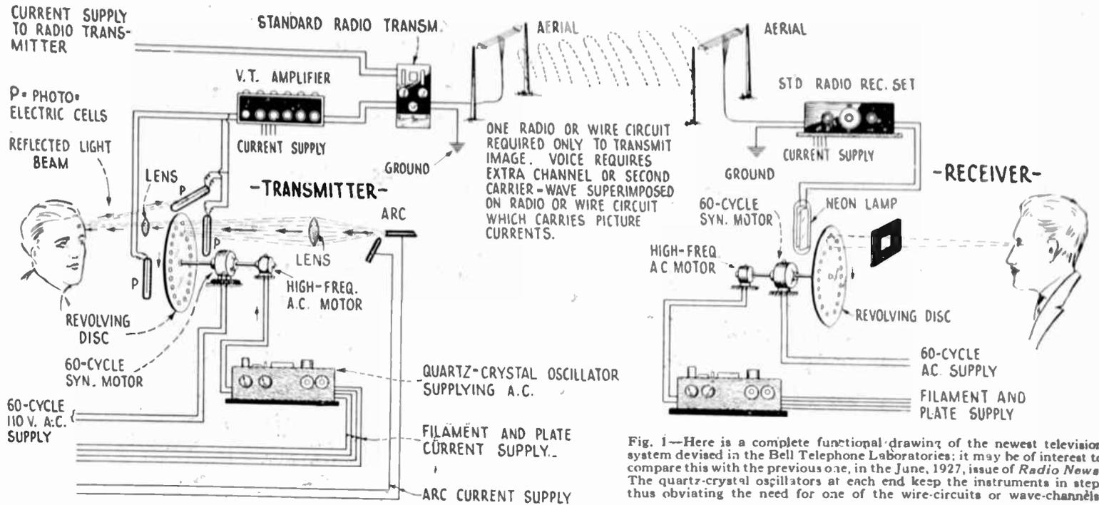
Fig. 1—Here is a complete functional drawing of the newest television system devised in the Bell Telephone Laboratories; it may be of interest to compare this with the previous one, in the June, 1927, issue of *Radio News*. The quartz-crystal oscillators at each end keep the instruments in step, thus obviating the need for one of the wire-circuits or wave-channels.
