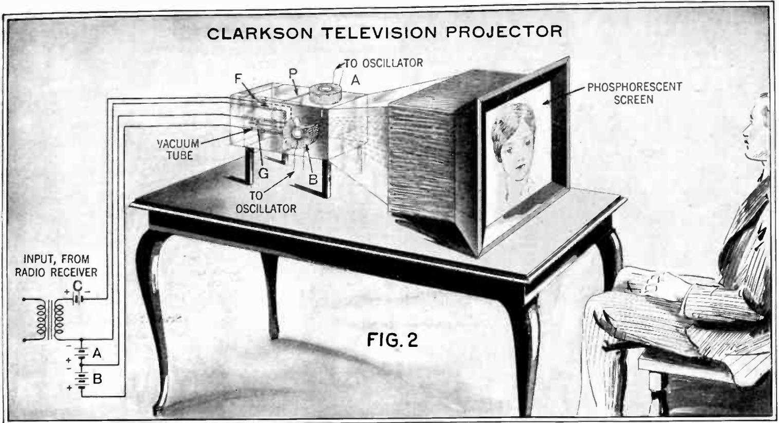
The receiving televisior, similar in construction to the transmitter, makes use of an identical two-element electron-projecting tube. The image will appear on a
