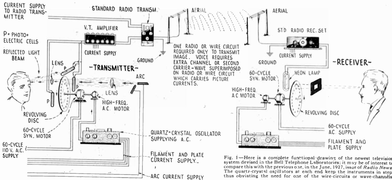
Fig. 1—Here is a complete functional drawing of the newest television system devised in the Bell Telephone Laboratories; it may be of interest to compare this with the previous one, in the June, 1927, issue of *Radio News*. The quartz-crystal oscillators at each end keep the instruments in step, thus obviating the need for one of the wire-circuits or wave-channels.
