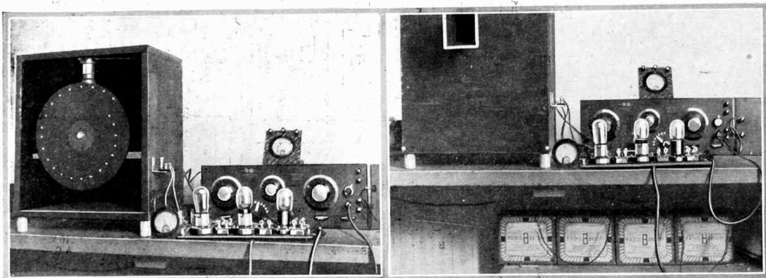
Here we see the disc cabinet at left with cover removed. The neon tube can be seen directly behind the disc. The amplifier appears at right.
