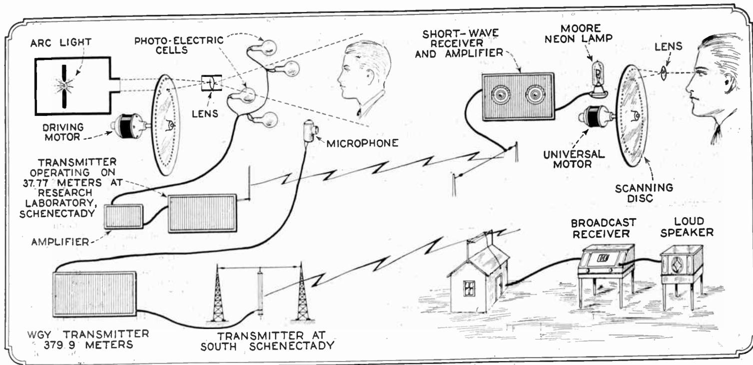
A diagram of the Alexanderson method of operation in the transmission and reception of television. At the upper left are the transmitter for the image and
