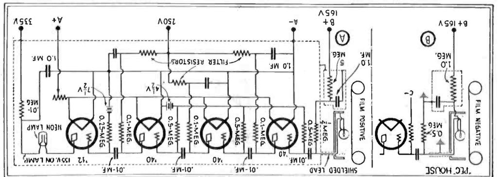
The electrical circuit of the home television projector and receiver described here; the phase-shifter is connected as shown at the left (B) for use with negative films; as at the right (A) with positives. It is the resistor and condenser shown in the grounded shield (dotted lines).
