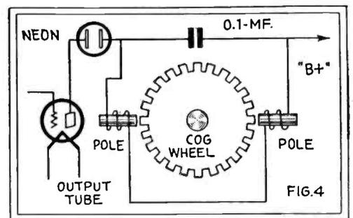
*Here we have the synchronizing regulator at the receiver, which is placed in series with the glow lamp, and responds to the strongest component of the signal.*
