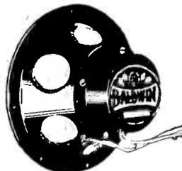
The ideal speaker for cabinet installation. Baldwin Quality — built to Baldwin high standards, which have been responsible for Baldwin world wide leadership—Superior tone quality. Diameter 9 inches, depth 7 inches. Field resistance of 2,500 ohms. This dynamic speaker can be used with A.C. Receivers that are equipped to supply the "B" current to speaker field.
