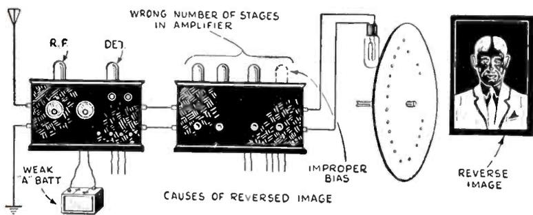
A negative image appearing on your television receiver may be caused by improper number of amplifier stages, wrong bias on power tube, weak "A" battery, etc.
