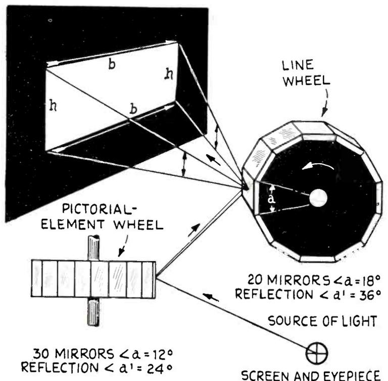
Fig. 3. Source of light—pictorial element wheel—line wheel—projection.
