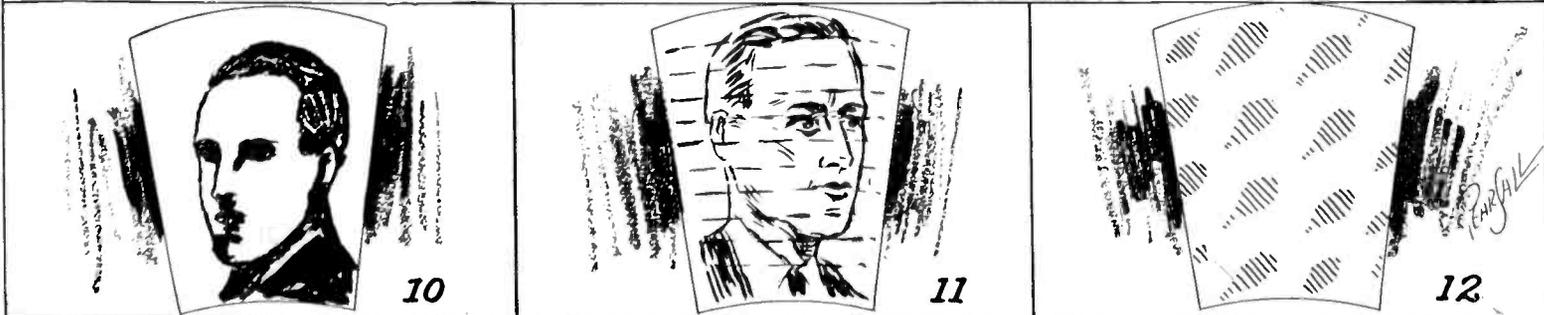
**10. NO DETAIL—PICTURE TOO CONTRASTING**—Cause: Lack of high frequencies in receiver. (a) Improper bias on audio tubes. (b) Improper detector circuit. (c) Regeneration. (d) Radio circuits too sharply tuned. Remedy: Find cause and correct. (a) Proper grid bias. (b) Proper detector circuit. (c) Eliminate regeneration. (d) Broaden radio circuits.
