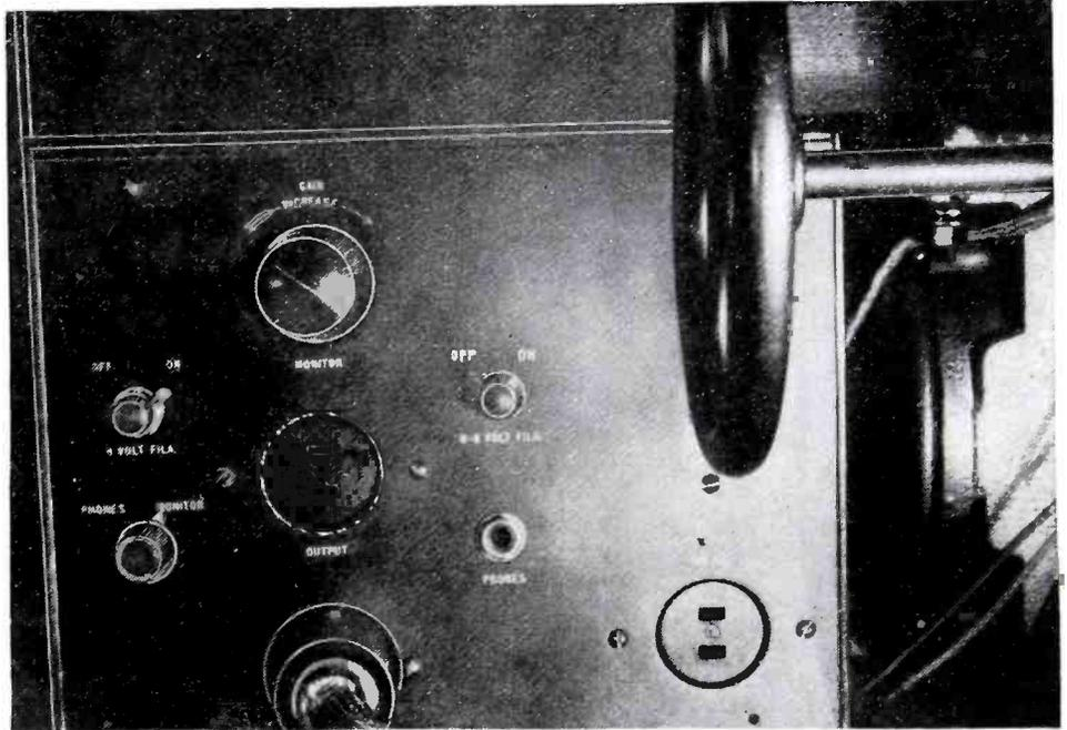
Some of the details which the television cameraman must care for: a close-up of the control board of the latest Jenkins television camera.
