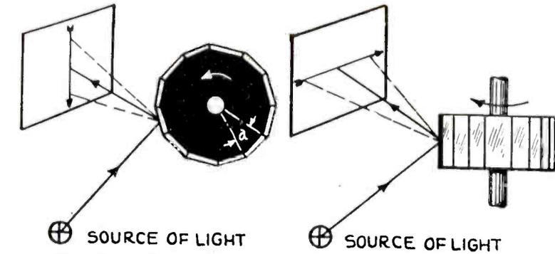
Fig. 1 (right). Horizontal or pictorial element scanning.
