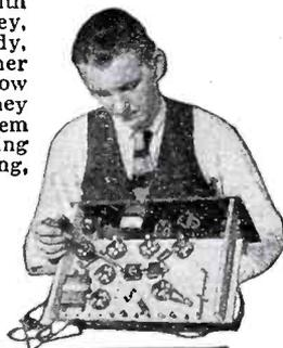
Back view of 5 tube Screen Grid A. C. tuned Radio frequency set—only one of many circuits you can build with my outfits.
