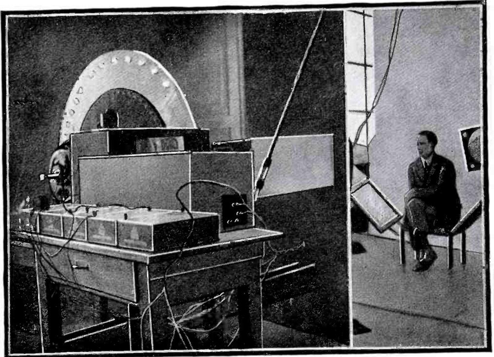
*The set-up of the Mihaly televisior for scanning subjects by natural daylight. Mirrors help to illuminate the subject properly; and a powerful lens concentrates the image upon the large scanning disc, which is placed in a dark room.*
