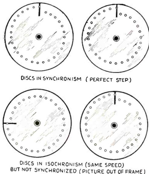
The illustration above shows that while you may have transmitter and receiver scanning discs revolving in step, the picture may still be out of frame.
