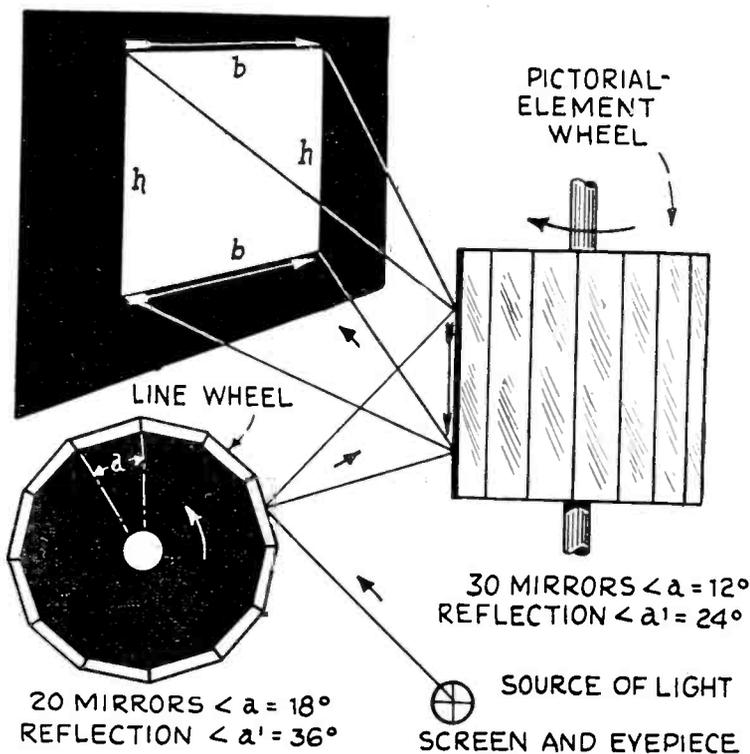
Fig. 4. Source of light—line wheel—pictorial element wheel—projection.
