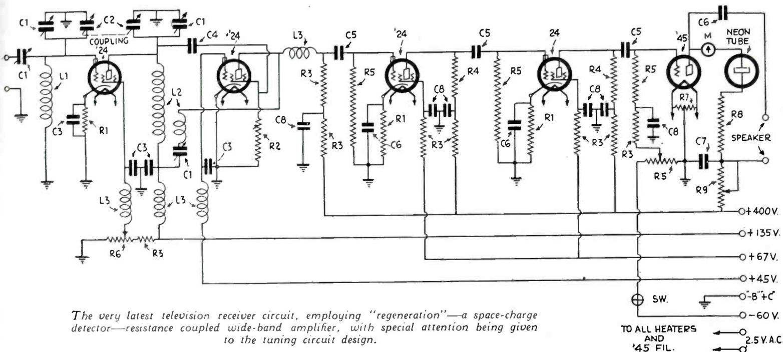
The very latest television receiver circuit, employing "regeneration"—a space-charge detector—resistance coupled wide-band amplifier, with special attention being given to the tuning circuit design.
