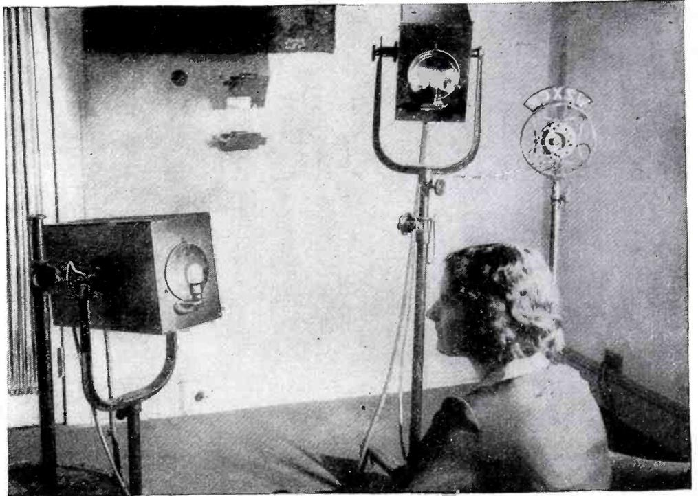
Direct pick-up equipment in Studio of Station W2XCR. This equipment is to be installed in a more favorable location to serve metropolitan New York. Note photo tube pick-up stands. These are made portable for maximum pick-up adjustment.
