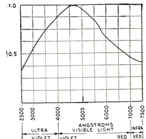
Fig. 3. Curve showing relative sensitivity of a certain photo-cell to different colors.
