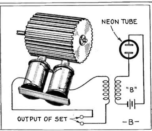
The Baird method, it is explained, differs in the use of the synchronizing impulse to actuate, not a phonic wheel (which is a true synchronous motor) but a speed controller which regulates the actual driving motor. This controller is a "cogwheel," built up of thin laminations of mild steel in later models, and cut with thirty equally-spaced teeth, one for each hole in the disc. This cogwheel is connected in series with the output of the television
