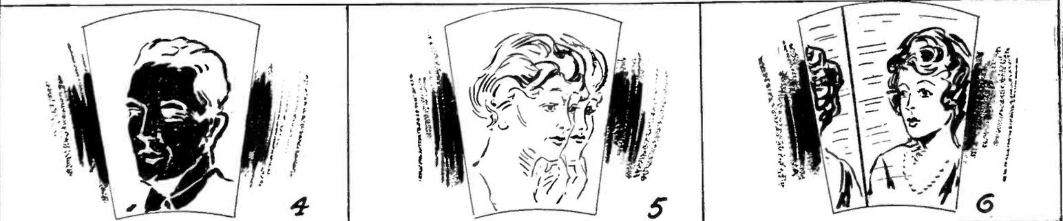
**4. REVERSED OR "NEGATIVE" IMAGE**—Cause: Output signal 180 electrical degrees out of phase, namely, positive impulse causes "decrease" of output plate current, instead of "increase". Remedy: Best to add or subtract one audio stage of resistance coupling. Another method is to change the type of detection from condenser grid-leak to grid bias type, or vice versa.
