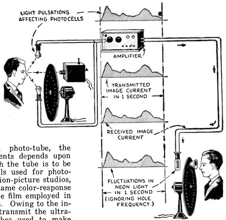
In designing a photo-tube, the choice of the elements depends upon the service in which the tube is to be used. In those cells used for photometric work in motion-picture studios, the cells have the same color-response characteristic as the film employed in making the pictures. Owing to the inability of glass to transmit the ultra-violet rays, the tubes used to make
