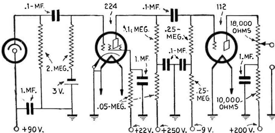
Fig. 5. Typical television amplifier for use with photo-cell.
