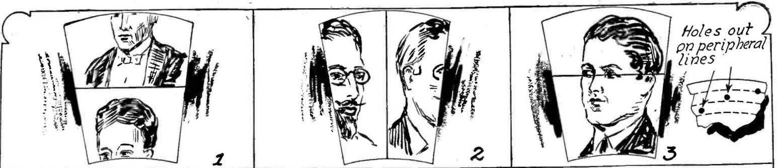
**1. OUT-OF-FRAME VERTICALLY**—Cause: Receiving scanning mechanism out of phase with transmitting scanner. Remedy: If using a synchronous motor stop and start motor until phase relation is same, as evidenced by the vertical centering of the picture. If using a double spiral disc shift lamp until image is centered.
