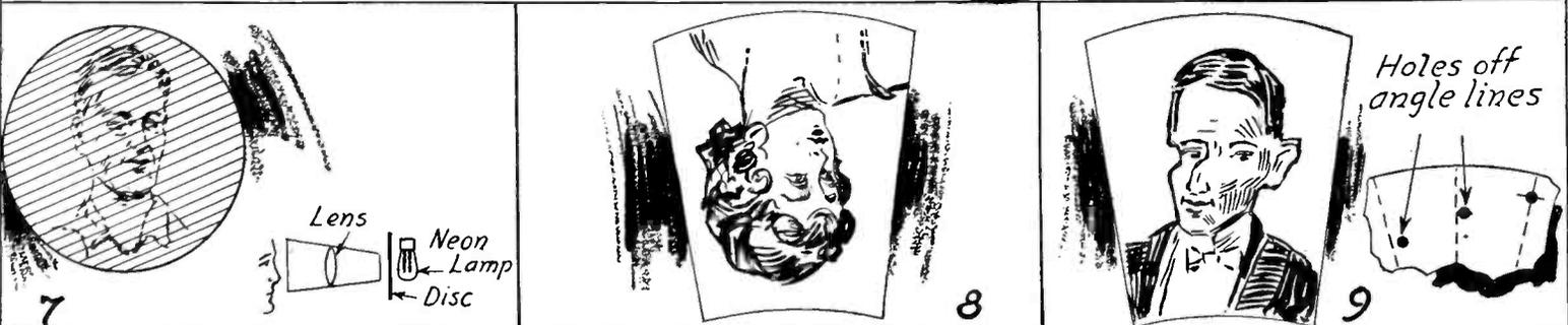
**7. DIM IMAGE**—Cause: (a) Insufficient signal strength. (b) Too much current through television lamp. (c) Too much outside light. Remedy: (a) Television signals should be uncomfortably loud on loudspeaker to properly operate television lamp. Use more powerful amplifier. (b) If television lamp is in series with output tube cut down current by increasing grid bias or reducing plate voltage, or inserting resistance in plate circuit. (c) Darken room.
