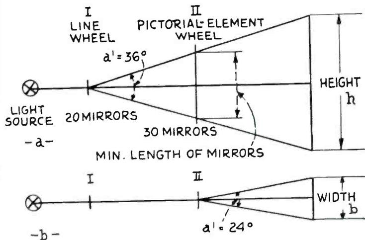
wheel,  $Av$  the number of mirrors of the vertical wheel. If we assume the horizontal wheel to have 30 mirrors and the vertical wheel 20, then with thirty-line scanning we get a ratio of 1:0.05. At the rate of  $12\frac{1}{2}$  pictures a second, that gives a ratio of 750:37.5.
