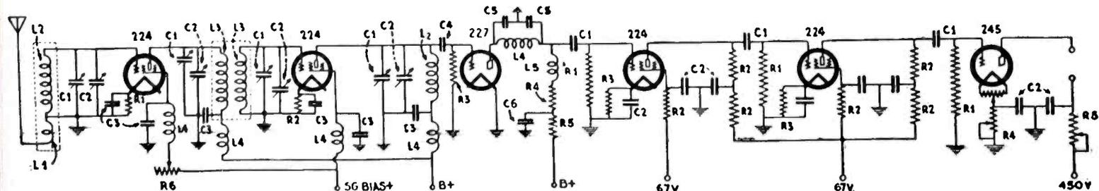
Radiovision receiver with band-pass filter, and 15 to 30,000 cycle radiovision amplifier—L1, 24 turns No. 32 DCC, 1 in. diameter; L2, 48 turns No. 32 DCC, 1 in. diameter; L3, 48 turns No. 32 DCC, 1 in. diameter (ends together); L4, R. F. choke; L5, 20-100 mh. choke; C1, .00015-mf. gang condenser (shielded); C2, trimmer condensers; C3, .01 mf. radio frequency by pass condenser;
