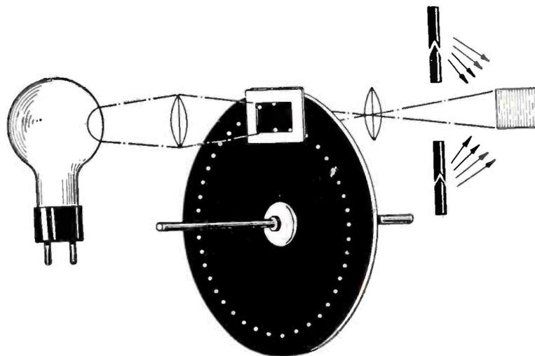
Fig. 2, at left, illustrates how the object (transmitted) is illuminated by light from say two sources; the reflected light beams are transmitted through the lens, scanning disc, diaphragm, second lens and on to photo-cell at extreme left. This cell converts the light pulsations into electric current variations.
