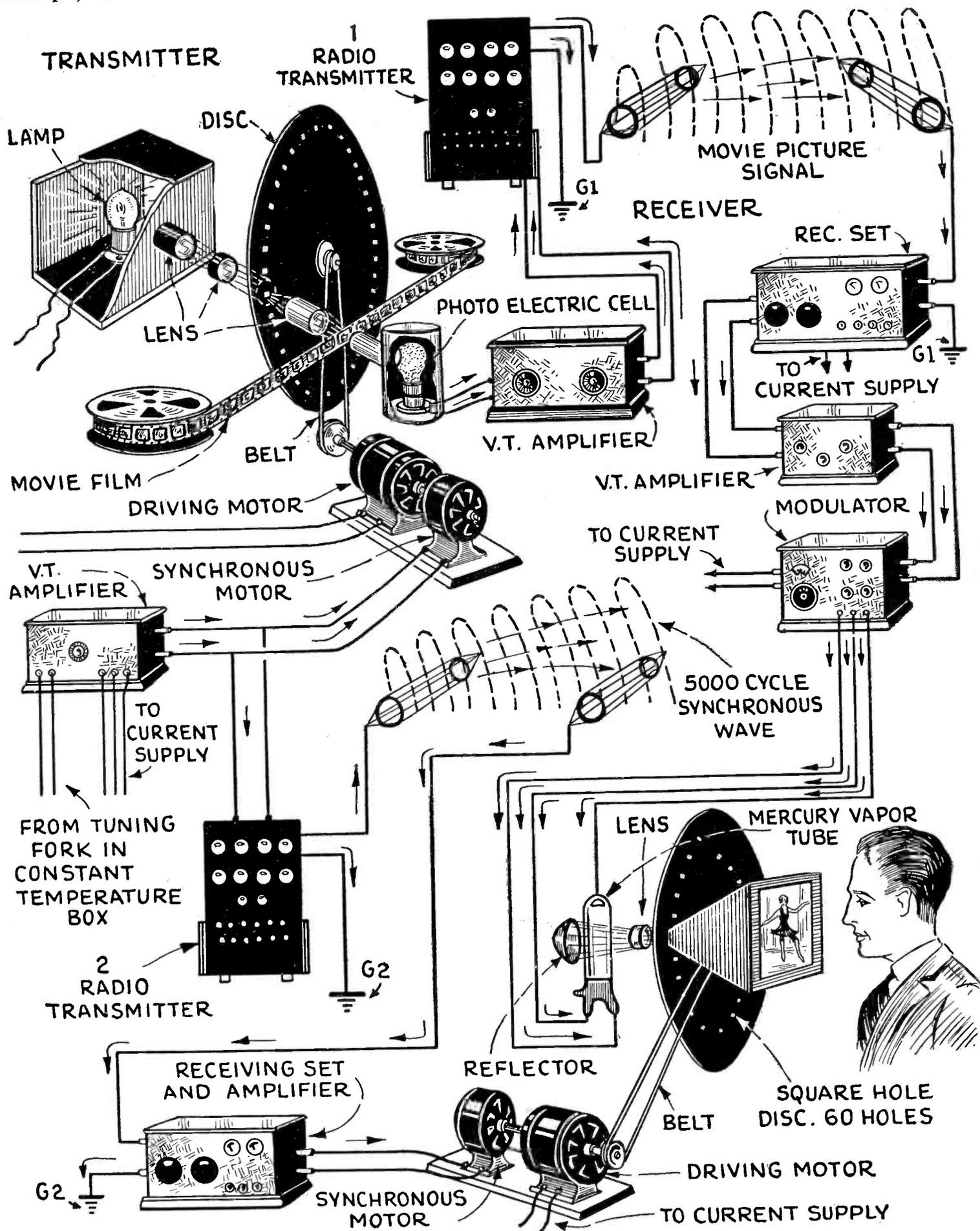
The Westinghouse television "movie" pick-up is shown at top of Diagram, while method of reproducing the movies is shown in lower right-hand corner of diagram. The transmitting and receiving scan-
