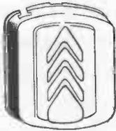
Cover to protect mechanism of the bell from dust and injury
