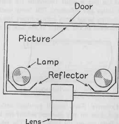
FIG. 199. — Top view of the reflectoscope with the cover removed to show the interior arrangement of the lamps and reflectors.
