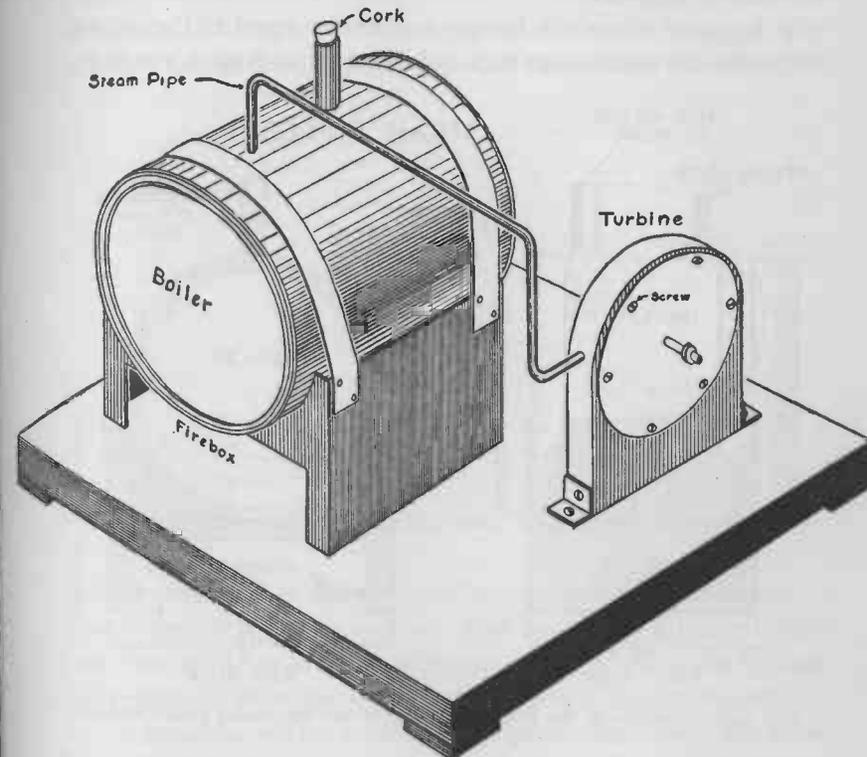
FIG. 146. — The model steam turbine and boiler.
