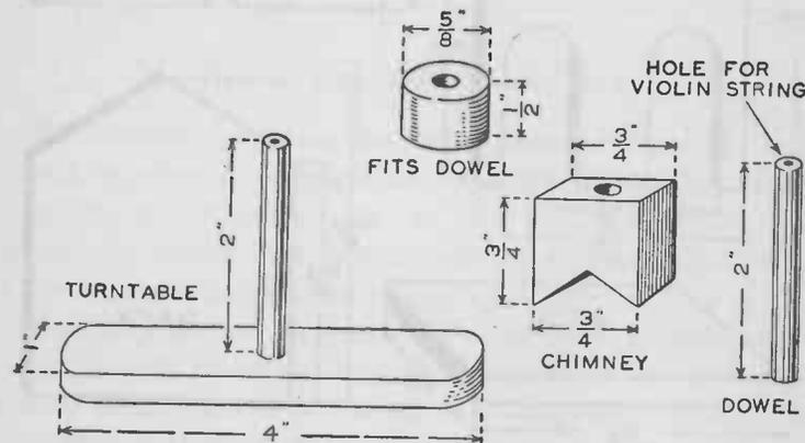
FIG. 280. — Details of the chimney and turntable for the cottage.
