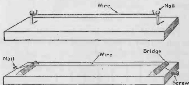
FIG. 121.—At the top is a simple sonometer and below a more elaborate form provided with bridges and tension screw.
