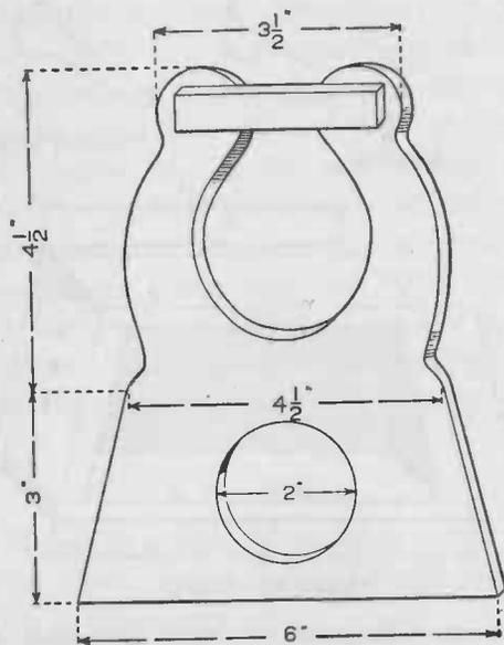
FIG. 124. — The sounding board which closes the front of the box is a lyre-shaped piece of wood as shown in the sketch above.
