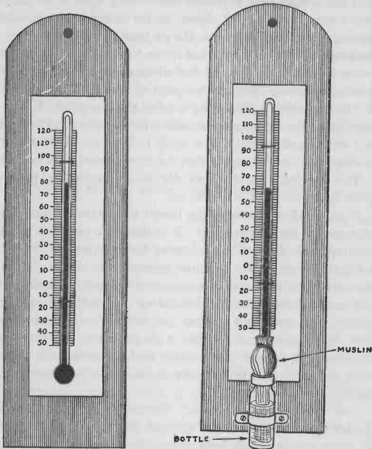
FIG. 278. — An ordinary Fahrenheit thermometer is shown at the left and at the right, the same thermometer converted into a "wet bulb" thermometer.
