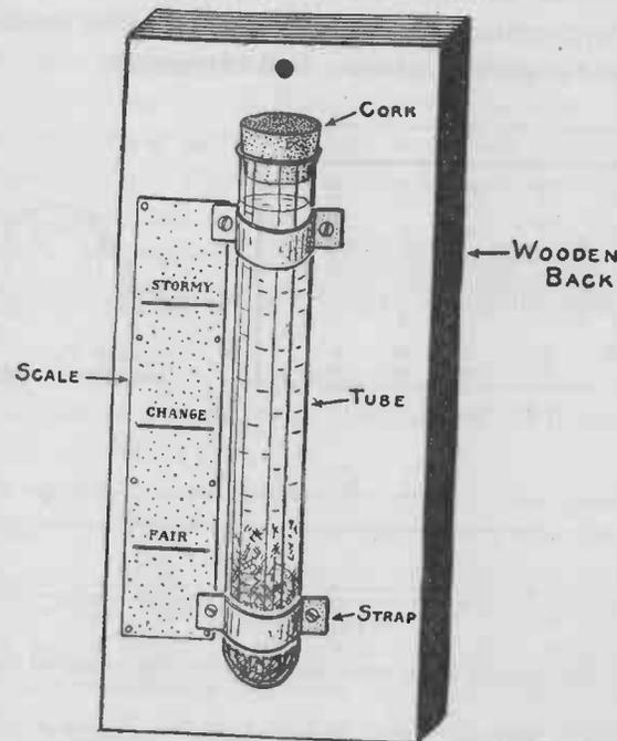
FIG. 287.— The completed weather glass.
