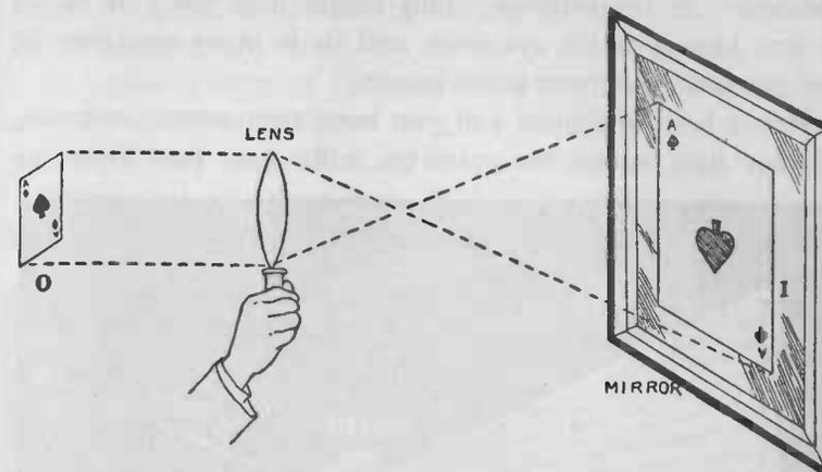
FIG. 168.—Another diagram which shows how a magnifying glass makes objects appear larger than they really are. The dotted lines show the path of the light rays.
