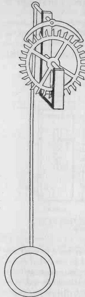
FIG. 57. — A practical use for the pendulum is to regulate clocks. The illustration shows the pendulum and escapement of a clock.
