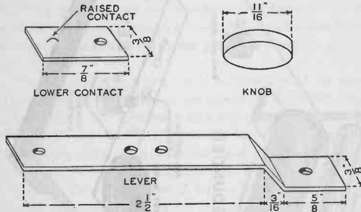
FIG. 238.—The details of the key lever, contact and knob.
