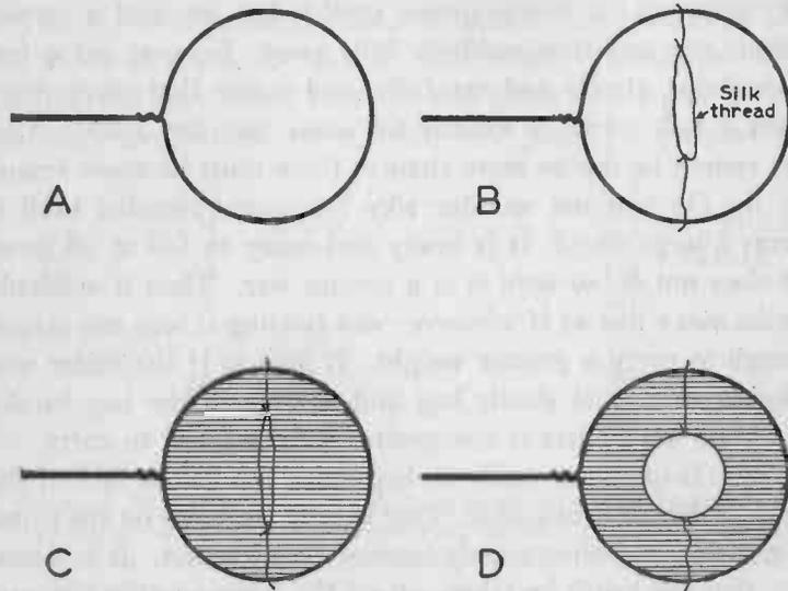
FIG. 75.—The tension of a water film can be shown by a small wire frame (A) with a loop of thread tied across it as at B. Dip the frame in a soap solution so as to form a soap film on the frame as at C. If the film is broken inside the loop by means of a hot wire, the tension of the film will pull the thread into a circle.
