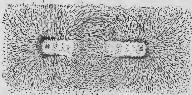
FIG. 214. — The "phantom" of a bar magnet.
