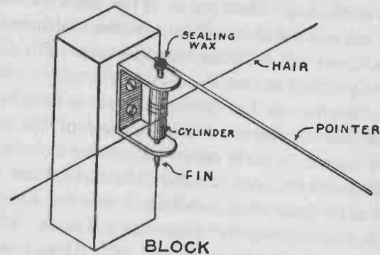
FIG. 277. — This sketch shows how the parts of the hygroscope are assembled.
