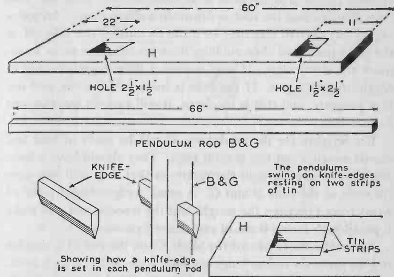
FIG. 59. — Details of the table, pendulum rod for the pen arm and the knife edges used on the harmonograph are shown above.
