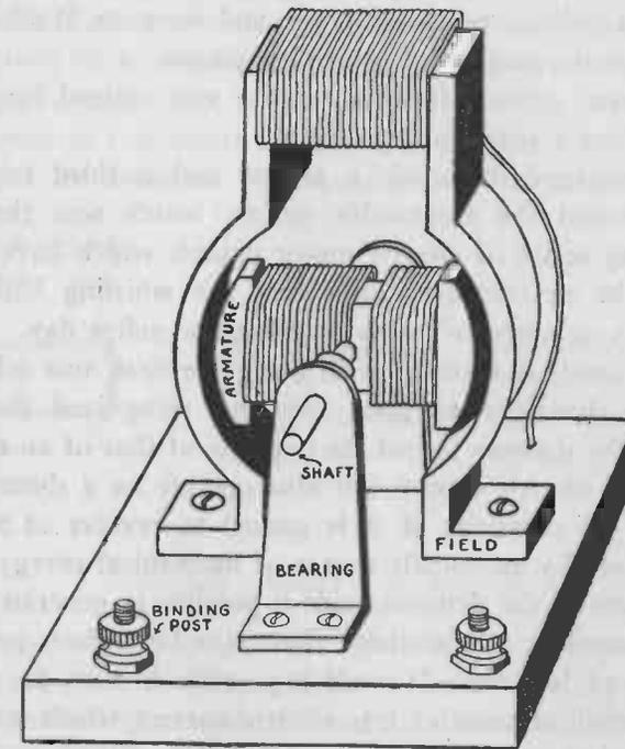
FIG. 233. — A small electric motor which you can build.
