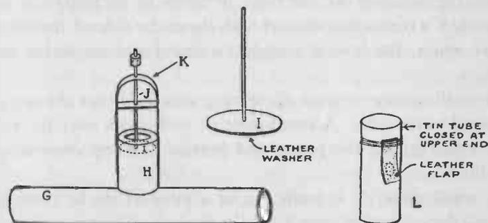
FIG. 108. — The sketch at the left shows the details of the spindle valve for the hydraulic ram. At the right is illustrated the valve L which prevents the water that is pumped upwards into the bottle from flowing back again.
