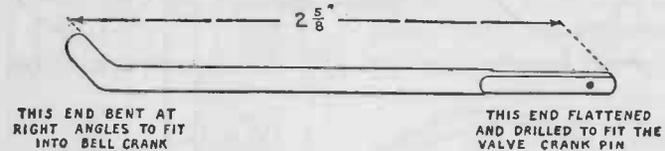
FIG. 155. — The valve rod.
