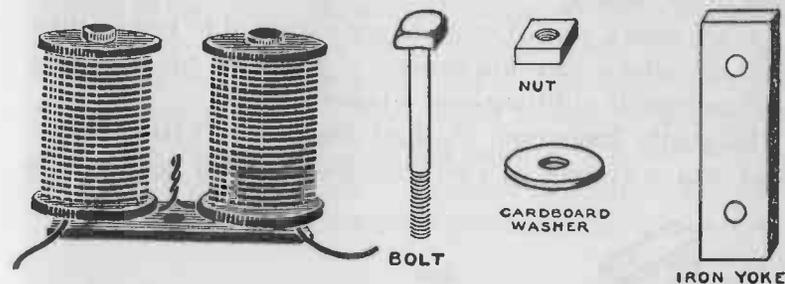
FIG. 227. — At the left is a horseshoe electromagnet. The parts for making a horseshoe electromagnet are also illustrated.
