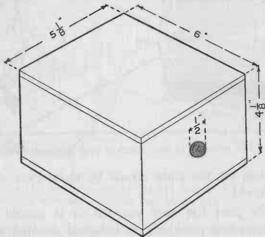
FIG. 179. — The box of the pinhole camera viewed from the front. The copper disk bearing the pinhole is placed over the hole in the front of the box.
