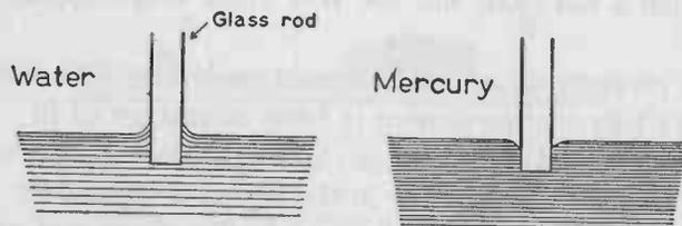
FIG. 77.— Water wets glass. The surface of water rises to meet a glass rod dipped into it. Mercury does not wet glass. A glass rod dipped into mercury depresses the surface.
