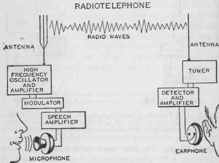
FIG. 246.—The Principle of Radiotelephony.
