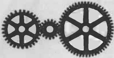
FIG. 46. — Gears are wheels whose motion is transmitted from one to another by means of teeth around their circumference.
