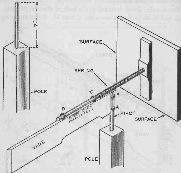
FIG. 274.—The pivot upon which the wind pressure gauge swings is an iron rod set into the top of a pole.
