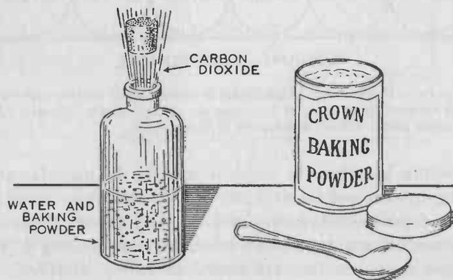
FIG. 20. — Put about one-half teaspoonful of baking powder in a small bottle and add a little water. Carbon dioxide will be generated so rapidly that if you put the cork in the bottle, it will be blown out again with a loud pop.
