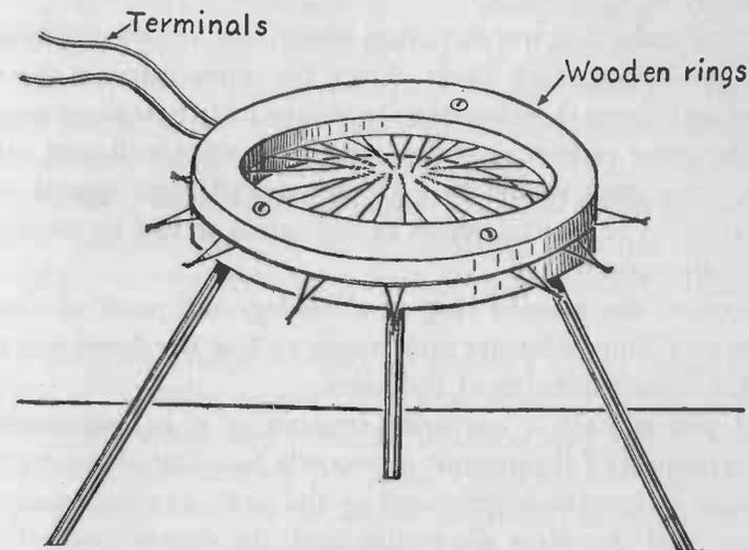
FIG. 144.—Complete thermopile. An alcohol lamp should be placed underneath the thermopile so that the flame heats the inside ends of the wires in the center of the wooden ring.
