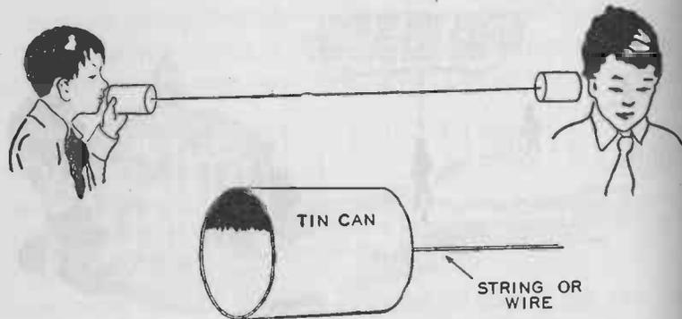
FIG. 112. — The tin can telephone is an illustration of how sound waves may be transmitted through a wire or string.
