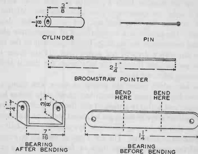
FIG. 276. — These details of the hygroscope are explained in the text.
