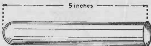
FIG. 285.—The test-tube used in making the weather glass.
