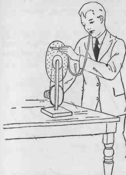
FIG. 113. — A simple siren wheel. If you blow through the holes in the revolving disk, a sound having the character of a musical note will be produced. Changing the speed of the disk will change the pitch of the note.
