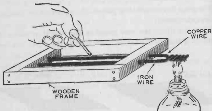
FIG. 137. — A simple apparatus for showing the relative heat-conducting power of iron and copper. A match may be ignited on the copper wire at a much greater distance from the flame than it can on the iron wire.
