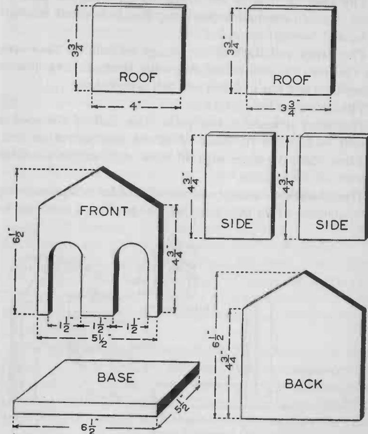
FIG. 279. — The wooden pieces which make up the weather cottage.
