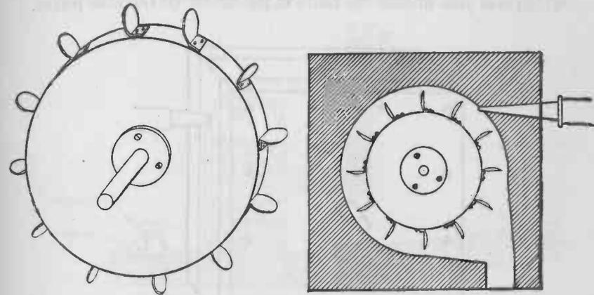
FIG. 104. — The completed wheel with the buckets and shaft in place is shown at the left. Alongside it is the motor with one side piece removed to show the position of the wheel and the nozzle.
