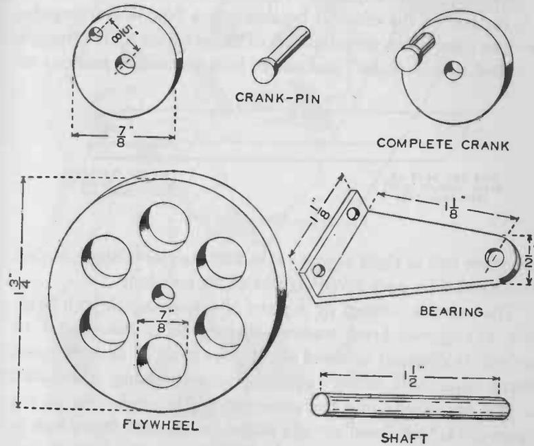
FIG. 154.—Details of the flywheel, crank, shaft and bearings.
