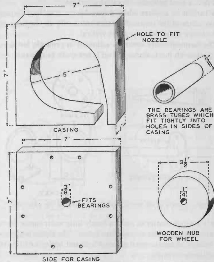
FIG. 102. — These parts for the water motor are easy to make. The casing and the sides for the casing are made of wood.
