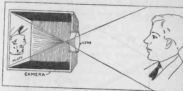
FIG. 178. — The principle of the camera is very similar to that of the eye.
