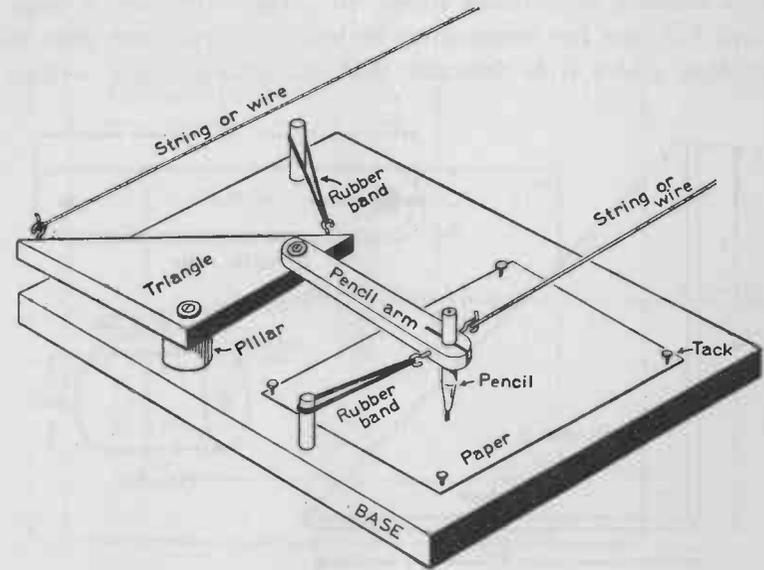
FIG. 51. — A mechanical telautograph like that above will transmit writing and drawing from one room to another.
