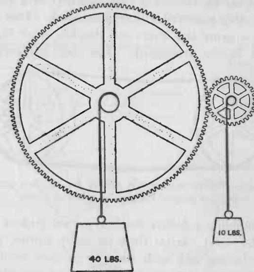
FIG. 47. — Gears are a form of lever. If a small gear is meshed with another gear four times its diameter, the small gear will revolve four times to each revolution of the large one.
