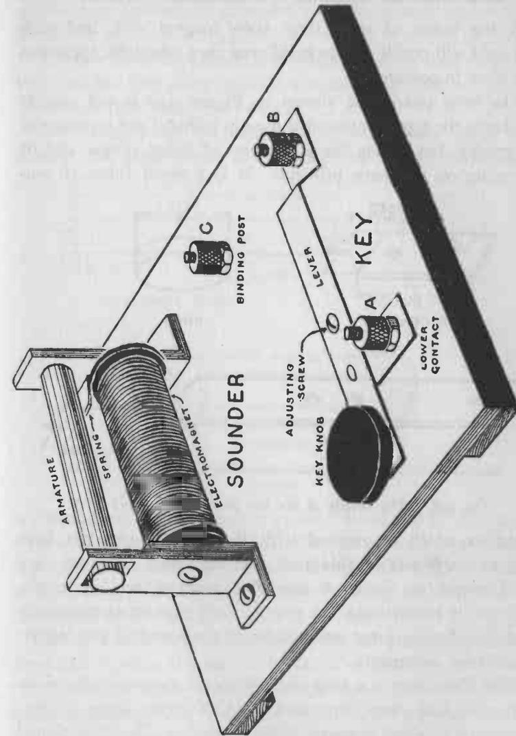
FIG. 237. — A homemade telegraph key and sounder.
