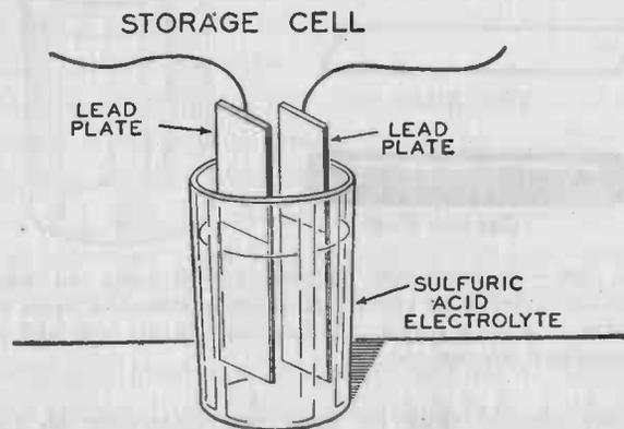
FIG. 221.—An experimental storage cell consisting of two strips of sheet lead immersed in a solution of sulfuric acid in water.
