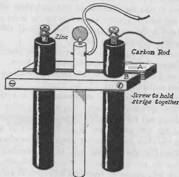
FIG. 219. — The elements of a homemade Voltaic cell, consisting of two carbon rods and a zinc rod may be clamped between two wooden strips. The strips should be painted with paraffin.
