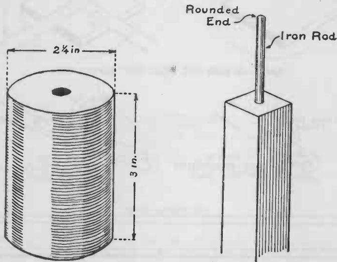
FIG. 271. — The rods and cones are fastened to the wooden cylinder and the cylinder is set upon an iron rod driven into a pole. The upper end of the rod should be rounded.
