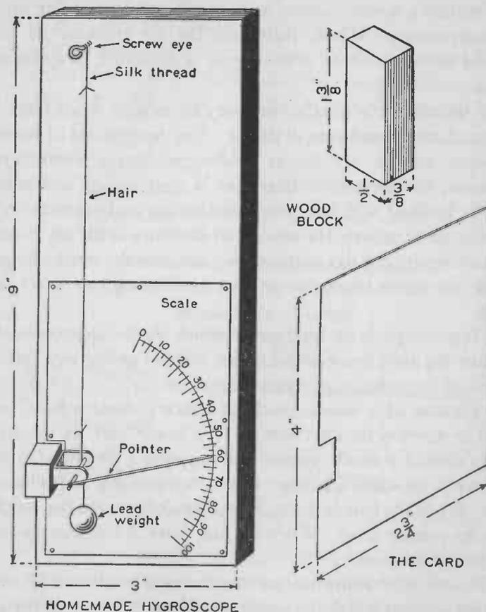
FIG. 275. — A homemade hygroscope for measuring the moisture in the air. For further details see Figure 276.
