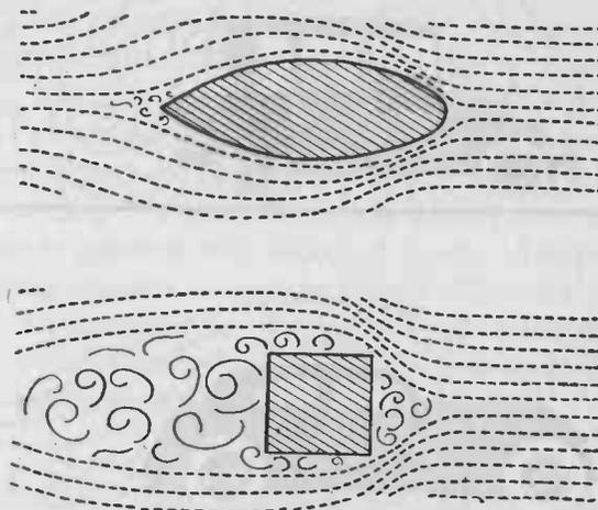
FIG. 71. — The dotted lines represent streams of air slipping past a square object and a streamlined form. Notice the turbulence or "air-hole" stirred up in the wake of the square object. The streamlined object is more easily pushed through the air because it creates less disturbance in its passage.
