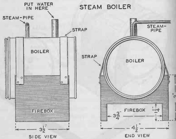
FIG. 147. — Details of the firebox and boiler for the model steam turbine.
