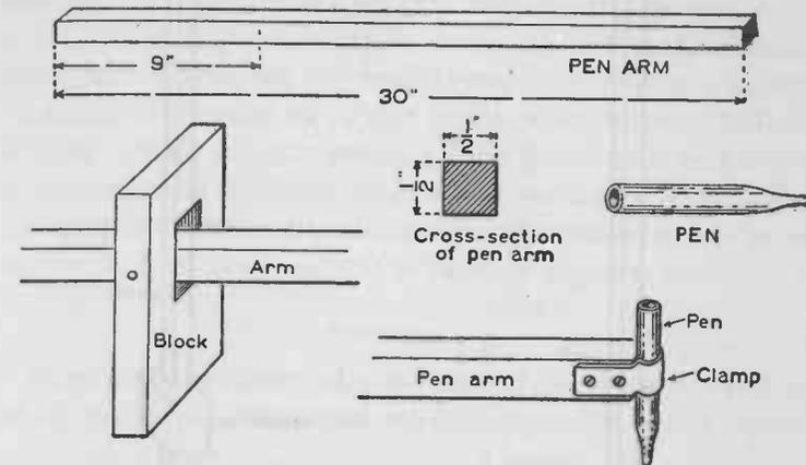
FIG. 60. — The pen is made from a piece of glass tubing. It is clamped on the end of the arm and the arm is supported in the block.
