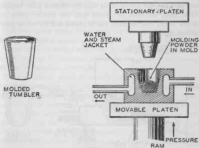
FIG. 33B.—Molding a Thermosetting Plastic. Heat and heavy pressure, the latter supplied by a hydraulic press, are required. The mold is for making the molded tumbler shown at the left. The portion of the mold called the cavity is shown in section.
