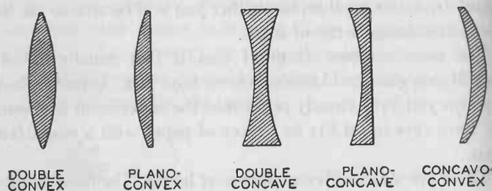
FIG. 165.—Cross-sections of the most common forms of lenses.
