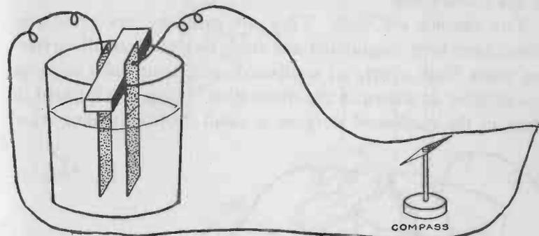
FIG. 223.—Oersted's famous experiment by means of which he discovered that an electric current will produce magnetism.
