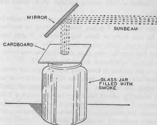
FIG. 160.—A simple method of showing how light is reflected and diffused by the millions of little particles in a jar of smoke.
