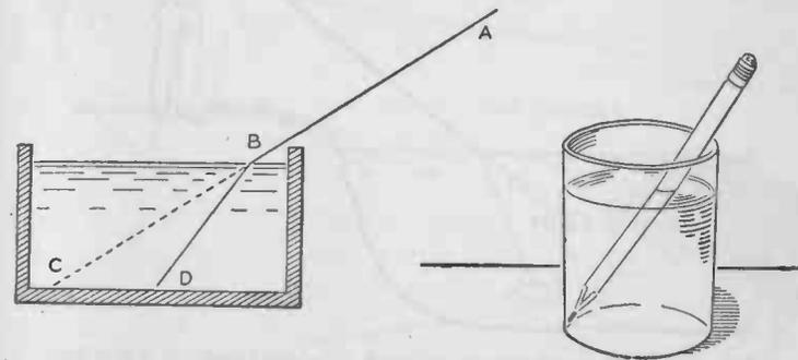
FIG. 161.—The diagram at the left represents a beam of light (AB) striking the surface of a tank of water. Since light tends to travel in a straight line it should continue in the direction shown by the dotted line BC. It is however really bent or refracted by the water and actually travels from B to D.
