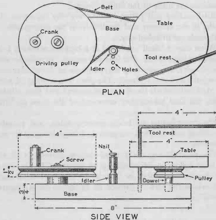
FIG. 30.—Plans for a small potter's wheel which can be used for shaping clay.
