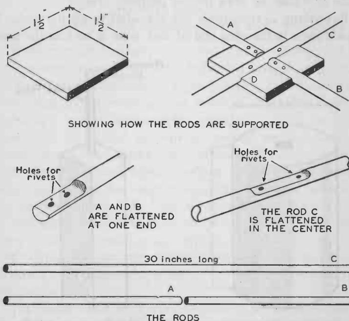
FIG. 270.—Details of some of the metal parts of the anemometer.
