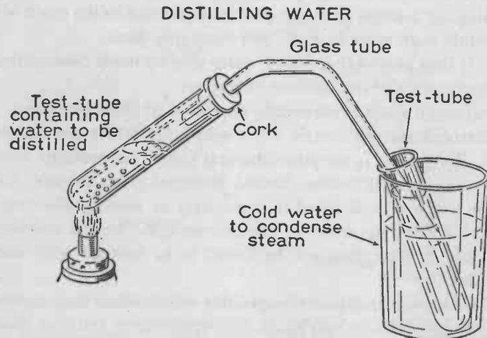
FIG. 12.— A simple distilling apparatus. Steam formed by boiling water in the left hand test-tube passes through the glass tube and is condensed into pure distilled water in the right hand tube.
