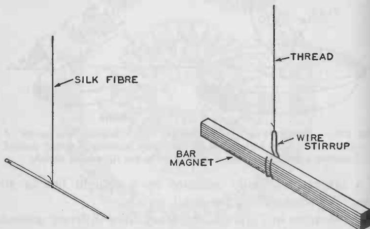
FIG. 213. — Two methods of making simple compasses by suspending bar magnets from threads. The bar magnet at the left is a magnetised sewing-needle.
