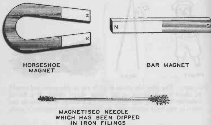
FIG. 208. — A common type of horseshoe magnet and a bar magnet. Iron filings will cling to the poles of a magnetised needle.
