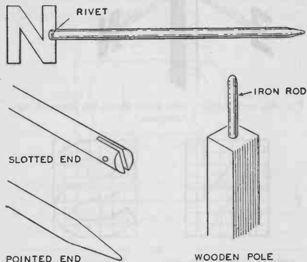
FIG. 267.—One end of each rod is pointed and the other is slotted. The letters are riveted or soldered into the slotted ends of the rods. The vane is set upon an iron rod driven into the top of the pole.
