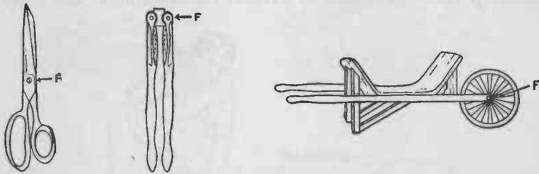
FIG. 41. — A pair of scissors, a nut-cracker and a wheel-barrow are common forms of levers. The fulcrum is located at the point marked F in the illustration.
