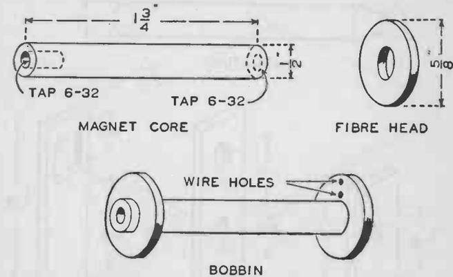
FIG. 239.—The core, magnet head and bobbin for the telegraph sounder.
