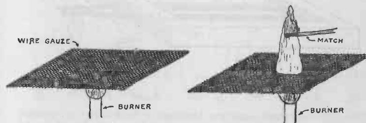
FIG. 136. — If a piece of copper gauze is held in the flame of an alcohol lamp, Bunsen burner or candle, the flame will burn below and not above the gauze, unless a lighted match is held above.
