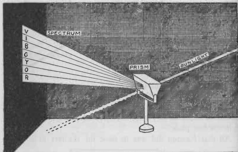
FIG. 170. — If a beam of white sunlight passes through a prism it becomes broken up into a beautiful band of rainbow colors called the spectrum. The dotted line shows the path which the sunbeam would follow if it were not refracted by the prism.
