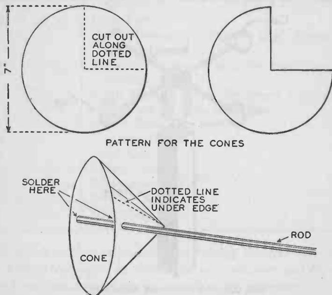
FIG. 269.—The pattern for the cones is a circle with a quadrant cut out as shown. A cone is soldered on each of the four rods.
