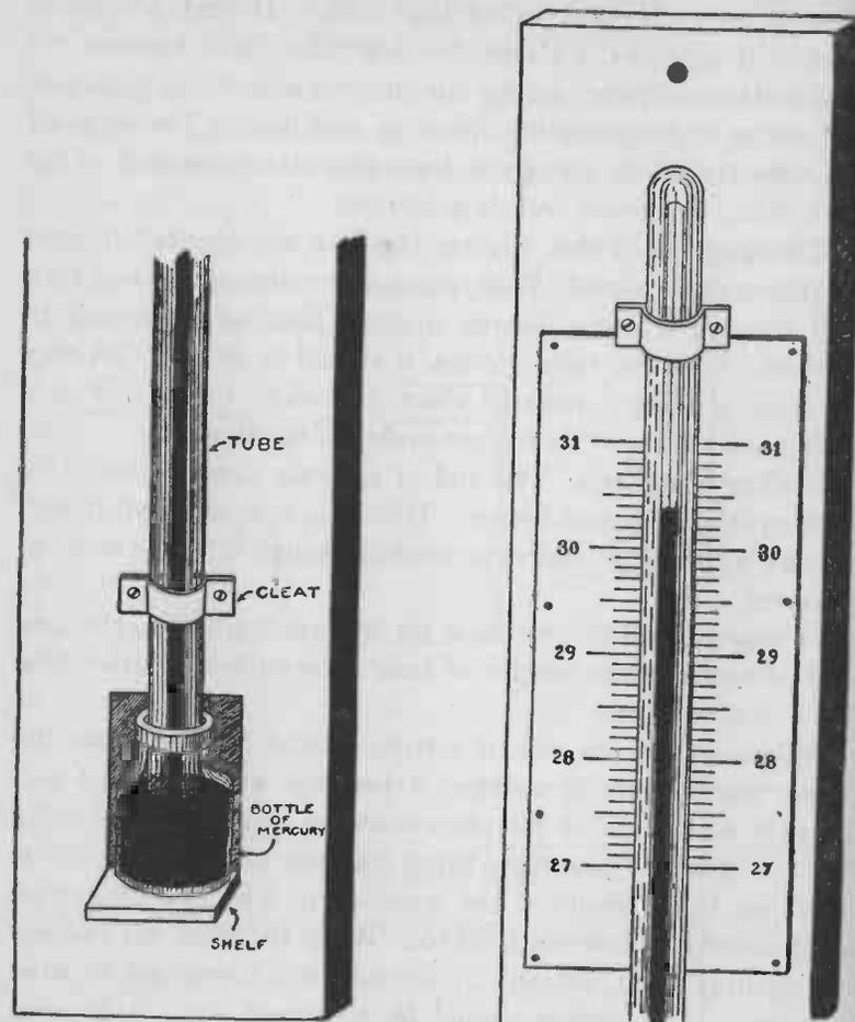
FIG. 289. — At the lower left is shown the lower end of the barometer and at the right, the upper end.
