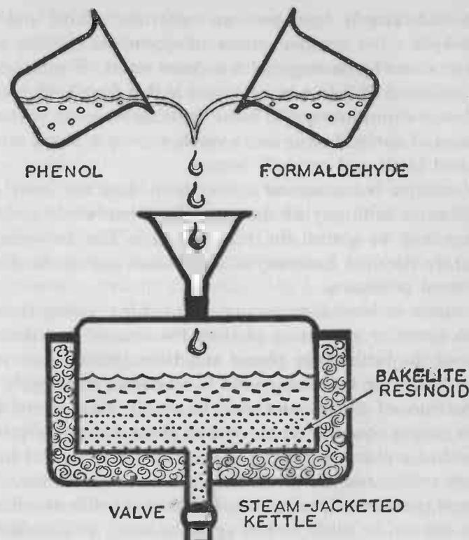
FIG. 33A. — The Bakelite Resinoid Process.
