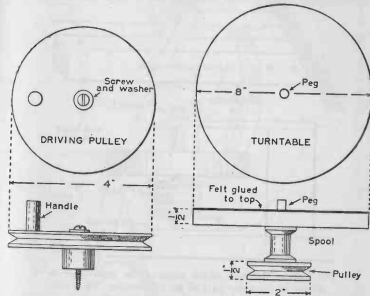
FIG. 129. — Details of the wooden turntable and driving wheel for the phonograph.
