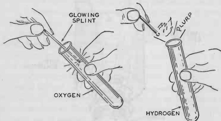
FIG. 11. — If a splinter of wood retaining a glowing spark is immersed in a test-tube containing oxygen, it will instantly burn brilliantly and burst into flame. If a match is held to the mouth of a test-tube containing hydrogen, the gas will burn with a "plurp" sound.
