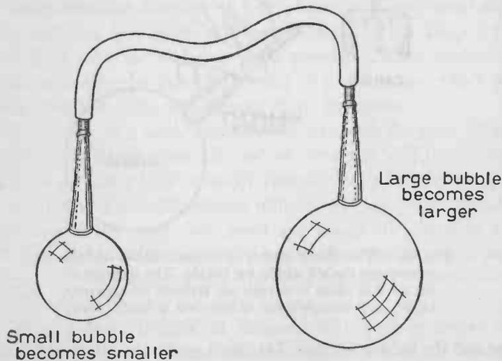
FIG. 85. — Two cigarette-holders and a piece of rubber tubing will enable you to perform an experiment which shows that the air pressure is greater in a small bubble than in a large one.
