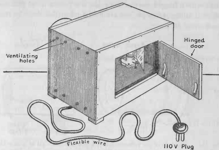
FIG. 198. — Back view of the reflectoscope with the door open.
