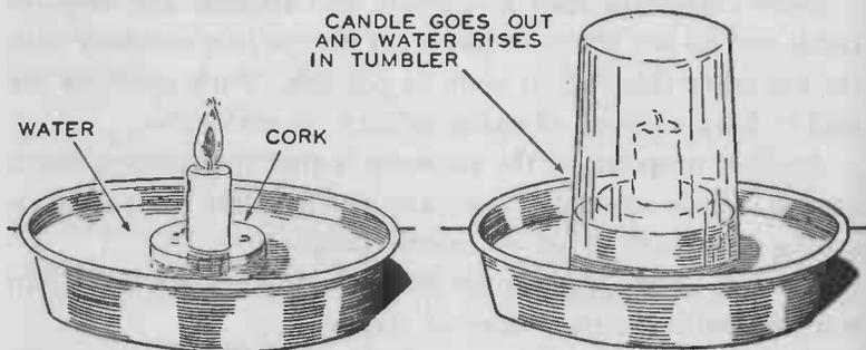
FIG. 9. — This simple apparatus will give a valuable clue regarding the composition of air. The candle will burn for a short time and then go out. The water will rise in the tumbler and there will be much *less* air enclosed in the tumbler.
