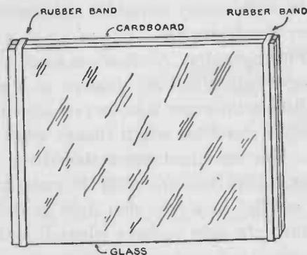
FIG. 175.—A simple printing frame for making photographs.
