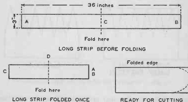
FIG. 282. — The petals of the floral barometer are cut from a long strip of paper folded and trimmed as shown above.
