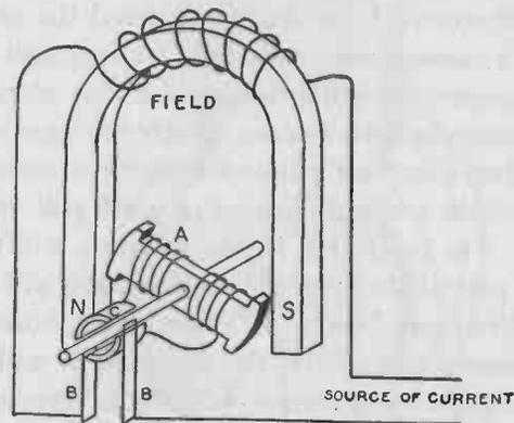
FIG. 232. — The principle of the electric motor is illustrated by this diagram. A is the armature, C is the commutator and BB the two brushes.
