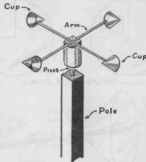
FIG. 268. — A homemade anemometer.
