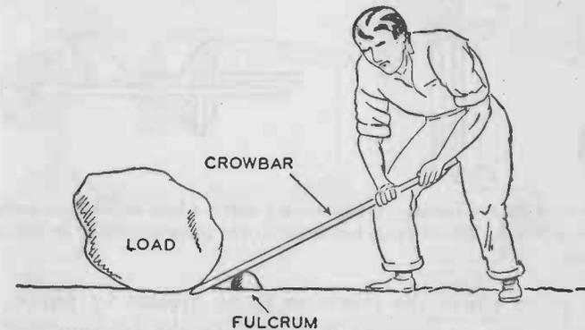
FIG. 40. — The crowbar is one of the most common forms of lever and is used for moving large stones and other heavy objects.
