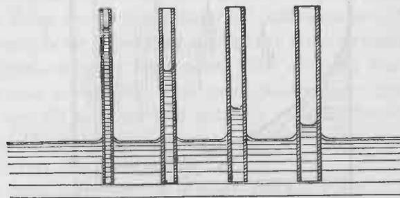
FIG. 78.— Capillary attraction raises water in a tube of small diameter. The water rises to the greatest height in the tube which has the smallest bore.
