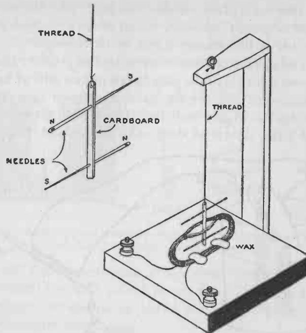
FIG. 225. — A simple form of Astatic galvanoscope which a boy can build.
