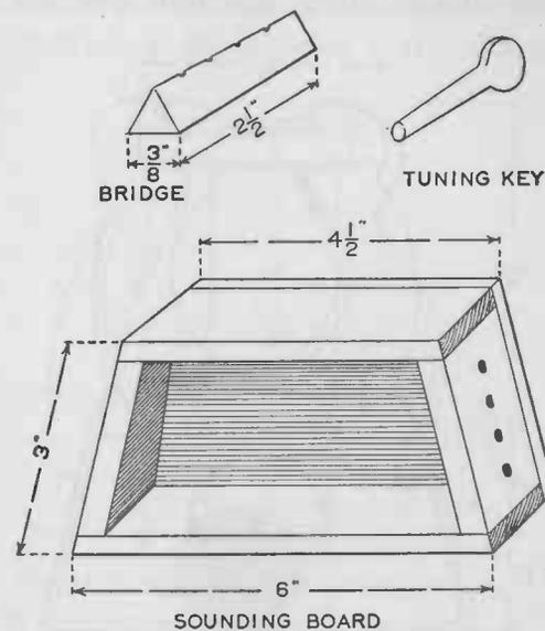
FIG. 123.—The sound box of the door zither is made of wood. At the top are shown the bridge and the tuning key.
