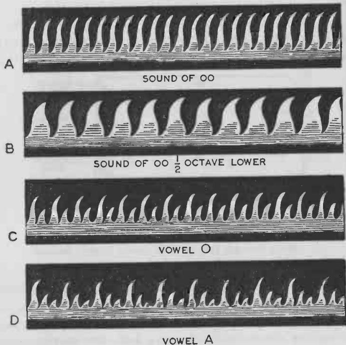
FIG. 120.—The manometric flame produced by the sound OO is shown at the top. The same sound an octave lower is also illustrated. The flames in the two bottom rows were produced by the sounds of the vowels O and A.
