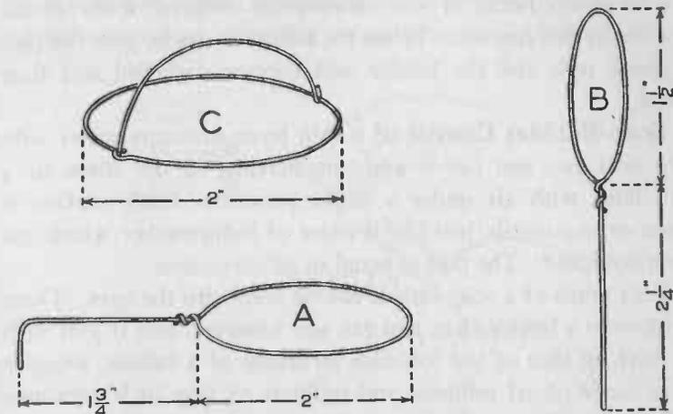
FIG. 83.— Make three or four wire rings like *A*, two like *B* and one like *C* to use in blowing "fancy" bubbles.
