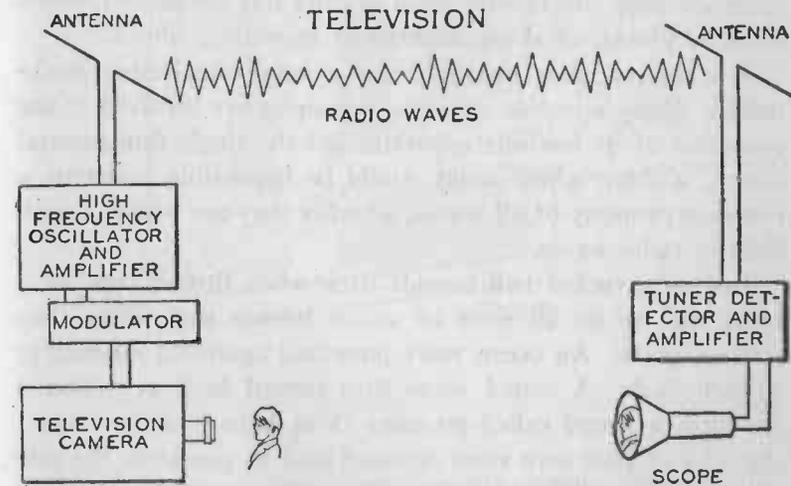
FIG. 247.—The Principle of Television. Notice that a type of antenna different from those shown in Figs. 245 and 246 is shown. The waves used in television are shorter than those commonly used for radio telegraphy and telephony and require a "short-wave antenna."
