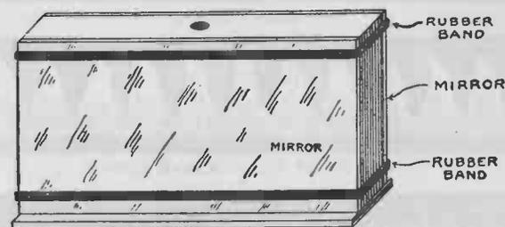
FIG. 119.—The mirrors are cemented to the wooden block with cement or glue. The rubber bands are added for safety sake to prevent the mirror from flying through the air if it should become loosened while rotating.
