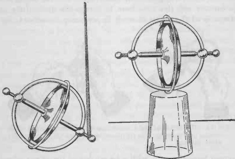
FIG. 65. — At the left a gyroscope is spinning in a loop of string. At the right a gyroscope is shown spinning on its circle on the bottom of a glass tumbler.
