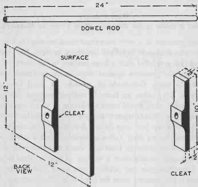
FIG. 272. — Details of the surface for the wind pressure gauge.
