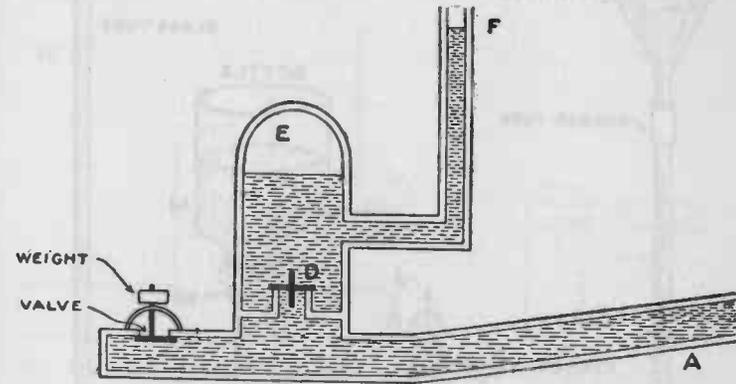
FIG. 106.—Cross-section of a hydraulic ram.
