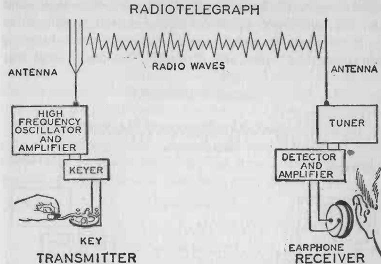
FIG. 245.— The Principle of Radiotelegraphy. By comparing this diagram with Figs. 246 and 247 you will understand that the basic difference between radiotelegraphy, radiotelephony and television lies in the method of modulating or impressing the message on the radio waves.
