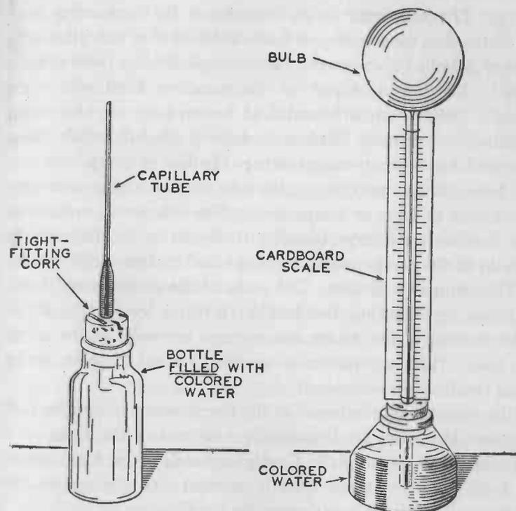
FIG. 142.— The left-hand sketch shows a bottle filled with colored water and provided with a capillary glass tube passing through a tight-fitting cork. At the right is shown an air thermometer.
