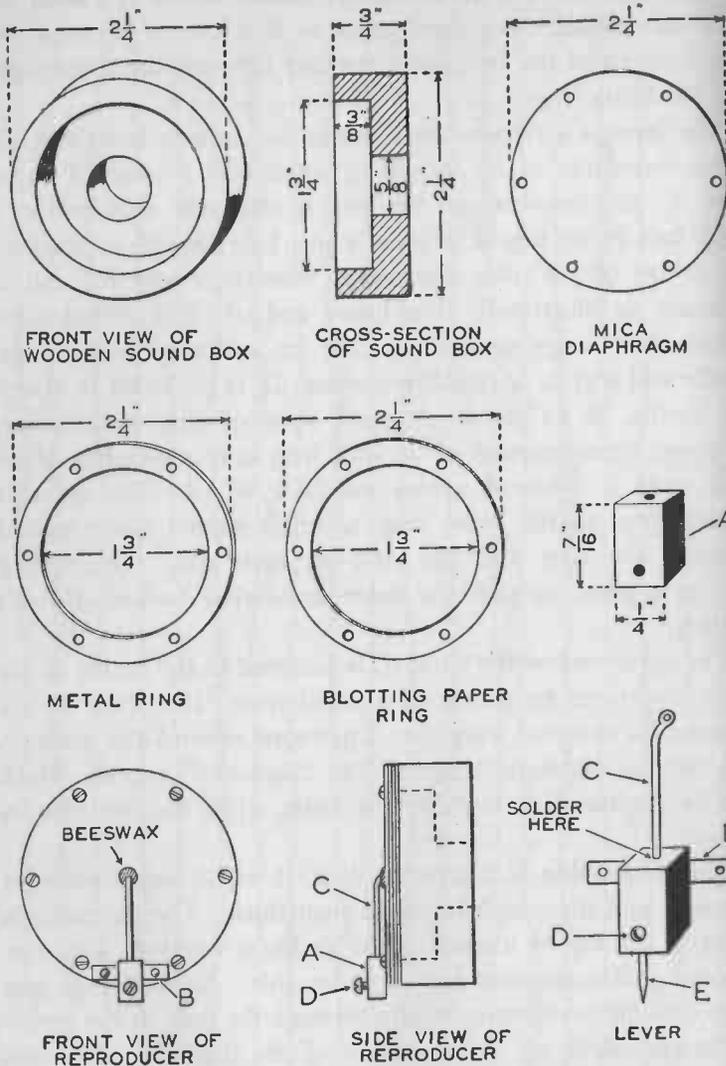
FIG. 128. — Details of the home-made phonograph reproducer.
