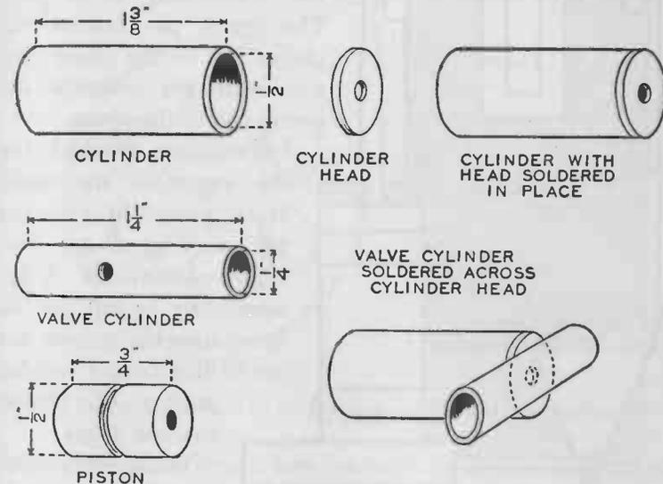
FIG. 152. — Details of the main cylinder, the valve cylinder and the piston.
