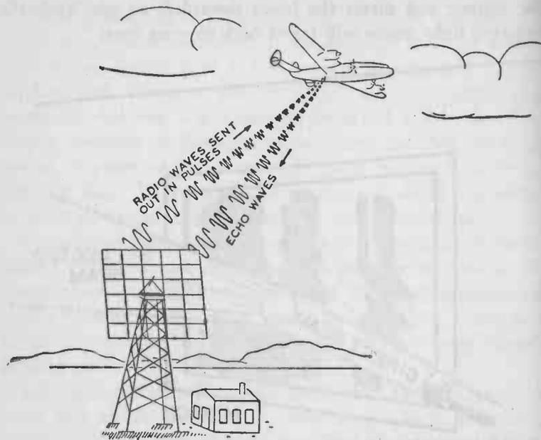
FIG. 249.—The Principle of Radar. Radio waves are sent out in pulses. When they strike an object they are reflected back to the transmitter. Ingenious apparatus locates the reflecting object.
