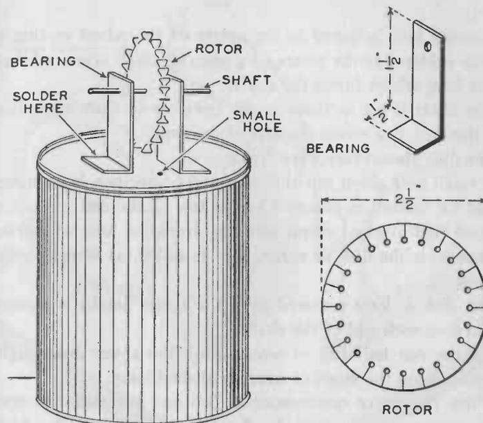
FIG. 145. — A simple steam turbine made from a tin can.
