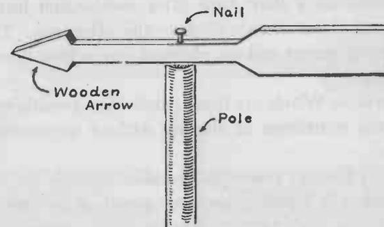
FIG. 262. — A simple wind vane consisting of a wooden arrow pivoted on top of a pole.
