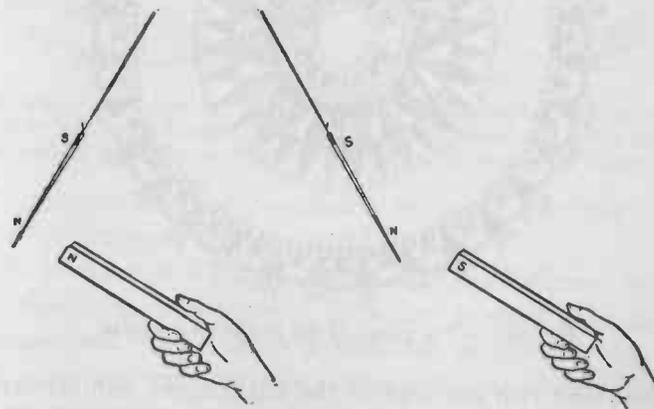
FIG. 210.—An experiment demonstrating that like poles repel and unlike poles attract.
