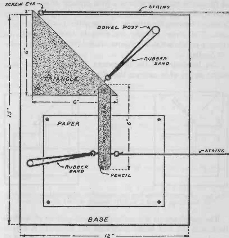
FIG. 53. — Plan of the complete mechanical telautograph.
