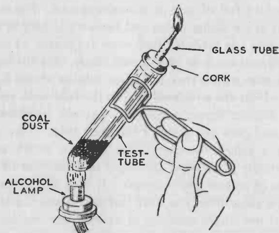
FIG. 25.—An experiment showing how illuminating gas, coke and coal-tar are produced by heating soft coal.
