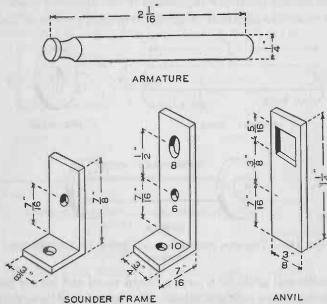
FIG. 240. — The sounder armature and parts of the sounder frame and anvil.
