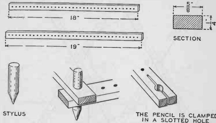
FIG. 49.— Parts of the pantograph.
