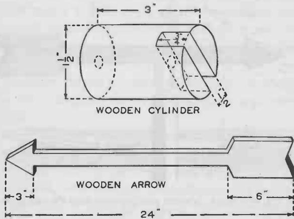
FIG. 264. — Details of the wooden arrow and cylinder for the weather vane.
