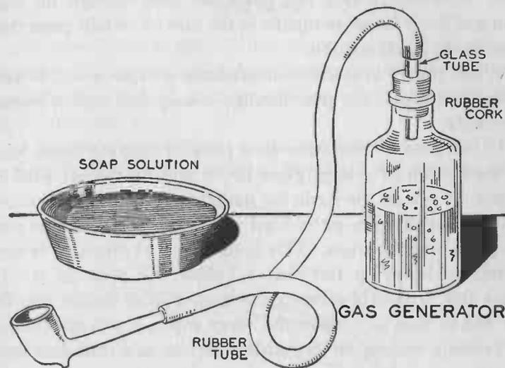
FIG. 87.— Bubbles filled with hydrogen are much lighter than the air which they displace. When released, they will rise like gas-filled balloons. You can fill bubbles with hydrogen by means of a home-made gas generator connected to a bubble pipe.
