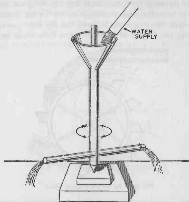
FIG. 98.—Barker's mill is a curious invention which operates on the same principle as Hero's engine but uses water in place of steam. It illustrates the important law of physics that the action and reaction of a force are always equal and opposite.
