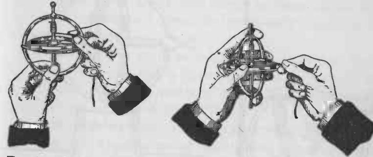
FIG. 64. — The left-hand sketch shows how to hold the gyroscope while winding on the string. The right-hand sketch shows how to start the wheel spinning.
