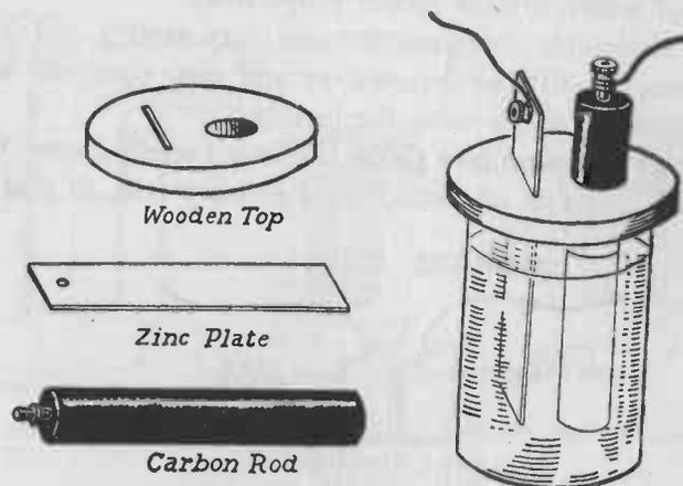
FIG. 220.—A homemade open-circuit cell using sal ammoniac solution as electrolyte is easily assembled from a strip of zinc, a carbon rod from an old dry cell and a paraffined wooden cover.
