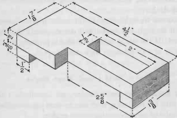
FIG. 151. — The wooden bed for the steam engine.
