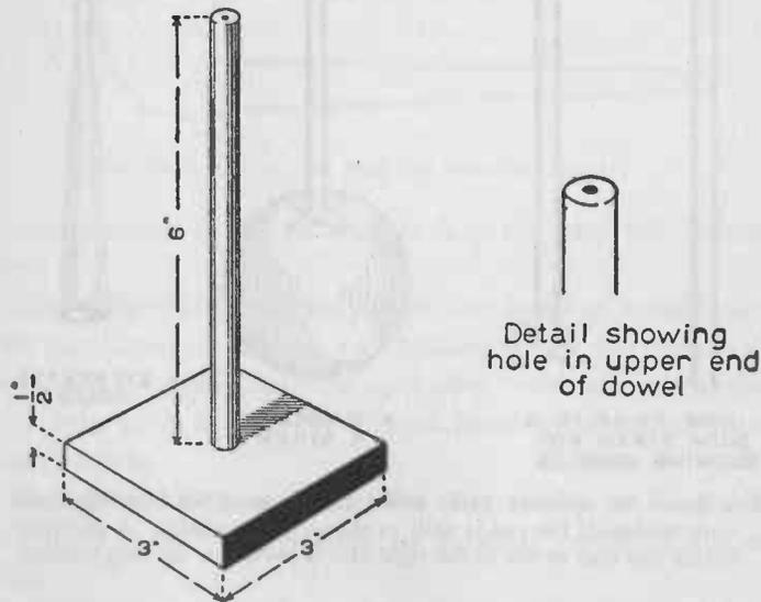
FIG. 82.— A stand made out of a square piece of wood and a dowel stick as shown in the illustration above is an important part of the apparatus needed for performing experiments described in this chapter.
