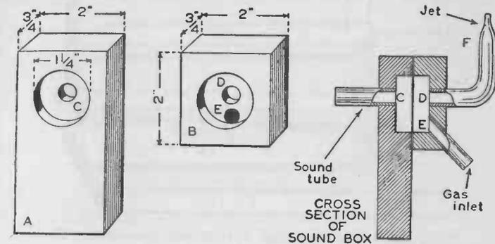
FIG. 117. — Details of the wooden sound box for producing manometric flames.
