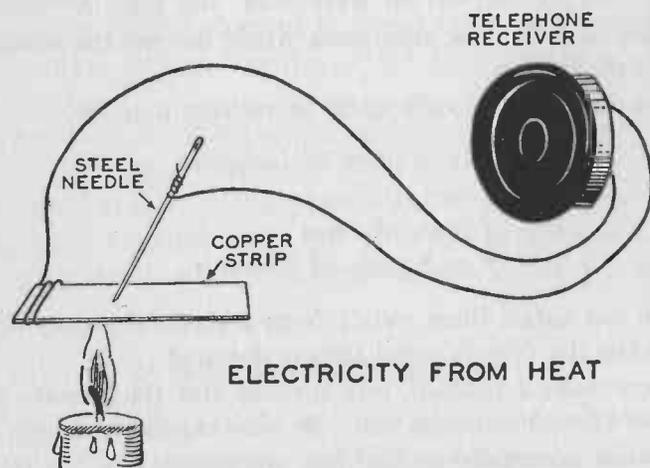
FIG. 143.—An experiment showing how electricity may be generated directly from heat.
