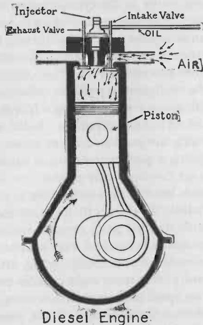
FIG. 158. — Diagram of a Diesel engine. Compare this with the gasoline engine shown in Fig. 157 and notice the absence of carburetor and spark plug.
