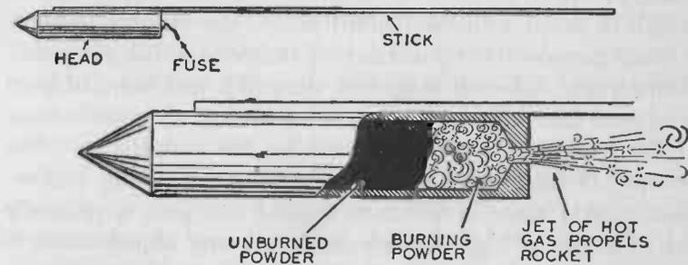
FIG. 72B.—The Skyrocket. In the enlarged view of the head the case is shown cut away to reveal the burning powder and the hot gases which form the jet.
