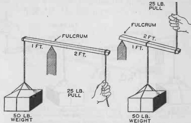
FIG. 42. — If a lever is arranged so that the distance from the fulcrum to the point where the power is applied is twice that between the fulcrum and the weight, the pull on the rope necessary to lift the object must be only slightly more than one-half the weight of the object to be lifted. A 25 lb. pull will lift a 50 lb. weight.
