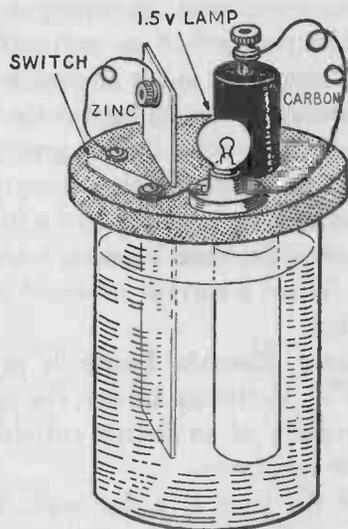
FIG. 231. — A simple homemade electric lamp.
