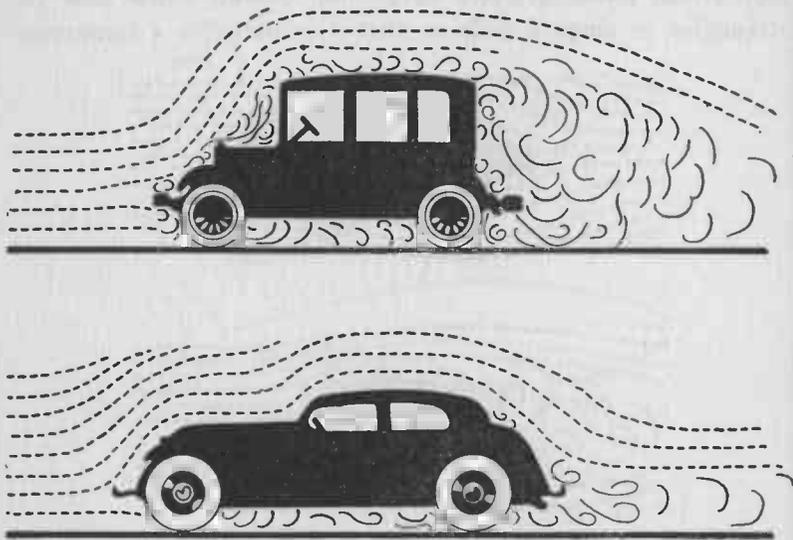
FIG. 72. — The disturbance created in the air by an old-fashioned automobile body is illustrated at the top. At the bottom is shown a modern streamlined automobile body and its effect in moving through the atmosphere.
