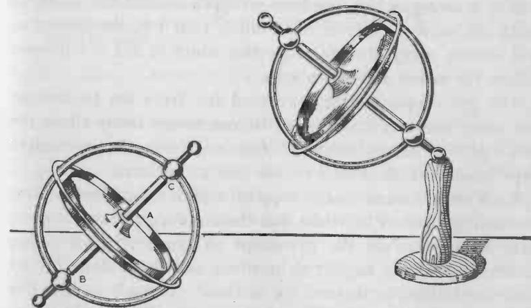
FIG. 62. — At the left is a toy gyroscope at rest. At the right, the same gyroscope is shown spinning on its stand.
