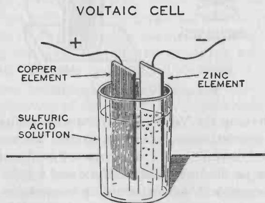
FIG. 218. — A simple Voltaic cell.
