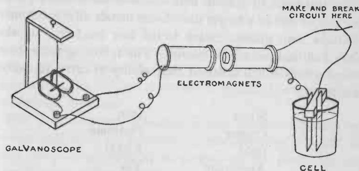
FIG. 230. — With this apparatus you can demonstrate the important principle of electromagnetic induction and also show that electricity can be produced by electromagnetism and motion.
