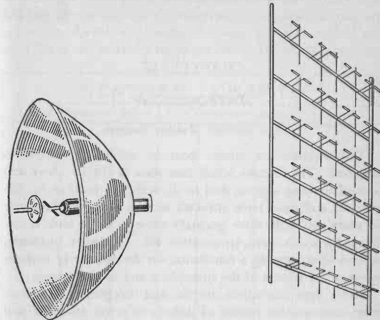
FIG. 251. — Radar Antennas. At the left is the parabolic reflector type and at the right a "bedspring" antenna.
