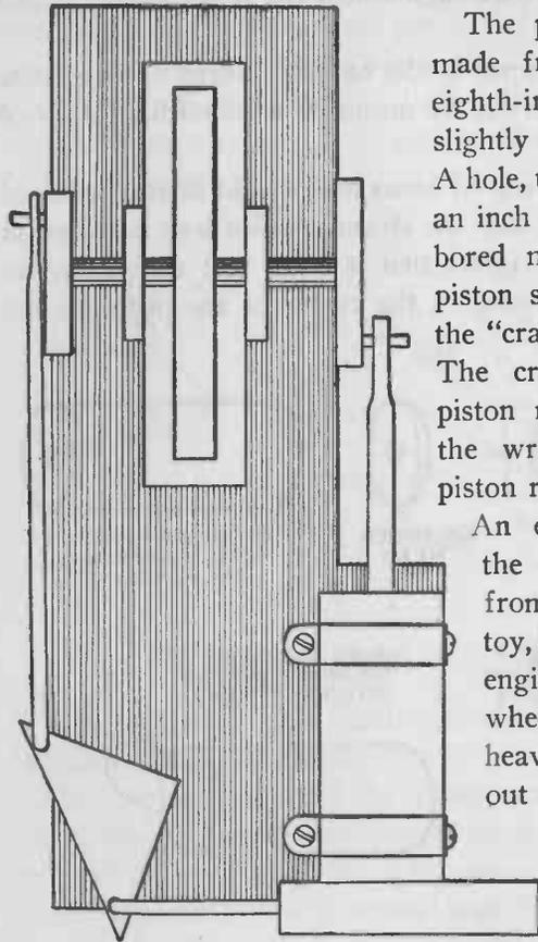
FIG. 153.—A full-size top view of the complete engine.
