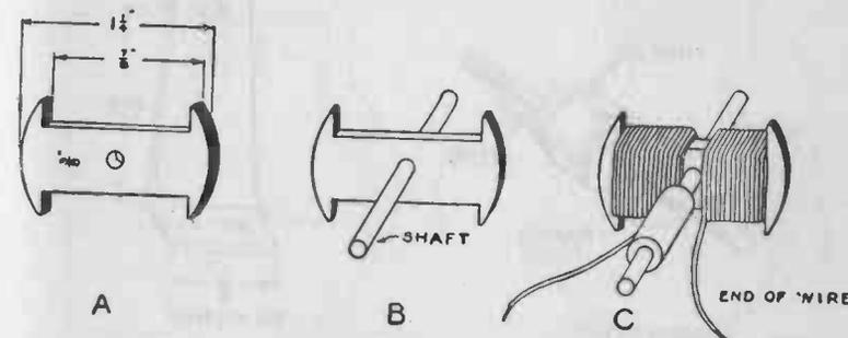
FIG. 234. — Details of the armature.
