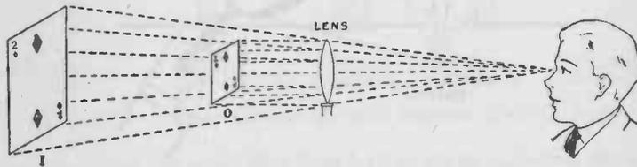
FIG. 167.—This diagram shows how a magnifying glass makes an object appear larger than it really is. The card I is the magnified image. O is the actual card.
