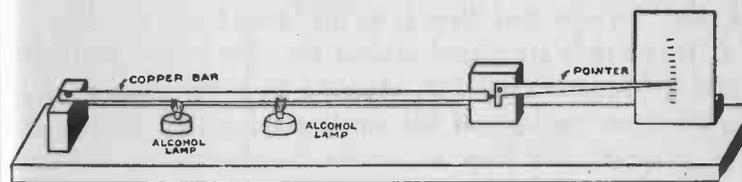
FIG. 141. — Simple apparatus for showing the expansion of a copper rod when it is heated.
