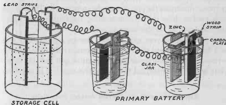
FIG. 222.—Charging the experimental storage cell with the current from two homemade cells.
