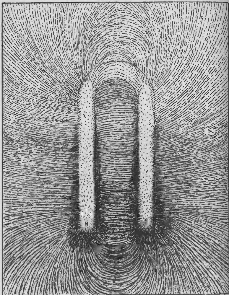
FIG. 215.— The phantom of a horseshoe magnet. The method of making a magnetic phantom is explained in the text.
