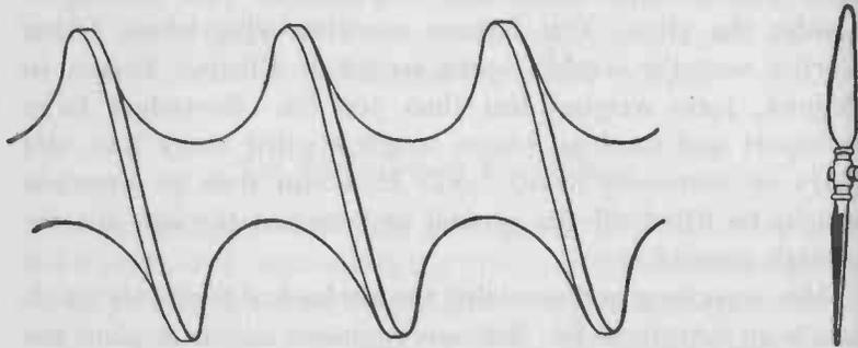
FIG. 69.— The airplane propeller shown at the right is in effect a huge screw such as that shown at the left. It “bores” its way into the air.
