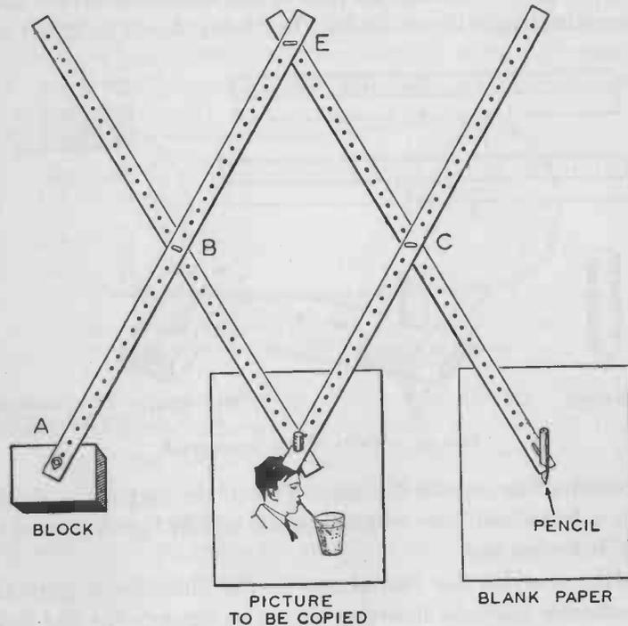
FIG. 50. — The completed pantograph.
