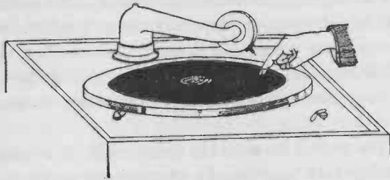
FIG. 126. — A simple experiment which shows that there is really no mystery about a talking machine. If you hold your finger nail in the sound track on a revolving phonograph record your finger nail will vibrate and reproduce the sounds recorded on the record.
