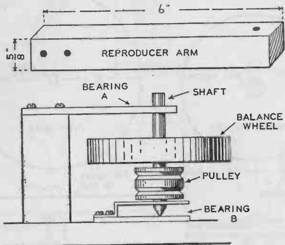
FIG. 130.—The arm which supports the reproducer is shown in the upper part of the illustration. The lower sketch shows the balance wheel and its pulleys.
