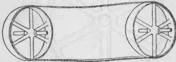
FIG. 48.— Power transmission pulleys are in effect gears which are coupled together by a belt or chain.
