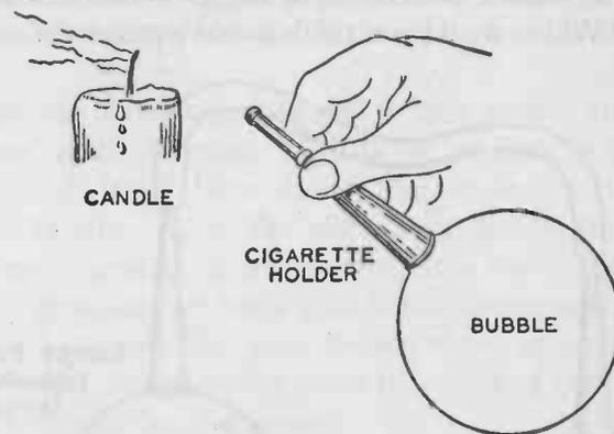
FIG. 84. — The elastic nature of a soap-bubble slightly compresses the air within the bubble. The pressure of the air will cause it to rush out through the cigarette holder with enough force to blow out a candle flame.
