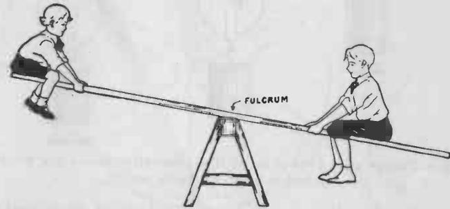
FIG. 44. — The seesaw is a form of lever. A light weight at one side will balance a much heavier weight on the other side if the lighter weight is farther away from the fulcrum.
