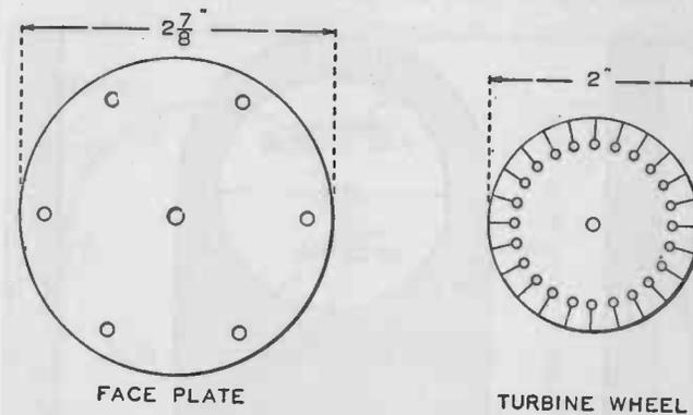
FIG. 148. — The turbine wheel and the face plate.
