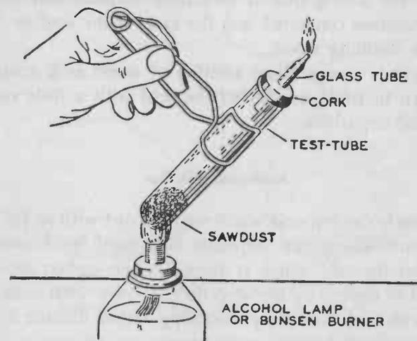
FIG. 28. — If you proceed as in the coal-gas experiment but use wood shavings or sawdust in the test-tube instead of soft coal, you can demonstrate the process of manufacturing wood alcohol.
