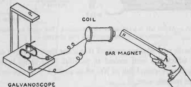
FIG. 229. — An experiment which shows how electricity can be generated by magnetism and motion.
