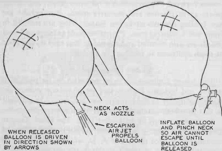
FIG. 72A.—A Toy Balloon Demonstrates the Reaction of a Jet and the Force that Drives a Rocket.
