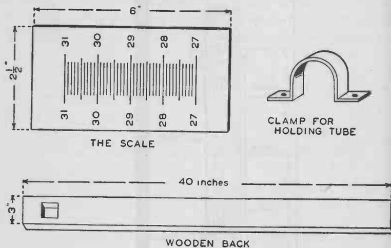
FIG. 288. — The wooden back, scale and clamp for the mercurial barometer.
