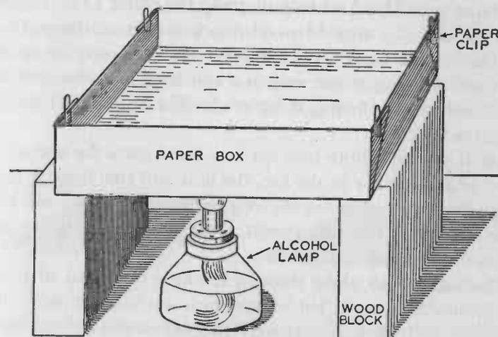
FIG. 135.— Water may be boiled in a paper box over the flame of an alcohol lamp or a Bunsen burner. The water draws the heat away from the paper so rapidly that it cannot become hot enough to ignite and burn until the water has boiled away.
