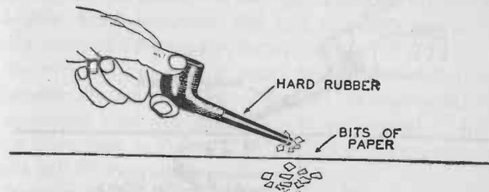
FIG. 204. — Rubbing a hard rubber pipe-stem with a piece of flannel will electrify the rubber so that it will attract small bits of paper.
