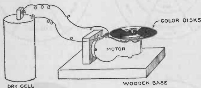
FIG. 173.—The color top for mixing colors.
