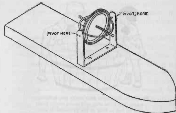
FIG. 67. — A model boat fitted with a toy gyroscope to show the stabilizing effect of its spinning wheel.
