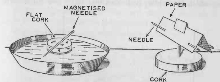
FIG. 212. — A magnetised needle lying on a cork floating in a saucer of water will come to rest in a north and south position. Another method of making a simple compass is illustrated in the right-hand sketch.
