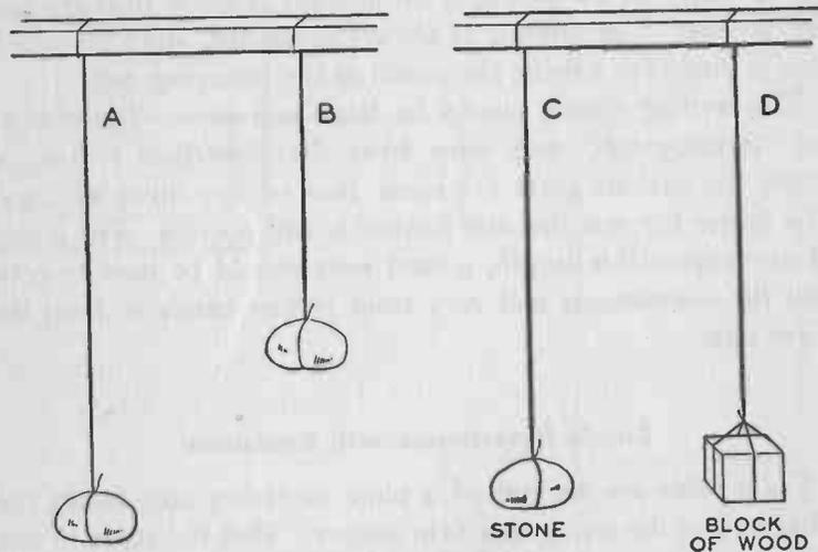
FIG. 56. — A is a simple pendulum consisting of a stone tied to a string. B is a pendulum of the same kind as A but has a shorter string. C and D are pendulums of exactly the same length. The weight used on C is a stone. The weight used on D is a block of light wood weighing less than the stone.
