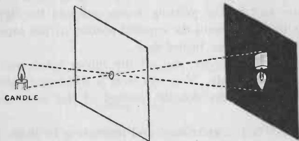
FIG. 176. — The image of a candle flame may be produced on a screen by letting light rays pass through a small hole in a piece of cardboard.
