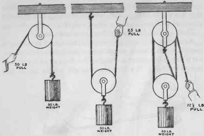
FIG. 45. — Pulleys are a form of lever. The illustration shows how much pull is required to balance a 50 lb. weight.
