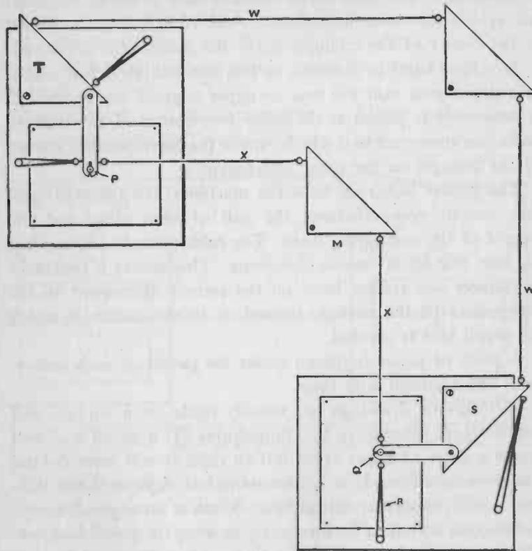
FIG. 55. — The wires or strings, *W* and *X*, connecting the telautographs can be made to turn a corner by utilizing two "bell cranks" as shown above.
