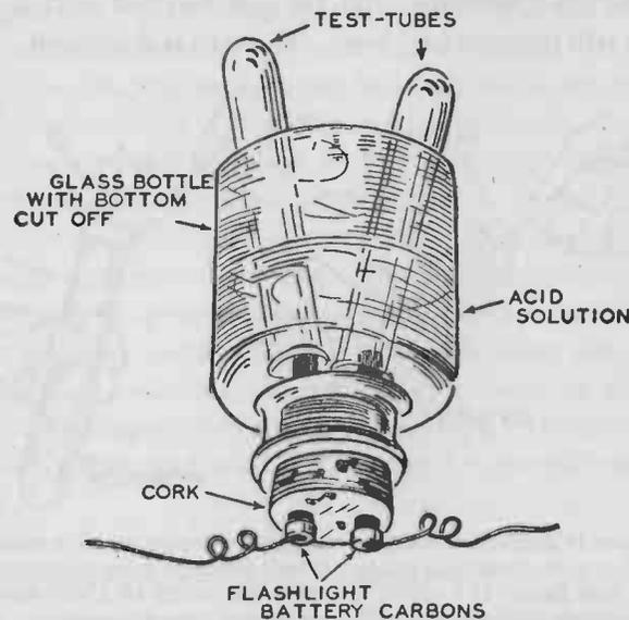
FIG. 10.— A simple apparatus for proving that water is composed of oxygen and hydrogen. It consists of a bottle with the bottom broken out and provided with a cork fitted snugly into the neck. Two carbon rods connected to two dry cells pass through the cork. When current passes through the acid solution in the bottle, the water is decomposed into oxygen and hydrogen.
