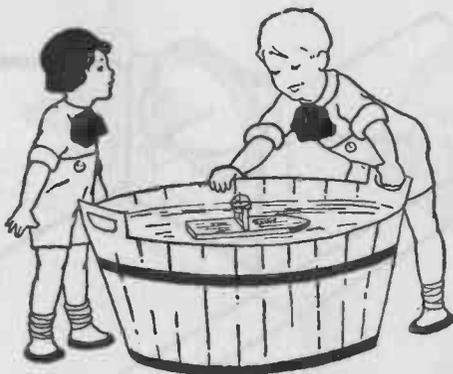
FIG. 68. — No matter how rough you make the water, the little ship will resist every tendency to roll as long as the gyroscope is spinning.
