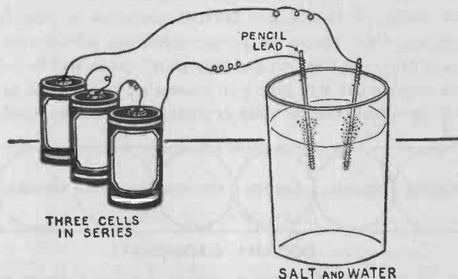
FIG. 17. — Experimental apparatus for decomposing a solution of salt water and showing how caustic soda, etc., are manufactured commercially.
