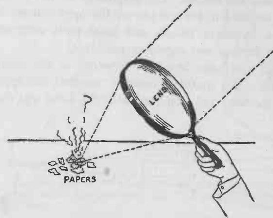
FIG. 166.—If a magnifying glass is held in the strong sunlight at the proper distance above a few scraps of paper, the paper will commence to smolder and soon catch fire. The lens bend the sun's rays and concentrate them at a point called the focus.
