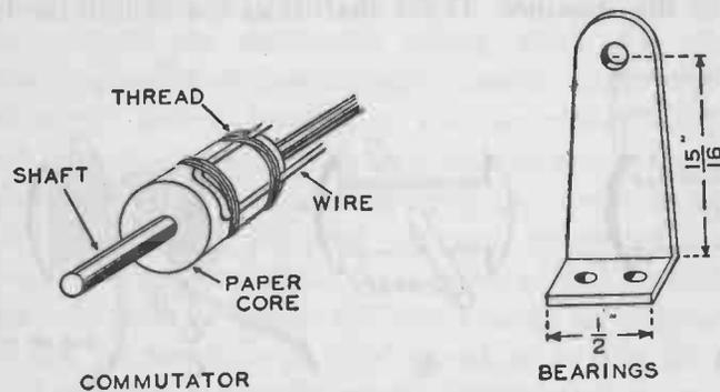
FIG. 235. — The commutator is formed by bending the ends of the armature wires and binding them in position on the paper core. The bearings are made according to the shape and dimensions shown above.
