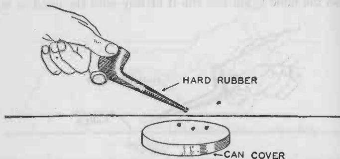
FIG. 205. — The apparatus used in the experiment illustrated above comprises an electrified pipe-stem, can cover, and some fragments of charcoal from a burnt match. The experiment shows the repulsion which takes place between two objects charged with the same kind of electricity.
