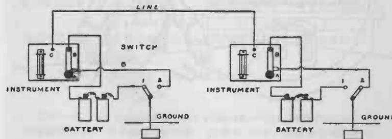
FIG. 242. — The circuit diagram for connecting two telegraph instruments.
