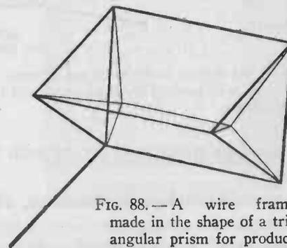
FIG. 88.—A wire frame made in the shape of a triangular prism for producing soap films.
