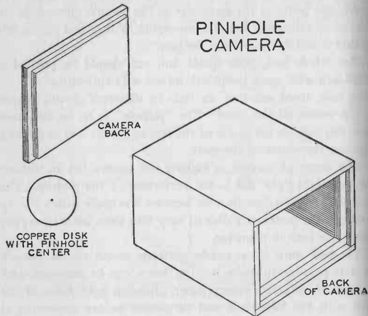
FIG. 180. — Details of the pinhole camera.
