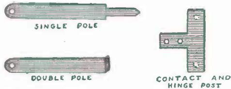
FIG. 97. — Metal Parts for the Knife Switches.
