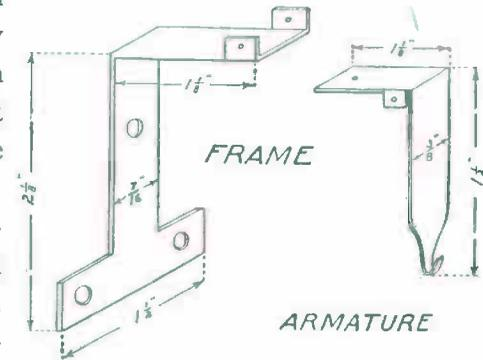
FIG. 129. — Details of the Drop-Frame and Armature.
