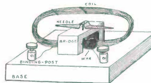
FIG. 111. — Galvanoscope.
