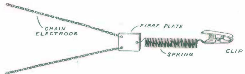
FIG. 127. — Details of the Chain Electrodes, etc.
