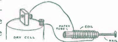
FIG. 85. — If you wind the Wire around a small Paper Tube into which a Nail will slide easily, the Coil will draw the Nail in when the Current is turned on.
