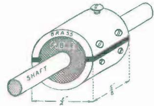
FIG. 257. — Details of the Commutator.
