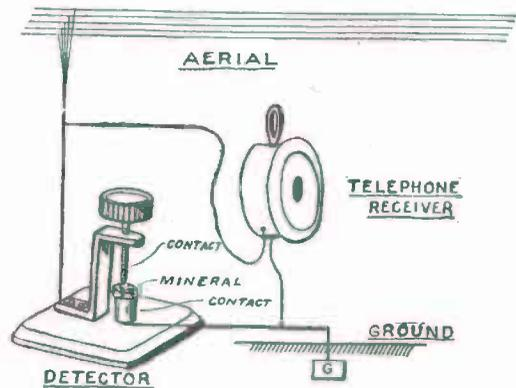
FIG. 195. — A Simple Receptor.
