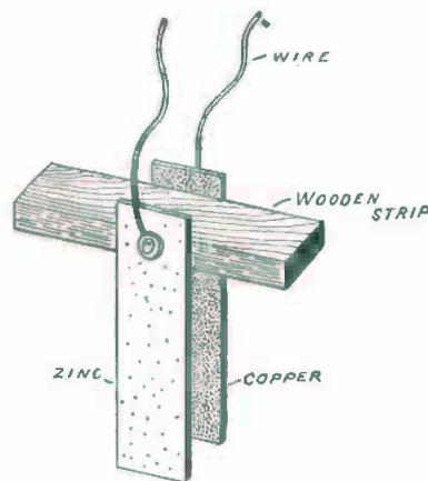
FIG. 53. — The Elements of Simple Voltaic Cell.
