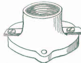
FIG. 310. — A Socket for holding the Lamp.
