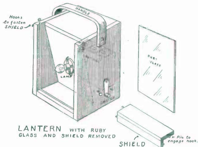
LANTERN WITH RUBY GLASS AND SHIELD REMOVED
