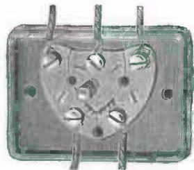
FIG. 99. — Lightning-Arrester and Ground-Wire Switch.
