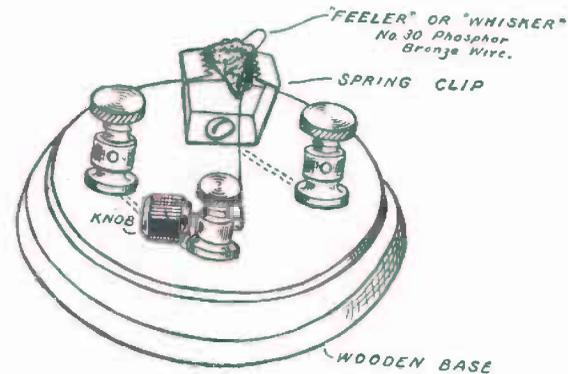
FIG. 212. — Details of the "Cat-Whisker" Detector.
