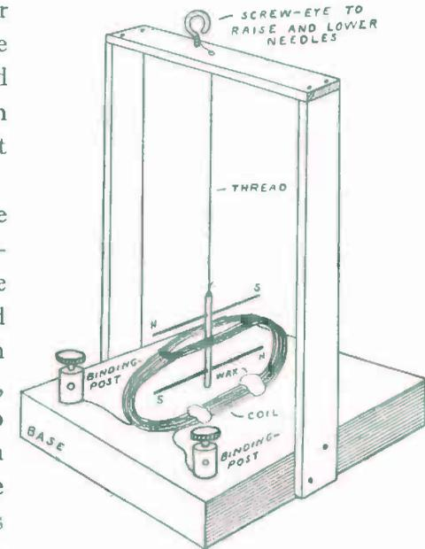
FIG. 112. — Astatic Galvanoscope.
