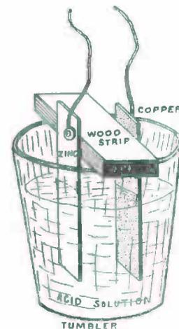
FIG. 54. — A Home-Made Voltaic Cell.
