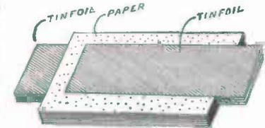
FIG. 215. — Building up a Fixed Condenser.
