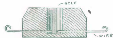
FIG. 46. — A Wooden Mortar for Igniting Gunpowder.
