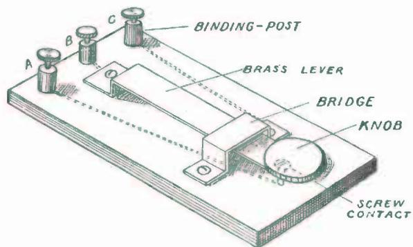
FIG. 132. — A Simple Home-made Telegraph Key.
