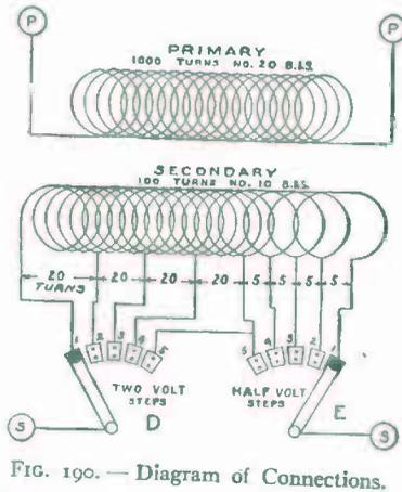
FIG. 190. — Diagram of Connections.
