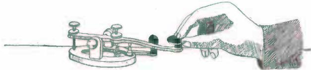
FIG. 141. — How to hold a Telegraph Key.
