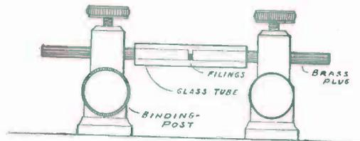
FIG. 234. — Details of the Coherer.
