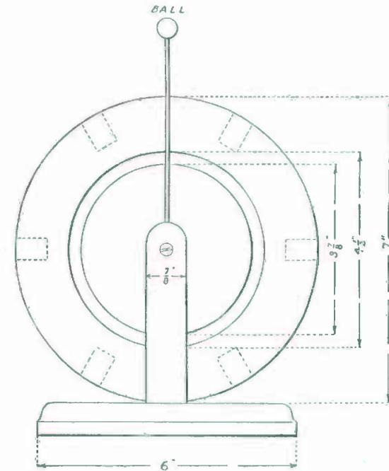
FIG. 321. — End View of the Complete Tesla Coil.
