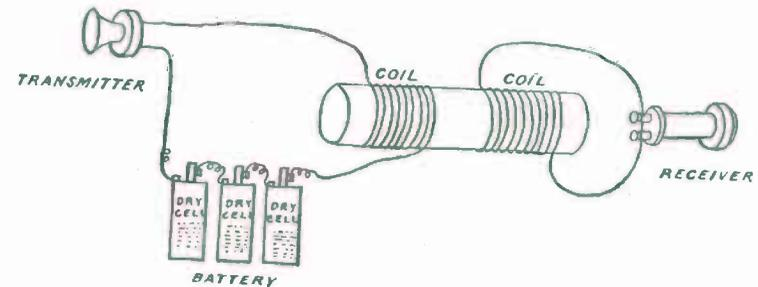
FIG. 238.—A Simple Wireless Telephone.
