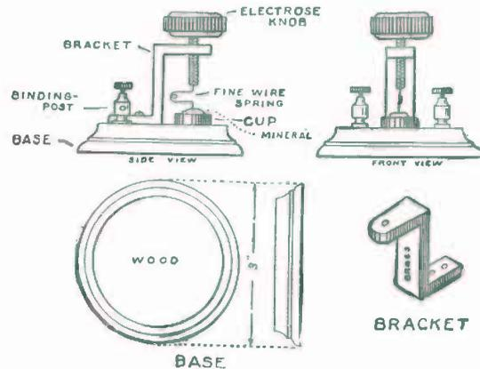
FIG. 211. — Details of the Crystal Detector.
