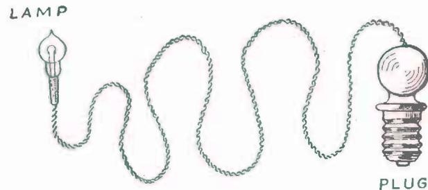
FIG. 300. — A "Pea" Lamp attached to a Flexible Wire and a Plug.
