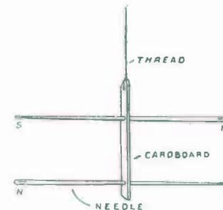
FIG. 113. — Astatic Needles.
