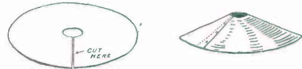
FIG. 293.— How the Reflector is made.
