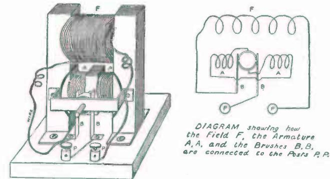
FIG. 250. — Complete Motor.
