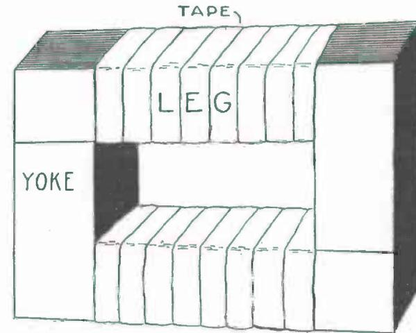
FIG. 181.—The Core, Assembled and Taped.
