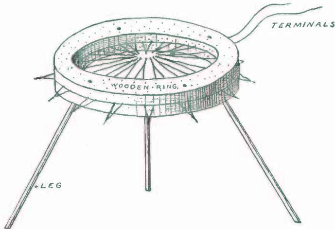
FIG. 305. — Complete Thermopile.
