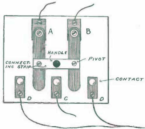
FIG. 315. — A Pole-Changing Switch or Current Reverser.
