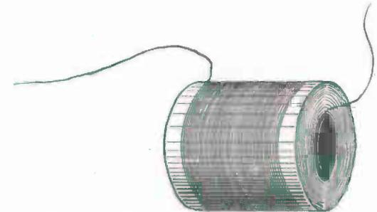
FIG. 163. — Completed Secondary Winding.
