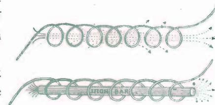
FIG. 82. — Showing how the Lines of Force "Leak" from a Coil of Wire, and how they are concentrated by an Iron Core.
