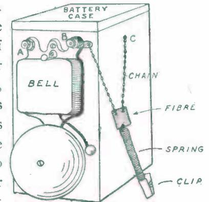
FIG. 126. — An Early-Riser's Electric Alarm Attachment for a Clock.
