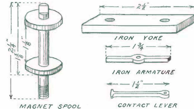
FIG. 138. — Details of the Relay Parts.
