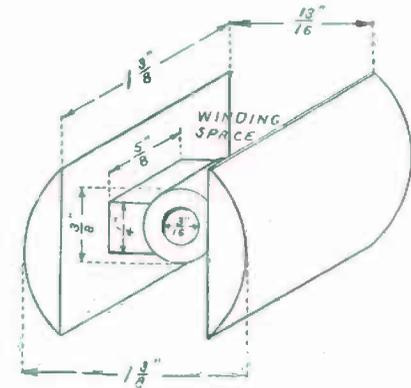
FIG. 256. — Details of the Armature Casting.
