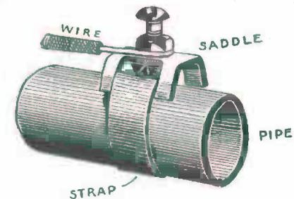
FIG. 200. — A Ground Clamp for Pipes.
