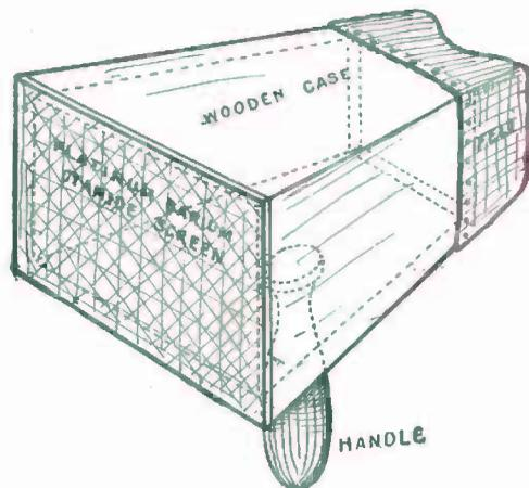
FIG. 173. — Fluoroscope.
