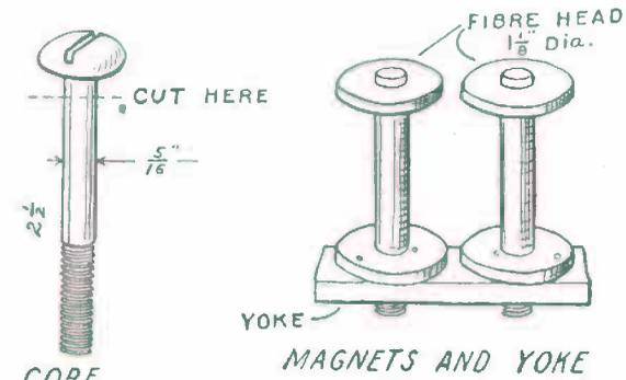
FIG. 119. — Details of the Magnet Spools, and Yoke for an Electric Bell.
