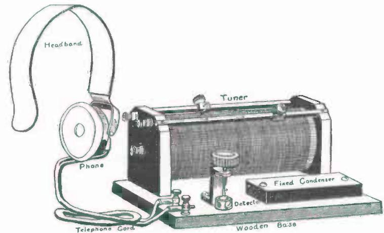
FIG. 316. — A Complete Wireless Receiving Outfit.
