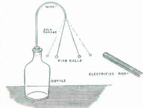
FIG. 23. — A Double Pith-Ball Electroscope.
