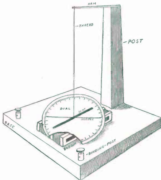
FIG. 115. — Completed Astatic Galvanometer.
