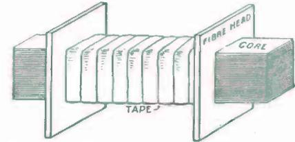
FIG. 184. — Leg with Heads in Position for Winding.
