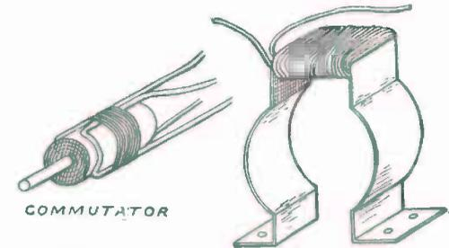
FIG. 246. — The Field and Commutator.
