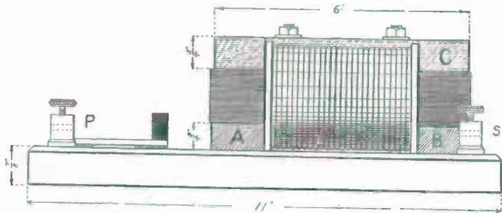
FIG. 192. — Side View of the Transformer.
