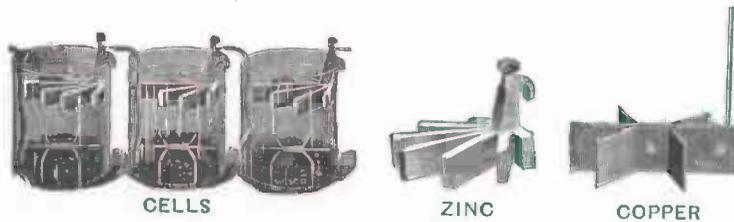
FIG. 75. — Gravity Cells.
