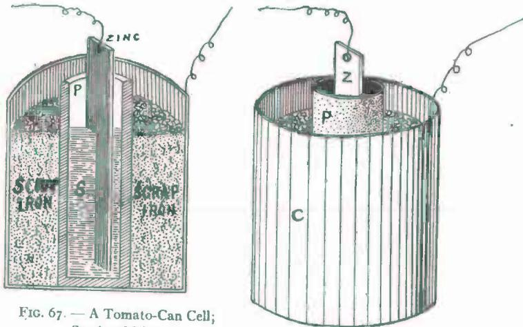
FIG. 67. — A Tomato-Can Cell; Sectional View.
