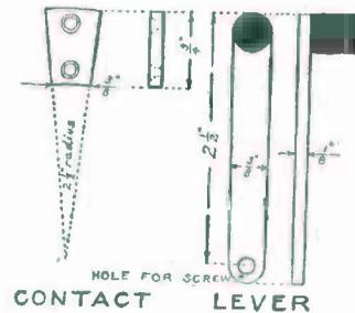
FIG. 188. — Details of the Switch Parts.
