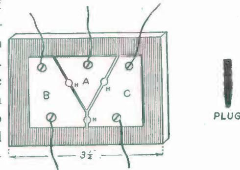
FIG. 100. — Home-made Lightning-Arrester.
