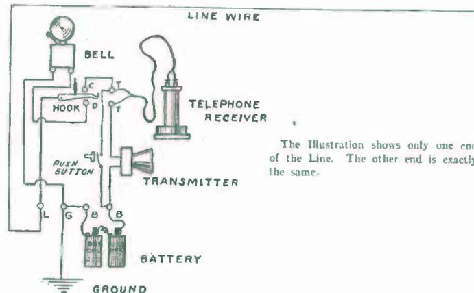
The illustration shows only one end of the Line. The other end is exactly the same.
