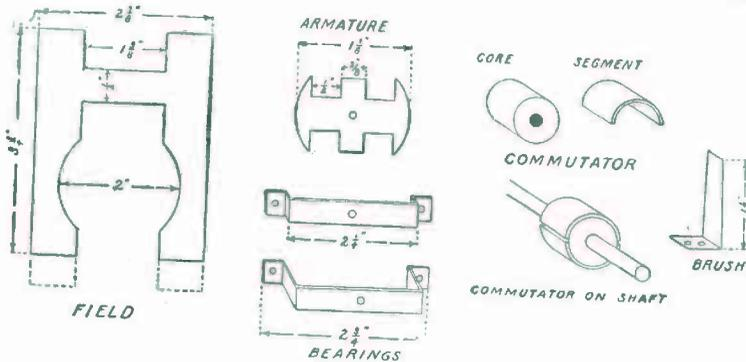
FIG. 249. — Details of the Motor.
