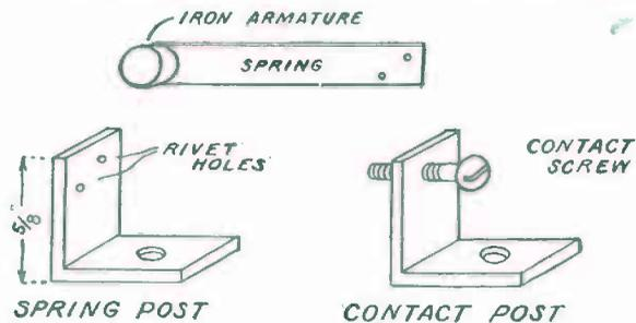
FIG. 155. — Details of Interrupter for Medical Coil.
