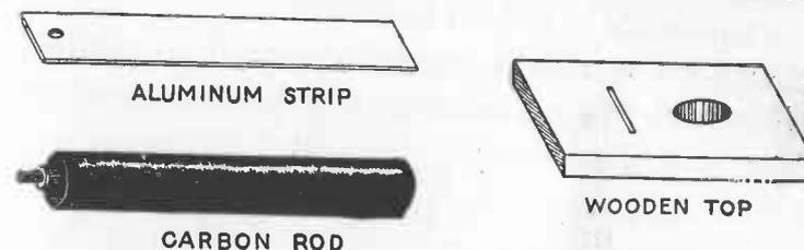
PARTS FOR AN ELECTROLYTIC RECTIFIER CELL
