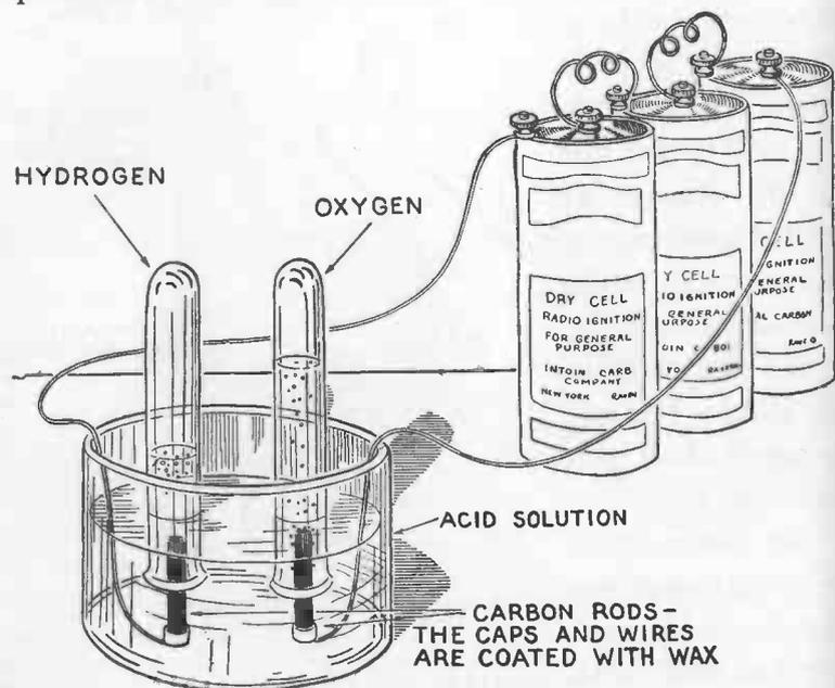
Another arrangement for producing oxygen and hydrogen from water.
