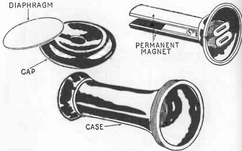
THE PARTS OF A TELEPHONE RECEIVER
