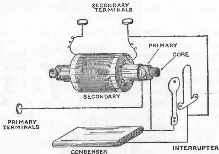
INSIDE THE MODEL "T" SPARK COIL
