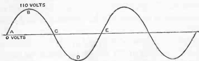
A PICTURE OF A SINGLE-PHASE ALTERNATING CURRENT
