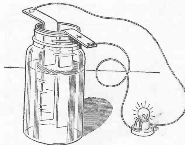
The current from the dry battery has changed the two strips of lead into the plates of a storage cell. The cell will light a small lamp, ring a bell, etc.
