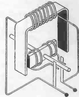
The field of a shunt motor is wound with more turns and with finer wire than a series motor of the same size. It is connected so that part of the current goes through the field and part through the armature. In a series motor all of the current that goes through the field also passes through the armature.
