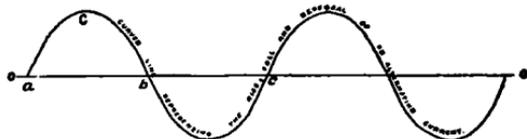
FIG. 41.—Diagram representing alternating current.
