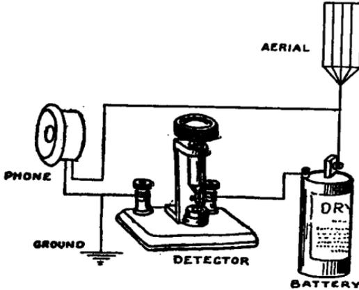
FIG. 73.—Electrolytic detector in circuit.
