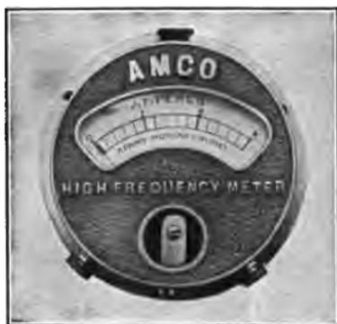
FIG. 88.—Hot-wire ammeter.
