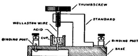
FIG. 72.—Electrolytic detector.
