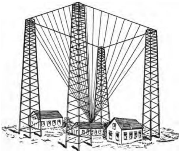
FIG. 16.—A diagram showing pyramid aerial.
