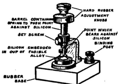
FIG. 71.—Silicon detector.
