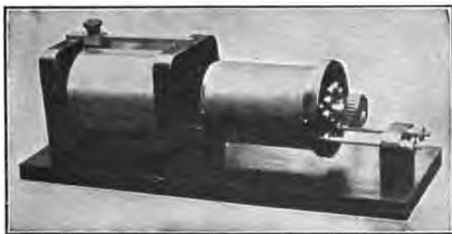
FIG. 92.—Loose coupled tuner.
