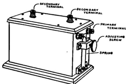
FIG. 35.—Induction coil for wireless telegraph purposes.
