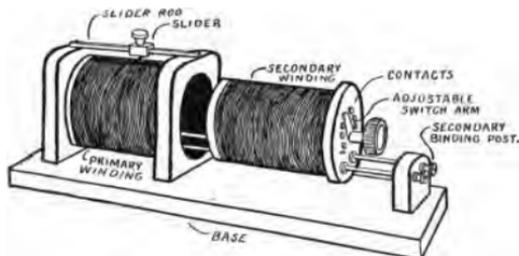
FIG. 91.—Loose coupled tuning coil.
