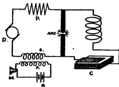
FIG. 145.—Arrangement of the speaking arc.
