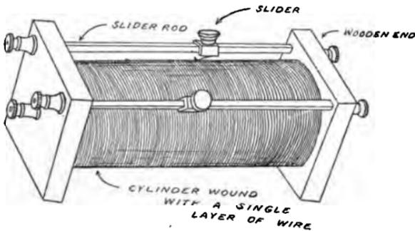
FIG. 78.—Tuning coil of the double slide type.
