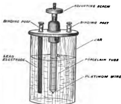
FIG. 38.—Electrolytic interrupter.
