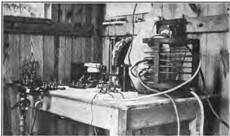
FIG. 150.—An amateur wireless telegraph station.
