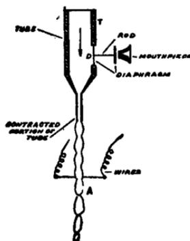
FIG. 148.—The Majorana wireless telephone transmitter.
