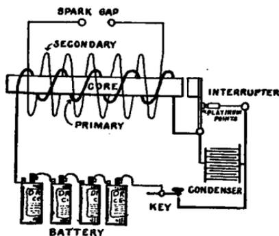
FIG. 34.—Diagram of induction coil.
