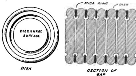
FIG. 53.—Quenched spark gap.
