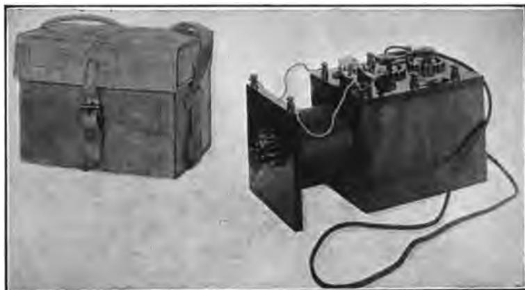
FIG. 60.—Portable receiving set and case.
