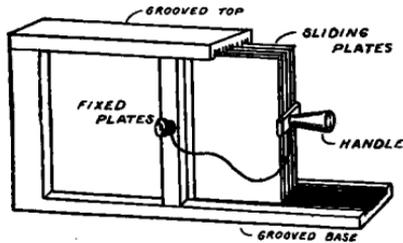
FIG. 84.—Sliding plate variable condenser.
