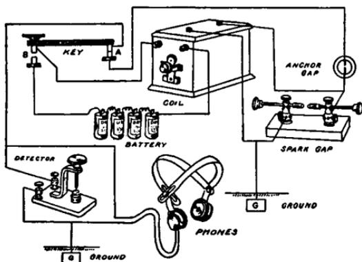
FIG. 118.—Breaking-in system.
