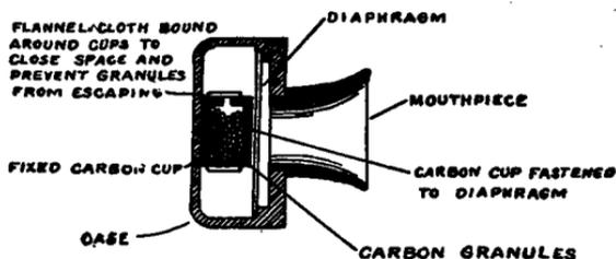
FIG. 131.—Diagram of a telephone transmitter.
