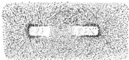
FIG. 31.—Magnetic phantom formed by bar magnet.
