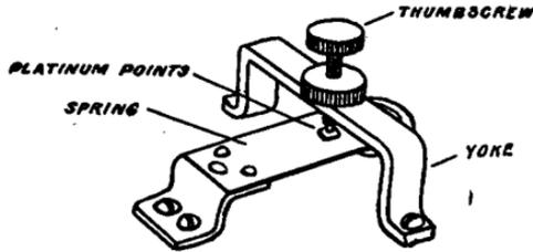
FIG. 37.—Interrupter for induction coil.
