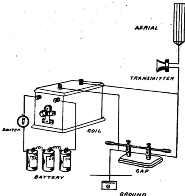
FIG. 139.—A "logical" form of wireless telephone which is impracticable.
