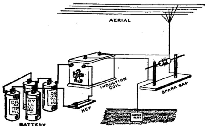
FIG. 7.—The simplest practical transmitter that it is possible to devise for the purpose of sending messages.
