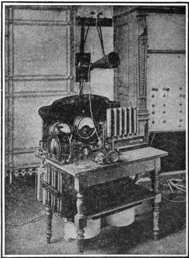
FIG. 147.—Poulsen wireless telephone equipment.
