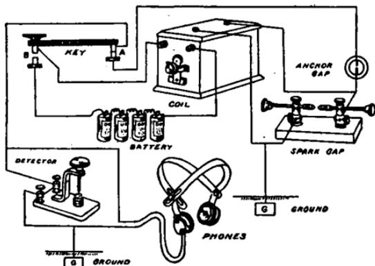
FIG. 118.—Breaking-in system.
