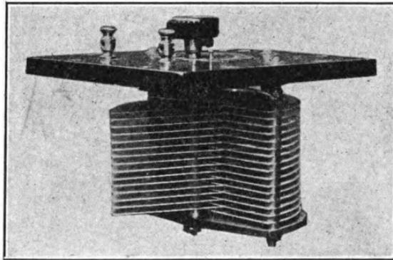
FIG. 82.—Interior of rotary variable condenser showing construction.
