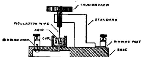
FIG. 72.—Electrolytic detector.
