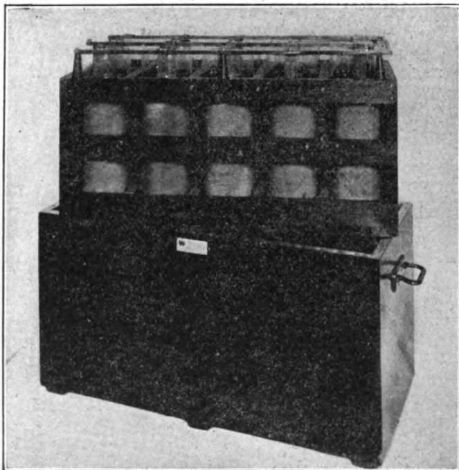
FIG. 44.—Leyden jar set for oil immersion to prevent losses from brush discharges.
