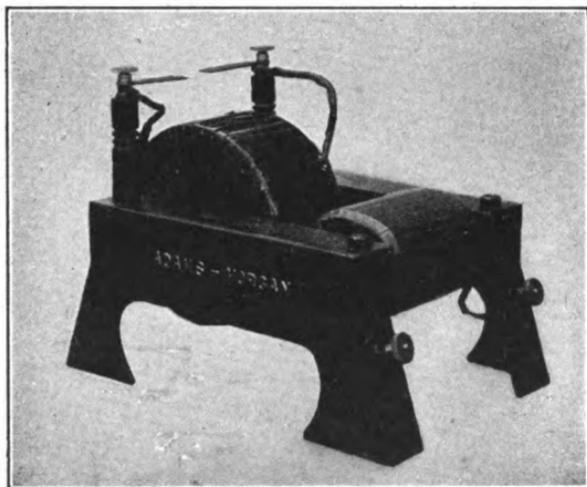
FIG. 43.—High potential closed core transformer for wireless work.
