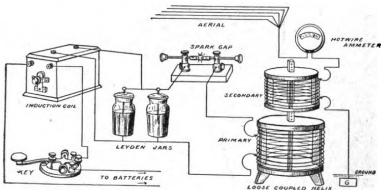
FIG. 90.—Diagram showing loose coupled helix in circuit.
