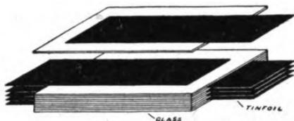
FIG. 46.—Diagram showing construction of condenser.
