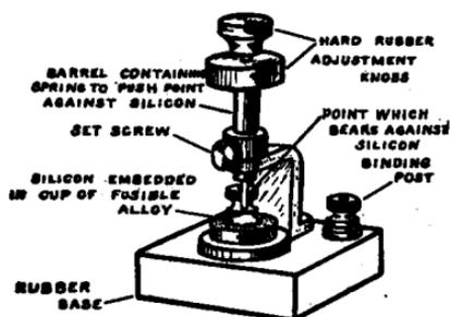
FIG. 71.—Silicon detector.
