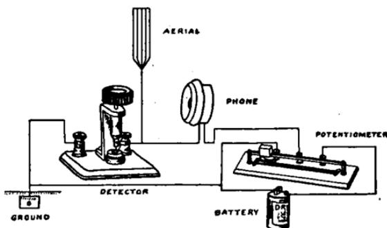
FIG. 75.—Diagram showing how potentiometer is connected in circuit.
