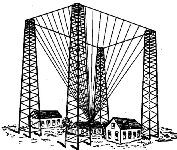
FIG. 16.—A diagram showing pyramid aerial.
