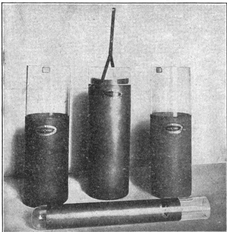
FIG. 6.—Navy type of Leyden jars. Coated with copper deposited upon the surface of the glass.
