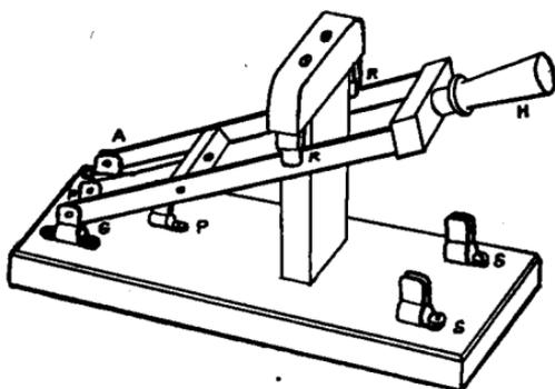
FIG. 54.—Diagram of aerial switch.
