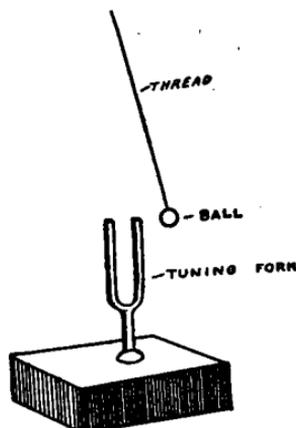
FIG. 123.—Experiment showing sounding bodies are in vibration.
