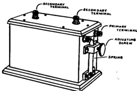
FIG. 35.—Induction coil for wireless telegraph purposes.
