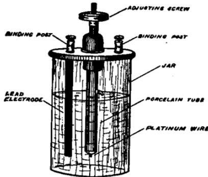
FIG. 38.—Electrolytic interrupter.
