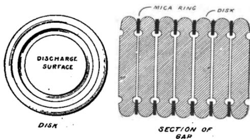
FIG. 53.—Quenched spark gap.
