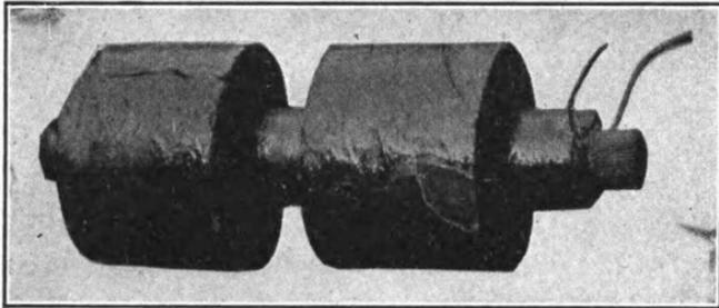
FIG. 36.—Induction coil, primary and secondary.
