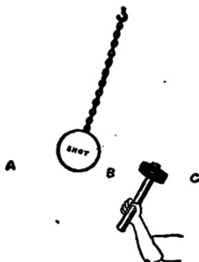
FIG. 86.—Chain and ball arranged to illustrate effect of tuning.
