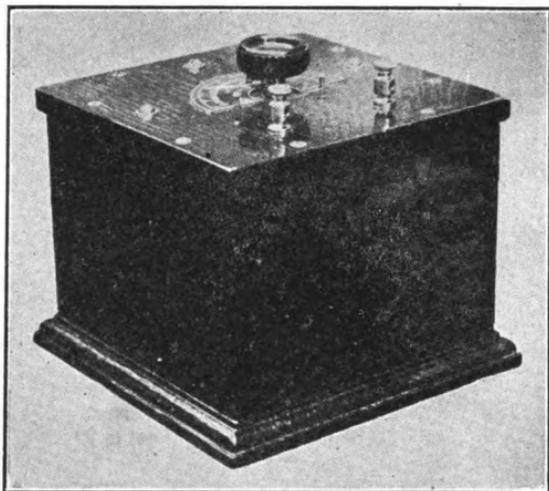
FIG. 81.—Rotary variable condenser.
