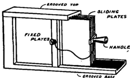
FIG. 84.—Sliding plate variable condenser.
