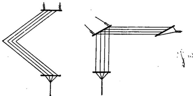
FIG. 18.—Aerials of the "V" and inverted "L" types.
