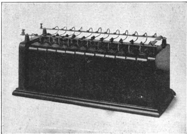
FIG. 95.—Transmitting condenser (molded dielectric).
