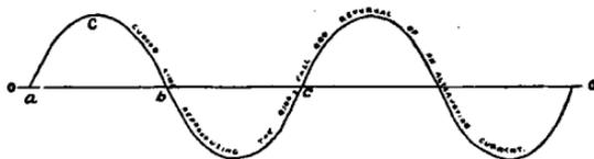
FIG. 41.—Diagram representing alternating current.
