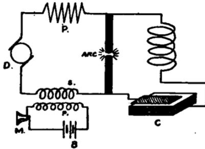
FIG. 145.—Arrangement of the speaking arc.
