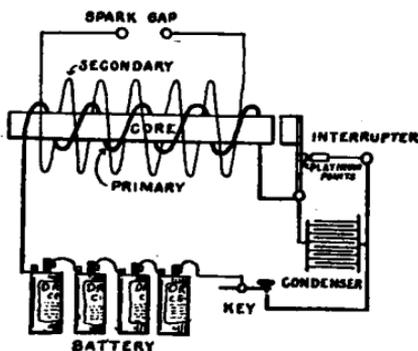
FIG. 34.—Diagram of induction coil.
