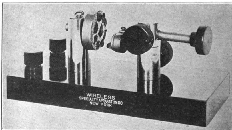
FIG. 67.—A new type of silicon detector in which a crystal of *arsenic* may be brought to bear against the surface of one of several *silicon* crystals.
