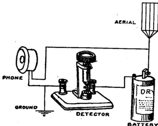
FIG. 73.—Electrolytic detector in circuit.
