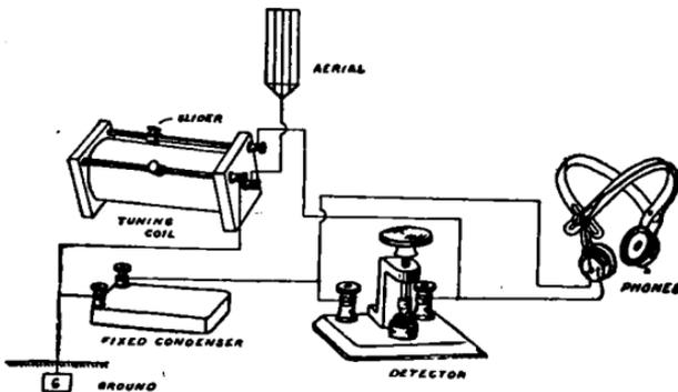
FIG. 79.—Diagram showing fixed condenser in circuit.
