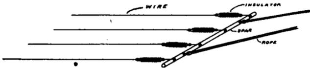
FIG. 24.—Showing how wires are arranged and insulated.
