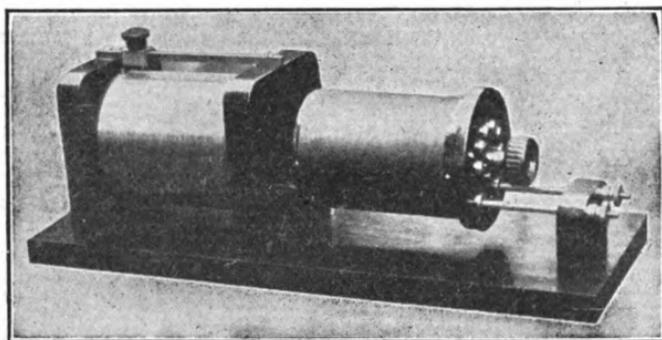
FIG. 92.—Loose coupled tuner.
