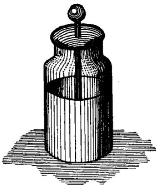
FIG. 2.—A Leyden jar is a glass jar lined inside and out with tinfoil for about two-thirds of its height.
