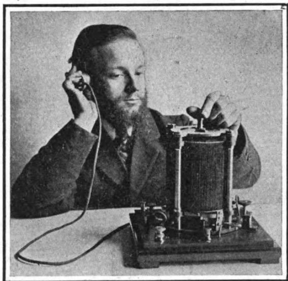
FIG. 97.—Bellini-Tosi radio-goniometer for directive wireless telegraphy.
