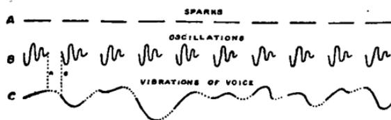
FIG. 143.—Diagram illustrating the reason why damped oscillations will not carry the voice.
