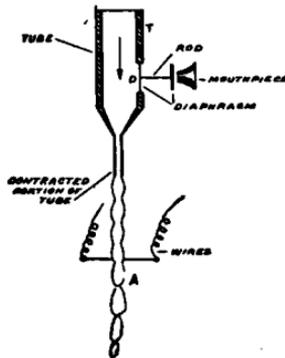
FIG. 148.—The Majorana wireless telephone transmitter.
