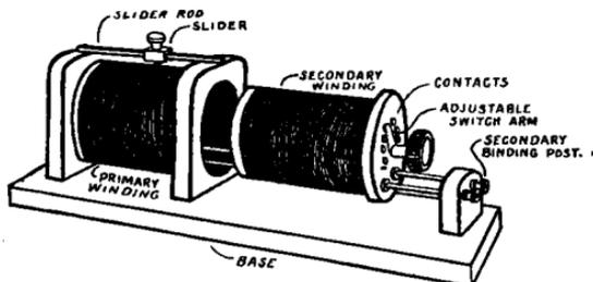
FIG. 91.—Loose coupled tuning coil.
