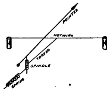
FIG. 89.—The principle of the hot-wire ammeter.
