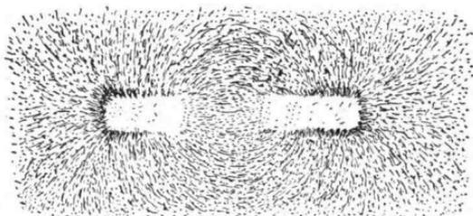
FIG. 31.—Magnetic phantom formed by bar magnet.
