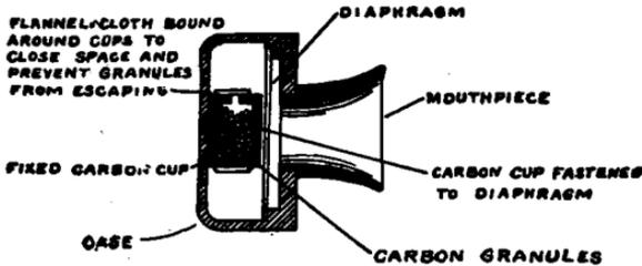
FIG. 131.—Diagram of a telephone transmitter.
