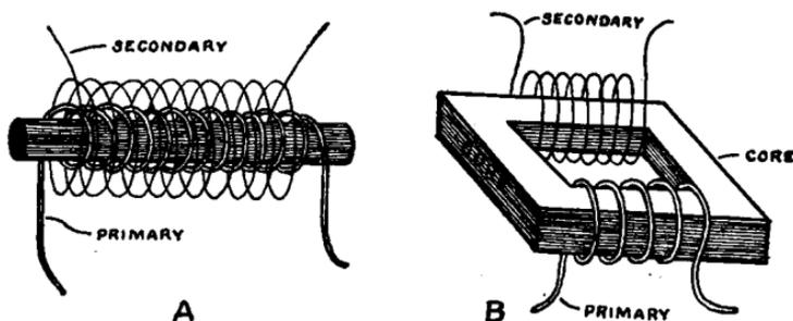
FIG. 39.—Open and closed core transformers.
