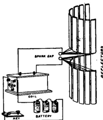
FIG. 96.—Braun's method for directing wireless telegraph signals.
