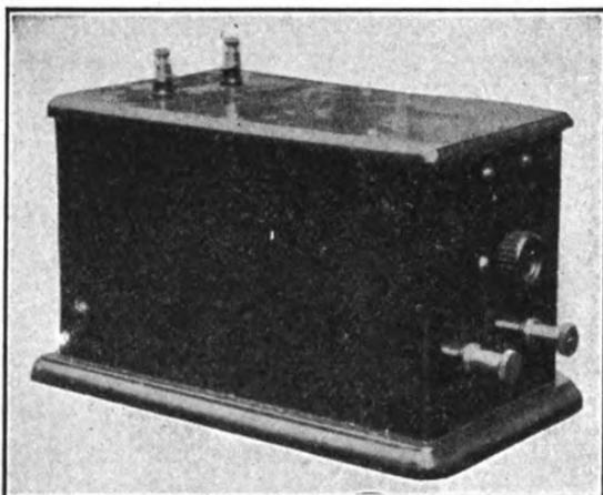
FIG. 42.—High potential “Humming” transformer.
