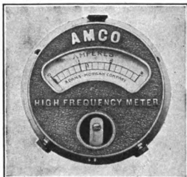
FIG. 88.—Hot-wire ammeter.
