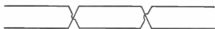
Fig. 1008 — Method of transposing a two-wire open transmission line to preserve balance to ground and nearby objects.
