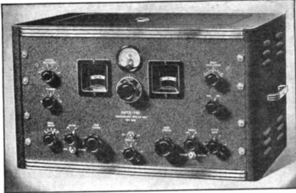
Fig. 1114 — The Hammarlund Super Pro 16-tube superheterodyne. The band-change switch is located between the two dial windows, just below the S meter.
